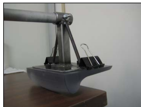
Figure 6. Wheel flangeway gap measurement instrument developed by TTCI
