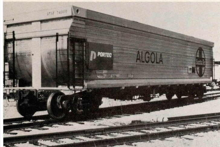
Portec's modified Algola car, now going into production for Santee Cooper, has end sheets that are rounded rather than vertical.
