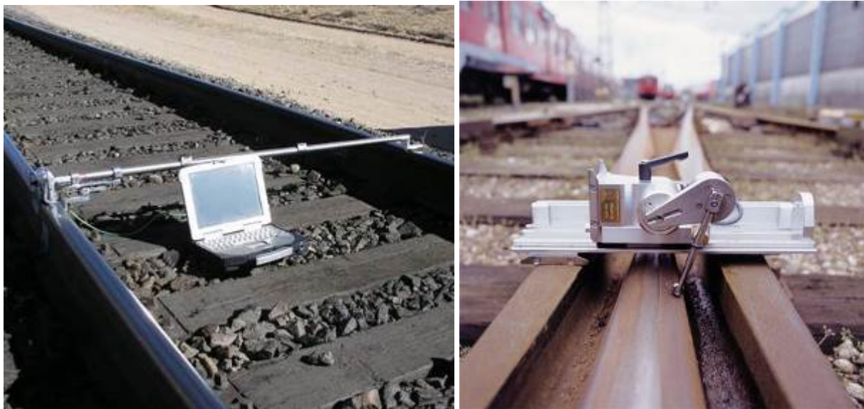
Figure 12. Photographs of MiniProf device ( www.railway-technology.com/contractors/track/greenwood )
