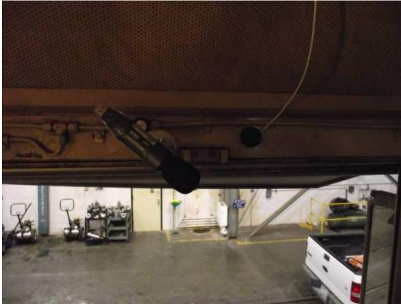
Figure 23. Remote SPL Logging Device (Conductor side)
