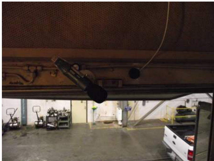
Figure 18. SPL Data Logger (conductor's side)
