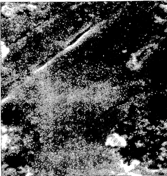
Fig. 15 Grain boundary openings on the fracture surface 11,000x.
