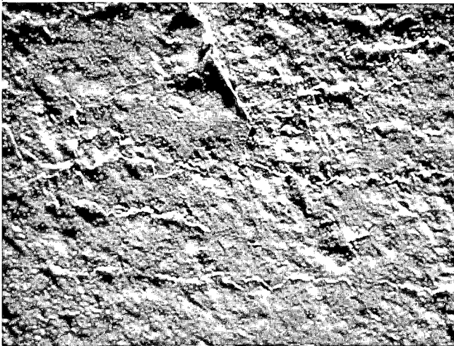
Fig. 11. SEM Photo (x 300) (the same as in Fig. 6 spot of the track) after running at .16 coefficient of friction.
