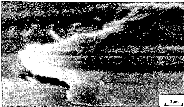
Initiation of delamination
