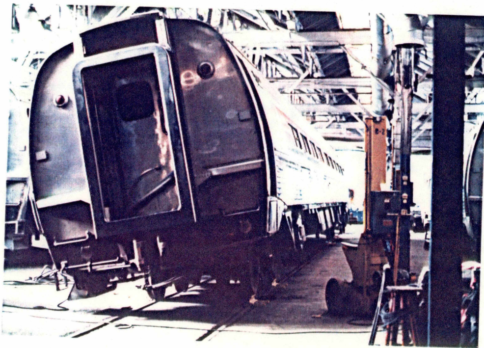
FIGURE 5-7: LEAN TEST - MEASUREMENT-PLUMP BOBS
