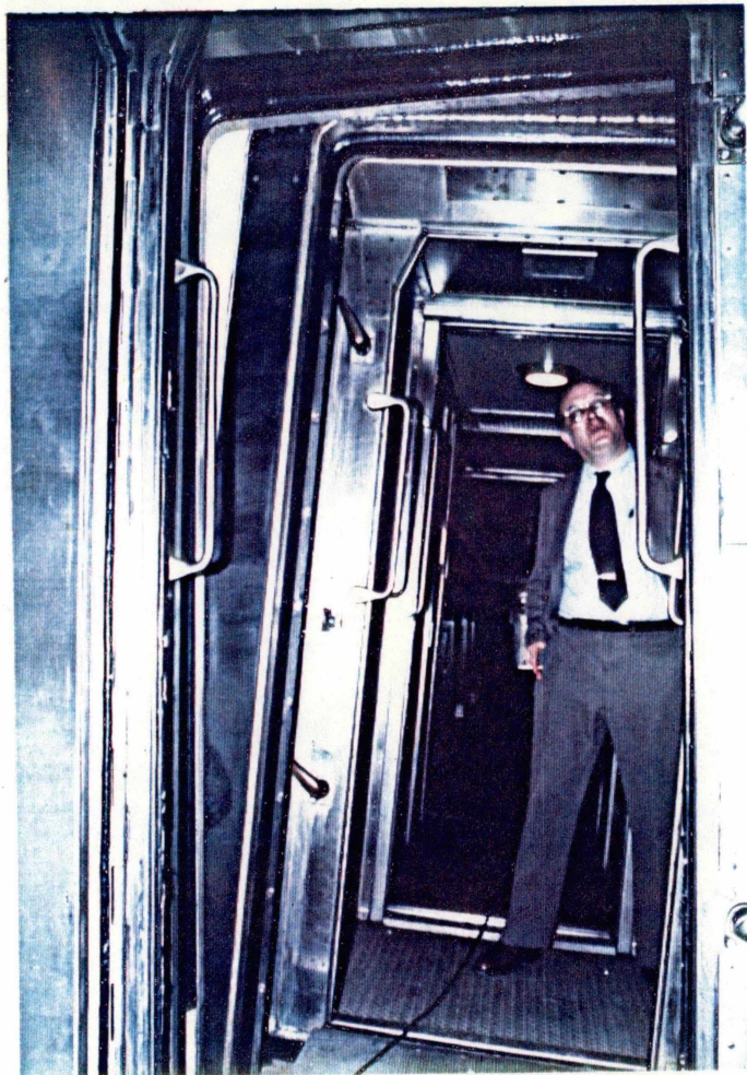
FIGURE 5-17: DIAPHRAM GAP BETWEEN TILTED AND STANDARD AMFLEET COACH .
