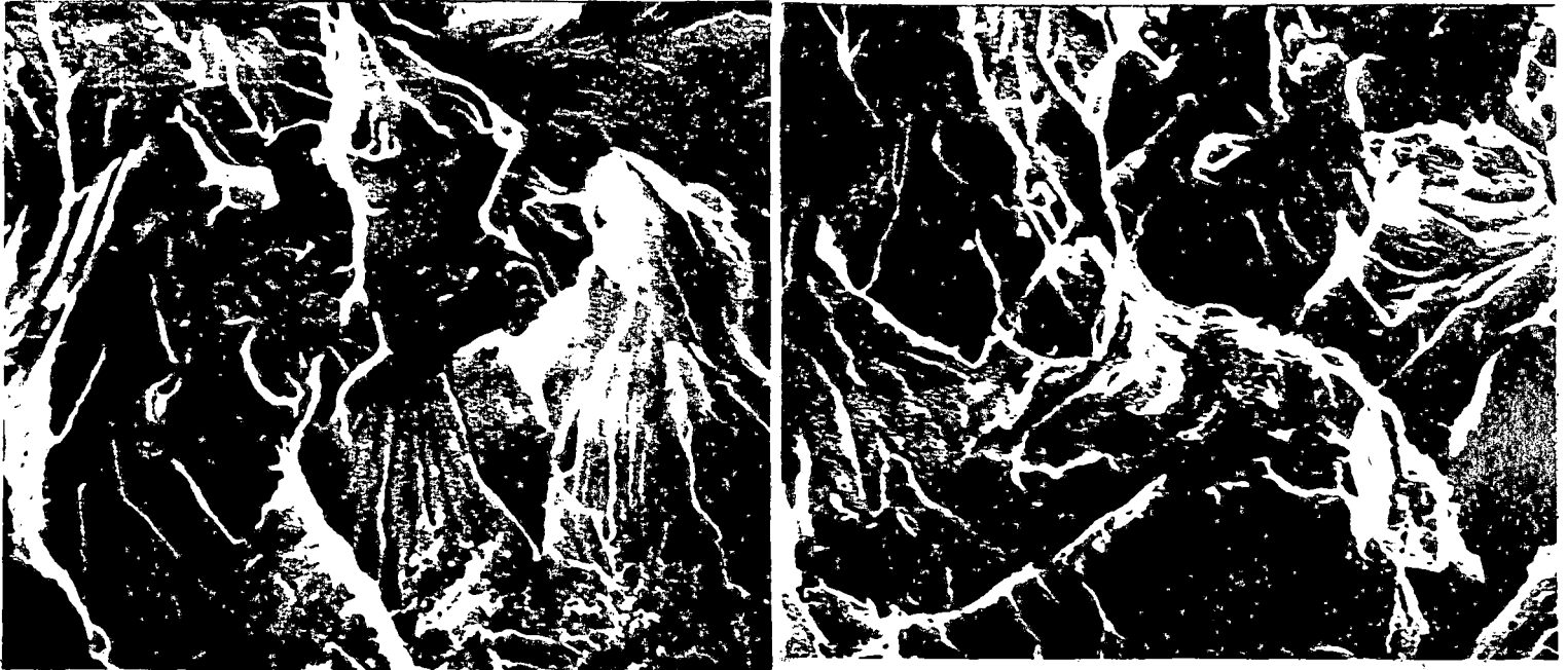
Figure 7. Fracture Surface of Class U Crack Arrest Specimen, Before (left) and After Crack Arrested; Mag. 500X.
