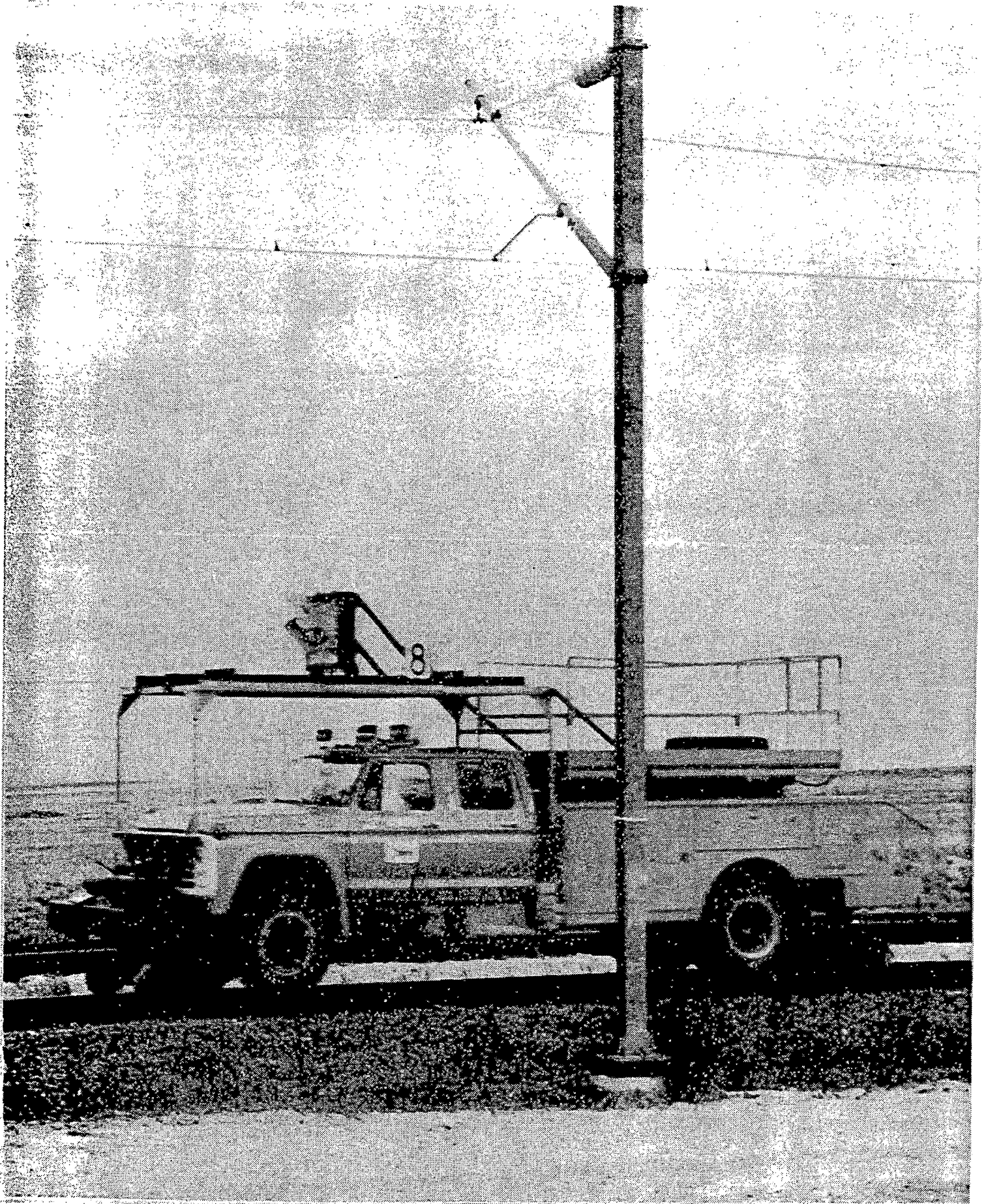
Figure A-1. Type I Large Object Impact Test at moment of impact.
