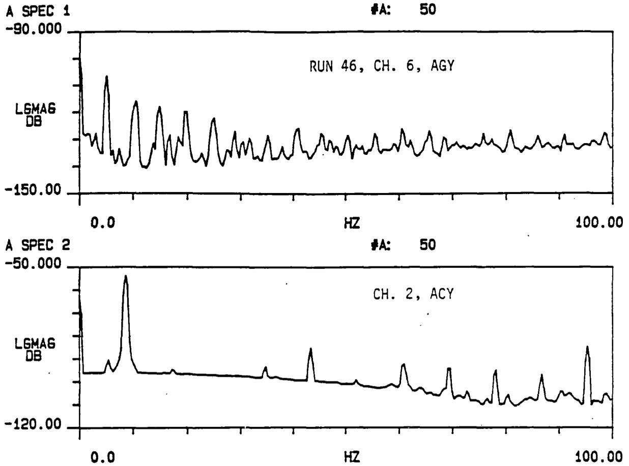
FIGURE 3.29 BALLAST AND CAR BODY LATERAL ACCELERATION AUTO SPECTRA OVER 0-100 HZ BANDWIDTH (HP 5420A)
