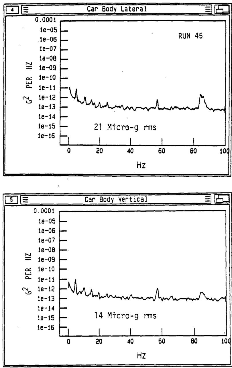
FIGURE 3.5 BACKGROUND ACCELERATION PSDs AT SITE #1, GENERATOR OFF, CAR BODY OVER TRAILING TRUCK
