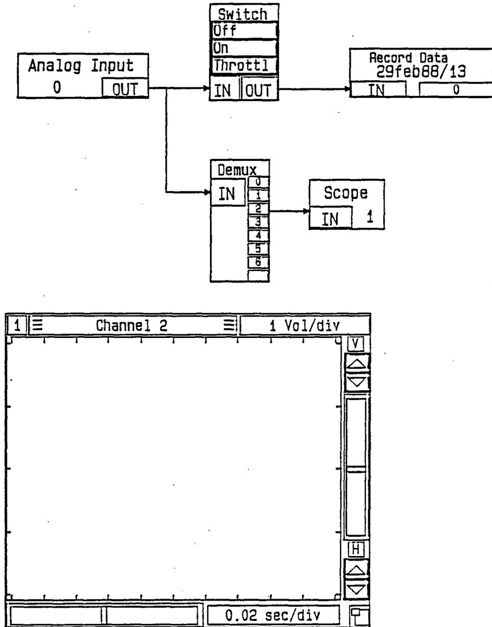
FIGURE 2.11 MASSCOMP MC-500 COMPUTER SYSTEM SET-UP STATE FOR A/D CONVERSION, RECORDING AND MONITORING
