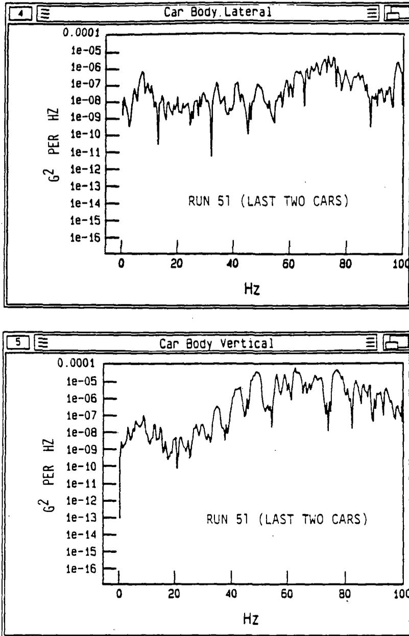
FIGURE 3.24 CAR BODY ACCELERATION PSDs OVER TRAILING TRUCK DURING CONSIST #3 45-MPH PASS-BY
