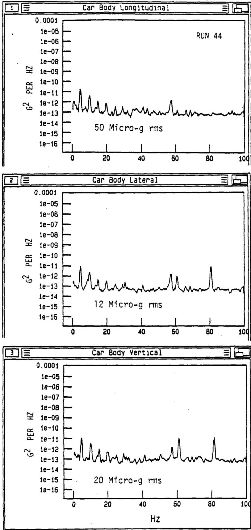
FIGURE 3.1 BACKGROUND ACCELERATION PSDs AT SITE #1, GENERATOR ON, CAR BODY OVER LEADING TRUCK
