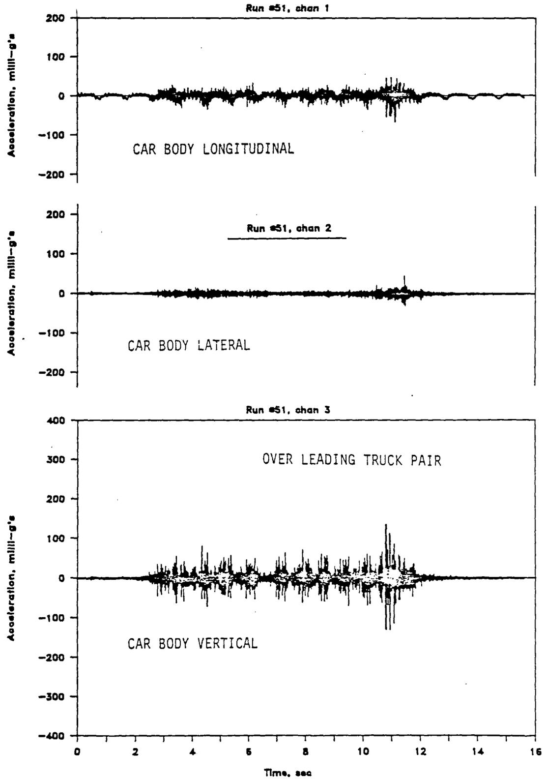
FIGURE 3.20 TIME HISTORIES OF CAR BODY ACCELERATION RESPONSE OVER LEADING TRUCK DURING CONSIST #3 45-MPH PASS-BY
