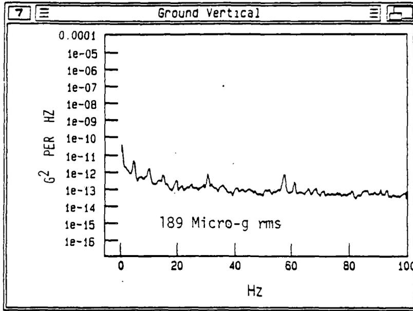
FIGURE 3.3 BACKGROUND ACCELERATION PSDs AT SITE #1, GENERATOR ON, BALLAST UNDER LEADING CAR AXLE
