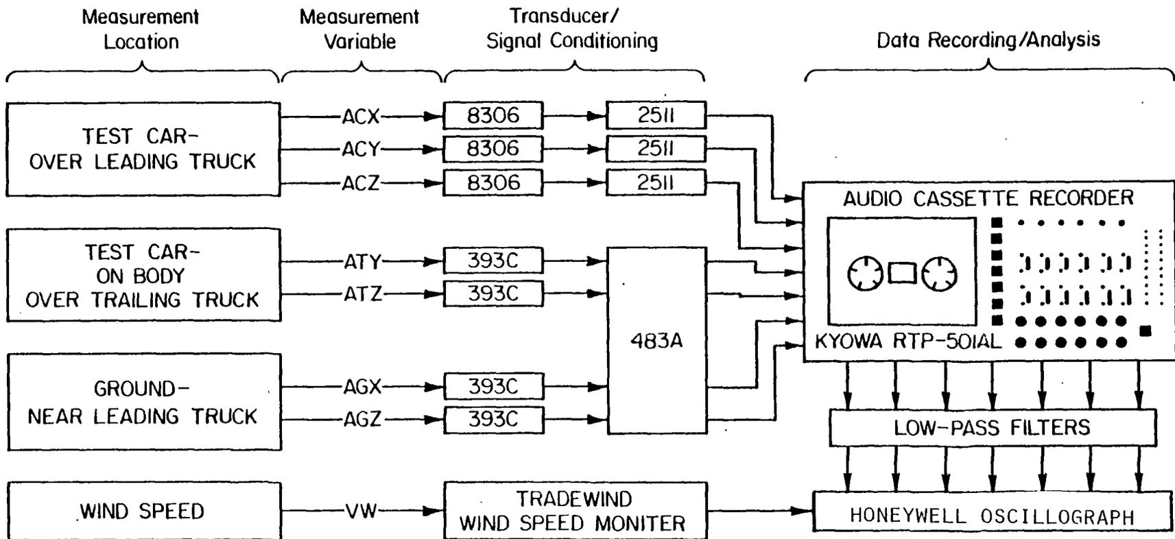
FIGURE 2.1 SCHEMATIC OF FIELD MEASUREMENT AND DATA ACQUISITION SYSTEM
