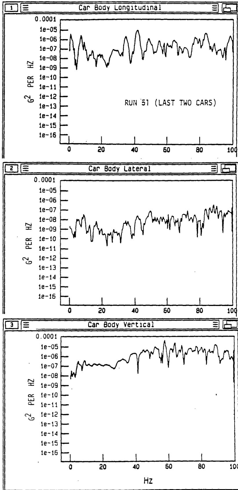
FIGURE 3.23 CAR BODY ACCELERATION PSDs OVER LEADING TRUCK DURING CONSIST #3 45-MPH PASS-BY
