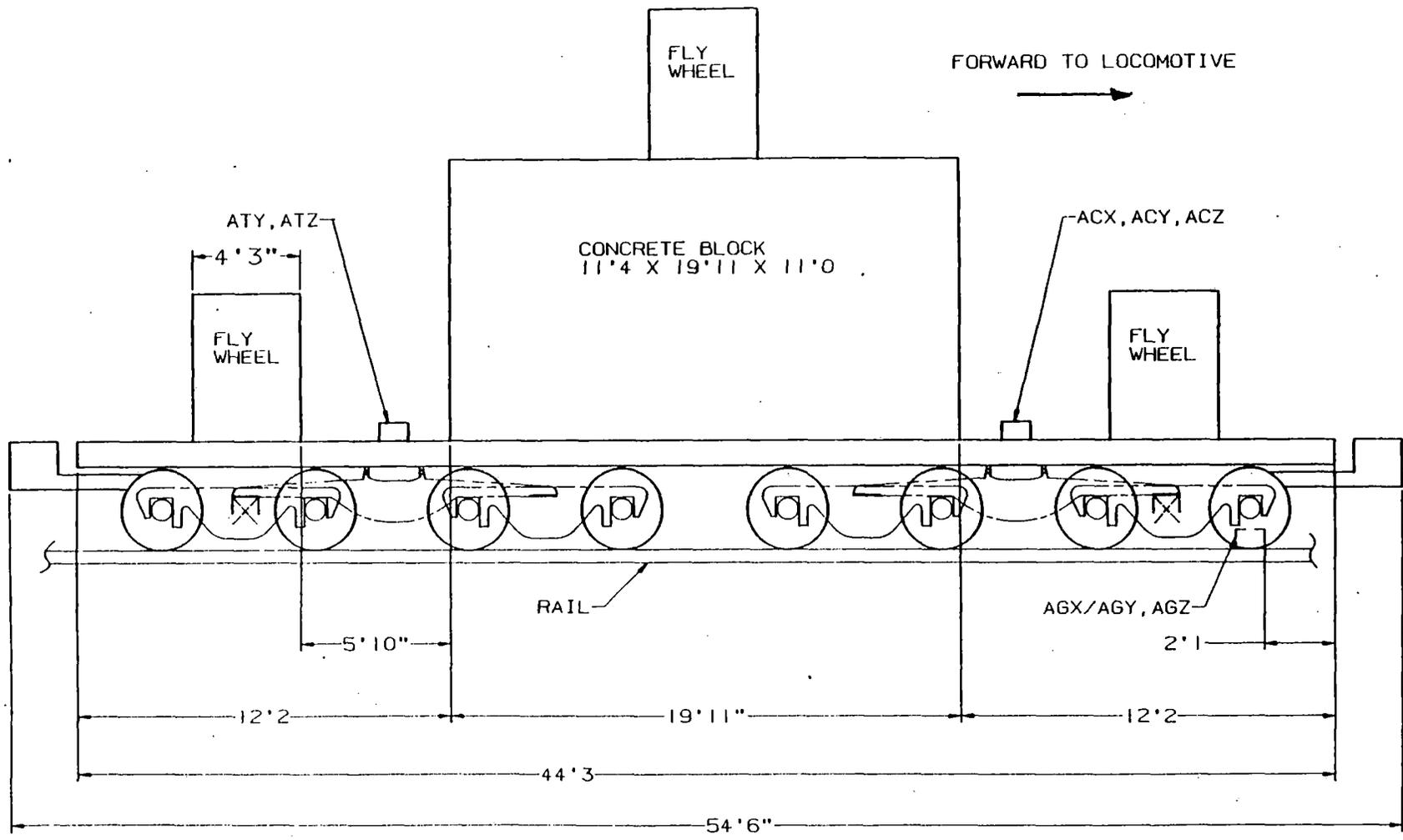
FIGURE 2.5 SKETCH OF SIMULATED MISSILE LAUNCH CAR WITH LOAD AND TRANSDUCER LOCATIONS
