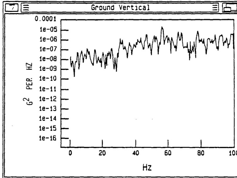
FIGURE 3.25 BALLAST ACCELERATION PSDs UNDER LEADING TRUCK DURING CONSIST #3 45-MPH PASS-BY
