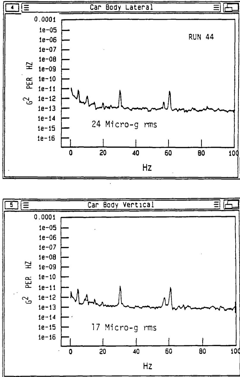
FIGURE 3.2 BACKGROUND ACCELERATION PSDs AT SITE #1, GENERATOR ON, CAR BODY OVER TRAILING TRUCK
