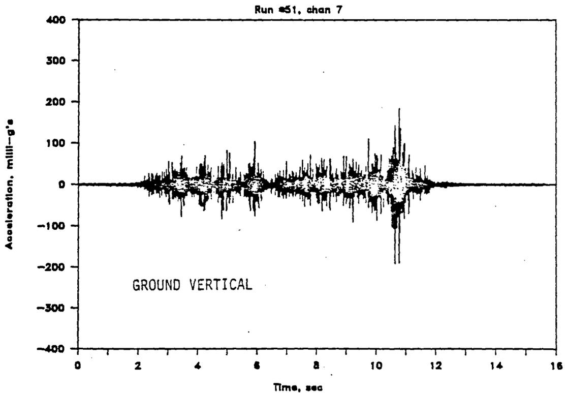
FIGURE 3.22 TIME HISTORIES OF BALLAST ACCELERATION RESPONSE UNDER LEADING TRUCK DURING CONSIST #3 45-MPH PASS-BY
