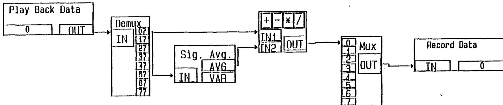
FIGURE 2.12 MASSCOMP MC-500 COMPUTER SYSTEM SET-UP STATE FOR DETRENDING ACCELERATION DATA SEGMENTS
