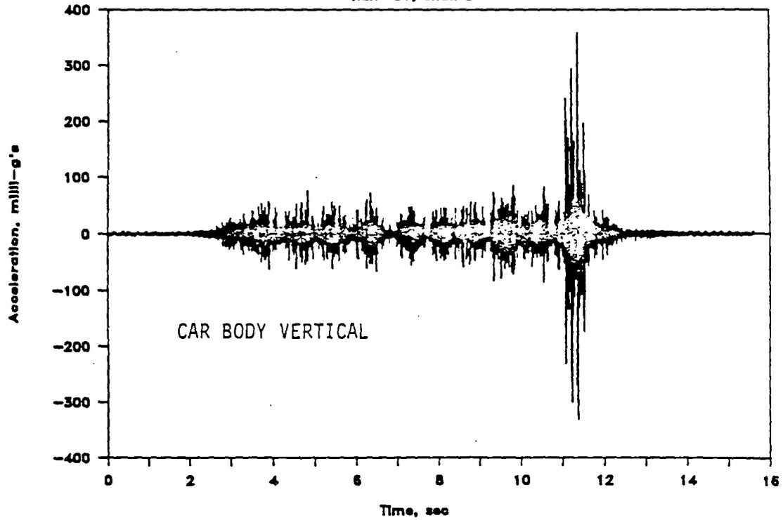
FIGURE 3.21 TIME HISTORIES OF CAR BODY ACCELERATION RESPONSE OVER TRAILING TRUCK DURING CONSIST #3 45-MPH PASS-BY
