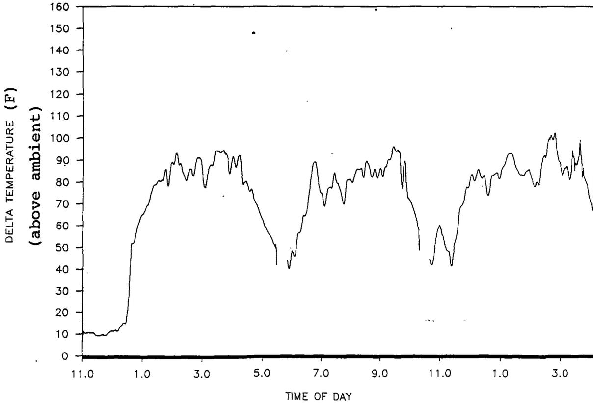
Electronic noise was again encountered on the double-stack bearing recorders, as it had been on the prototype test. Obviously anomalous values have been removed from the figures. We are unable to explain the source of the noise on only the double-stack recorders; the TTX flatcar was in closer proximity to the locomotives over two thirds of the test run and suffered no interference. The interference particularly occurred during stops.
