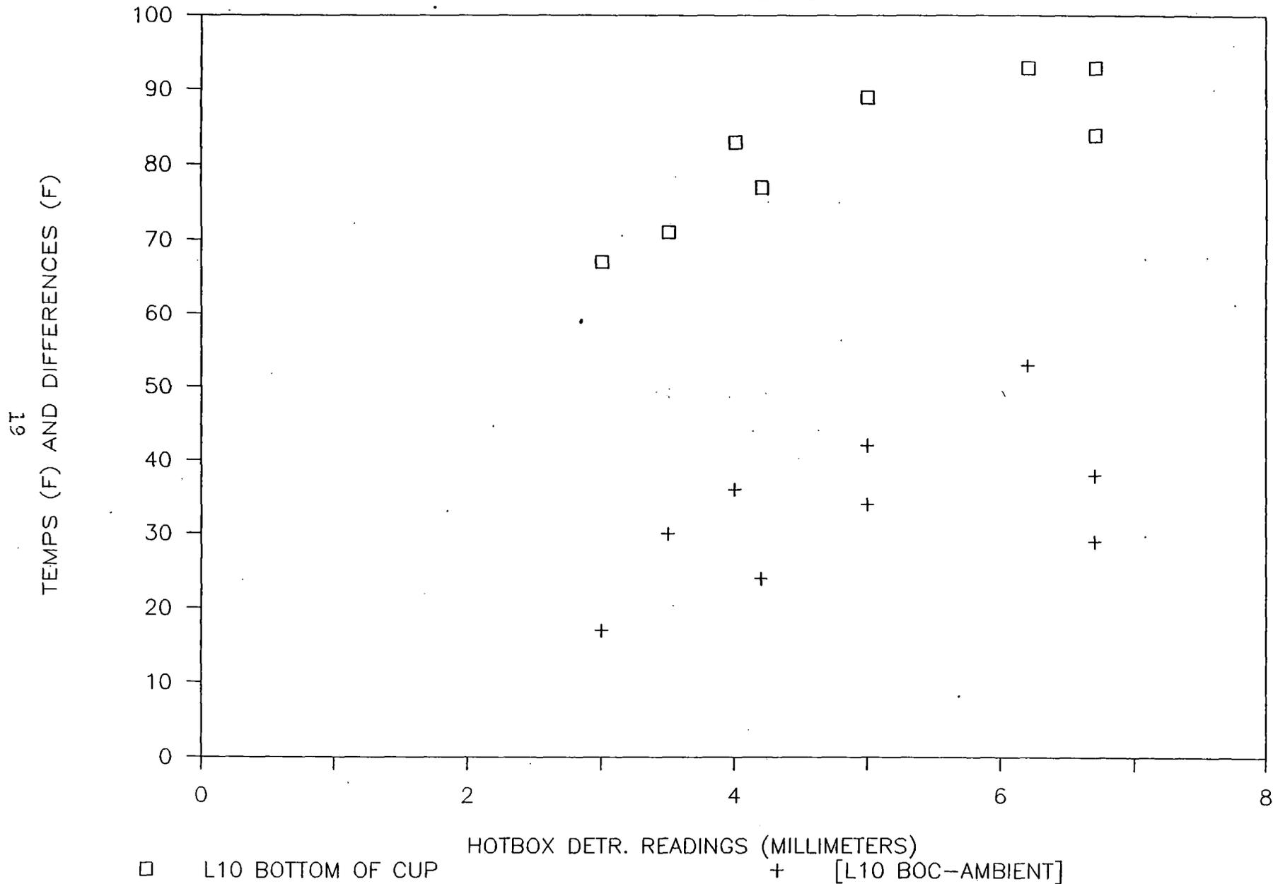
Fig 8. Detector Readings vs Measured Temp
