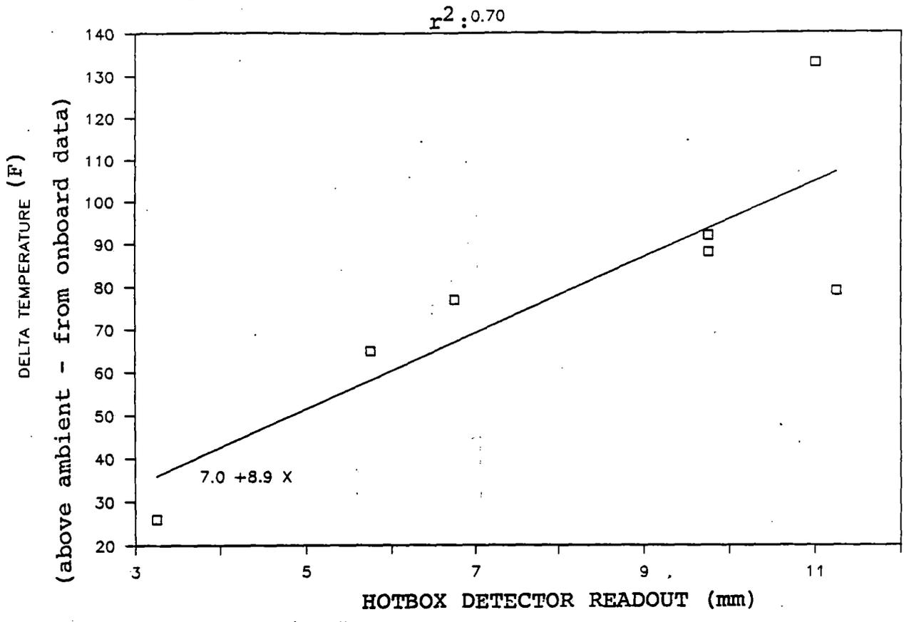
Fig. 42: HOT BOX DETECTOR # 12 (Cuba, MS.)
