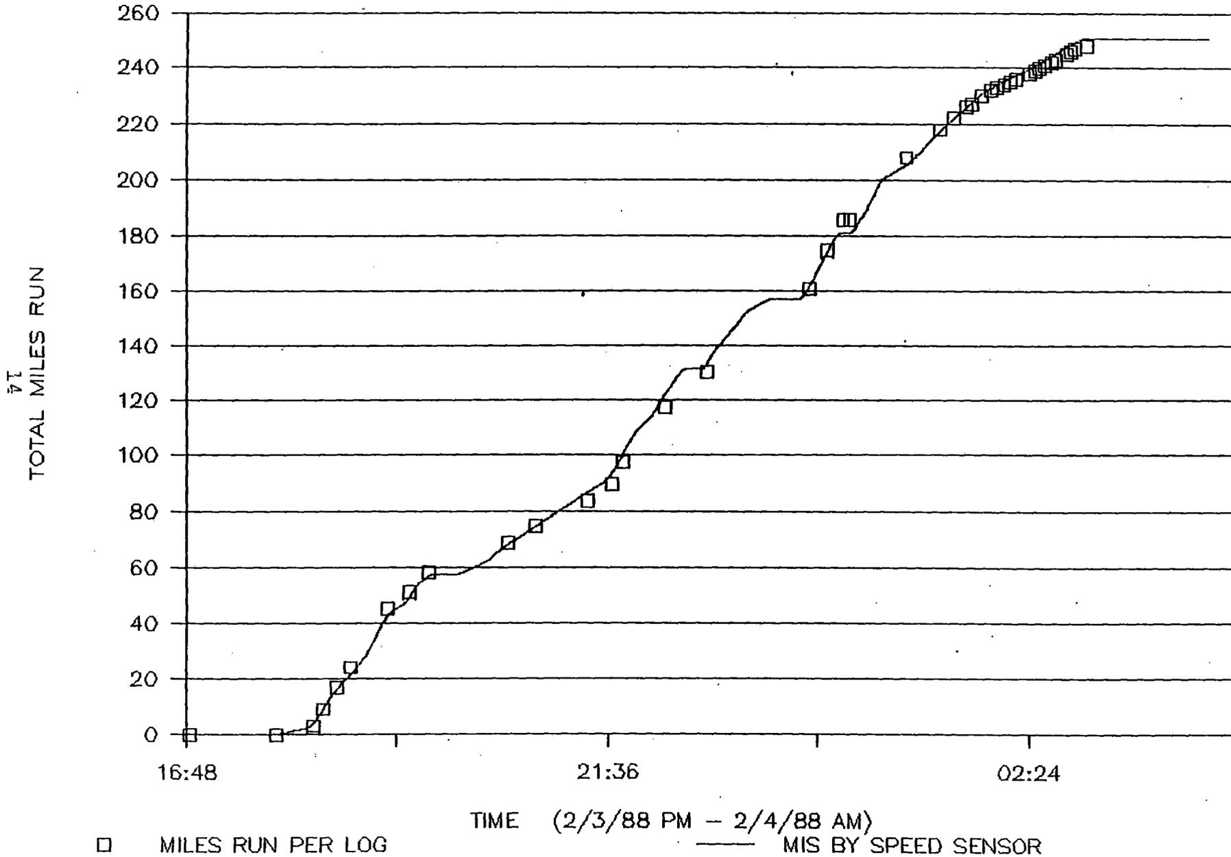
Fig 6. Miles Run and Integrated Pulse Count (Eastbound)
