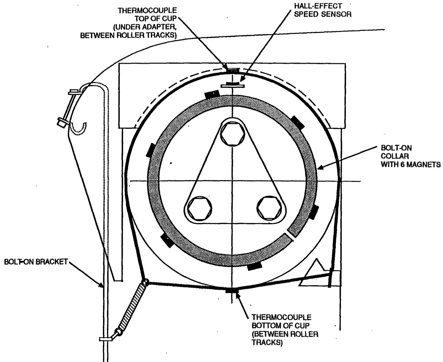
FIGURE 1 TEMPERATURE AND SPEED SENSING INSTRUMENTATION
