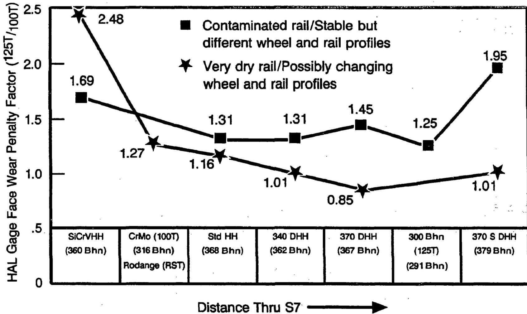
Figure 5. Variation of Penalty Factor with Position-In-Curve, Metallurgy, and Lubrication Condition
