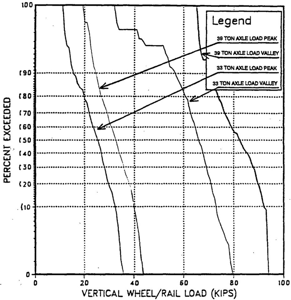
Figure 7. Dynamic Vertical Load Data
