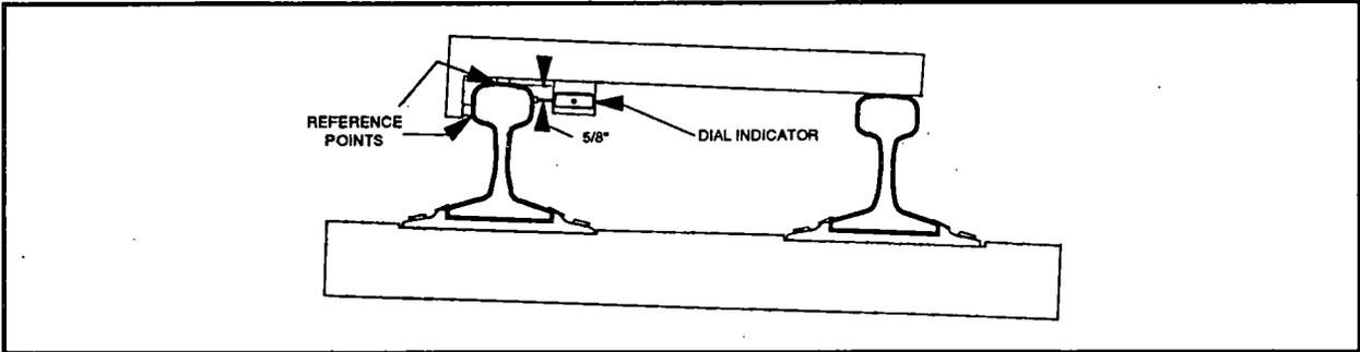
Figure 1. Gage Face Wear Measurement
