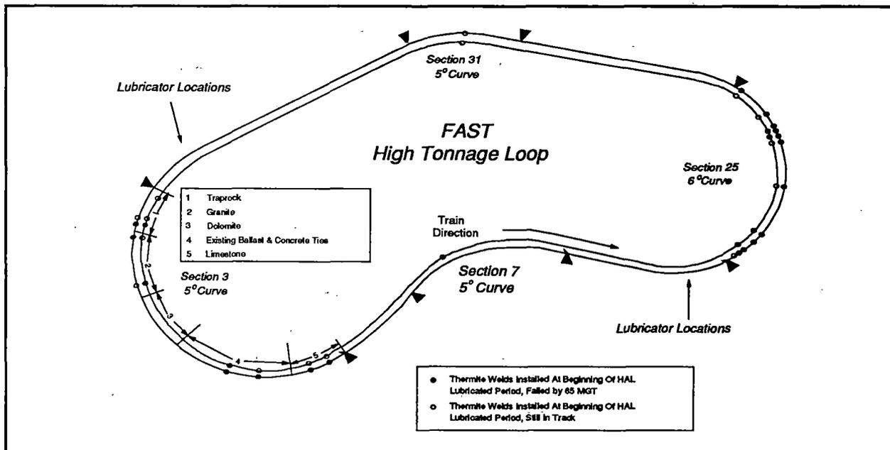
Figure 1. Location of Thermite Welds on FAST Track
