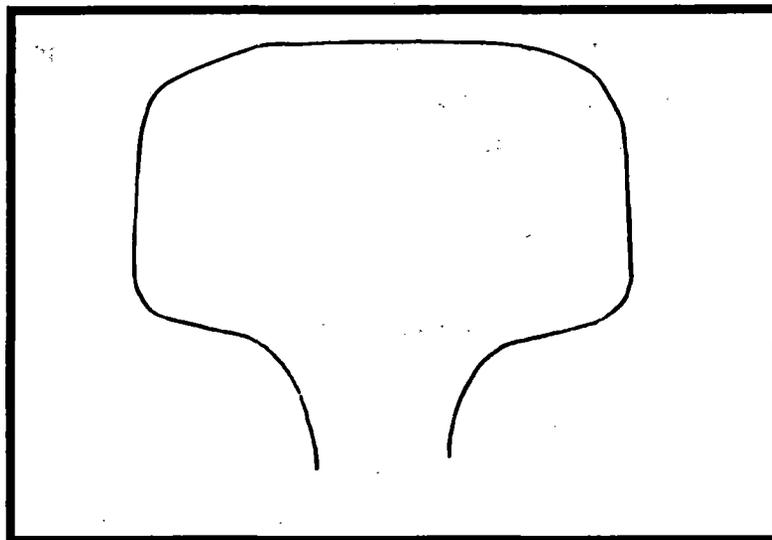
**Figure 1. High Rail Gage Corner Grind
