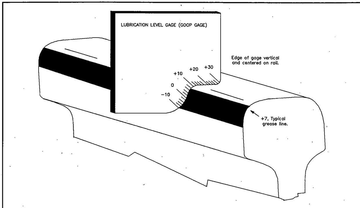
**Figure 9. TTC's Lubricant Level Gage (Goop Gage)**
