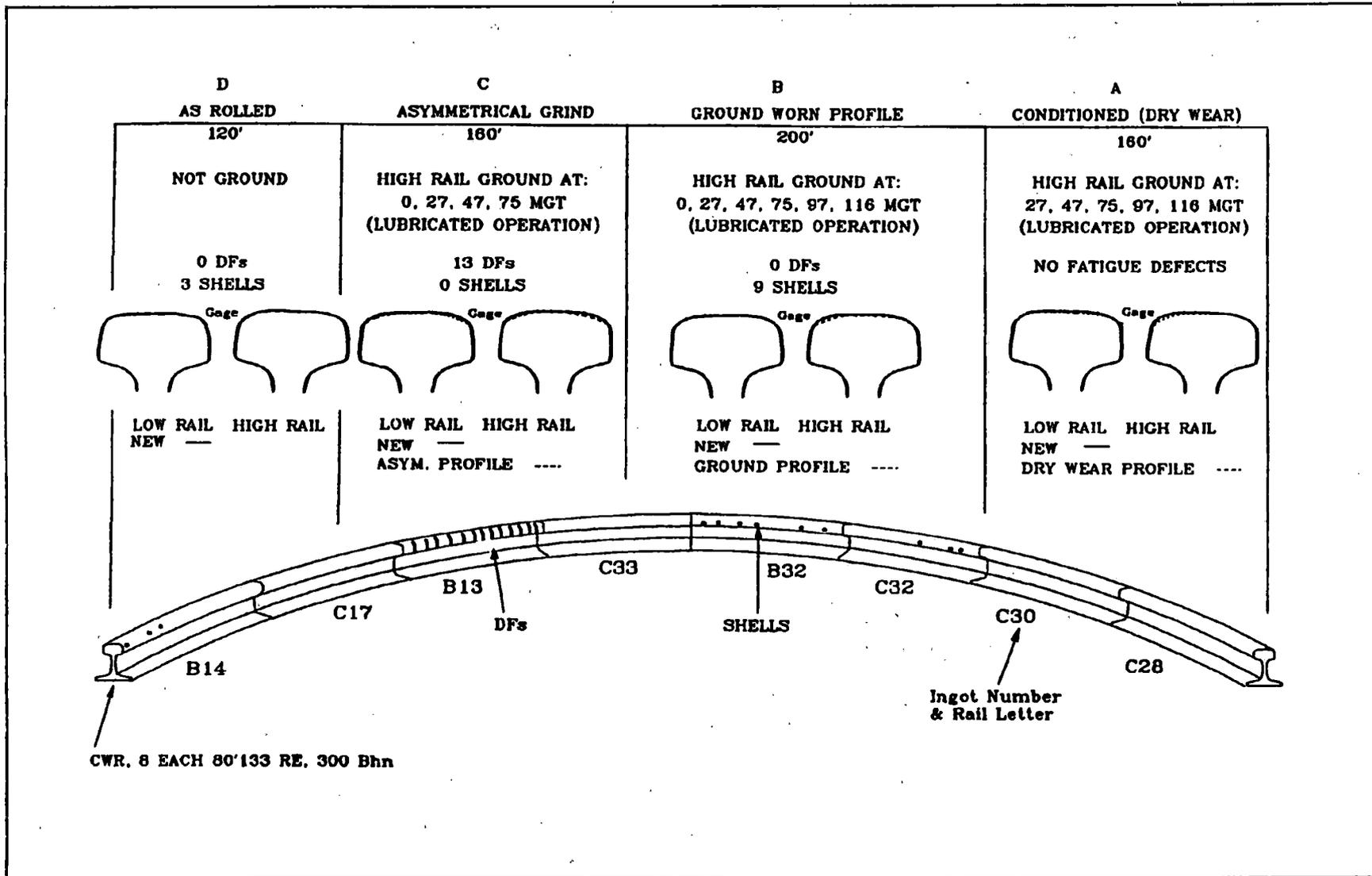
Figure 3. Grind Zone -- High Rail of HTL Section 25
