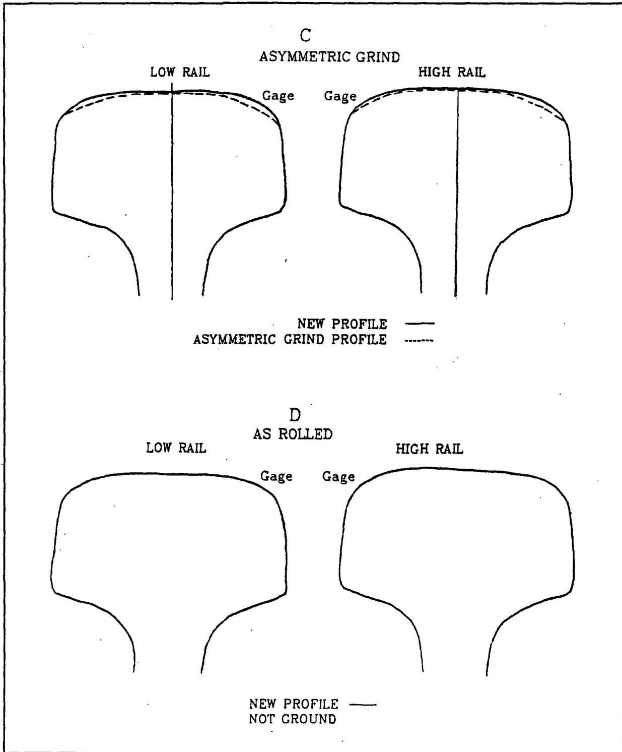
Figure 4b. Ground Asymmetric and As Rolled Profiles
