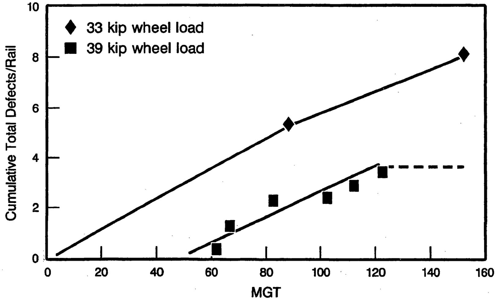
Figure 12. Fatigue Defect Accumulation Behavior as a Function of Service Exposure/Bethlehem 289 Old Unused
