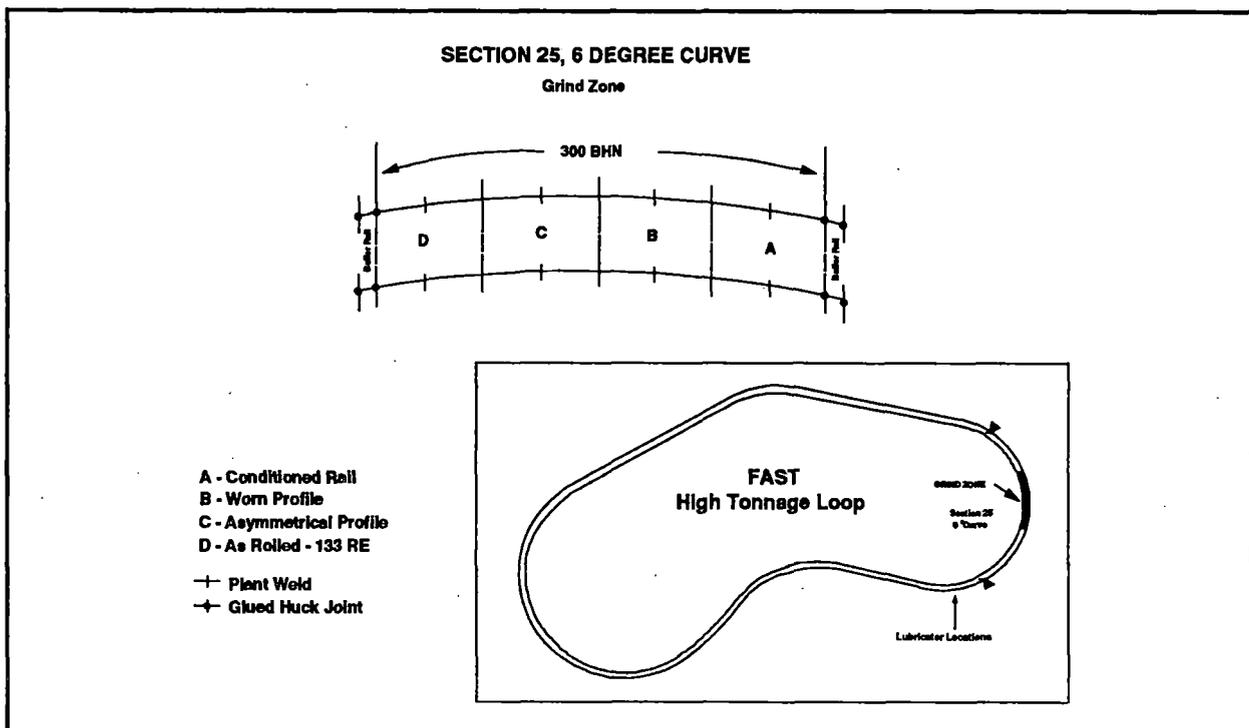
Figure 2. Layout of Grind Zone in High Tonnage Loop
