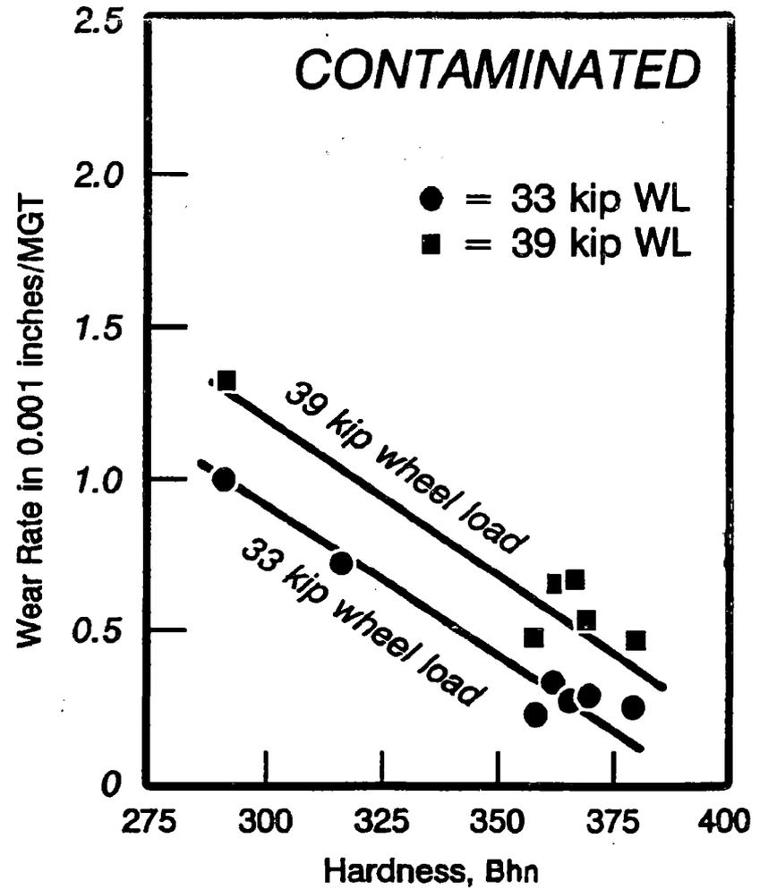
Figure 7. High Rail Head Height Loss Rates as a Function of Hardness
