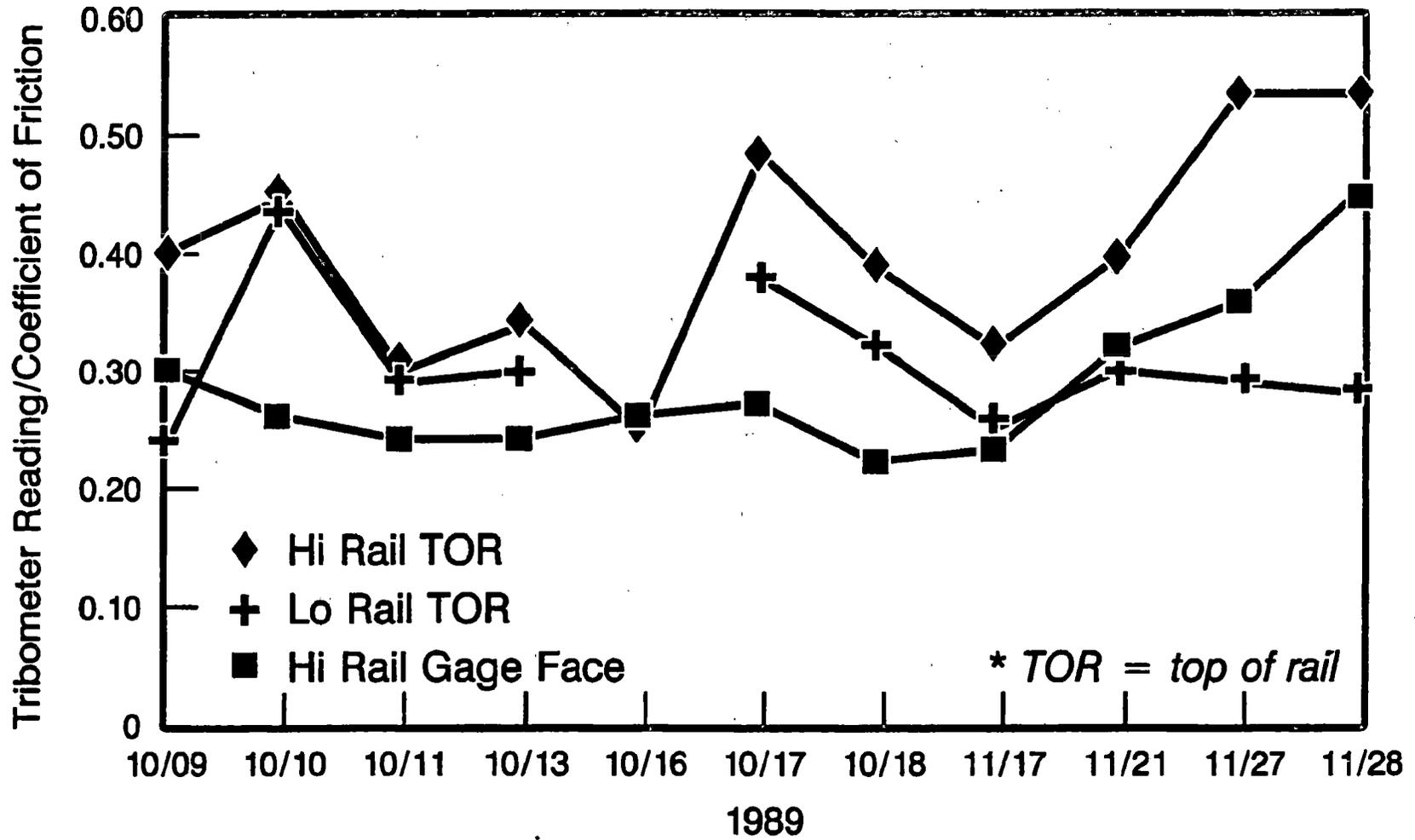
Figure 9. Tribometer Measurement of Rail Lubrication/Location 070093
