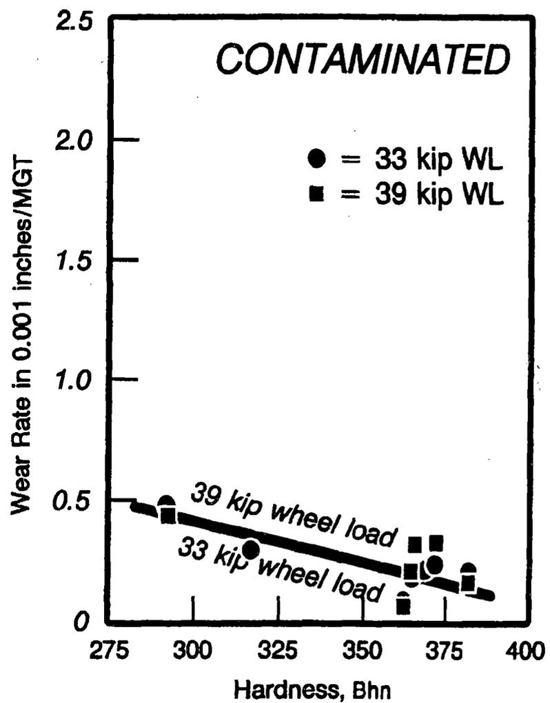
Figure 8. Low Rail Head Height Loss Rates as a Function of Hardness
