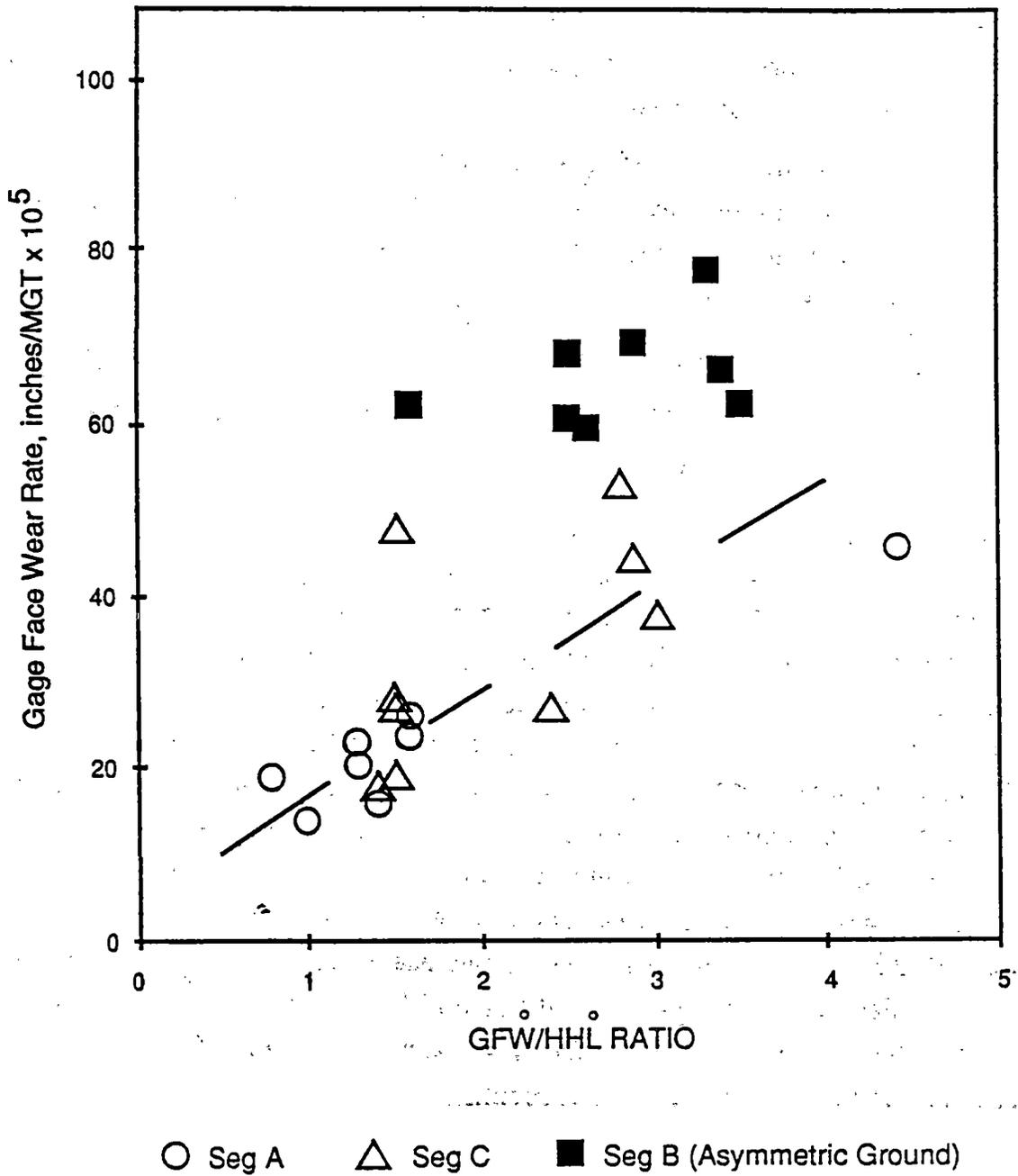
Figure 3. Lubricated Wear Rates, S25 33 KIP Wheel Load Test
