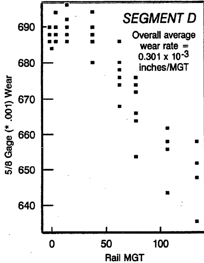
One final observation is relevant. It was intended to grind segments A and B to the worn profile removing about 2 mm/100 MGT. Head height loss measurements suggested that the removal rate was much closer to 1 mm/100 MGT.
