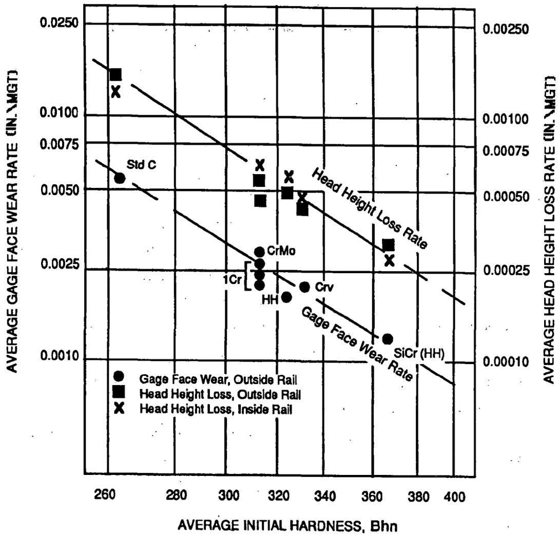
Figure 1. Average Wear Rates as a Function of Average Initial Hardness
