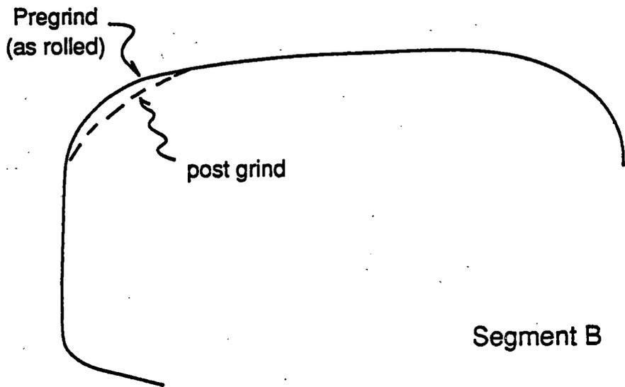
**Figure 20. Asymmetric Profile Initially Ground on Rail in Segments A and B**
