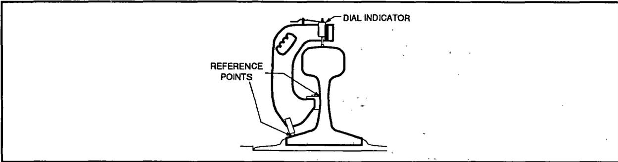
**Figure 3. Head Height Loss Measurement**
