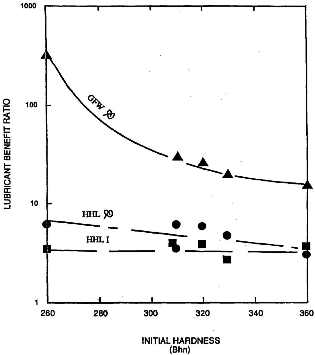
Figure 2. The Variation of Lubrication Benefit Ratio with Hardness
