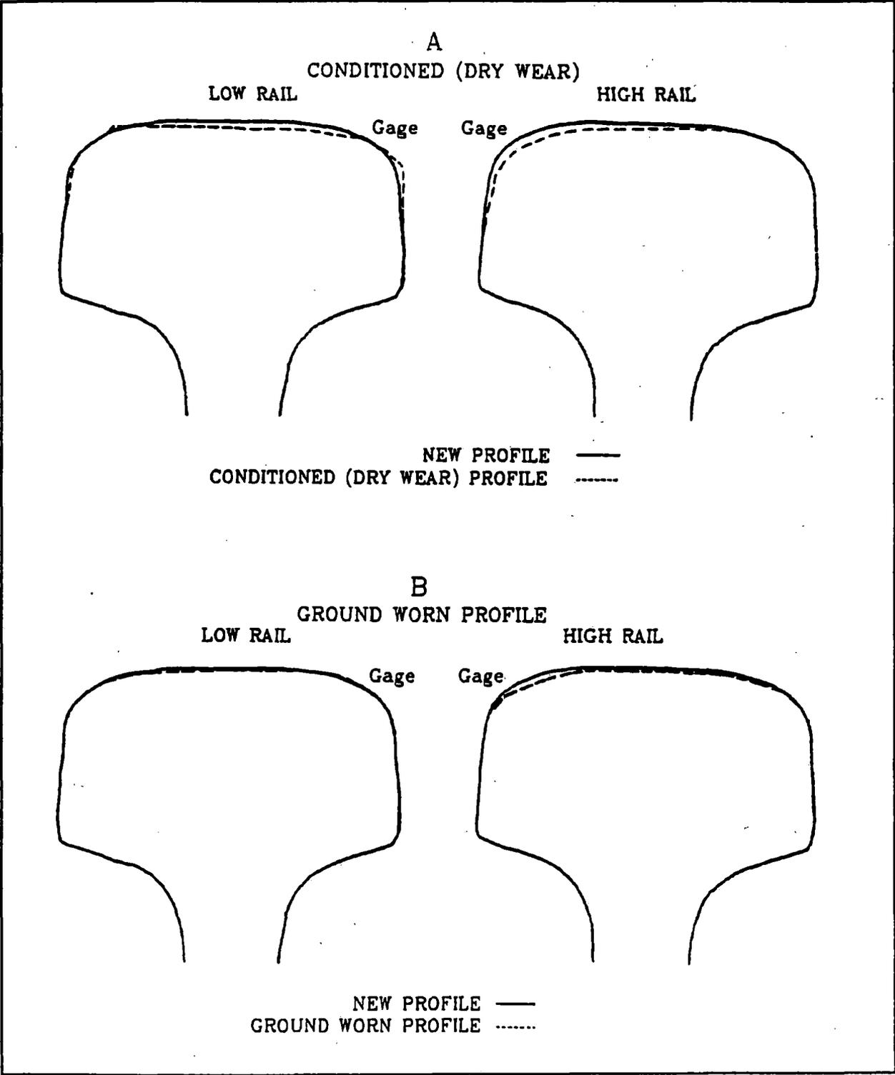
Figure 4a. Dry Wear and Ground Worn Profiles
