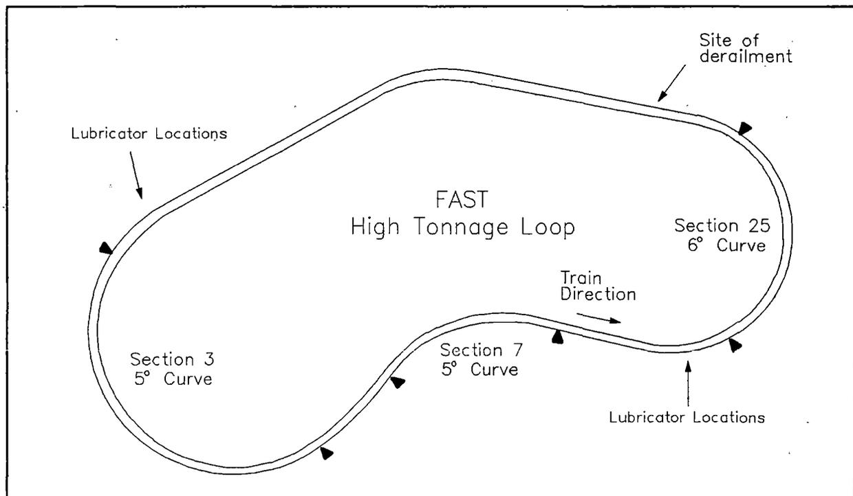
**Figure 3. Lubricator Locations on the High Tonnage Loop**
