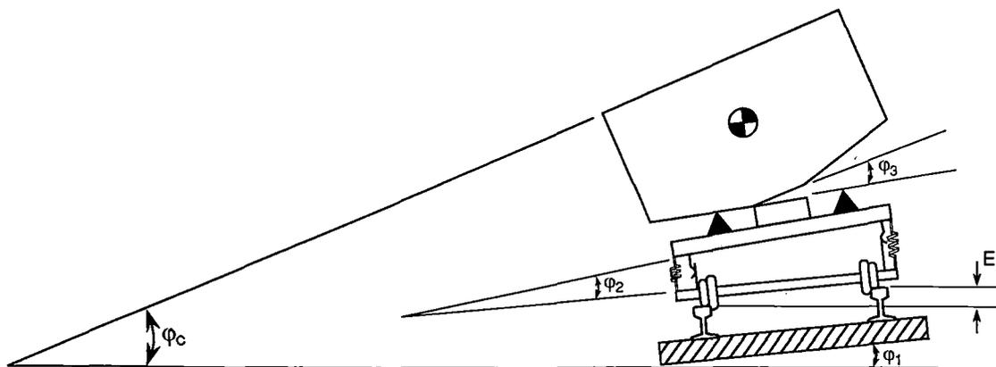
*Model for Analyzing Rail Vehicle Response to Track Twist*
