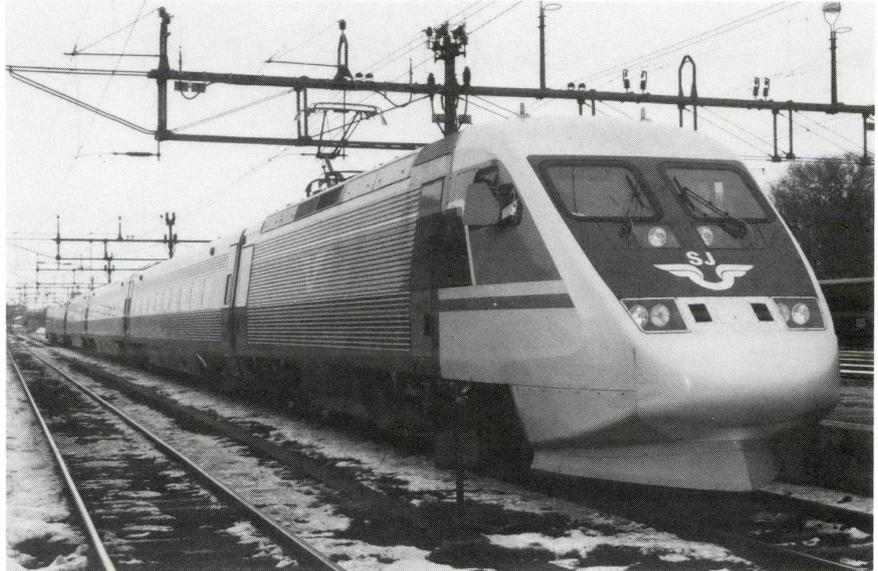
*The X2000 Tilting Train: Cab-Car End Forward at a Stop in Sweden Where It Operates over Existing Mixed Traffic Lines at 200 km/h (125 mph)*
