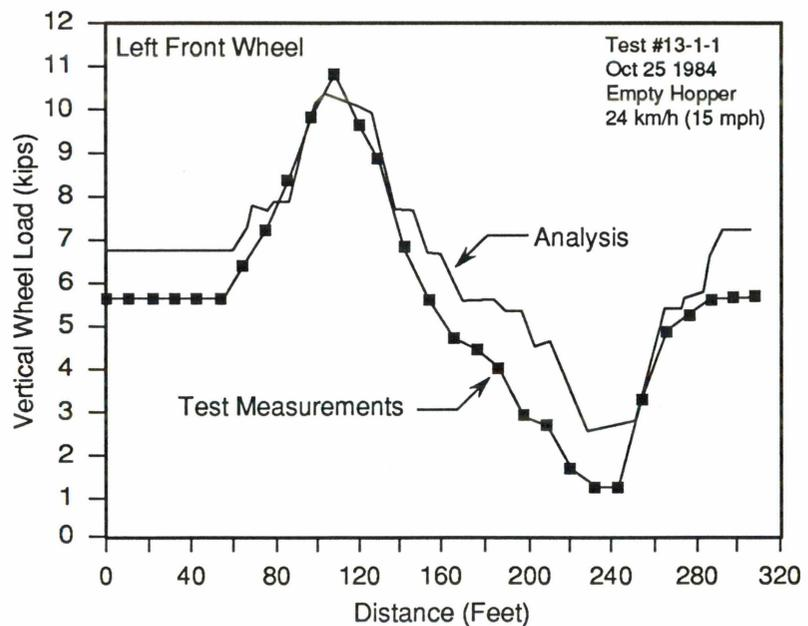
*Comparison of Model Prediction and Test Measurements of Rail Vehicle Response to Track Twist*
