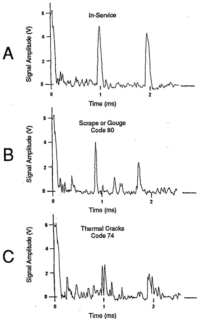
Typical Analog Signals Resulting from Initial Field Evaluations on the Prototype Wheel Crack Detection Unit, Train Speed: 8 km/h (5 mph)
