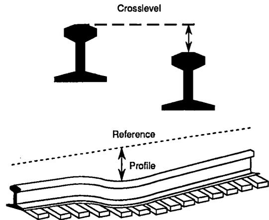
*Gauge Geometry and Profile Geometry*
