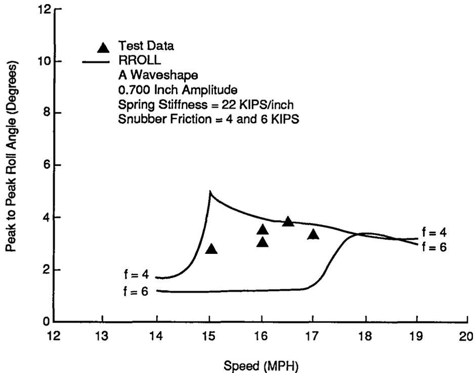
*Comparison of Model Prediction and Test Measurements of Rail Vehicle Harmonic Roll Behavior*
