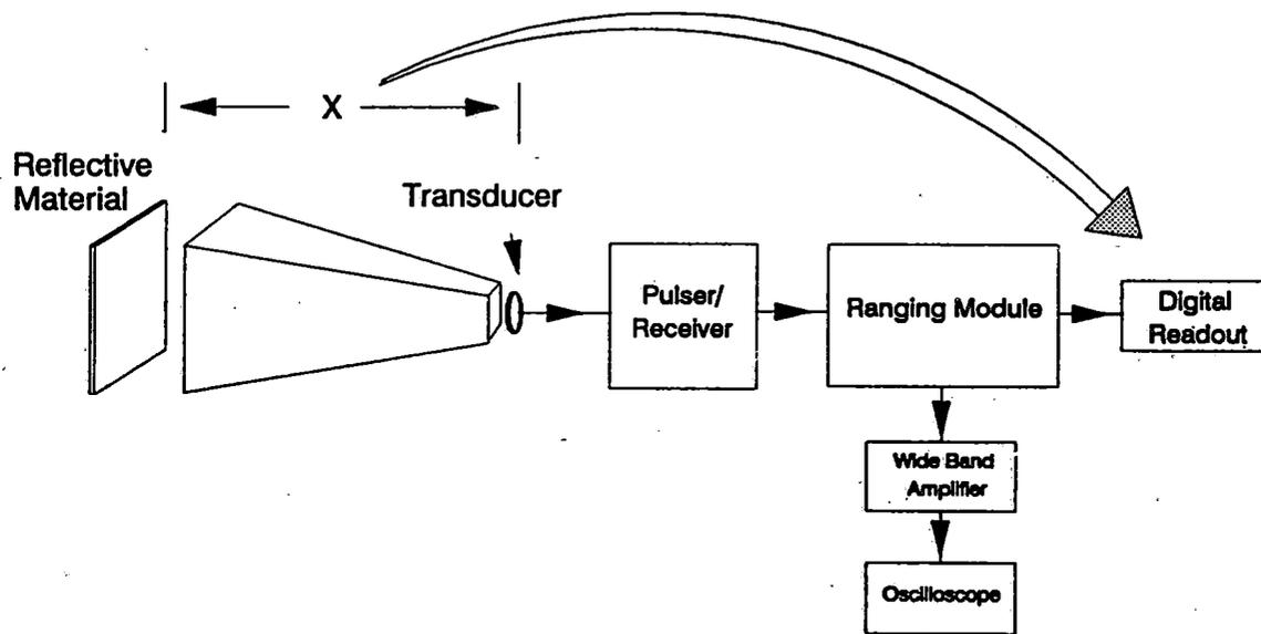
Figure A2-1: Test setup used for determining the feasibility of using air coupled ultrasonics for snow detection.
