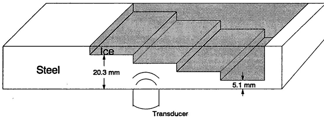
Figure A1-1: Cross-section of steel plate used in ice measurement tests.
