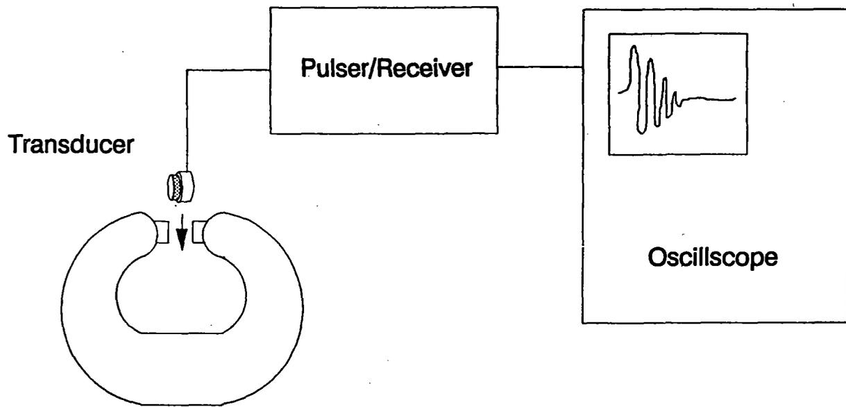
Figure A3-2: Test setup used for subjecting piezoelectric transducers to magnetic fields.
