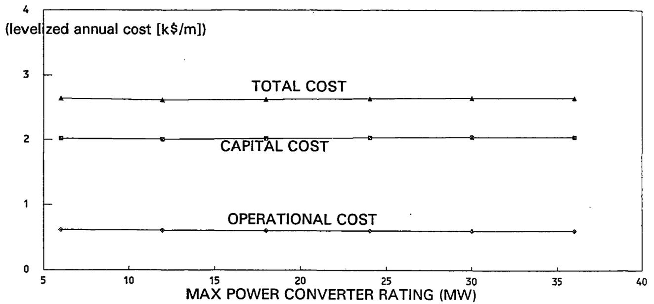
Figure 9 Effect of power supplied (graph)
