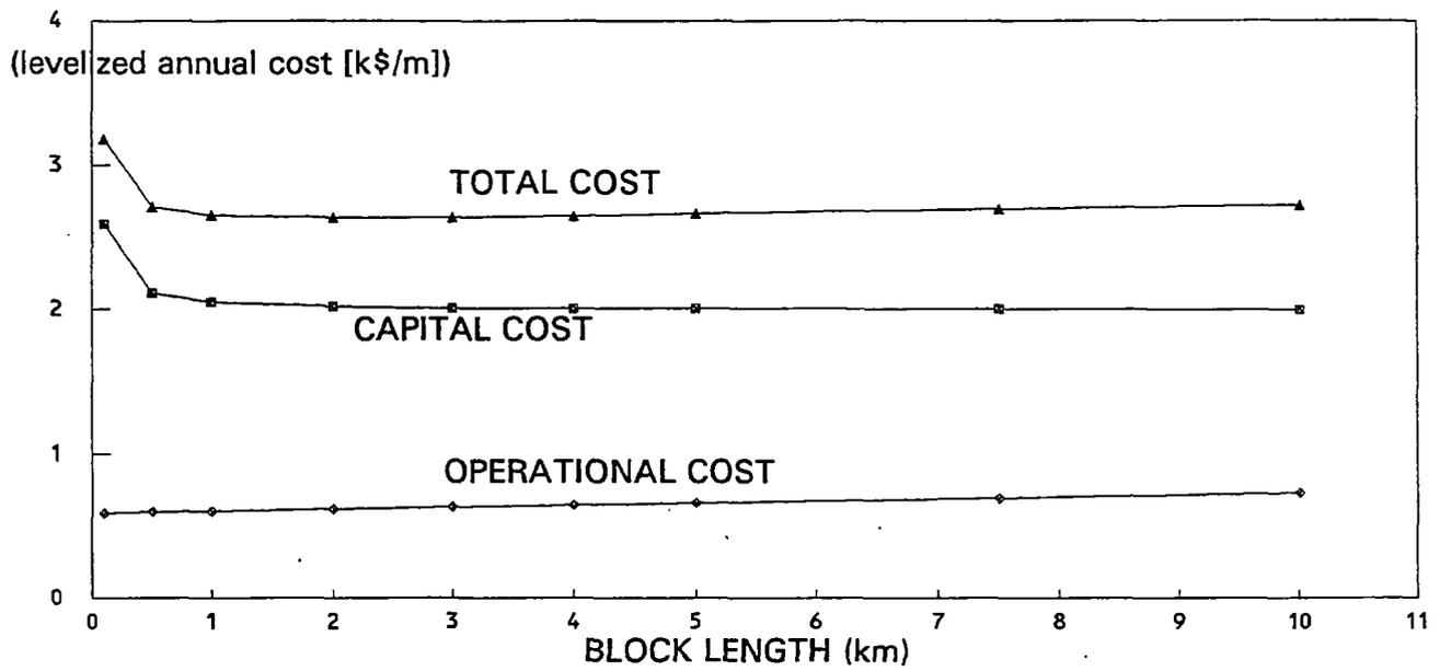
Figure 14 Effect of block length (graph)
