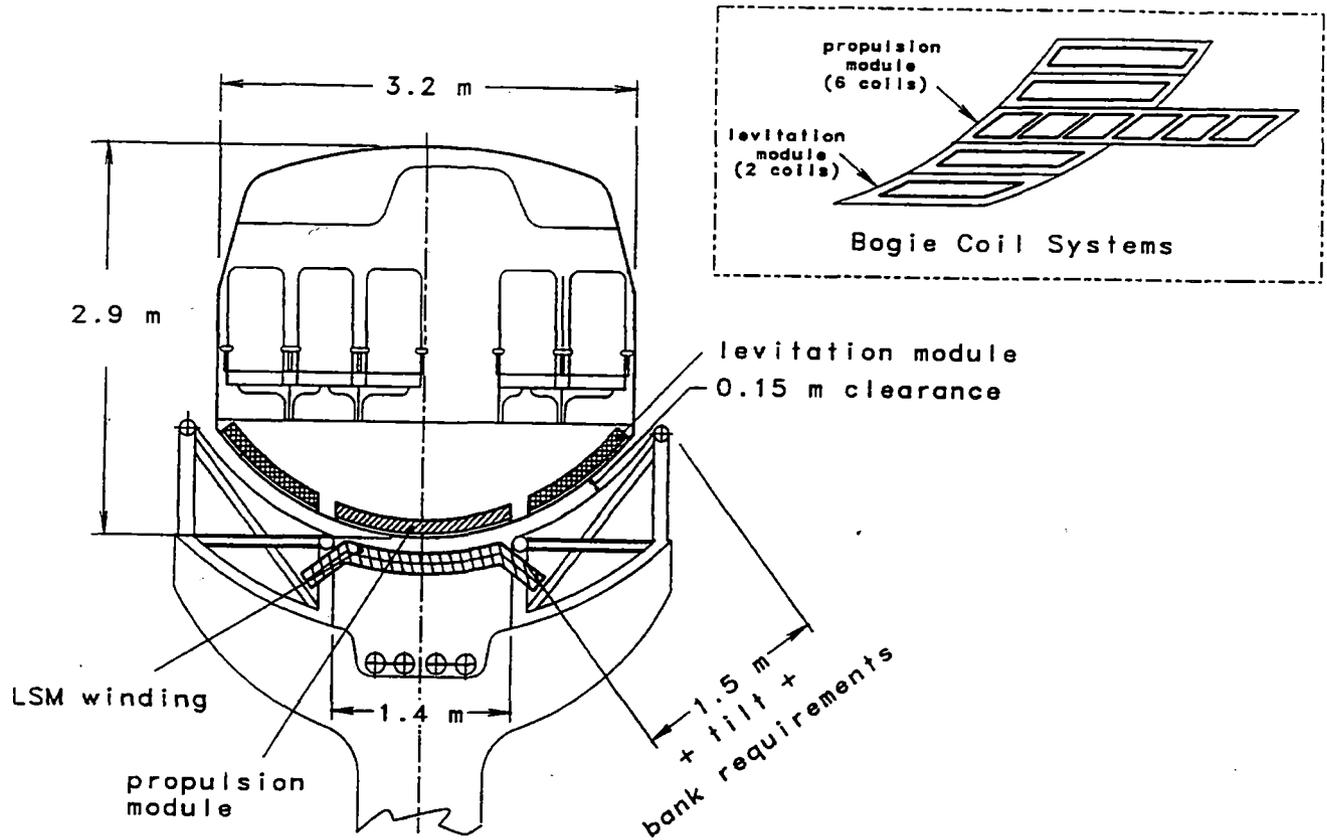
Figure 7 Vehicle cross-section sketch (dimensions approximate)
