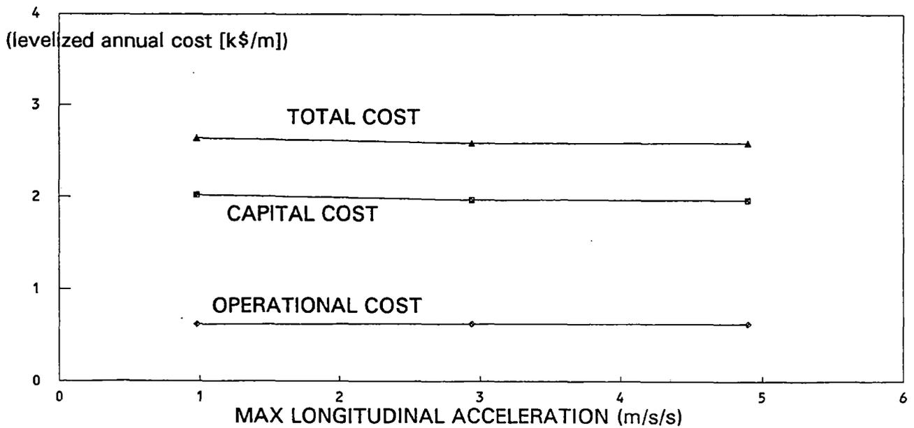
Figure 5 Effect of longitudinal acceleration (graphs)
