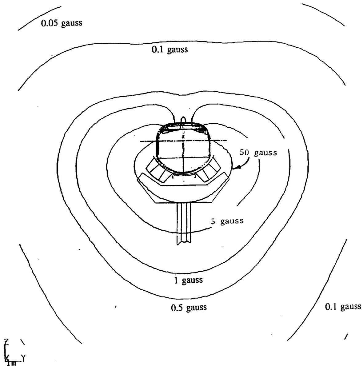
Figure 21 Contours of constant flux density in a transverse plane through the bogies with shield active (M07)
