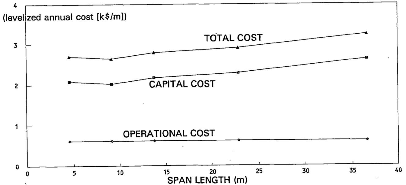
Figure 18 Effect of span length (values, graph)
