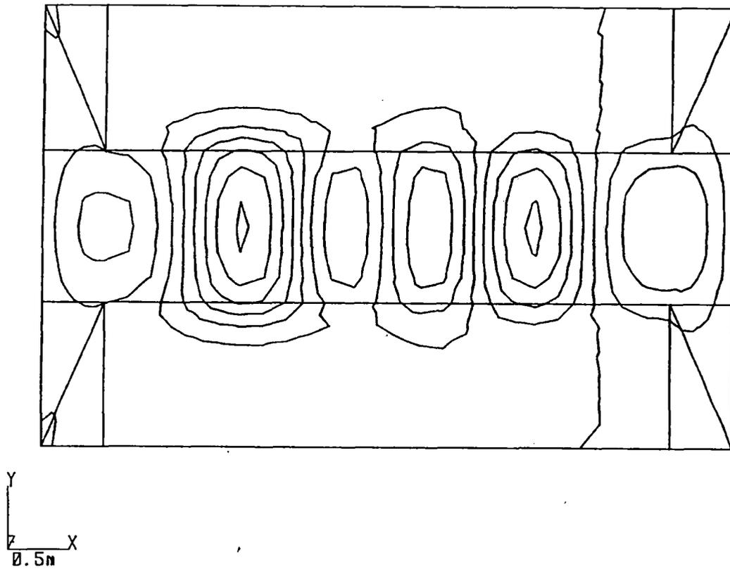
Figure 14 Plan view of ideal current pattern for shield coils
