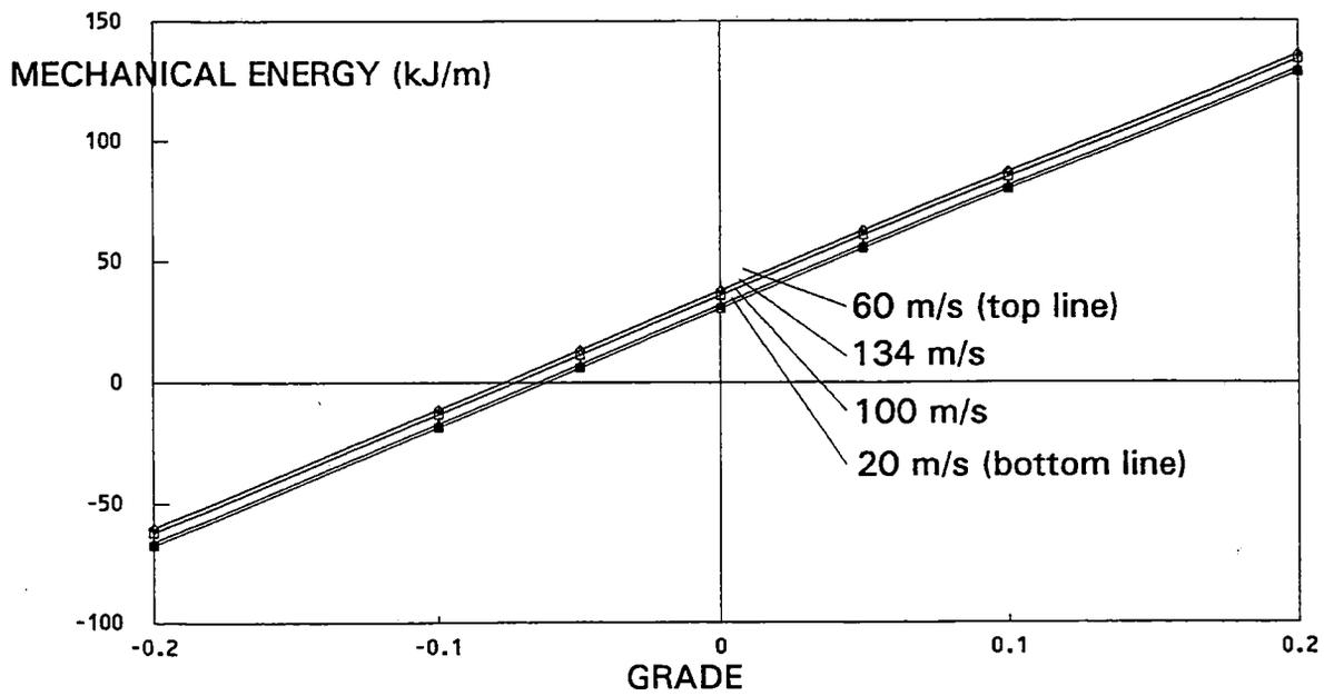
Figure 2 Mechanical power and energy requirements for various grades and velocities
