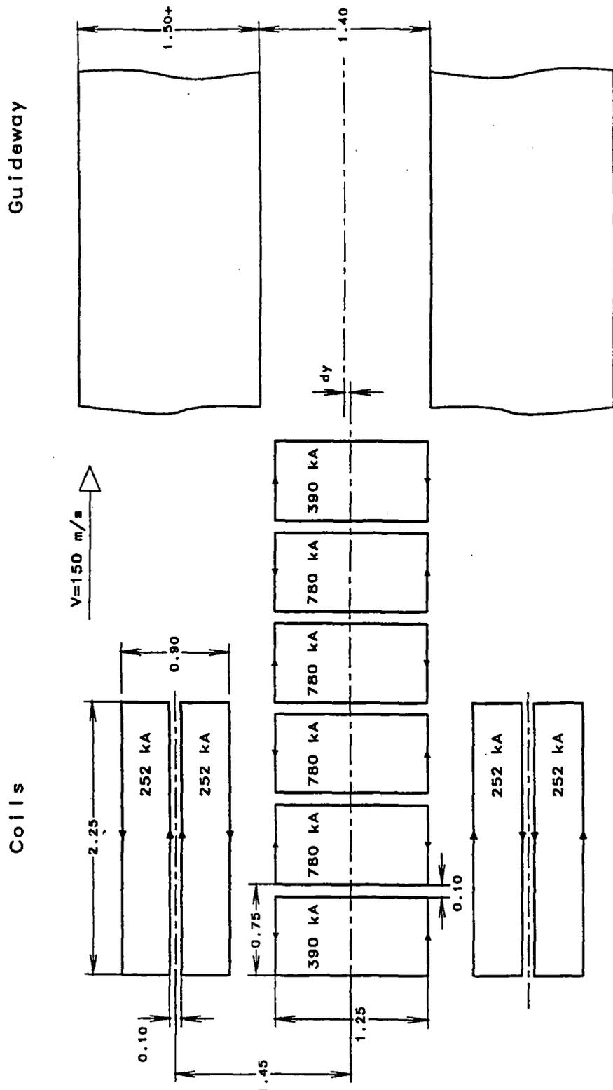
Figure 10 Schematic of coil and magway for forward bogie
