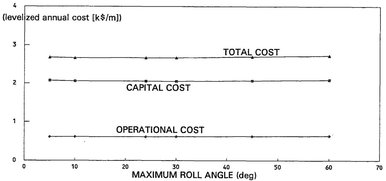
Figure 7 Effect of maximum roll angle (graph)
