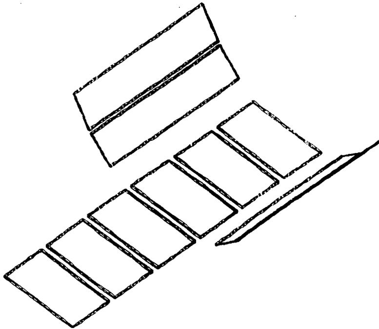
**Figure 11** Outline of propulsion and levitation coils in one bogie
