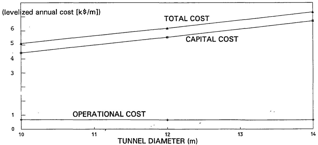
**Figure 15** Effect of tunnel diameter (values, graph)
