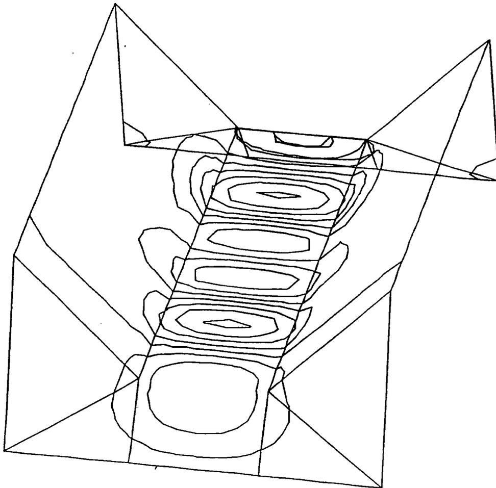
**Figure 13** Isometric view of ideal current pattern for shield coils
