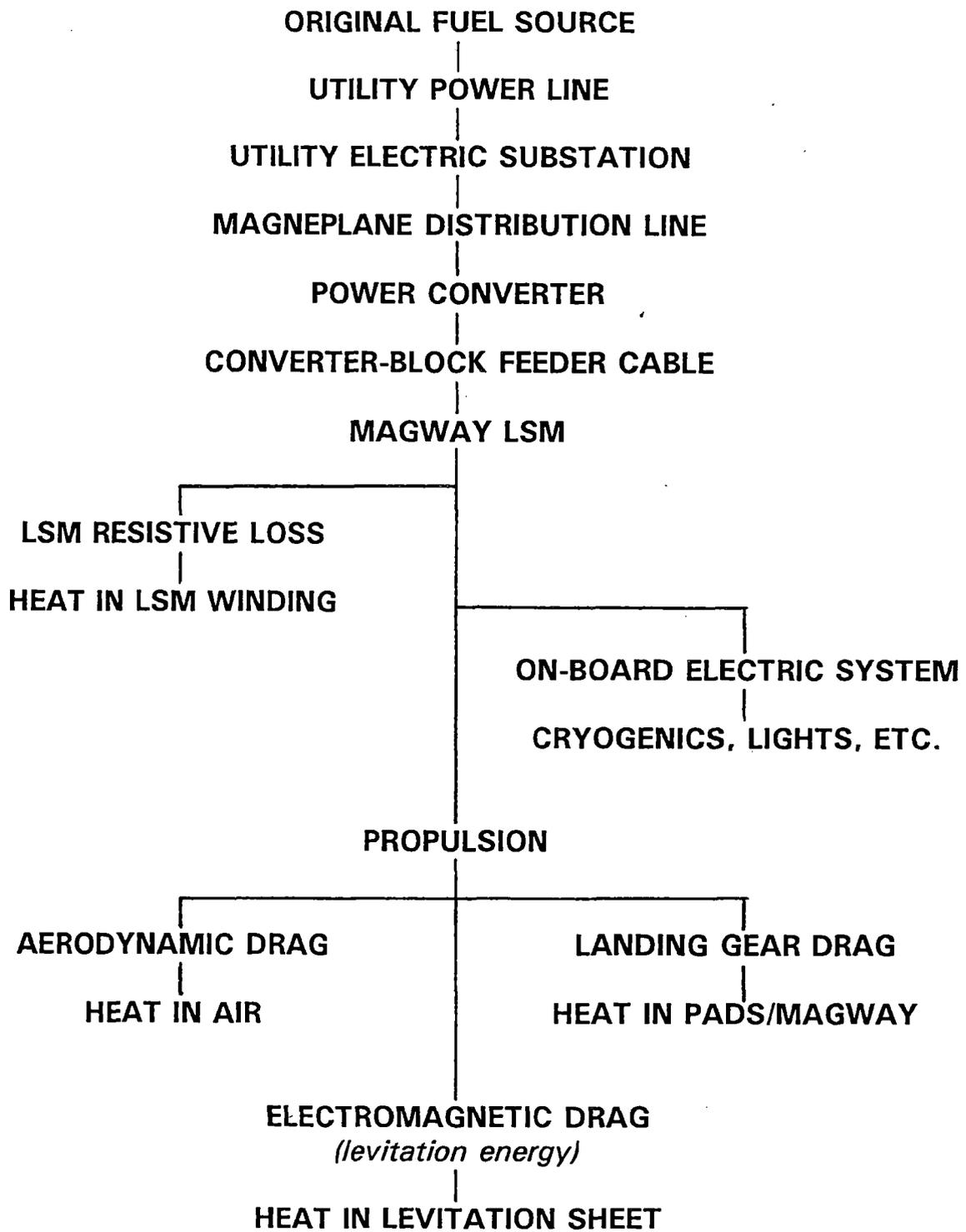
Figure 1 Energy flow diagram for the Magneplane system
