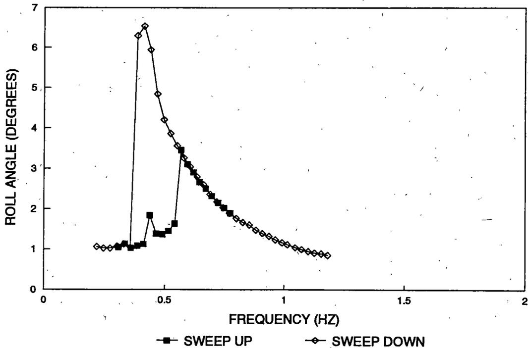
**Figure 14. 3/4-inch Side Bearing Clearance VTU Test Results (Configuration 7) -- Truck 1, B-End Car Body Roll Angle Versus Frequency, 13/32" Peak-to-peak Cross Level VTU Excitation**
