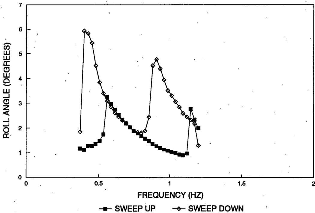
**Figure 19. 3/4-inch Side Bearing Clearance VTU Test Results (Configuration 12) -- Truck 2, B-End Car Body Roll Angle Versus Frequency, 13/32" Peak-to-peak Cross Level VTU Excitation**
