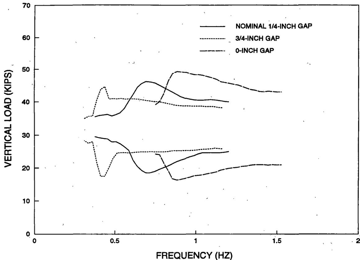
**Figure 24. Comparison of Wheel Unloading for VTU-Test Configurations 1 (nominal), 7 (3/4-inch clearance), and 3 (zero clearance)**
