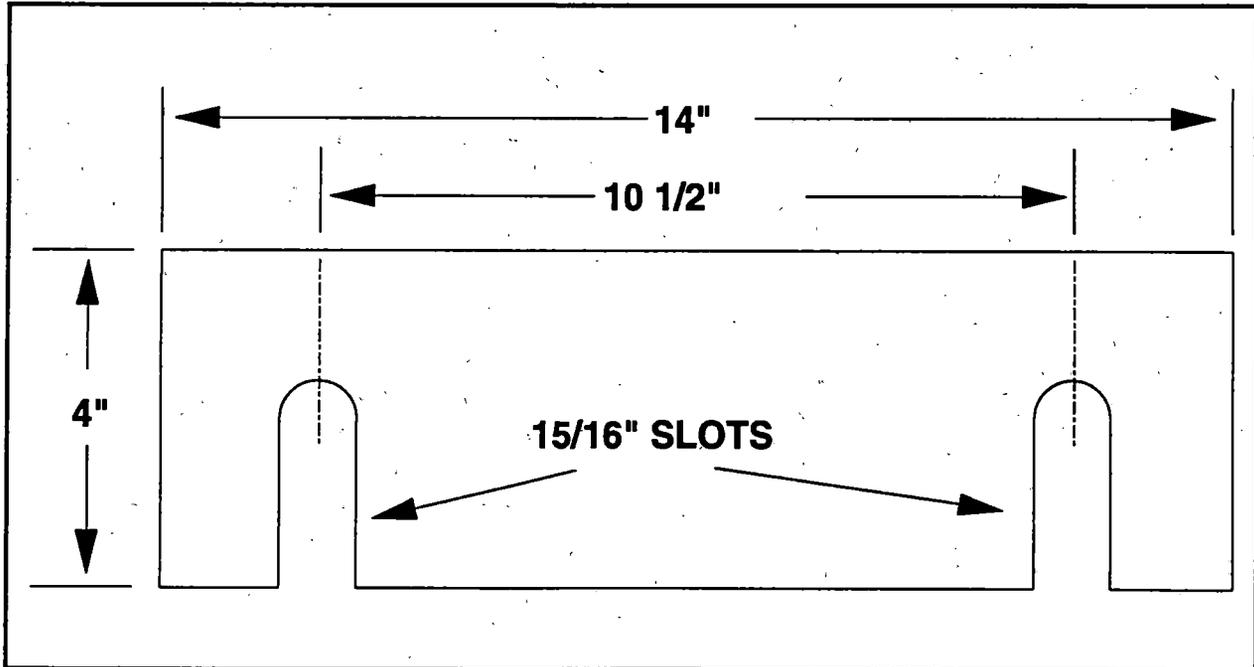
**Figure 4. Side Bearing Shim Design**
