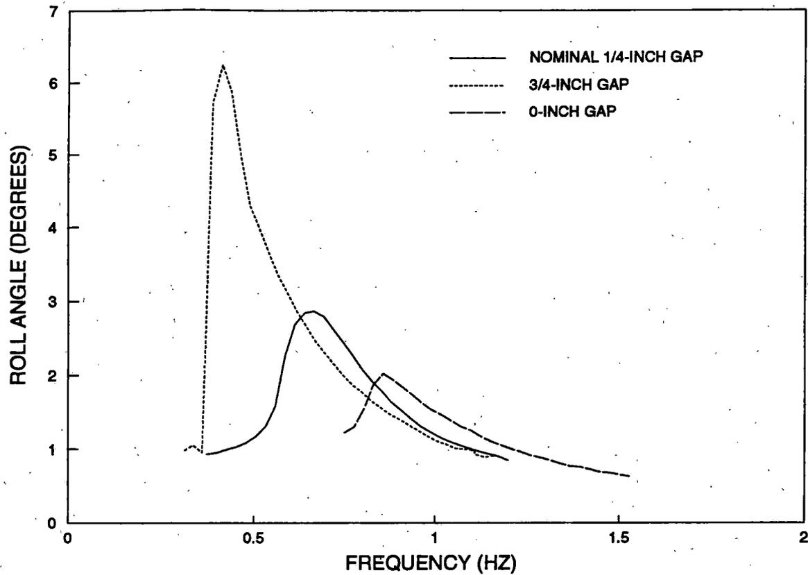
**Figure 21. Comparison of Car Body Roll Response for Test Configurations 1 (nominal), 7 (3/4-inch clearance), and 3 (zero clearance)**
