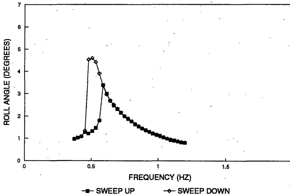
Figure 1. Example of Jump Response Phenomena in Car Body Roll
