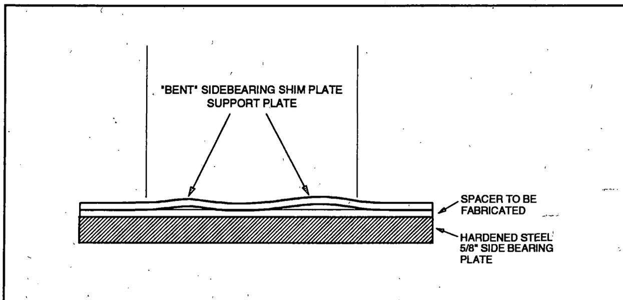
**Figure 2. Uneven Side Bearing Plate Support Surface to Be Repaired**
