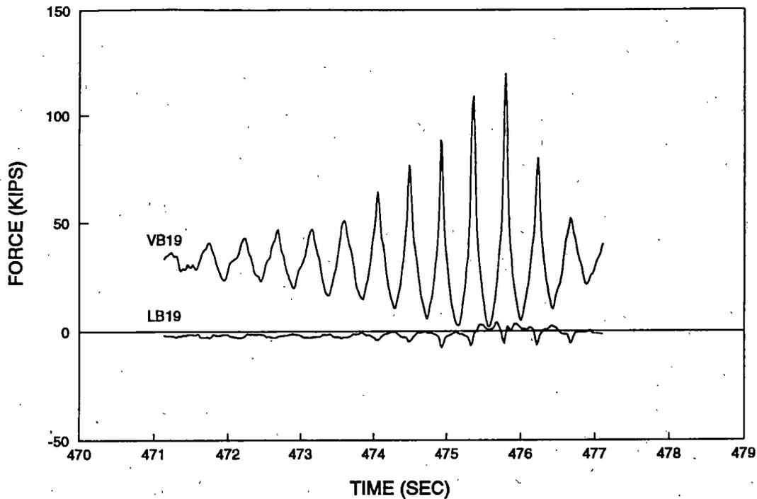
**Figure 38. P&B Test Configuration 1, Axle 1 Right Wheel -- Vertical & Lateral Wheel Force Time History Run 5**
