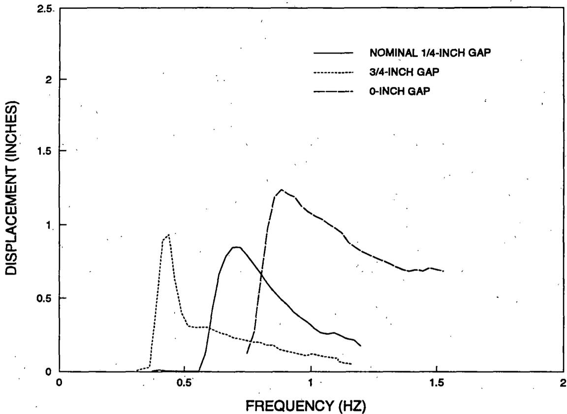
**Figure 22. Comparison of Spring Nest Displacement for VTU-Test Configurations 1 (nominal), 7 (3/4-inch clearance), and 3 (zero clearance)**
