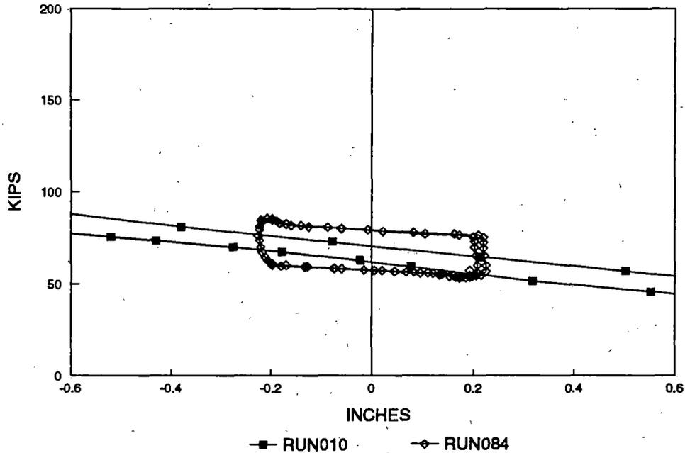
**Figure 11. Expanded Vertical Suspension Characteristics, Trucks 1 and 2, Runs 10 and 84**
