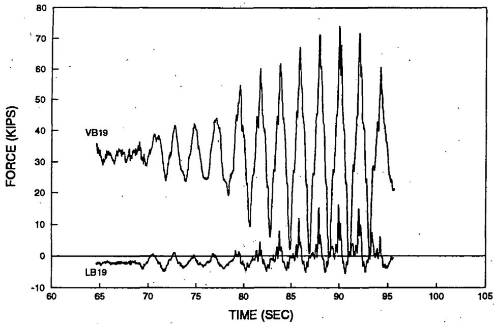
**Figure 32. T&R Test Configuration 7, Axle 1 Right Wheel – Vertical & Lateral Wheel Force Time History Run 39**
