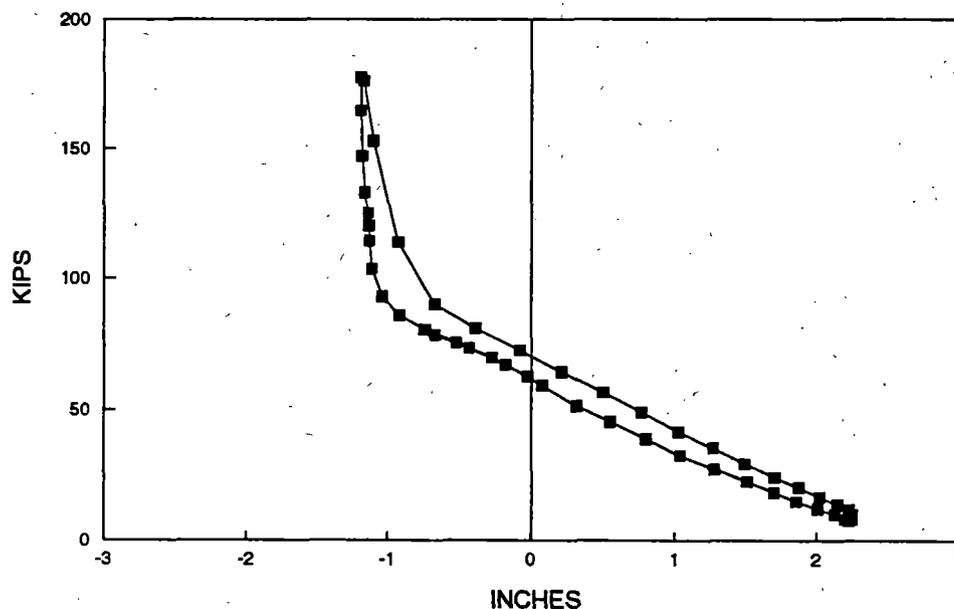
Figure 8. Truck 1 Vertical Suspension Characteristics, Run 10, B-end, Right Side
