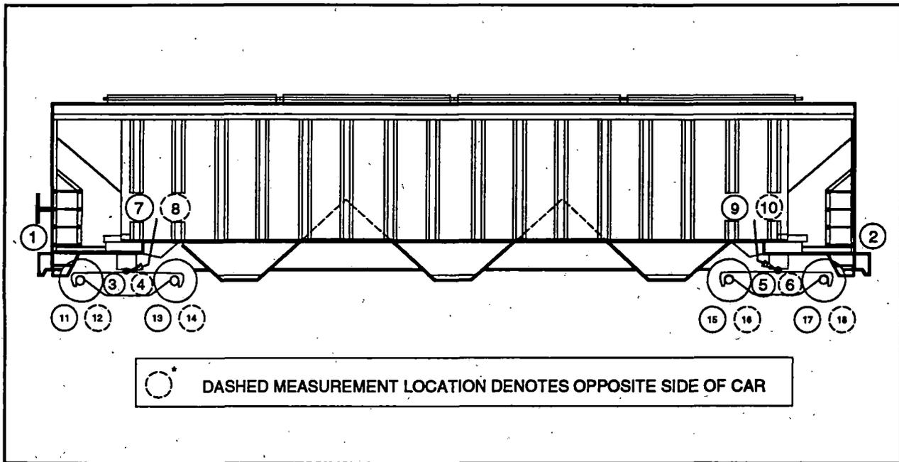
**Figure 6. VTU Test Measurement Locations**
