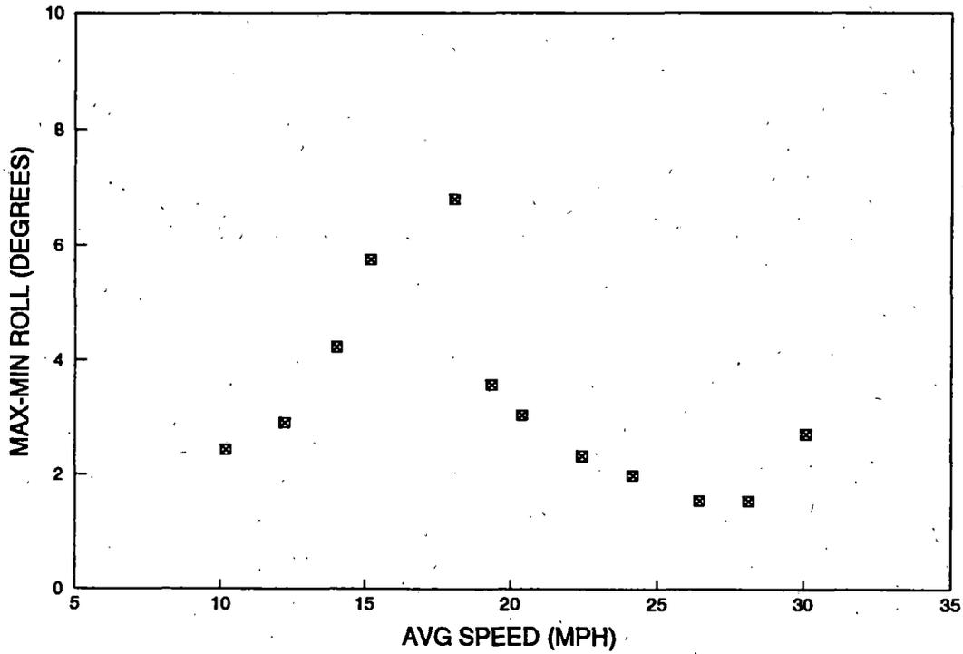
**Figure 28. T&R Test Configuration 1, A-End Car Body Roll Angle Versus Speed**
