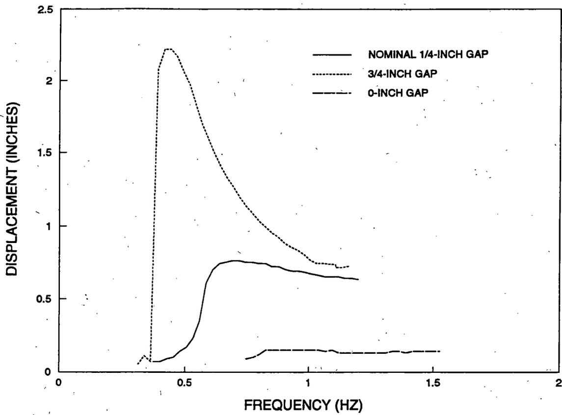
**Figure 23. Comparison of Displacement Across Side Bearing Gaps for VTU-Test Configurations 1 (nominal), 7 (3/4-inch clearance), and 3 (zero clearance)**
