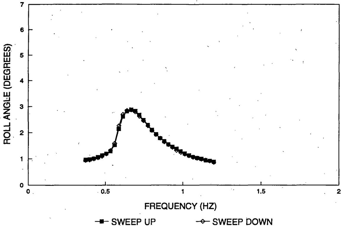
**Figure 12. Nominal 1/4-inch Side Bearing Clearance VTU Test Results (Configuration 1) – Truck 1, B-End Car Body Roll Angle Versus Frequency, 3/8" Peak-to-peak Cross Level VTU Excitation**
