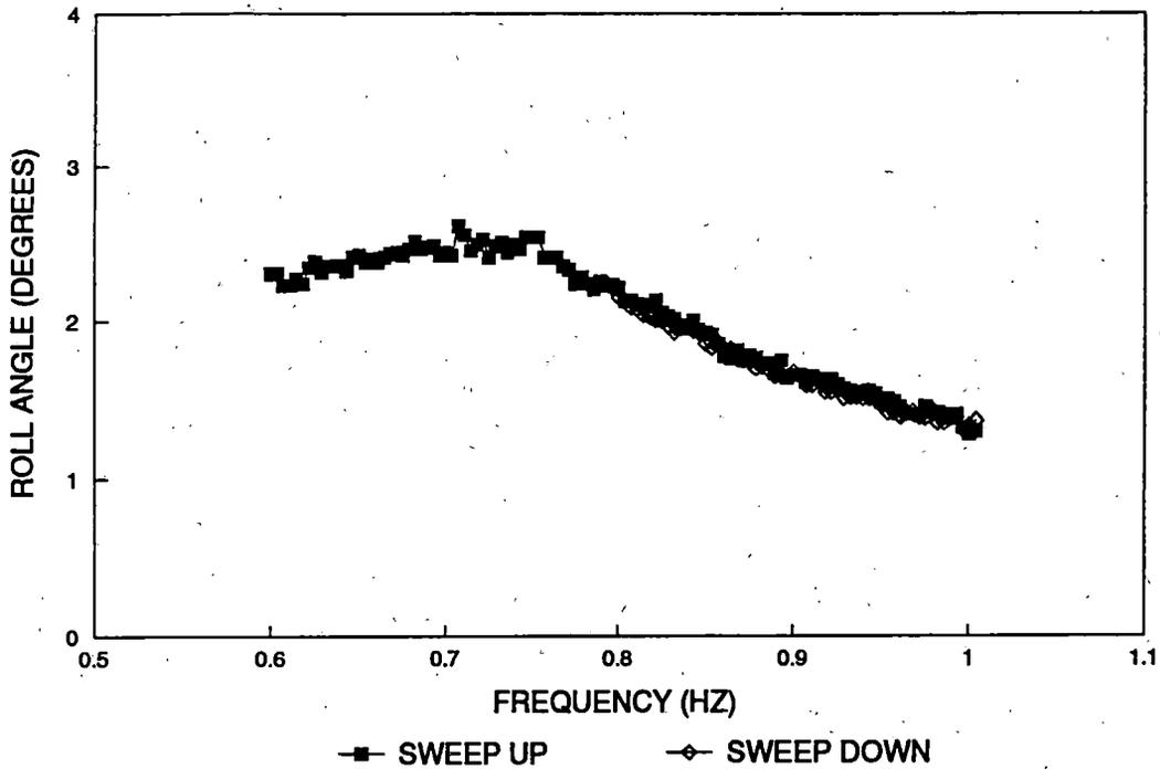
**Figure 18. Nominal 1/4-inch Side Bearing Clearance VTU Test Results (Configuration 11) -- Truck 2, B-End Car Body Roll Angle Versus Frequency, 13/32" Peak-to-peak Cross Level VTU Excitation**
