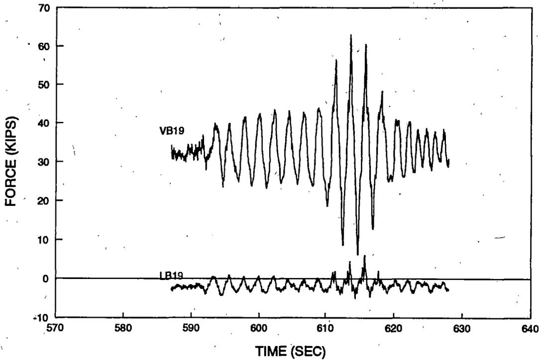
**Figure 33. T&R Test Configuration 7, Axle 1 Right Wheel – Vertical & Lateral Wheel Force Time History Run 25**
