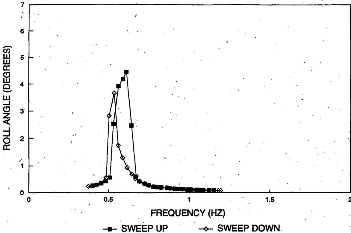
**Figure 17. Nominal 1/4-inch Side Bearing Clearance VTU Test Results, Snubbers Disabled (Configuration 2) -- Truck 1, B-End Car Body Roll Angle Versus Frequency, 1/16" Peak-to-peak Cross Level VTU Excitation**
