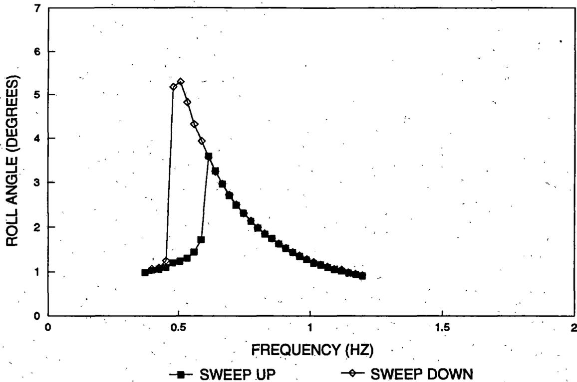
**Figure 15. Constant Contact Side Bearing VTU Test Results (Configuration 9) – Truck 1, B-End Car Body Roll Angle Versus Frequency, 13/32" Peak-to-peak Cross Level VTU Excitation**
