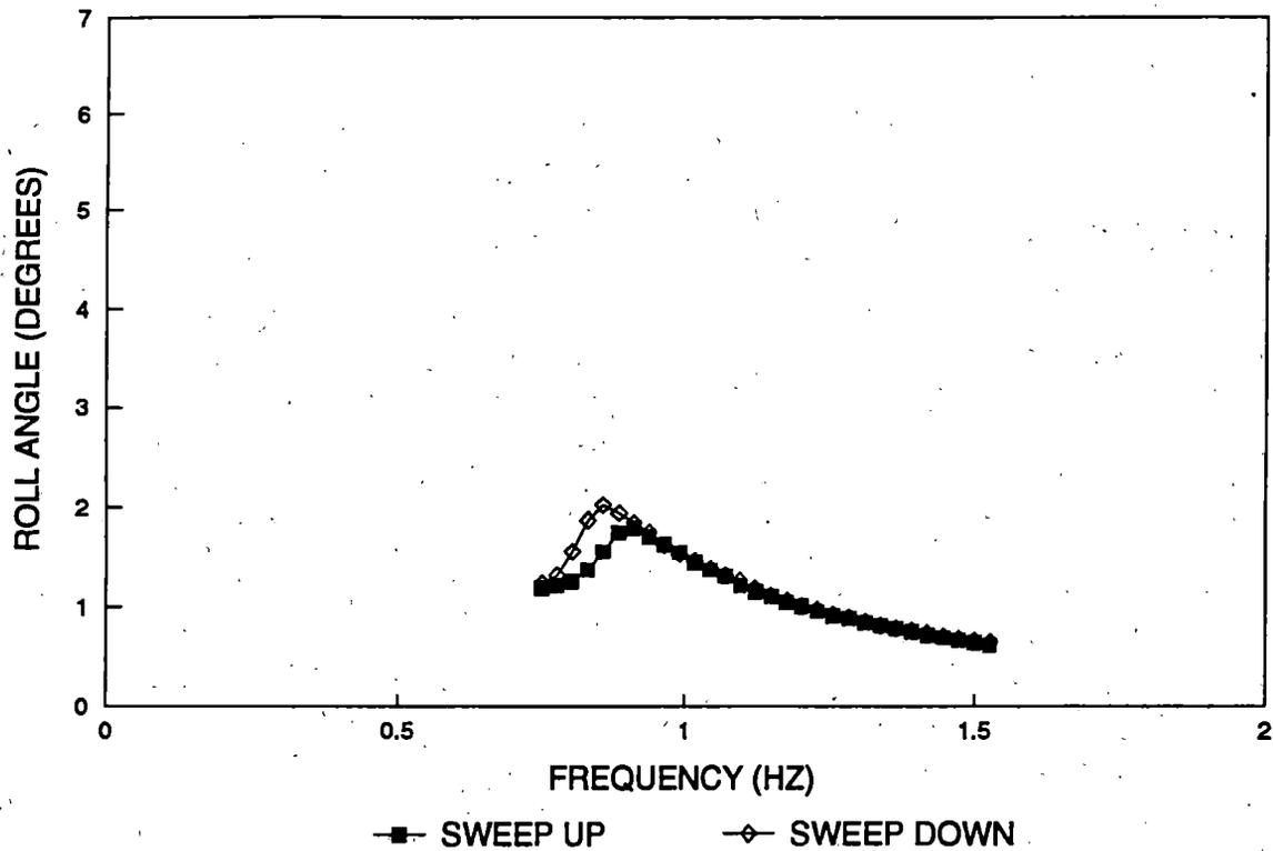
**Figure 16. Zero Side Bearing Clearance VTU Test Results (Configuration 3) -- Truck 1, B-End Car Body Roll Angle Versus Frequency, 3/8" Peak-to-peak Cross Level VTU Excitation**
