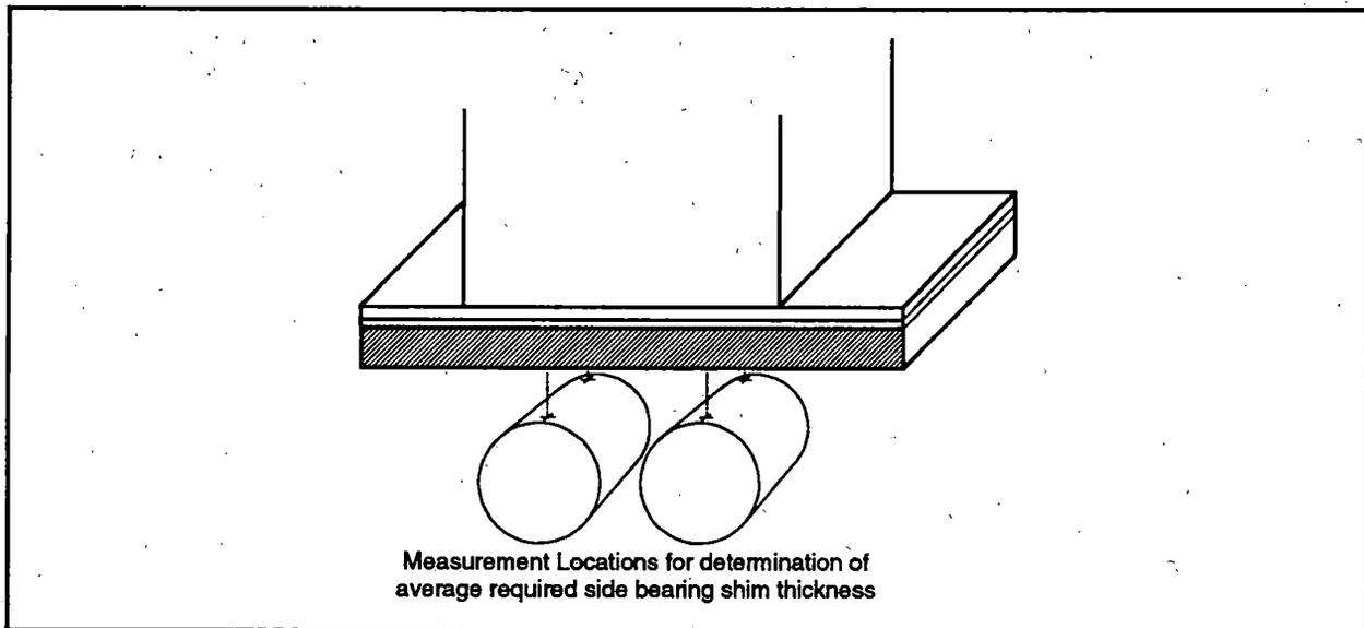
**Figure 3. Locations Measured to Determine Side Bearing Shim Thickness**
