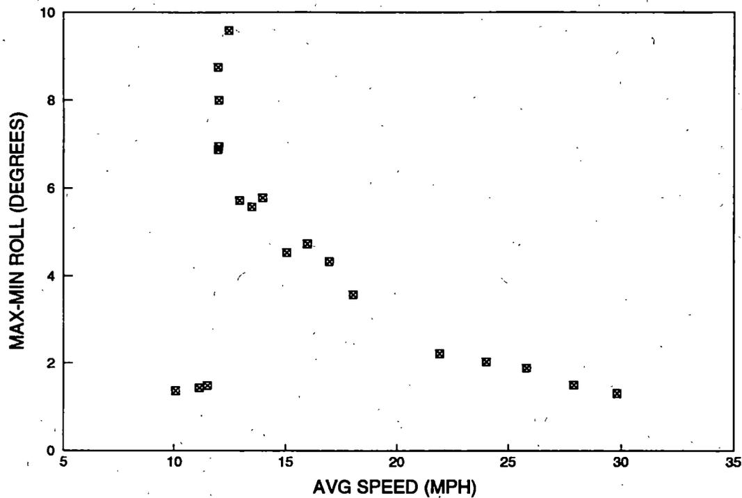
**Figure 34. T&R Test Configuration 7, A-End Car Body Roll Angle Versus Speed**
