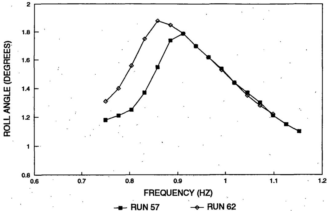
**Figure 20. Zero Side Bearing Clearance VTU Test Results (Configuration 3) -- Truck 2, B-End Car Body Roll Angle Versus Frequency, 3/8" Peak-to-peak Cross Level VTU Excitation**
