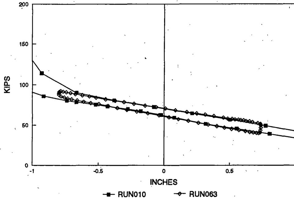
**Figure 9. Expanded Vertical Suspension Characteristics, Runs 10 and 63, B-end, Right Side**
