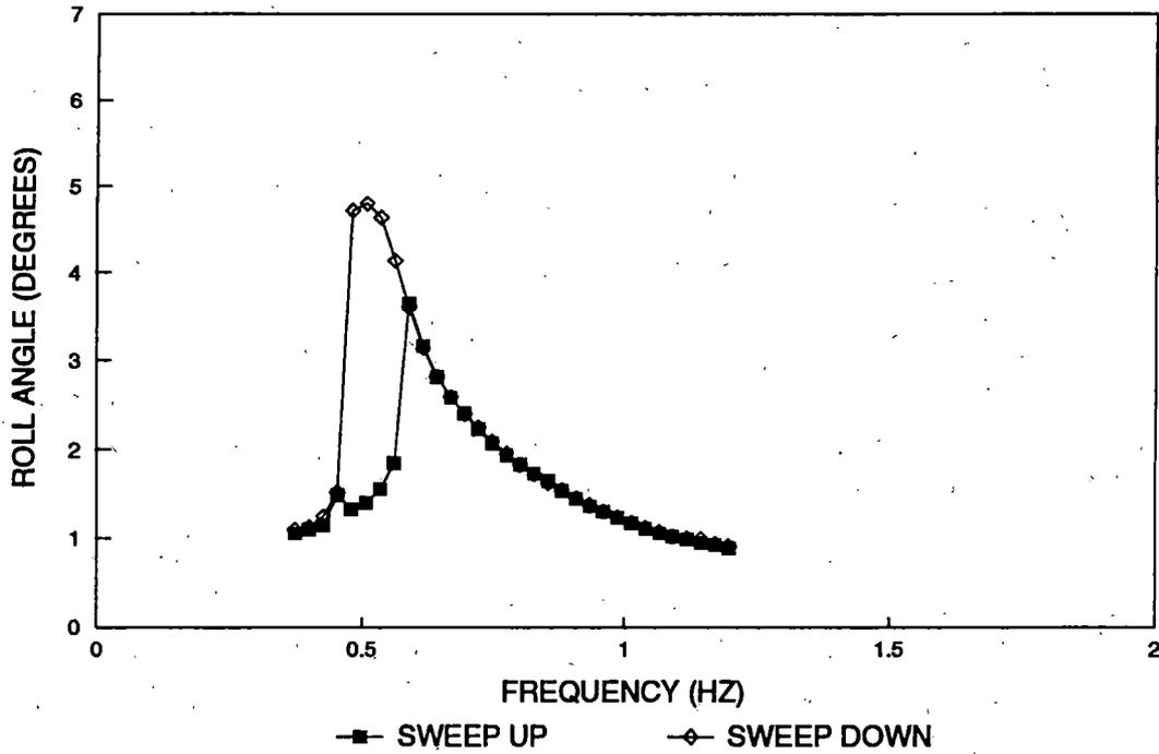
**Figure 13. 1/2-inch Side Bearing Clearance VTU Test Results (Configuration 5) -- Truck 1, B-End Car Body Roll Angle Versus Frequency, 13/32" Peak-to-peak Cross Level VTU Excitation**
