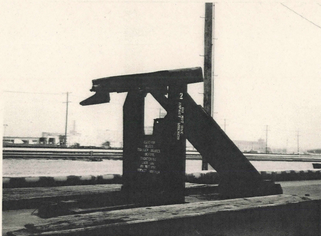
E - 11 Wrench operated retractable hitch with screw type locking plate.
