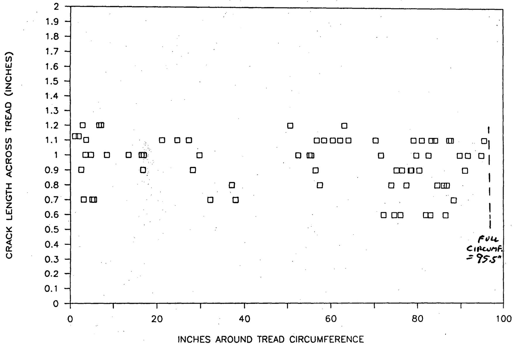
**TABLE 2: WHEEL #1501 CRACK INCIDENCE**
