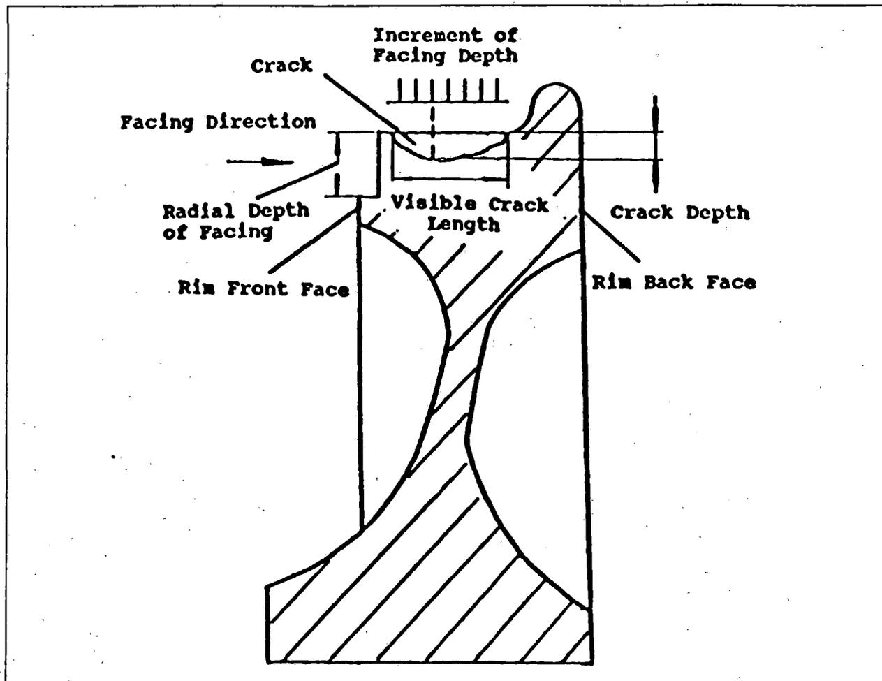
**Figure 1: Wheel Peeling Procedure**
