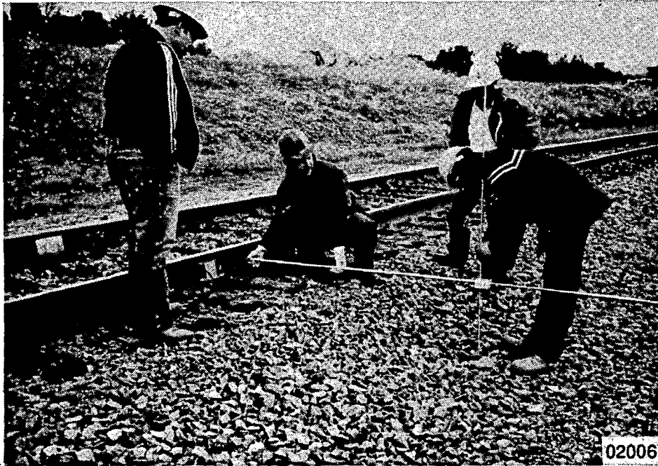
Figure 2-3. Radial Measurement Device
