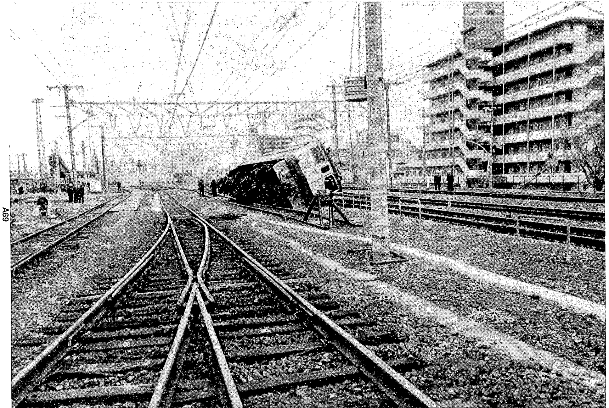
HC-3. Hankyu Corporation passenger car derailed from its out-of-service siding. Notice the buildings appear undamaged. (photo courtesy of M. Yashinsky)
