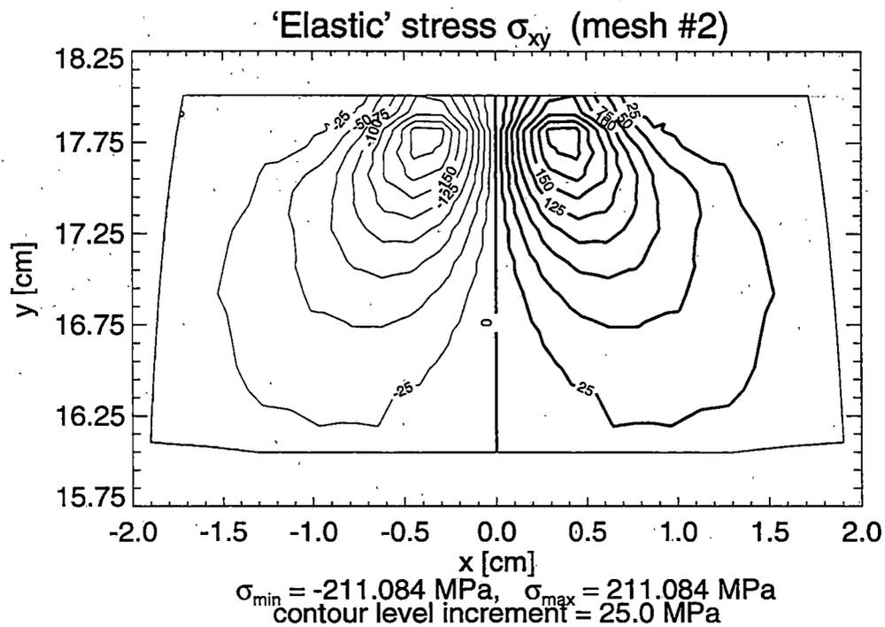
**Figure 2.35** Contour Lines of Normal  $\sigma_{zz}$  and Shear  $\sigma_{xy}$  'Elastic' Stresses in the Railroad Rail under Vertical Loading – Solution for Mesh #2
