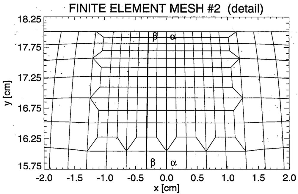
**Figure 2.21 Finite Element Mesh #2 in the Problem of a Railroad Rail under Contact Loading – Head and Detail**
