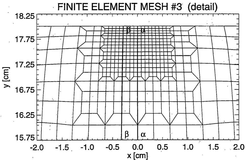
**Figure 2.22 Finite Element Mesh #3 in the Problem of a Railroad Rail under Contact Loading – Head and Detail**
