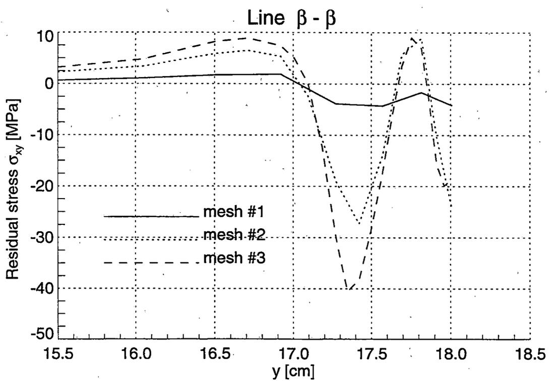
Figure 3.2 Normal  $\sigma_{zz}$  and Shear  $\sigma_{xy}$  Residual Stresses in the Railroad Rail under Vertical Loading (Loading Case #1)
