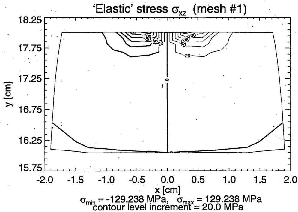
**Figure 2.43 Contour Lines of Shear 'Elastic' Stresses  $\sigma_{yz}$  and  $\sigma_{xz}$  in the Railroad Rail under Horizontal Loading – Solution for Mesh #1**
