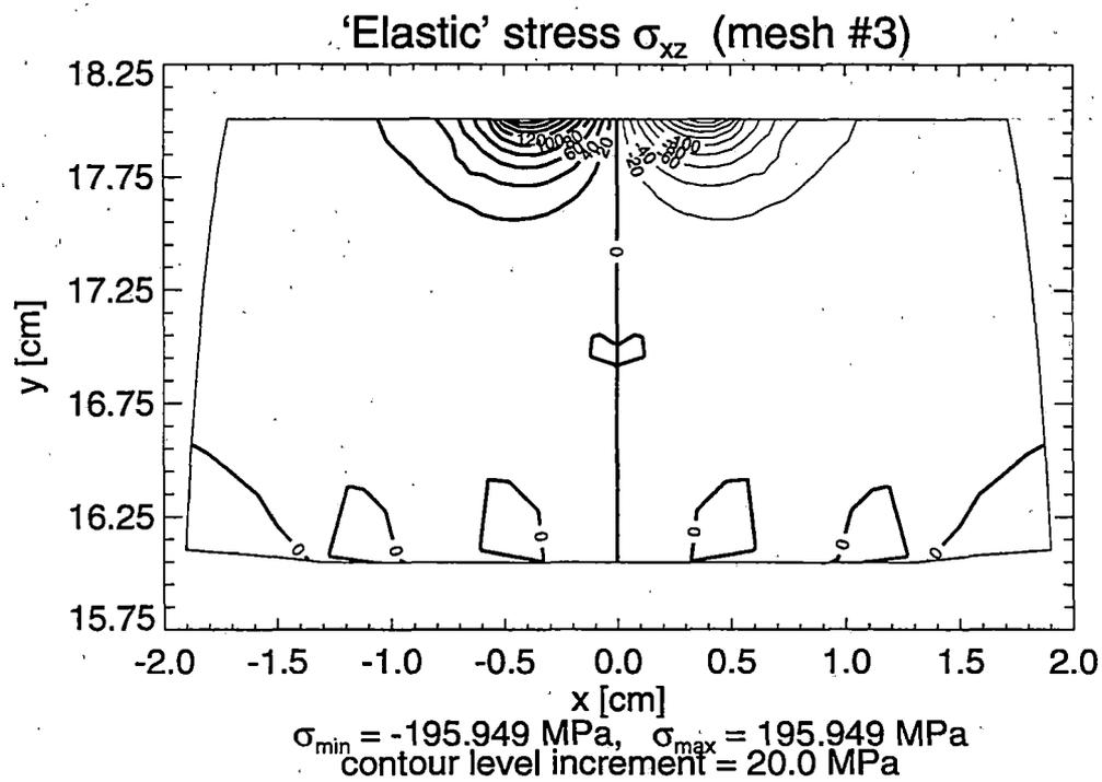
**Figure 2.45 Contour Lines of Shear 'Elastic' Stresses  $\sigma_{yz}$  and  $\sigma_{xz}$  in the Railroad Rail under Horizontal Loading Solution for Mesh #3**
