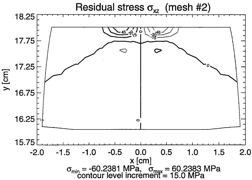
**Figure 3.11 Contour Lines of Shear Residual Stresses  $\sigma_{yz}$  and  $\sigma_{xz}$  in the Railroad Rail under Vertical and Horizontal Loading (Loading Case #2) – Solution for Mesh #2**
