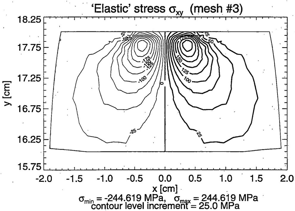
**Figure 2.36 Contour Lines of Normal  $\sigma_{zz}$  and Shear  $\sigma_{xy}$  'Elastic' Stresses in the Railroad Rail under Vertical Loading – Solution for Mesh #3**
