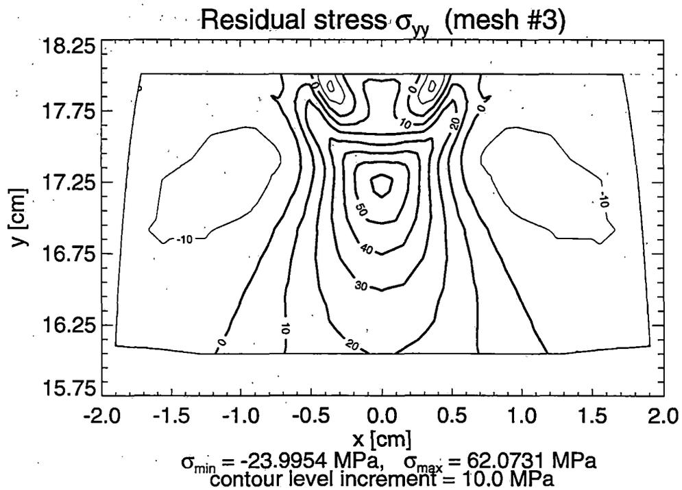
**Figure 3.8 Contour Lines of Normal Residual Stresses  $\sigma_{xx}$  and  $\sigma_{yy}$  in the Railroad Rail under Vertical and Horizontal Loading (Loading Case #2) – Solution for Mesh #3**
