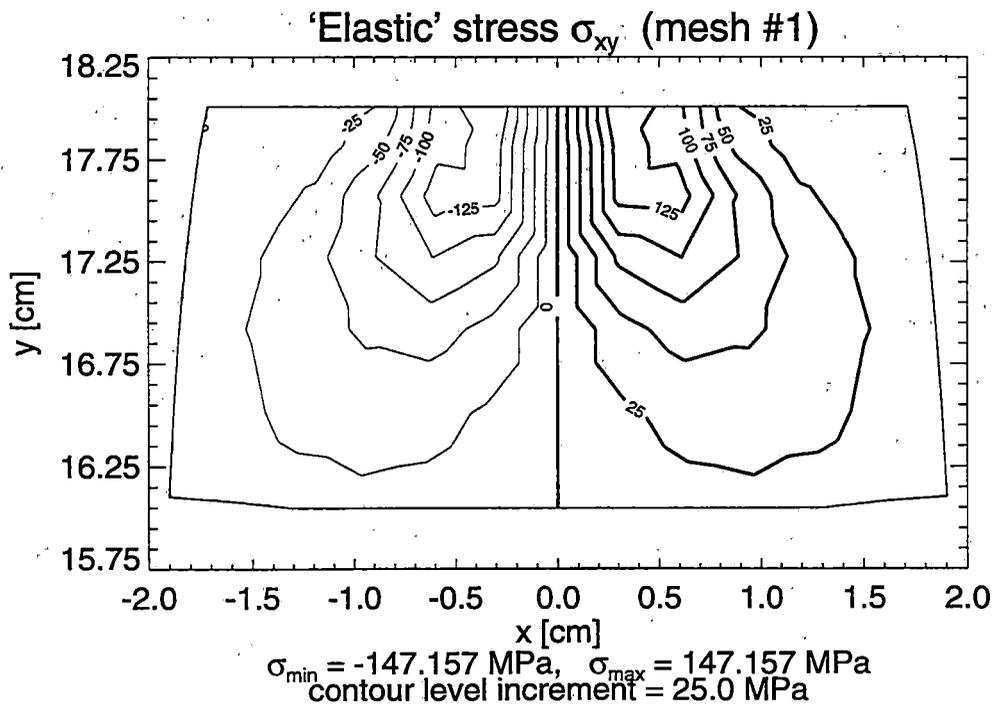
**Figure 2.34 Contour Lines of Normal  $\sigma_{zz}$  and Shear  $\sigma_{xy}$  'Elastic' Stresses in the Railroad Rail under Vertical Loading – Solution for Mesh #1**
