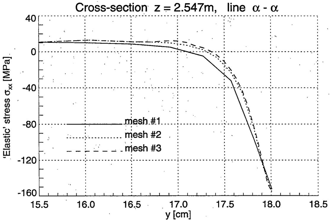
Figure 2.23 Normal 'Elastic' Stresses  $\sigma_{xx}$  in the Railroad Rail under Vertical Loading
