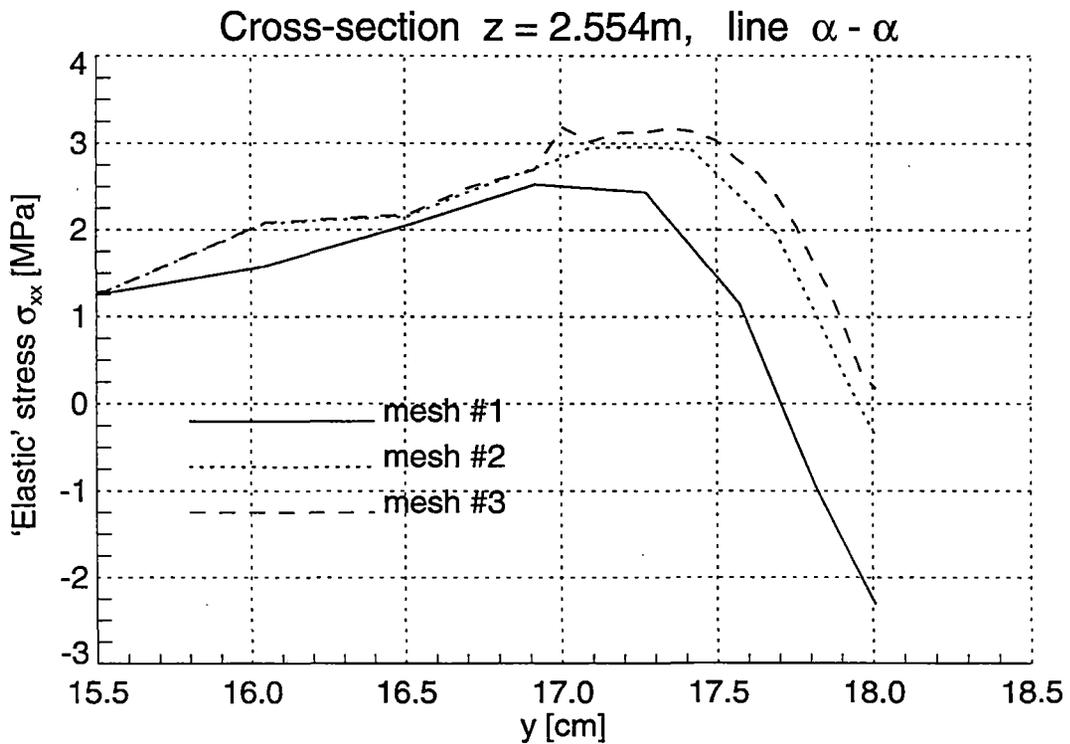
Figure 2.37 Normal 'Elastic' Stresses  $\sigma_{xx}$  in the Railroad Rail under Horizontal Loading
