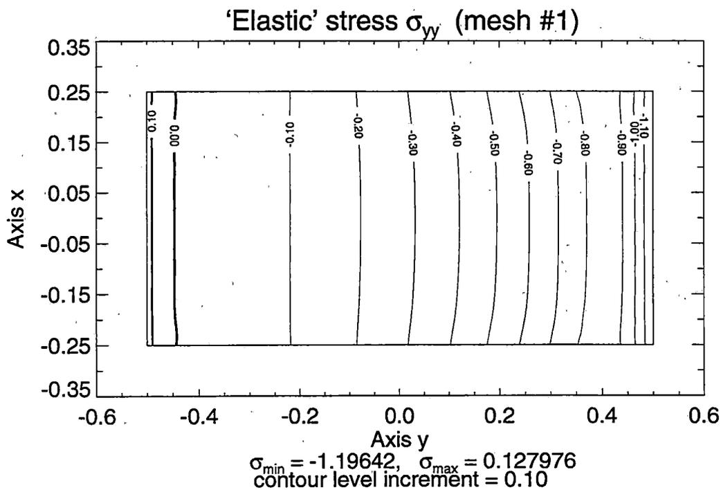
**Figure 2.10 Contour Lines of Normal 'Elastic' Stresses  $\sigma_{xx}$  and  $\sigma_{yy}$  in the Simply Supported Beam under Vertical Surface Traction – Solution for Mesh #1**
