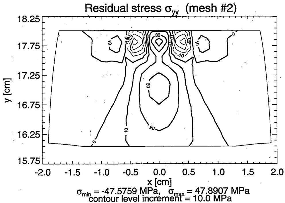
**Figure 3.3 Contour Lines of Normal Residual Stresses  $\sigma_{xx}$  and  $\sigma_{yy}$  in the Railroad Rail under Vertical Loading (Loading Case #1) – Solution for Mesh #2**
