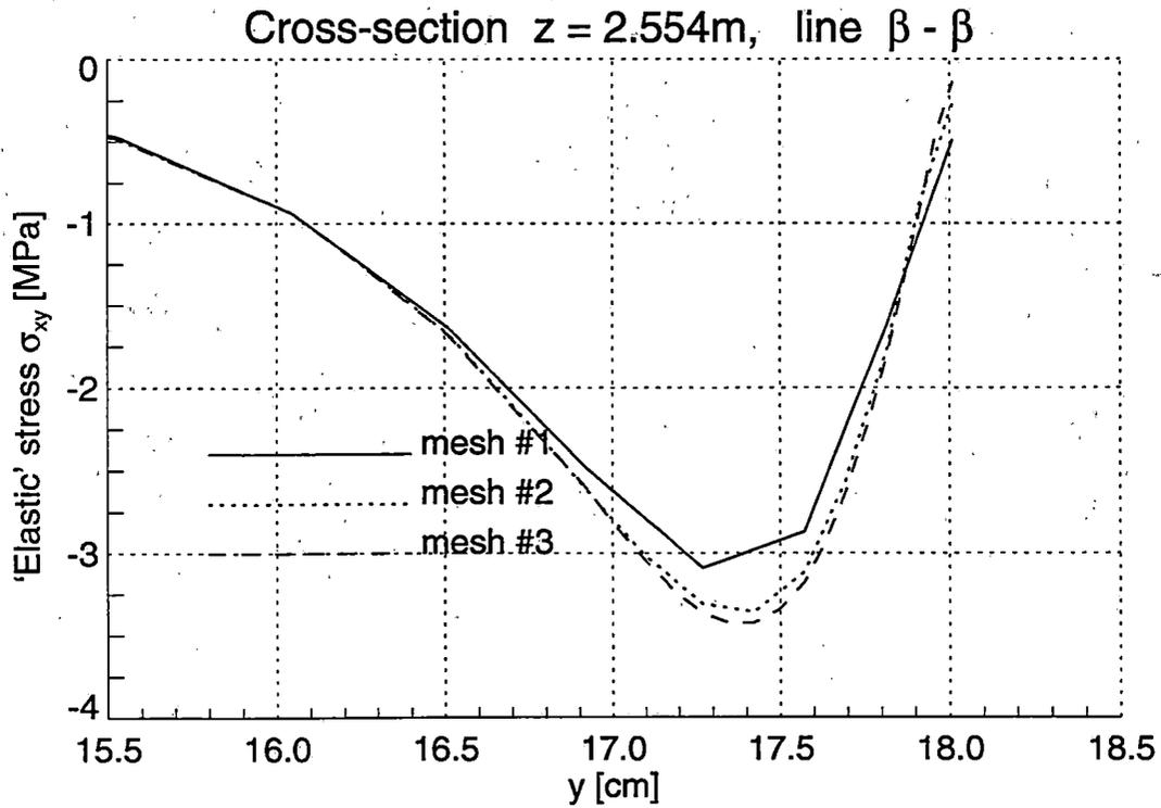
Figure 2.40 Shear 'Elastic' Stresses  $\sigma_{xy}$  in the Railroad Rail under Horizontal Loading
