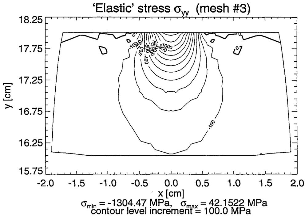
**Figure 2.33** Contour Lines of Normal 'Elastic' Stresses  $\sigma_{xx}$  and  $\sigma_{yy}$  in the Railroad Rail under Vertical Loading – Solution for Mesh #3
