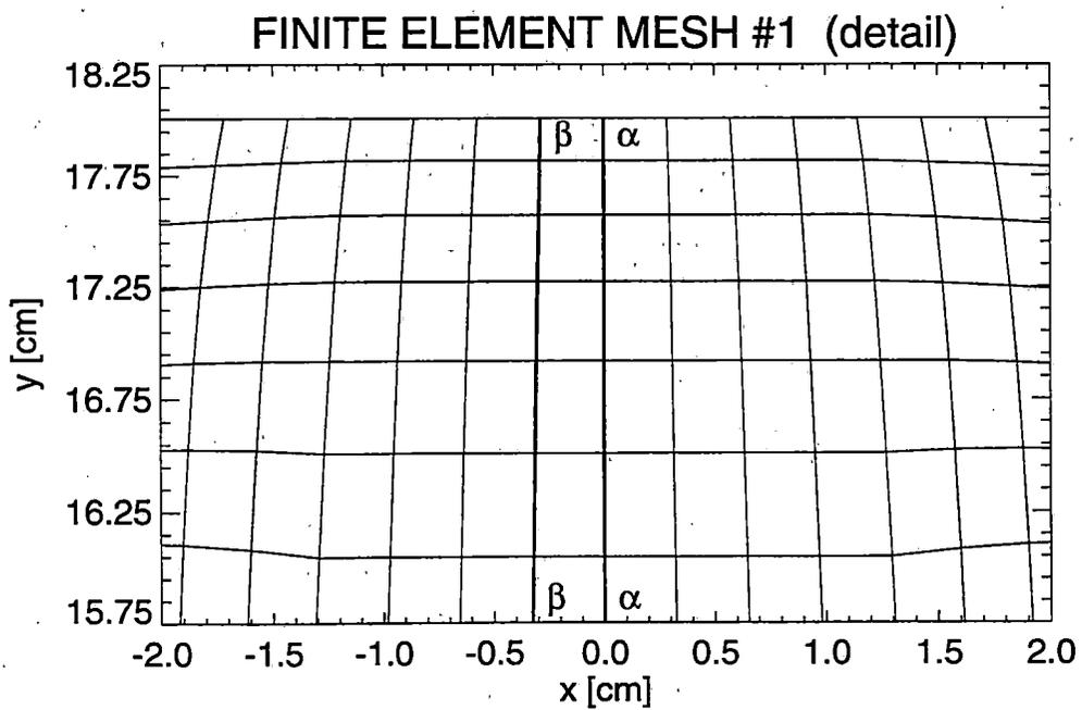
**Figure 2.20 Finite Element Mesh #1 in the Problem of a Railroad Rail under Contact Loading – Head and Detail**
