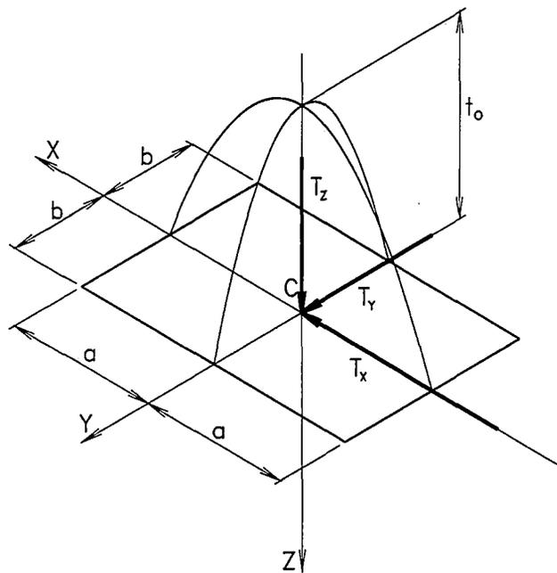
Figure 2.4 Conventions for a Rectangular Contact Zone with Bi-Parabolic Distribution of Surface Traction
