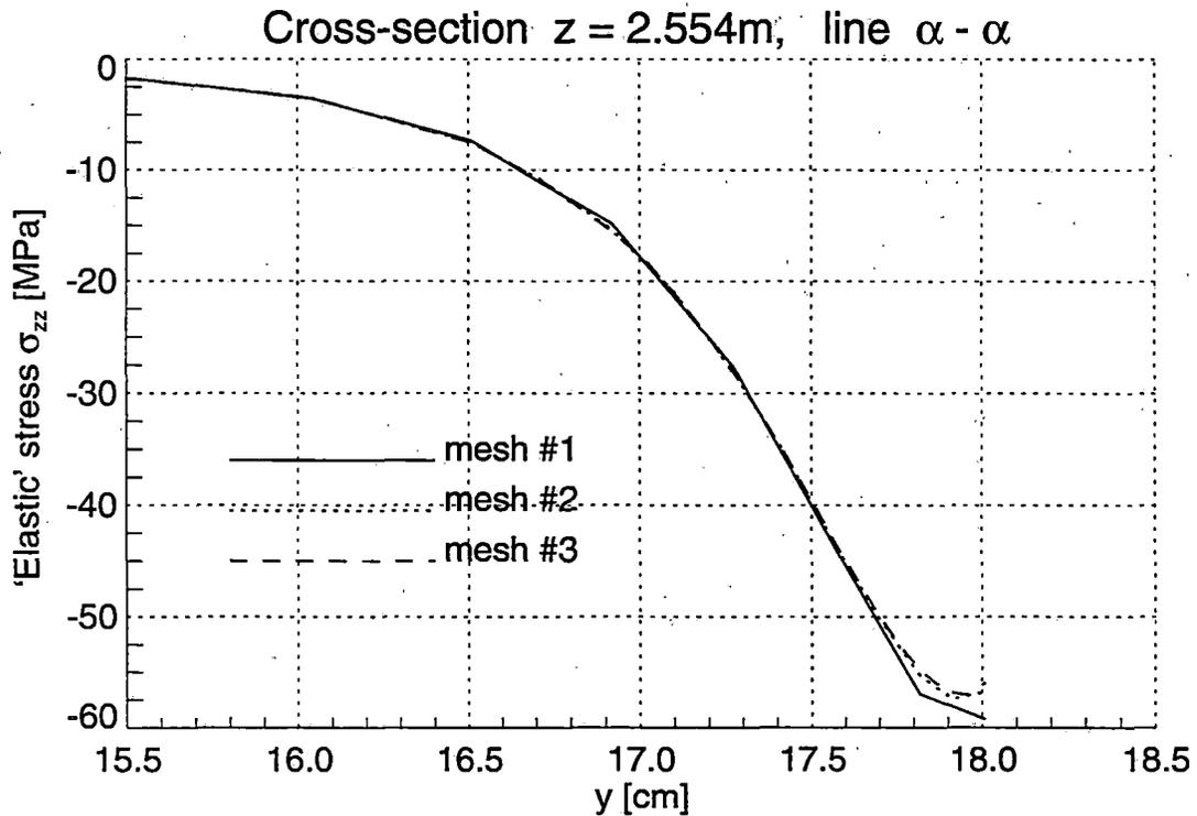
Figure 2.39 Normal 'Elastic' Stresses  $\sigma_{zz}$  in the Railroad Rail under Horizontal Loading
