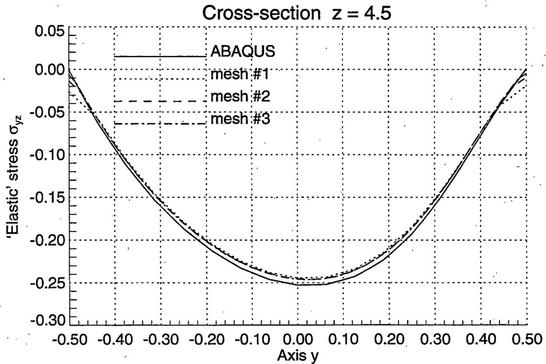
Figure 2.9 Shear 'Elastic' Stresses  $\sigma_{yz}$  in the Simply Supported Beam under Concentrated Vertical Surface Traction
