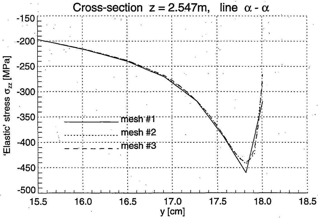
Figure 2.25 Normal 'Elastic' Stresses  $\sigma_{zz}$  in the Railroad Rail under Vertical Loading
