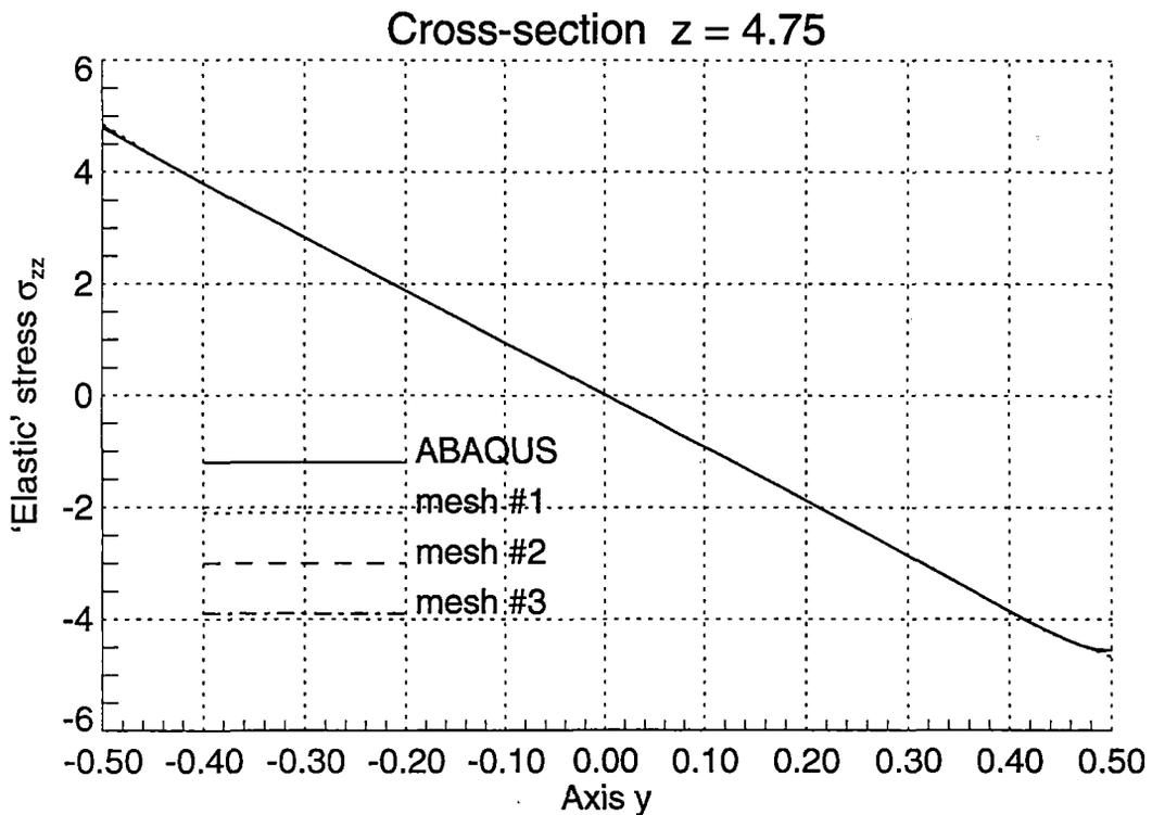
**Figure 2.8 Normal 'Elastic' Stresses  $\sigma_{zz}$  in the Simply Supported Beam under Concentrated Vertical Surface Tractions**
