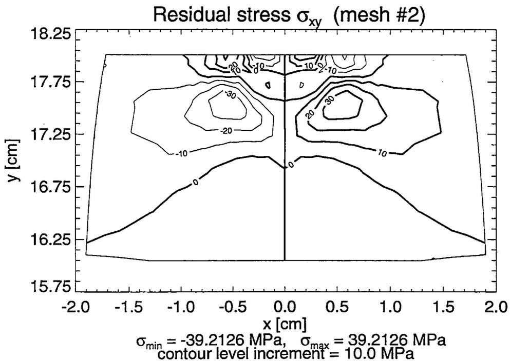
**Figure 3.5 Contour Lines of Normal  $\sigma_{zz}$  and Shear  $\sigma_{xy}$  Residual Stresses in the Railroad Rail under Vertical Loading (Loading Case #1) – Solution for Mesh #2**
