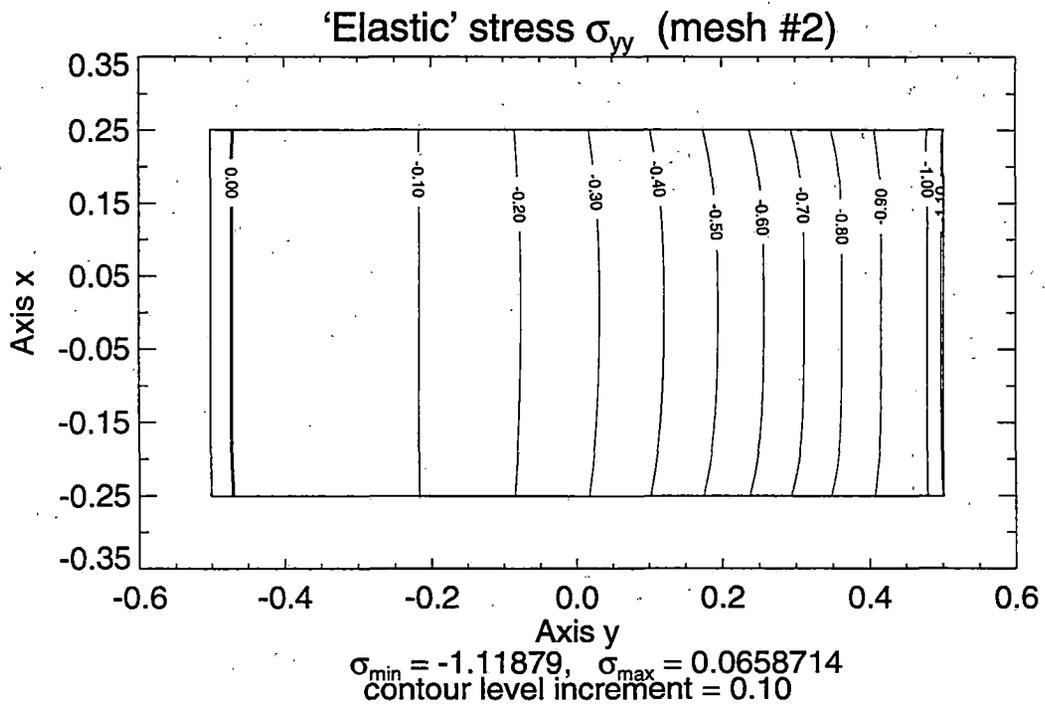
**Figure 2.11 Contour Lines of Normal 'Elastic' Stresses  $\sigma_{xx}$  and  $\sigma_{yy}$  in the Simply Supported Beam under Vertical Surface Tractions – Solution for Mesh #2**
