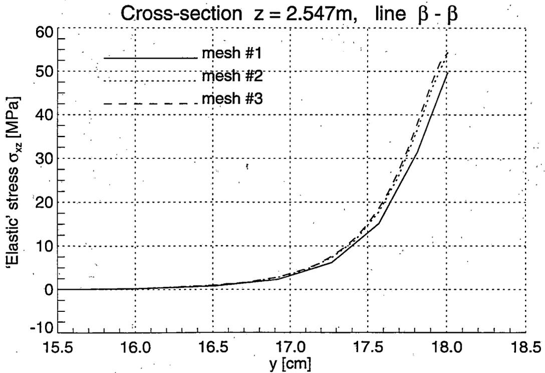
Figure 2.42 Shear 'Elastic' Stresses  $\sigma_{xz}$  in the Railroad Rail under Horizontal Loading
