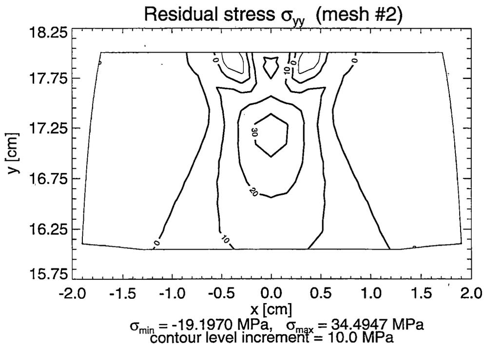
**Figure 3.7 Contour Lines of Normal Residual Stresses  $\sigma_{xx}$  and  $\sigma_{yy}$  in the Railroad Rail under Vertical and Horizontal Loading (Loading Case #2) – Solution for Mesh #2**
