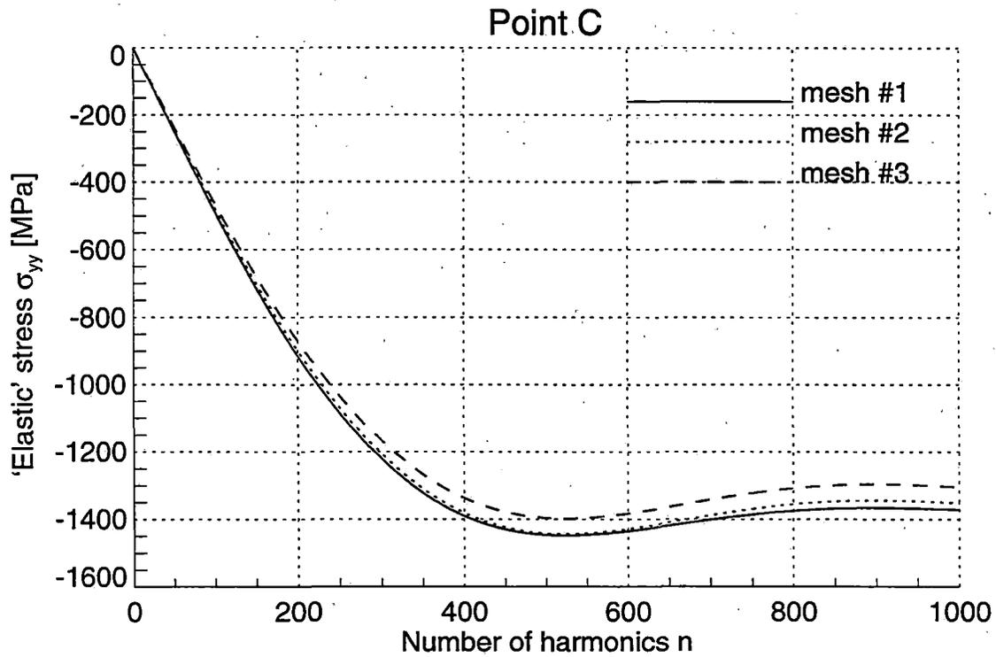
**Figure 2.29 Normal 'Elastic' Stresses  $\sigma_{xx}$  and  $\sigma_{yy}$  as a Function of the Number of Fourier Modes in the Railroad Rail under Vertical Loading**
