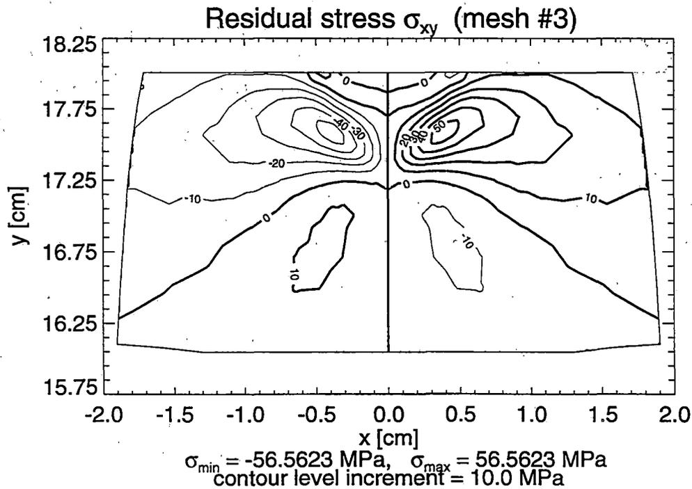
**Figure 3.10 Contour Lines of Normal  $\sigma_{zz}$  and Shear  $\sigma_{xy}$  Residual Stresses in the Railroad Rail under Vertical and Horizontal Loading (Loading Case #2) – Solution for Mesh #3**
