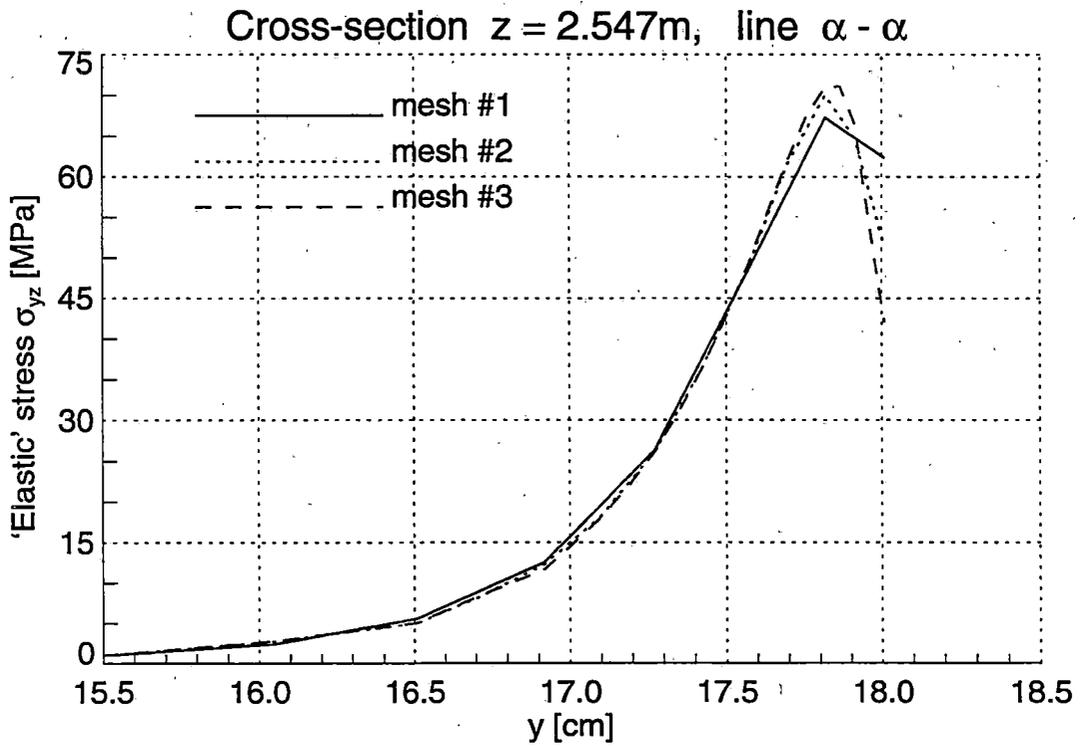
Figure 2.41 Shear 'Elastic' Stresses  $\sigma_{yz}$  in the Railroad Rail under Horizontal Loading
