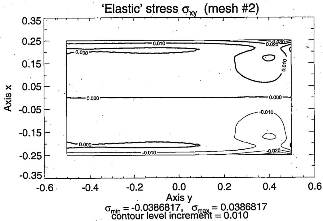
**Figure 2.14 Contour Lines of Normal  $\sigma_{zz}$  and Shear  $\sigma_{xy}$  'Elastic' Stresses in the Simply Supported Beam under Vertical Surface Tractions – Solution for Mesh #2**
