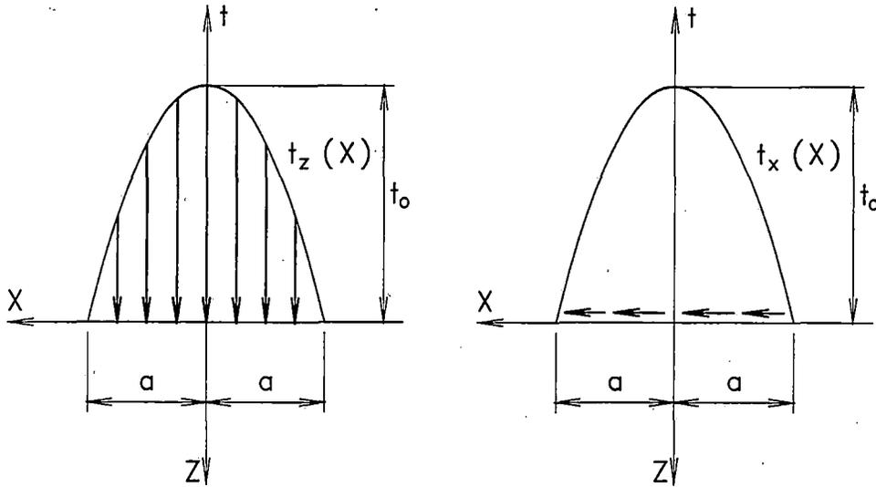
**Figure 2.6 Vertical and Horizontal Surface Traction in the Simply Supported Beam Problem**
