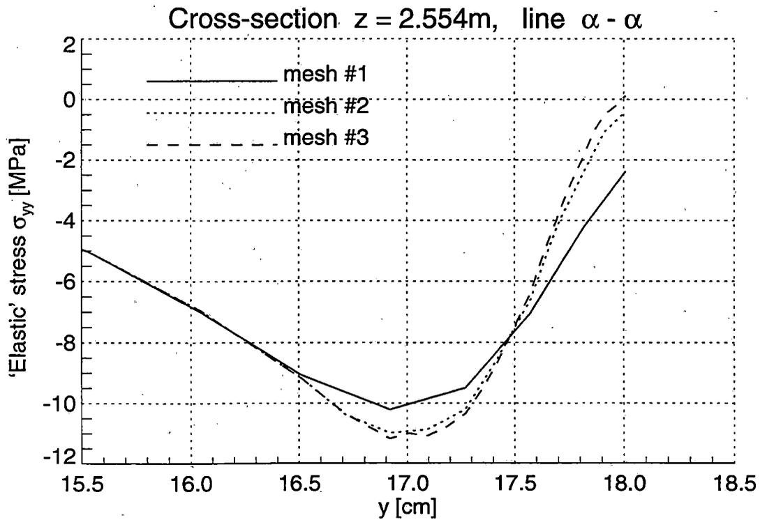
Figure 2.38 Normal 'Elastic' Stresses  $\sigma_{yy}$  in the Railroad Rail under Horizontal Loading
