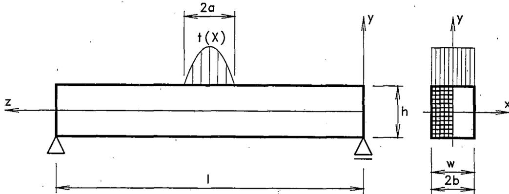
**Figure 2.5 Simply Supported Beam under Concentrated Surface Traction**
