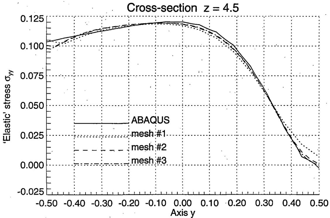
Figure 2.16 Normal 'Elastic' Stresses  $\sigma_{yy}$  in the Simply Supported Beam under Concentrated Horizontal Surface Traction
