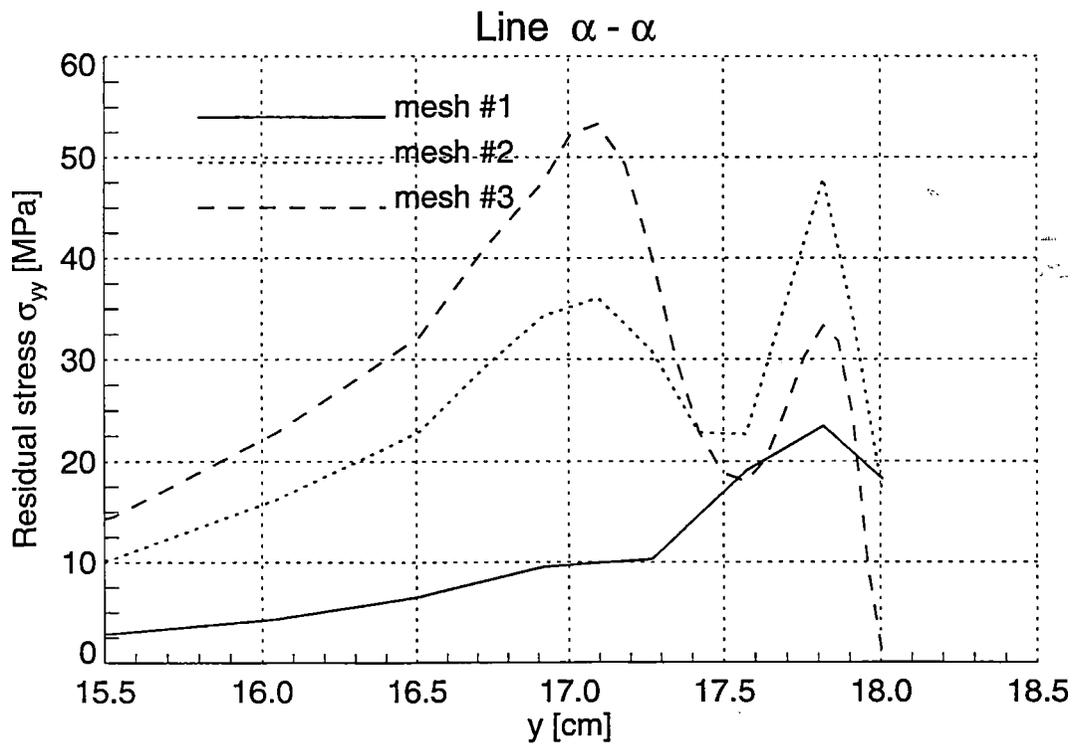
Figure 3.1 Normal Residual Stresses  $\sigma_{xx}$  and  $\sigma_{yy}$  in the Railroad Rail under Vertical Loading (Loading Case #1)
