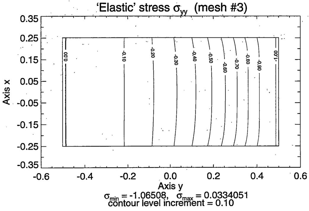
**Figure 2.12 Contour Lines of Normal 'Elastic' Stresses  $\sigma_{xx}$  and  $\sigma_{yy}$  in the Simply Supported Beam under Vertical Surface Traction – Solution for Mesh #3**
