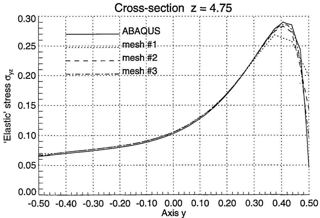
Figure 2.18 Shear 'Elastic' Stresses  $\sigma_{yz}$  in the Simply Supported Beam under Concentrated Horizontal Surface Traction
