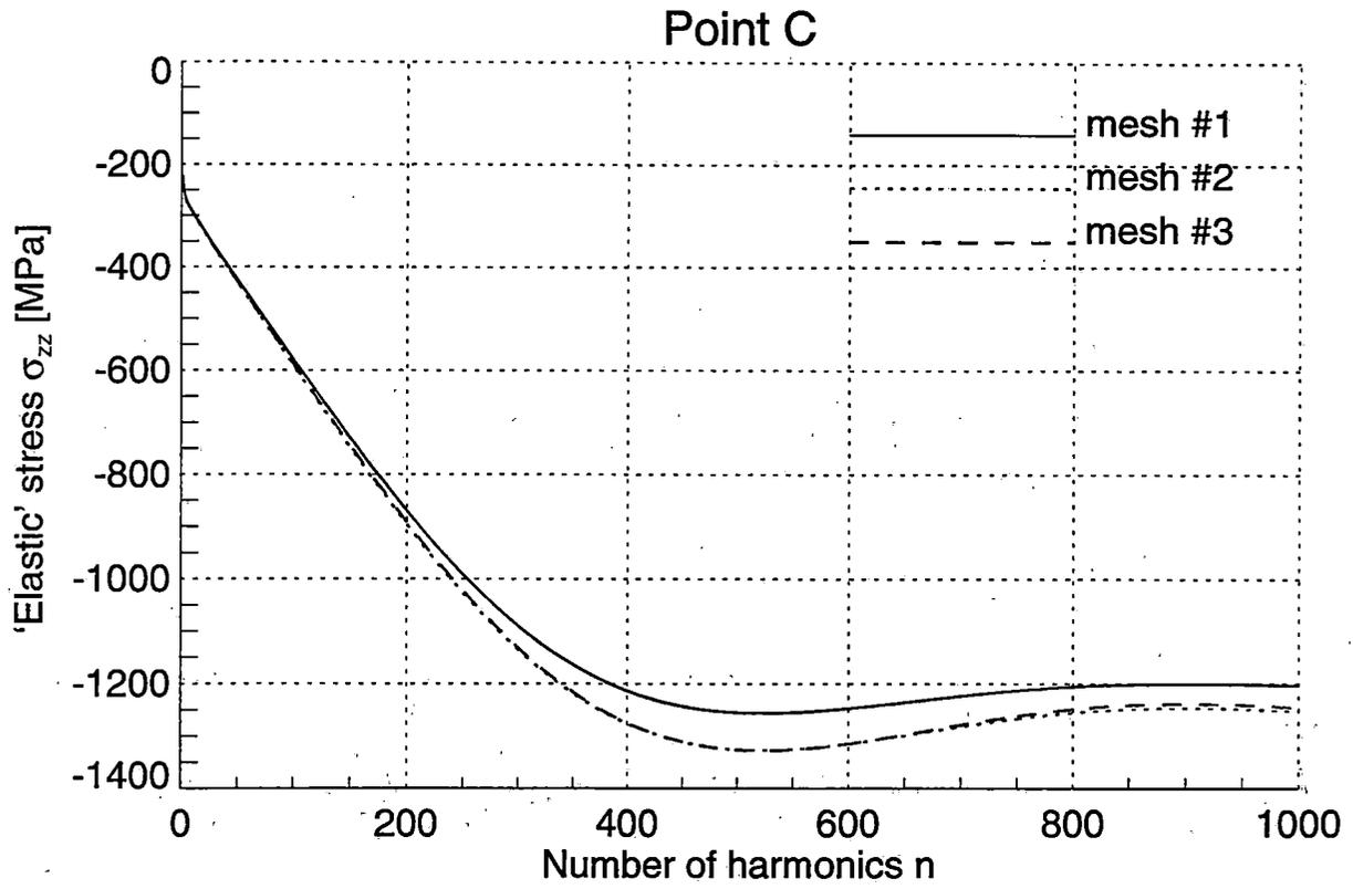
**Figure 2.30 Normal 'Elastic' Stresses  $\sigma_{zz}$  as a Function of the Number of Fourier Modes in the Railroad Rail under Vertical Loading**
