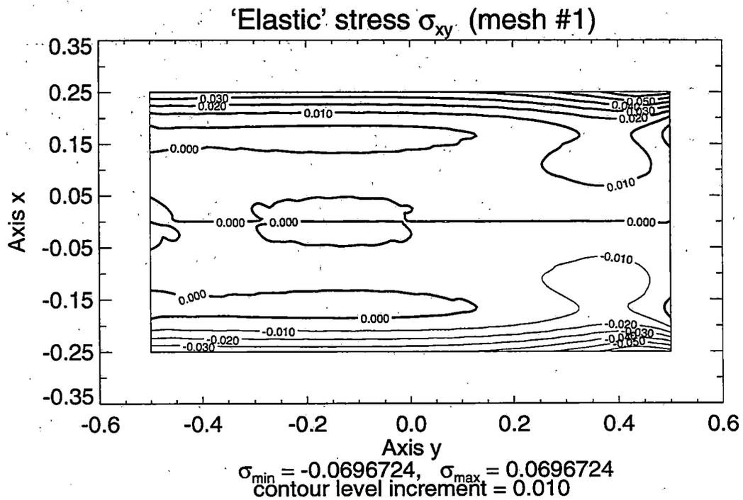
**Figure 2.13 Contour Lines of Normal  $\sigma_{zz}$  and Shear  $\sigma_{xy}$  'Elastic' Stresses in the Simply Supported Beam under Vertical Surface Traction – Solution for Mesh #1**
