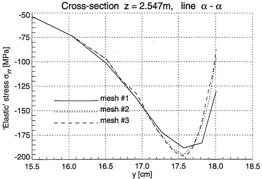
Figure 2.24 Normal 'Elastic' Stresses  $\sigma_{yy}$  in the Railroad Rail under Vertical Loading
