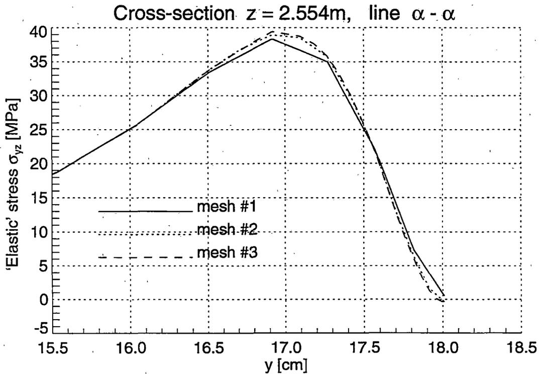
Figure 2.27 Shear 'Elastic' Stresses  $\sigma_{yz}$  in the Railroad Rail under Vertical Loading
