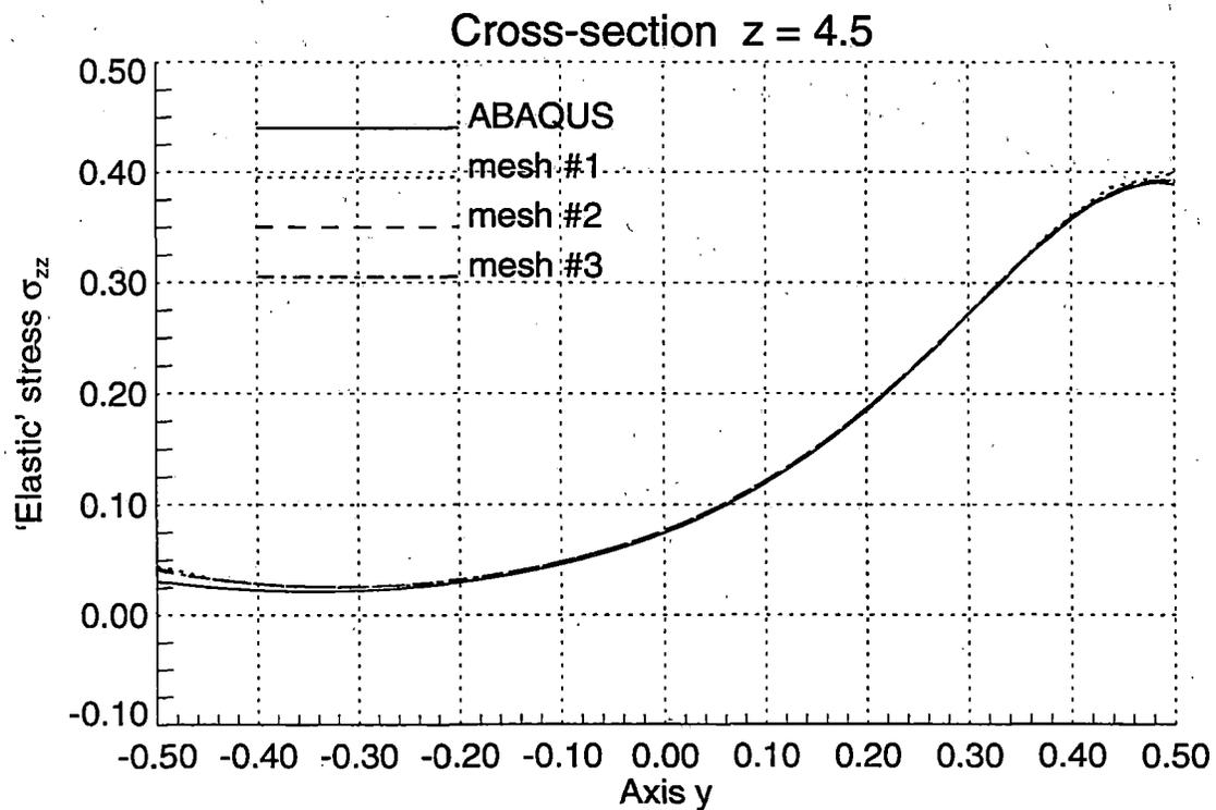
**Figure 2.17 Normal 'Elastic' Stresses  $\sigma_{zz}$  in the Simply Supported Beam under Concentrated Horizontal Surface Traction**
