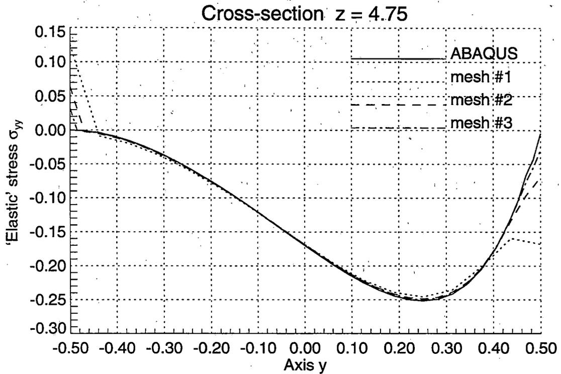
**Figure 2.7 Normal 'Elastic' Stresses  $\sigma_{yy}$  in the Simply Supported Beam under Concentrated Vertical Surface Traction**
