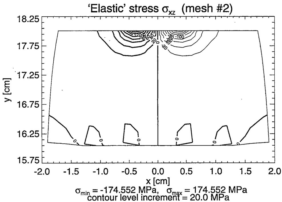
**Figure 2.44 Contour Lines of Shear 'Elastic' Stresses  $\sigma_{yz}$  and  $\sigma_{xz}$  in the Railroad Rail under Horizontal Loading Solution for Mesh #2**
