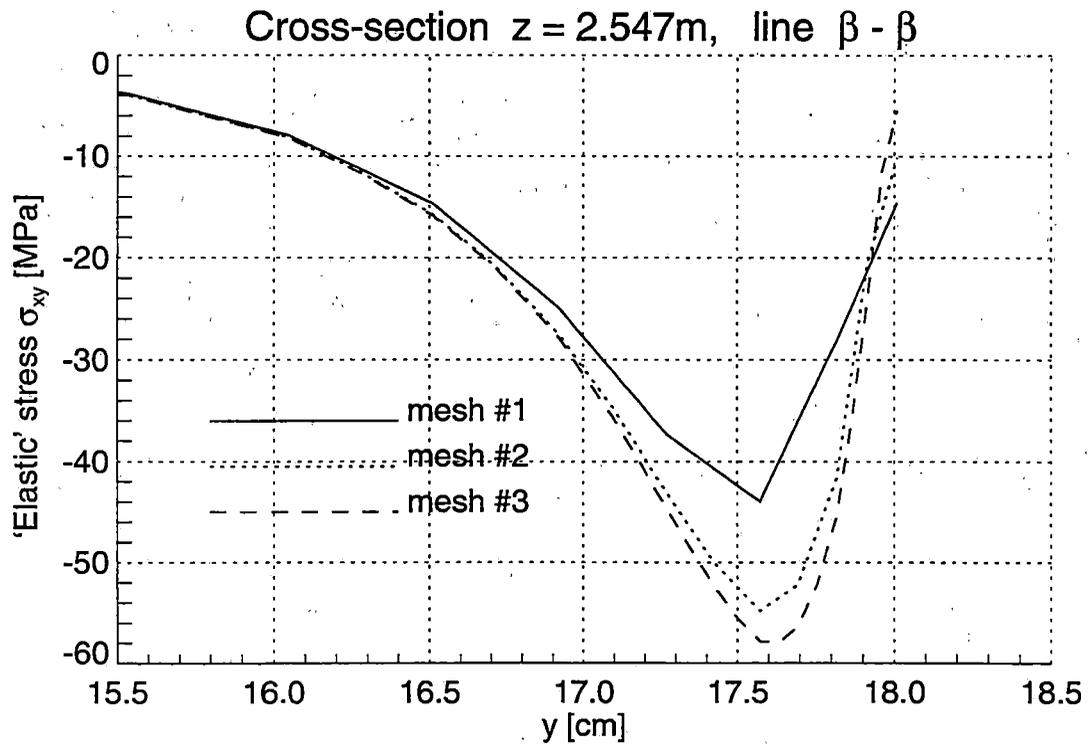
Figure 2.26 Shear 'Elastic' Stresses  $\sigma_{xy}$  in the Railroad Rail under Vertical Loading
