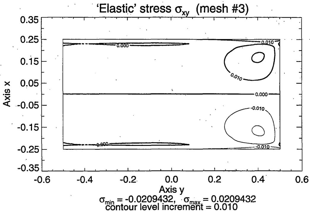
**Figure 2.15 Contour Lines of Normal  $\sigma_{zz}$  and Shear  $\sigma_{xy}$  'Elastic' Stresses in the Simply Supported Beam under Vertical Surface Traction – Solution for Mesh #3**
