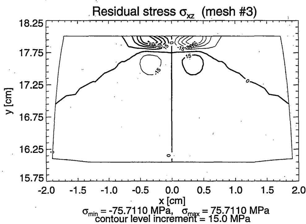
**Figure 3.12 Contour Lines of Shear Residual Stresses  $\sigma_{yz}$  and  $\sigma_{xz}$  in the Railroad Rail under Vertical and Horizontal Loading (Loading Case #2) – Solution for Mesh #3**
