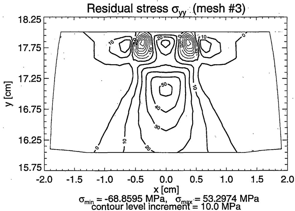
**Figure 3.4 Contour Lines of Normal Residual Stresses  $\sigma_{xx}$  and  $\sigma_{yy}$  in the Railroad Rail under Vertical Loading (Loading Case #1) – Solution for Mesh #3**
