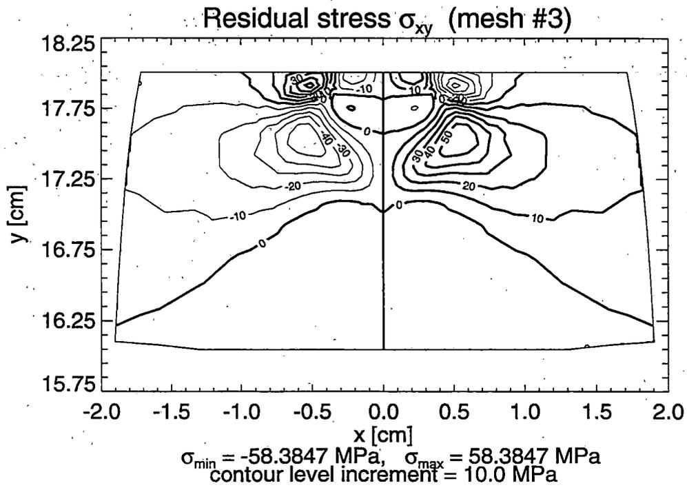
**Figure 3.6** Contour Lines of Normal  $\sigma_{zz}$  and Shear  $\sigma_{xy}$  Residual Stresses in the Railroad Rail under Vertical Loading (Loading Case #1) – Solution for Mesh #3
