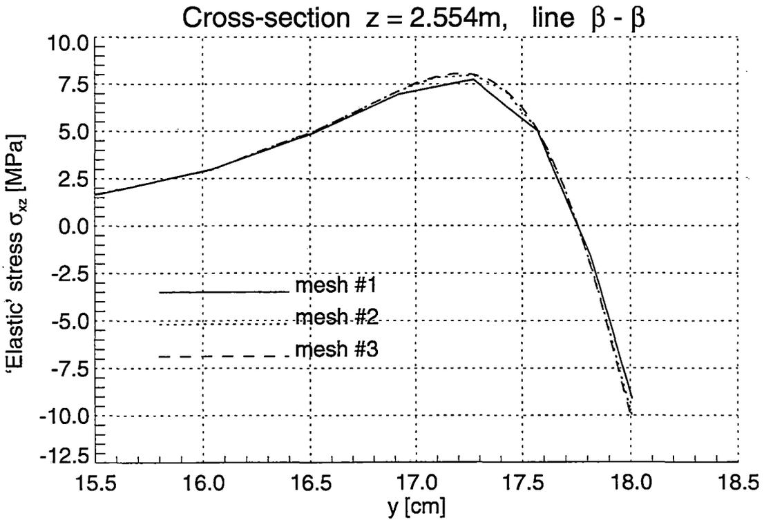
Figure 2.28 Shear 'Elastic' Stresses  $\sigma_{xz}$  in the Railroad Rail under Vertical Loading
