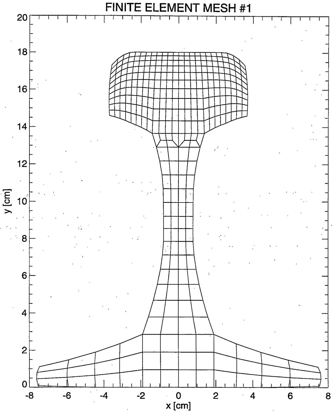
**Figure 2.19 Finite Element Mesh #1 in the Problem of a Railroad Rail under Contact Loading**
