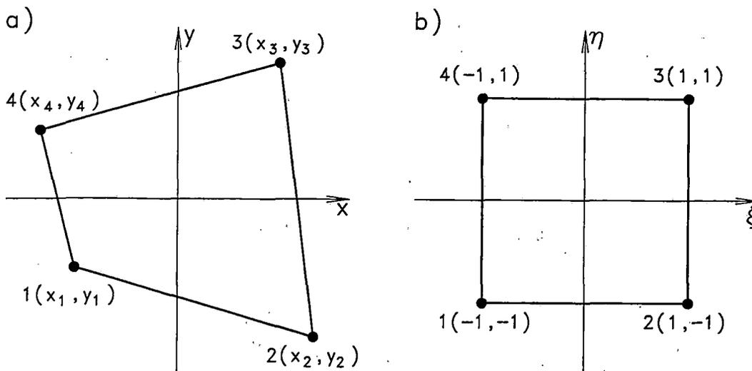
Figure 2.1 Quadrilateral Finite Element
