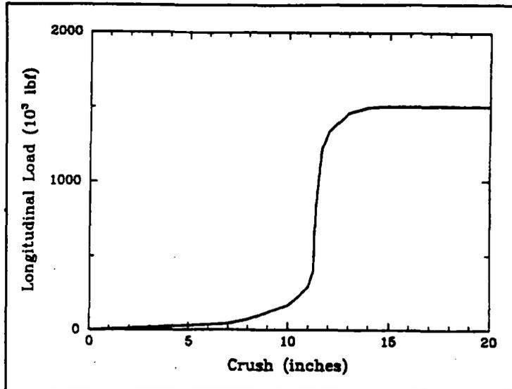
**Figure 3.5** Calculated Load-Crush Curve for the Concept Short Hood/Collision Posts
