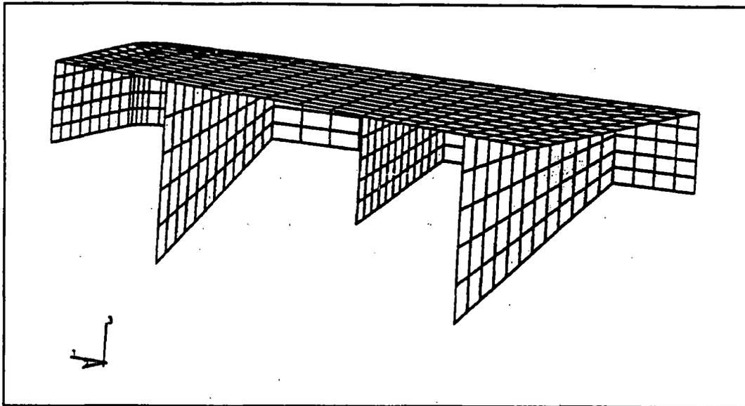
**Figure 3.16 Finite Element Mesh of the Anticlimber Modeled to Satisfy AAR S-580 Requirements (looking forward from sill end; only left half of anticlimber structure is shown)**
