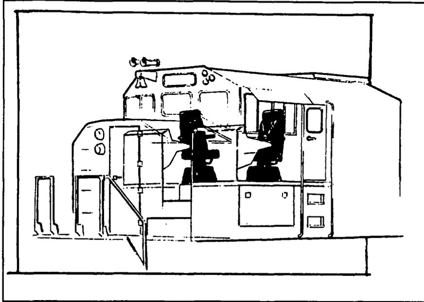
**Figure 3.11 Illustration of the Rotating Seat Crash Refuge Concept**
