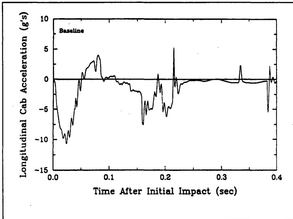
**Figure 3.3 The Locomotive Cab Crash Pulse for the Baseline Crash Scenario**
