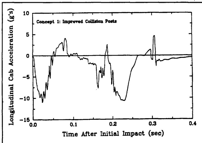
**Figure 3.6** Cab Crash Pulse for the Concept Collision Post Locomotive
