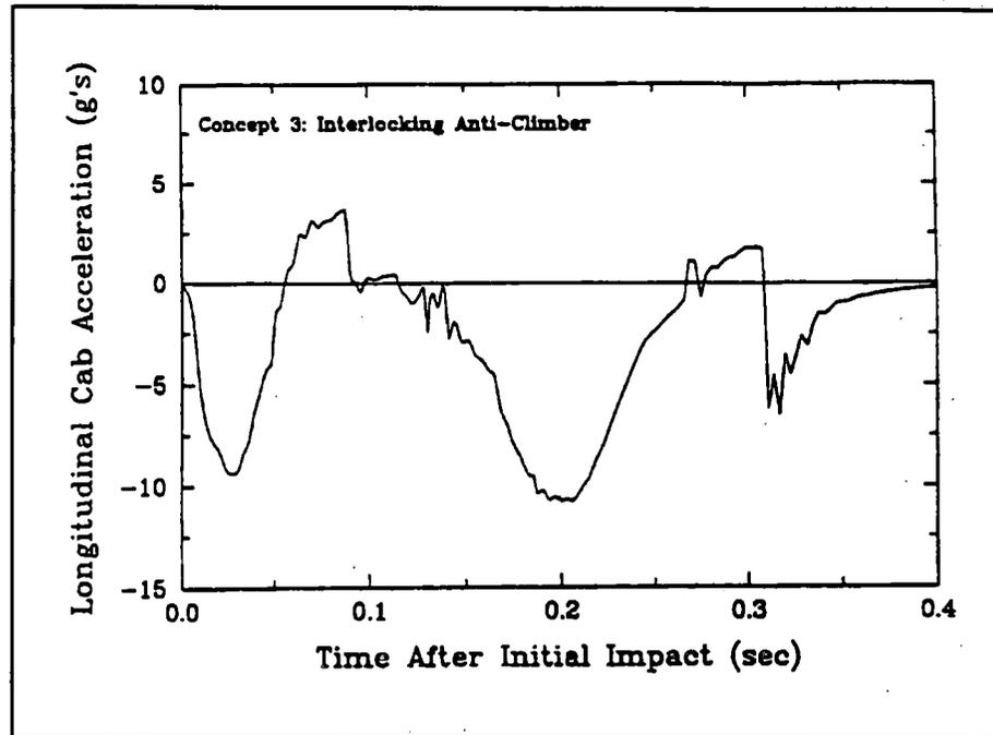
**Figure 3.18 Cab Crash Pulse for the Interlocking Anticlimber Concept**
