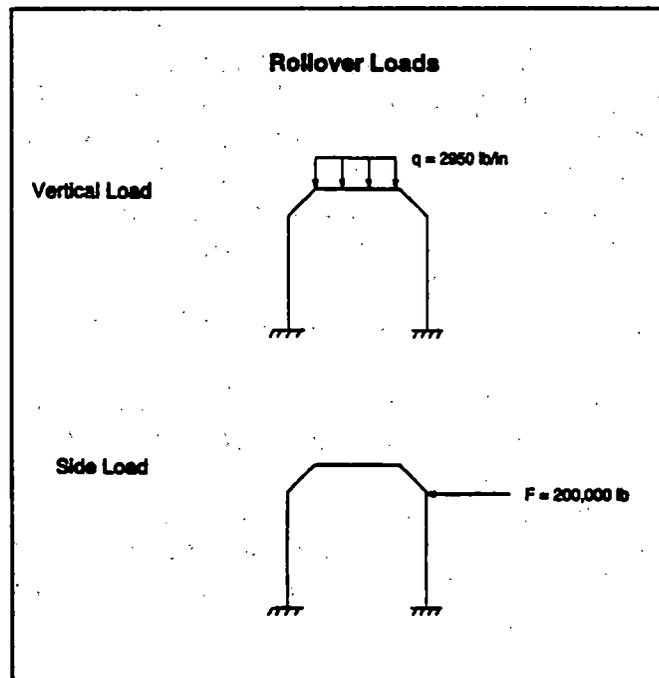
**Figure 3.8 Design Crash Loads for the Roll Bar Concept**
