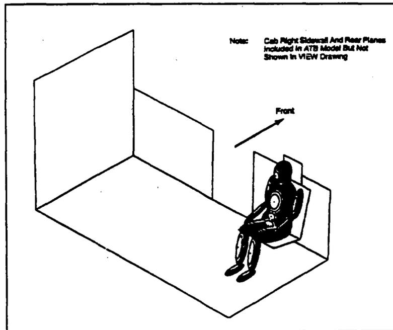
**Figure 3.13 Occupant Position in the Rotate and Lock Seat Crash Refuge Concept**
