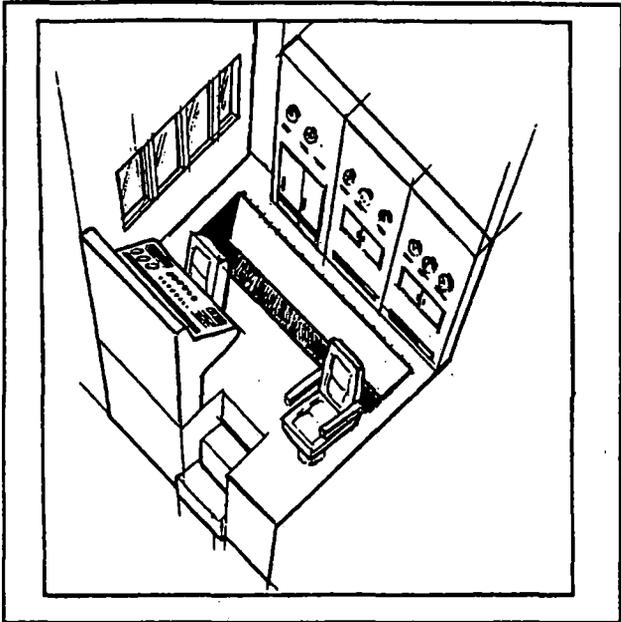
**Figure F.1 Illustration of the Trench Crash Refuge Concept**
