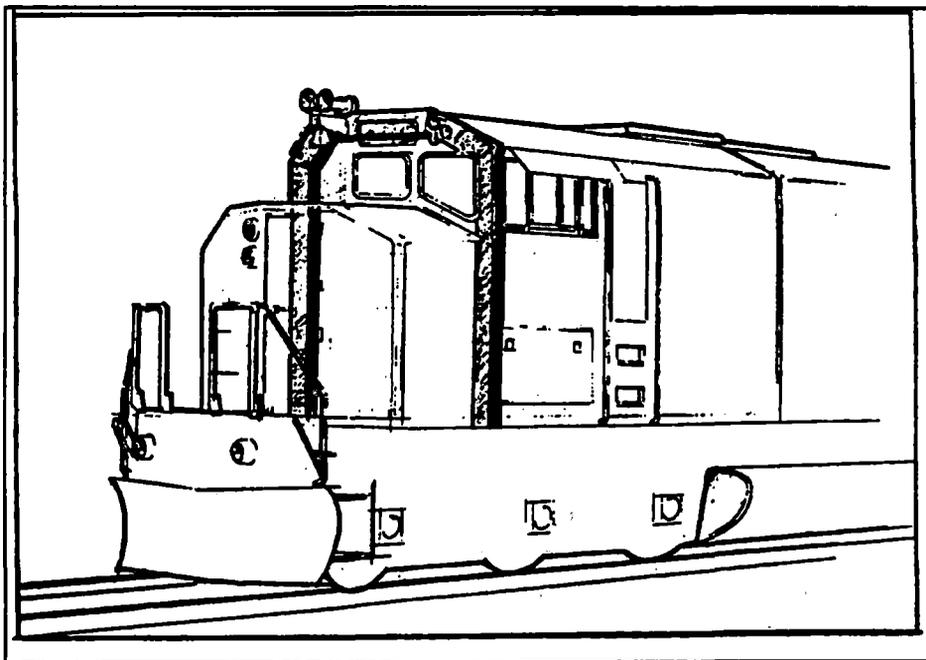
**Figure 3.7** Illustration of the Roll Bar Concept
