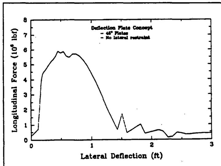
**Figure 3.10 Load-Lateral Deflection Curve for the 45 Degree Deflection Plate Concept**
