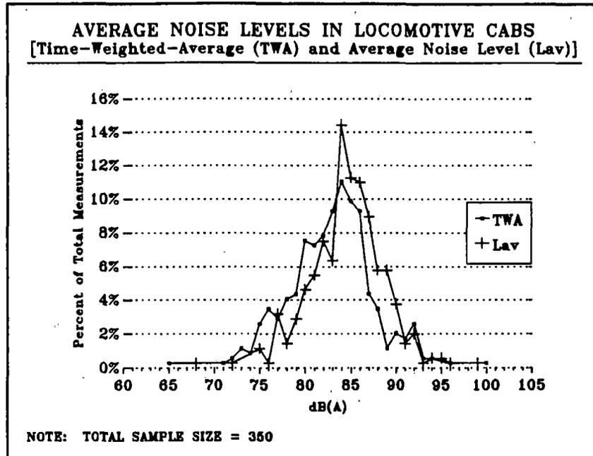
Figure 6.3 Average Noise Levels in Locomotive Cabs
