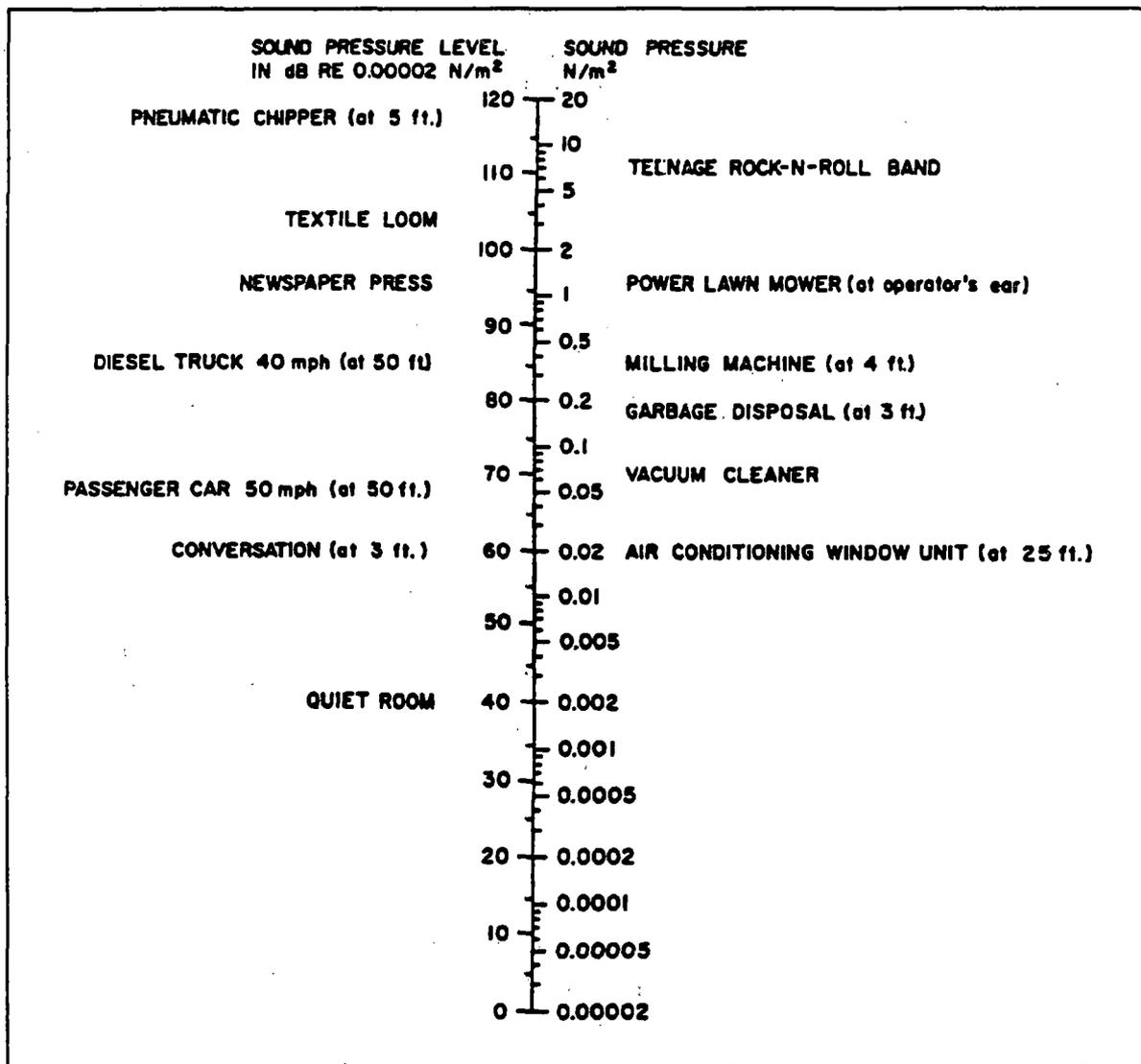
Figure 6.1 Relationship Between Sound Pressure Level in Decibels (dB) and Sound Pressure in Pa ( $N/m^2$ )
