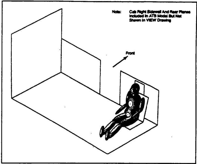
**Figure 3.14 Occupant Position in the Rotate, Lock, and Drop Crash Refuge Concept**
