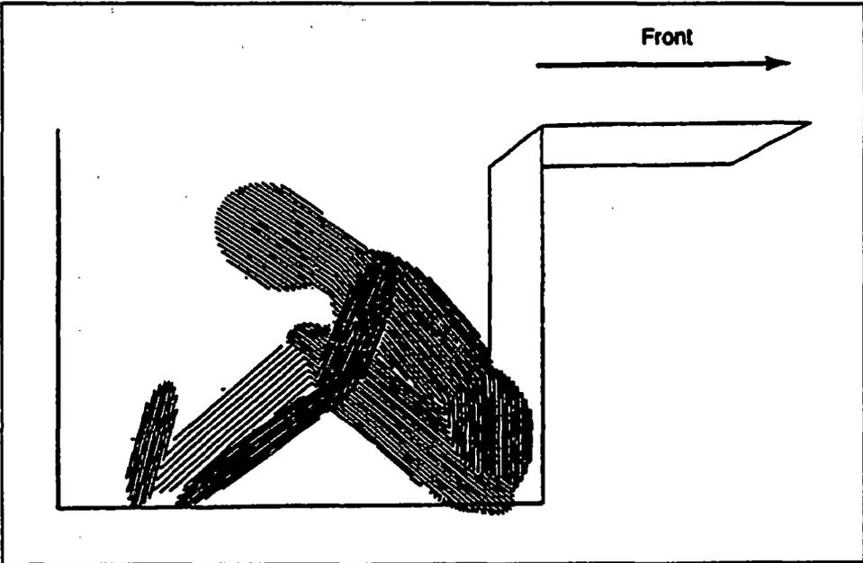
**Figure F.2 Occupant Position in the Trench Crash Refuge Concept**
