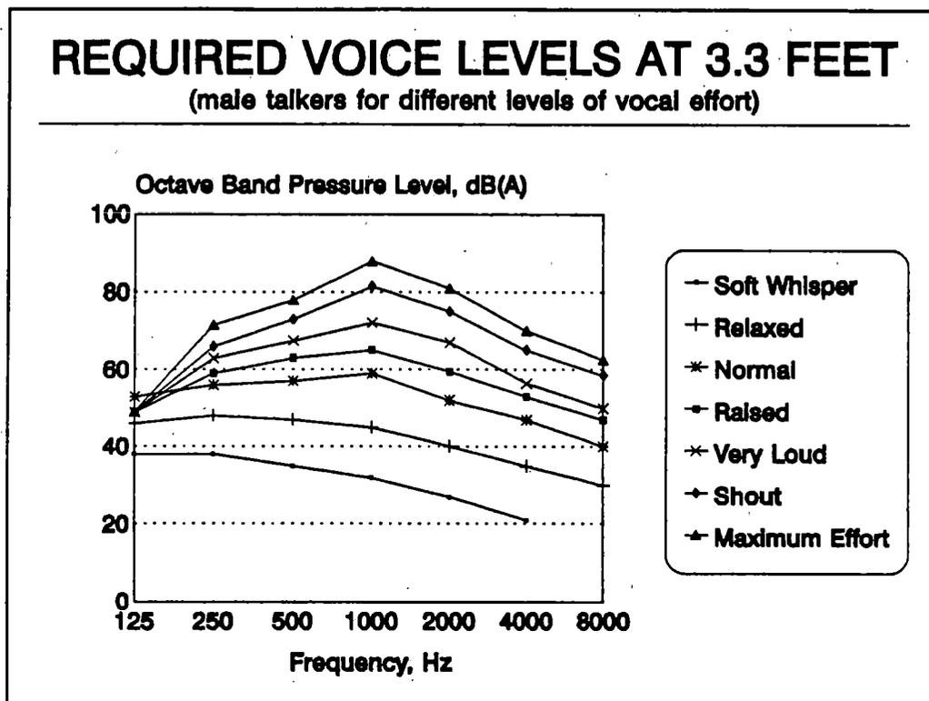
Figure 6.2 Human Voice Levels Required for Sustained Verbal Communication
