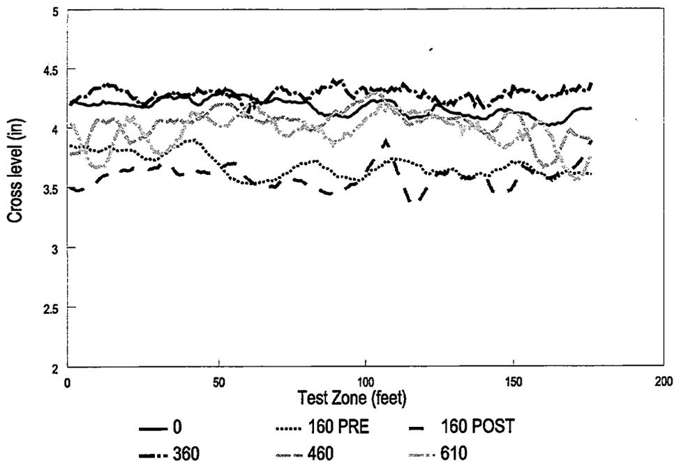
**Exhibit 19. Cross-Level Measurements — Traprock Ballast**
