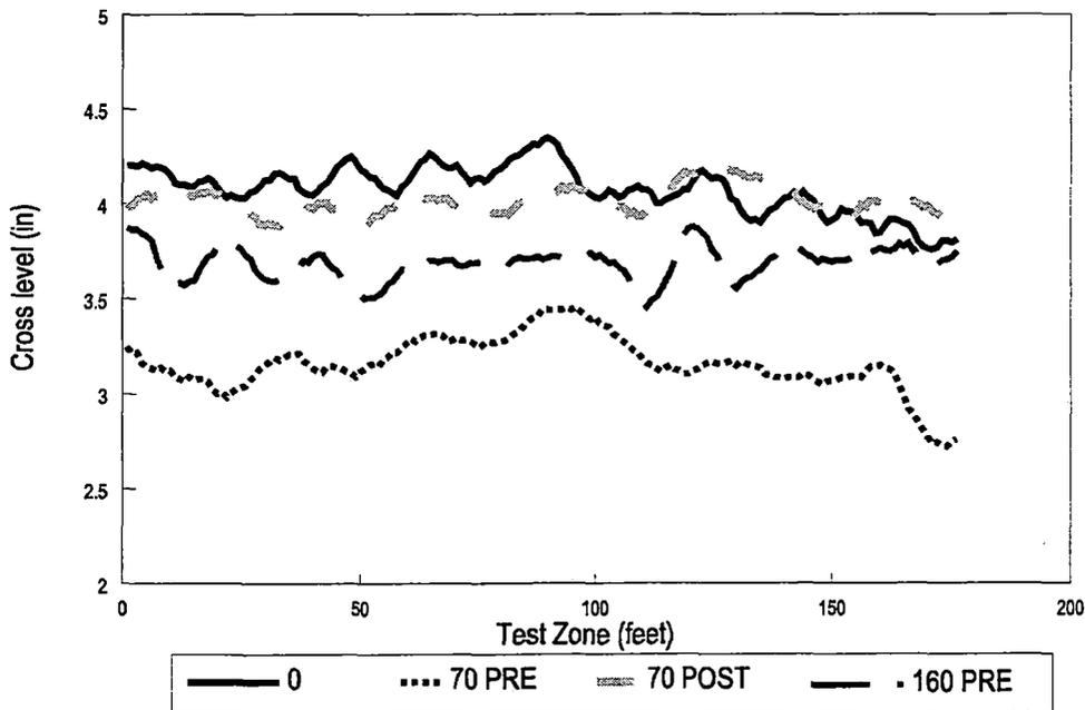
**Exhibit 16. Cross-level Measurements — Limestone Ballast**
