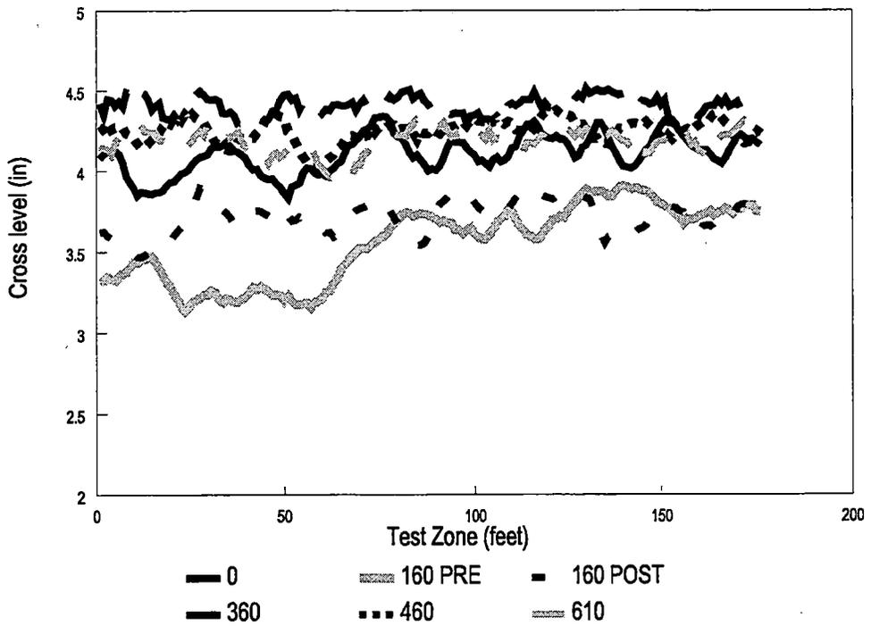
**Exhibit 18. Cross-Level Measurements — Granite Ballast**
