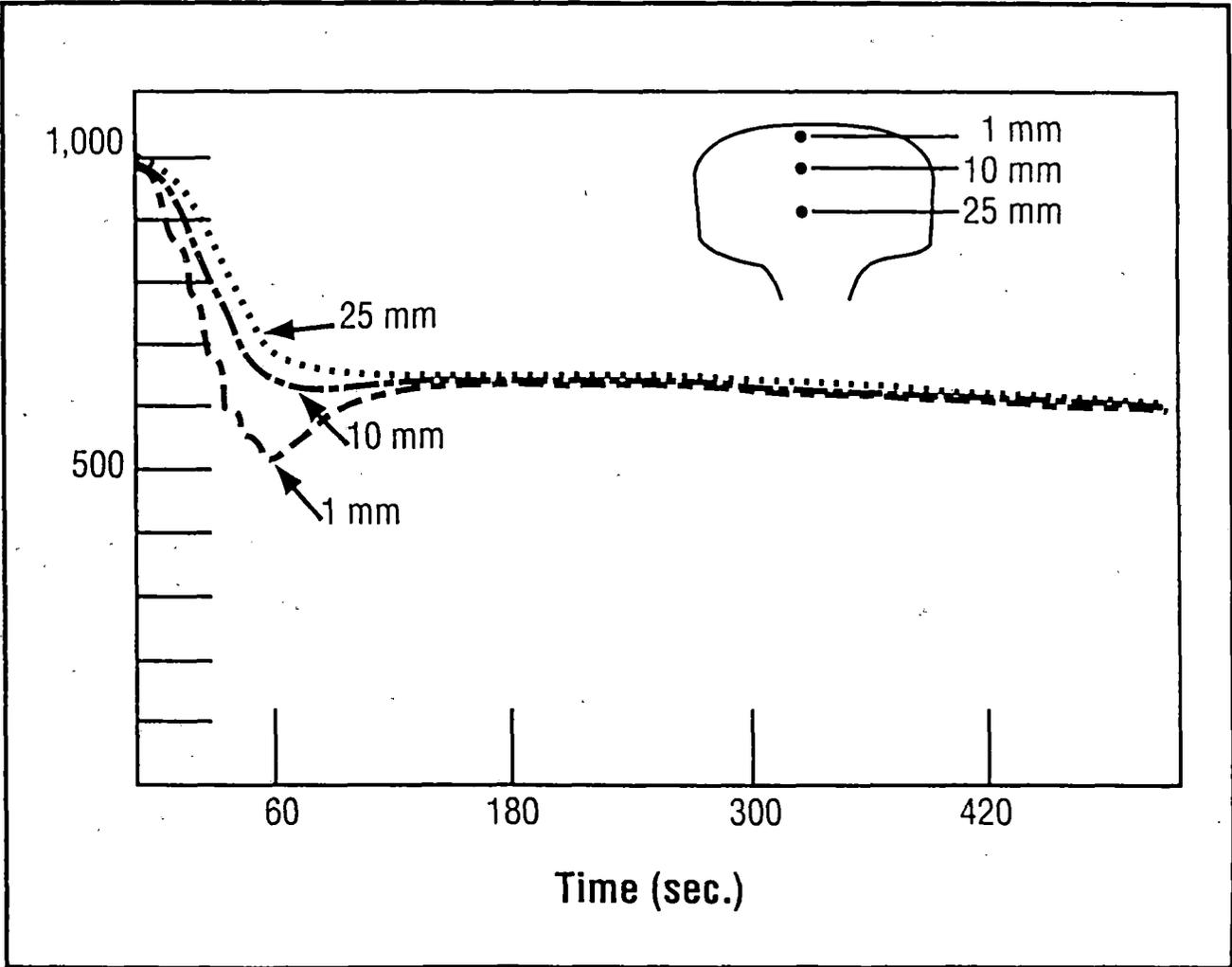
Figure 4: Cooling Curves of Rail at Three Locations (Source: Bramfitt, Ref 2)
