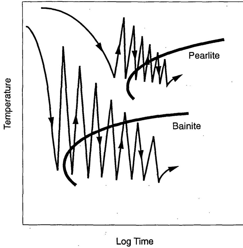
Figure 7: Conceptual Illustration of Bainite Compared to Pearlite Surface Cooling Paths
