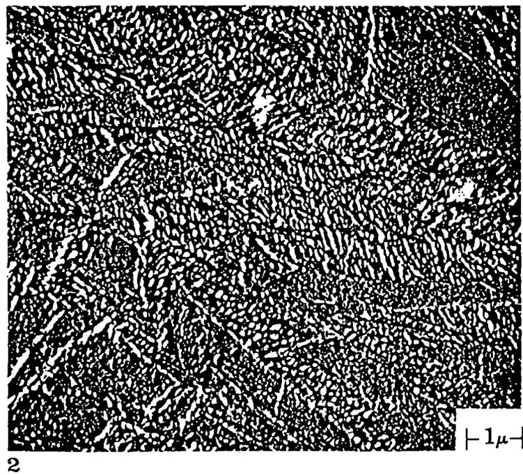
Figure 17: Typical Microstructures for Upper (1) and Lower (2) Bainite in a High Carbon Steel (Source: Habracken/Economopoulos, Ref 11)
