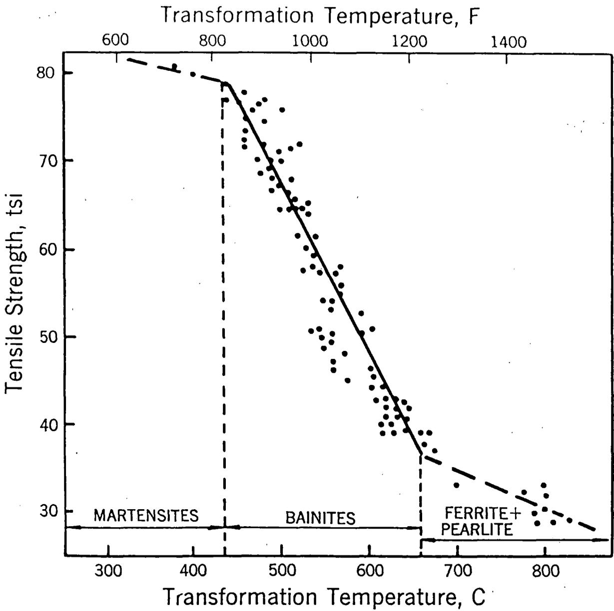
Figure 21: Effect of Transformation Temperature on Tensile Strength
