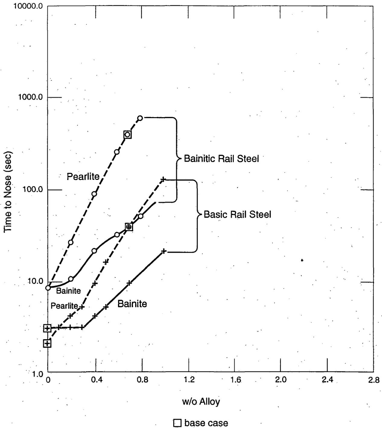
Figure 33: Effect of Molybdenum without Boron on the Times to Pearlite and Bainite Noses
