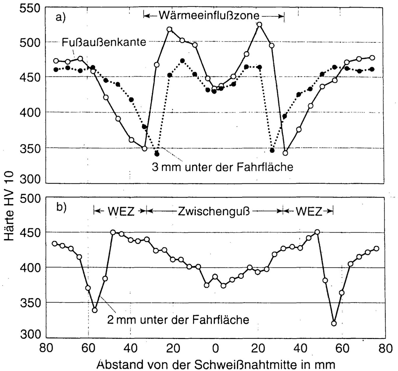
Figure 47: Hardness Traverses of Electric Flash Butt and Thermite Welds (Source: deBoer et. al. Ref 10)
