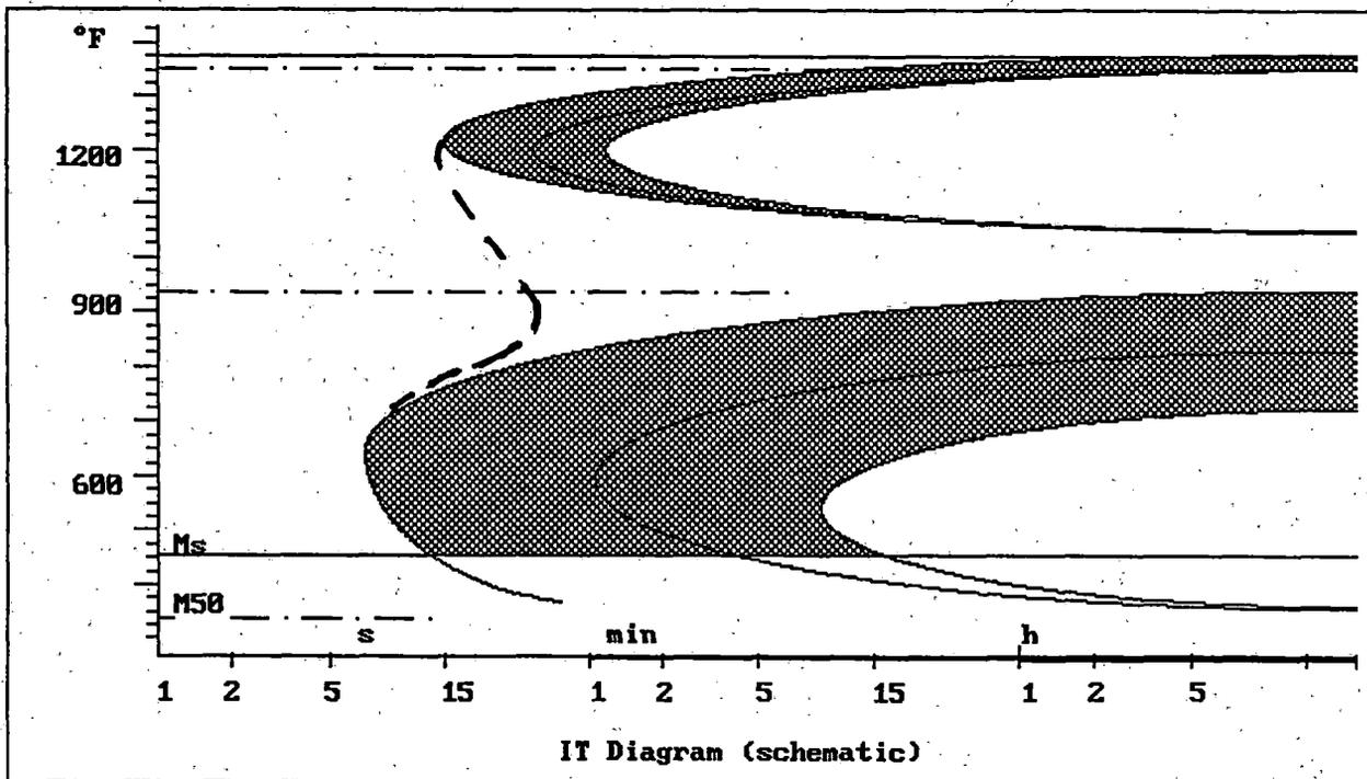
Figure 48: SteCal™ Prediction of the TTT Diagram for a Commercial CrMo Rail Steel
