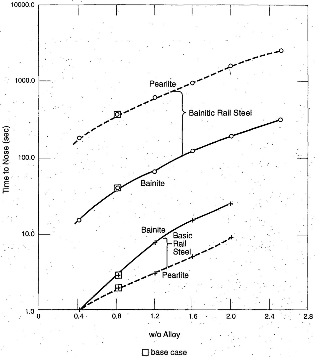
Figure 29: Effect of Manganese on the Times to Pearlite and Bainite Noses
