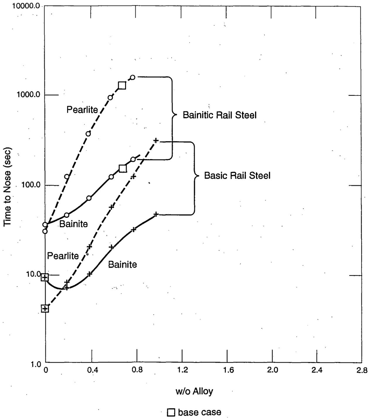
Figure 34: Effect of Molybdenum with Boron on the Times to Pearlite and Bainite Noses
