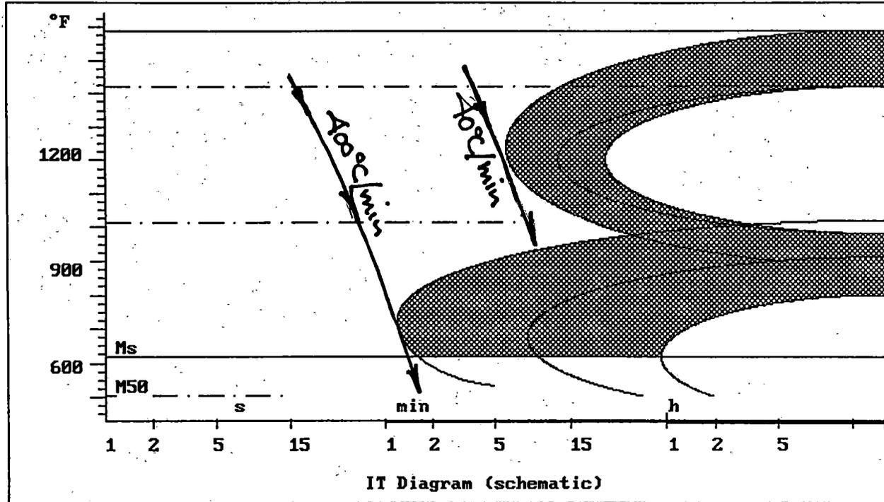
Figure 45: Critical Cooling Paths in the Modified Bainitic Rail Steel Composition
