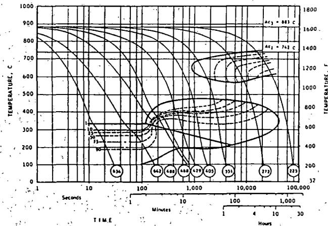
Figure 44: Experimentally-Determined CCT Diagrams for Alloy Similar in Composition to de Boer et al Alloy (Source: Cias, Ref 24)
