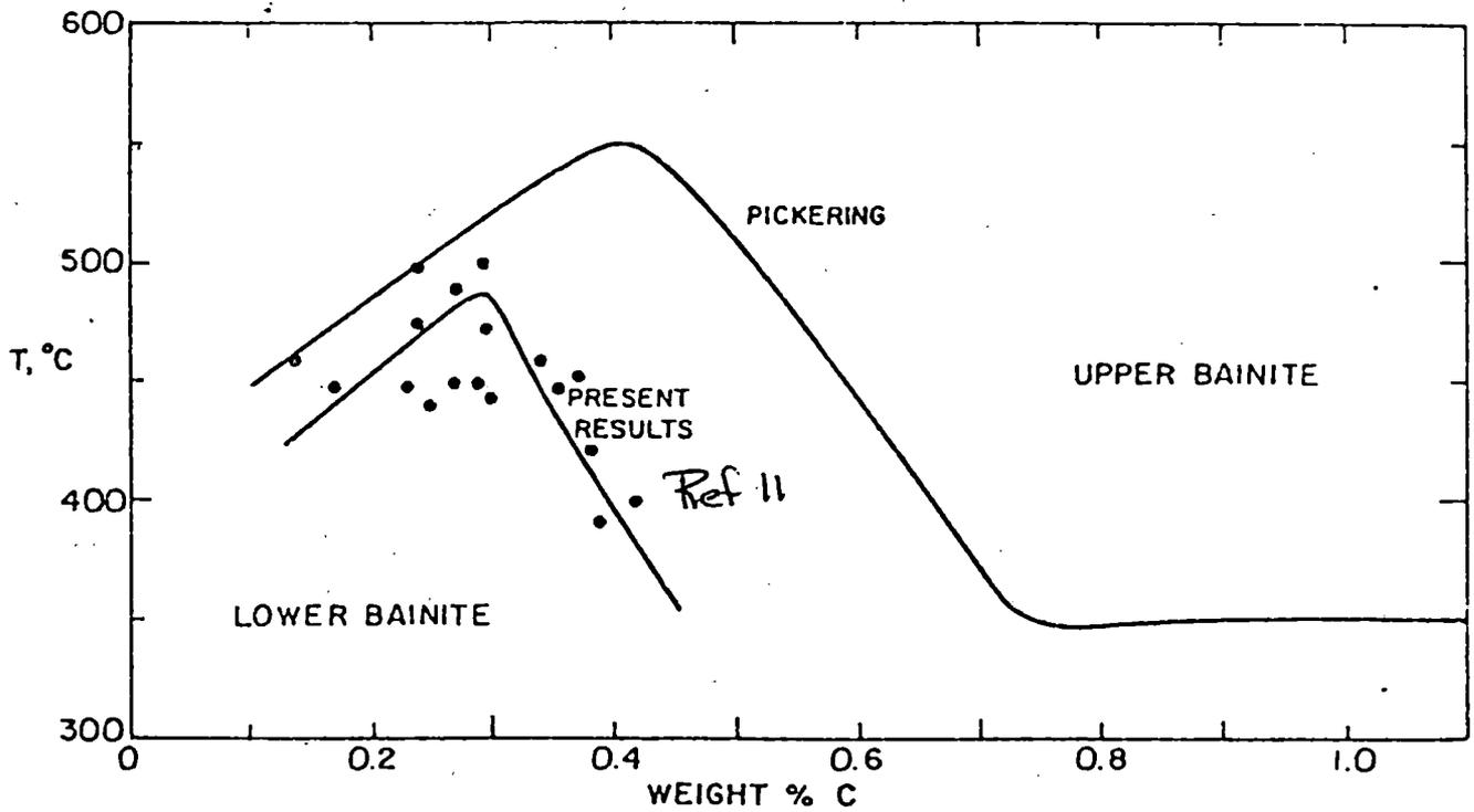
Figure 18: Effect of Carbon on the Temperature Change from Upper to Lower Bainite (Source: Parker, Ref 15)
