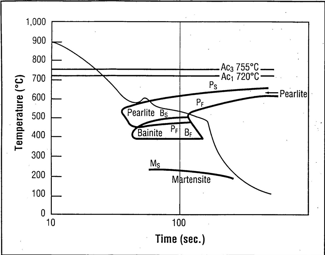
Figure 3: Continuous Cooling Transformation Diagram Showing Cooling Path for In-Line Process (Source: Bramfitt, Ref 2)
