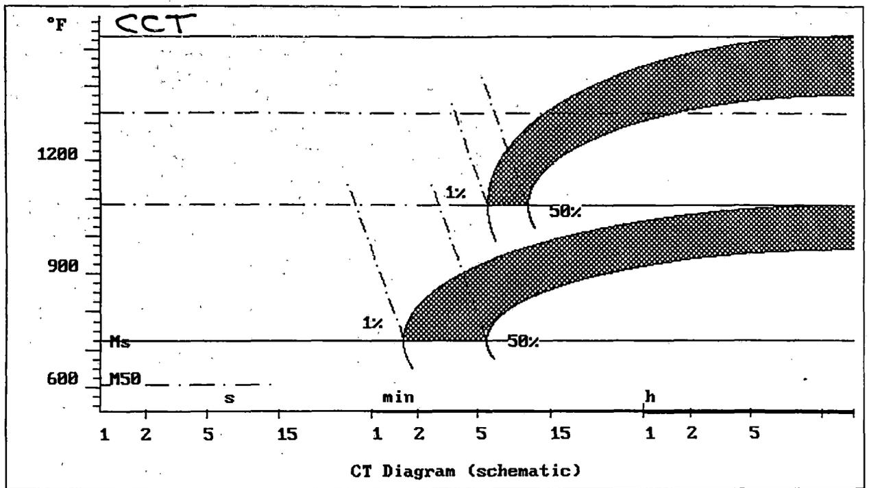
Figure 52: SteCal™ Prediction of the Effect of Lowering Manganese Content in the Modified TC 128 Alloy
