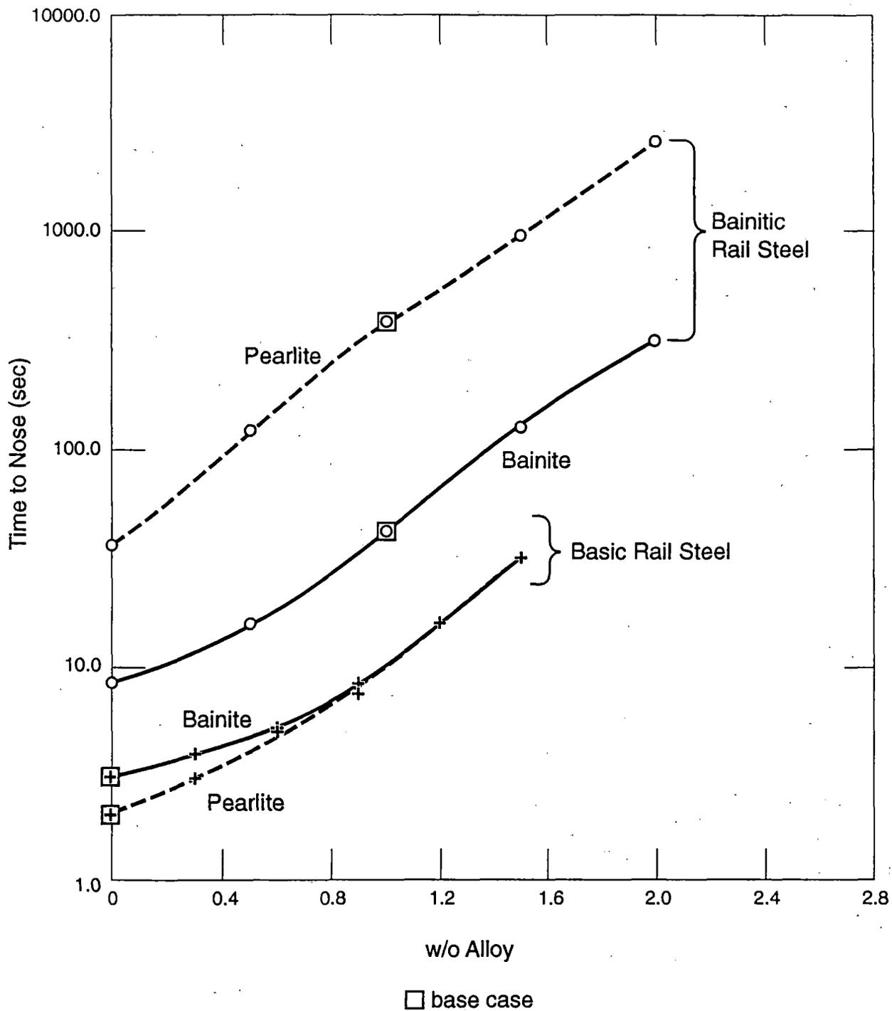
Figure 31: Effect of Chromium on the Times to Pearlite and Bainite Noses
