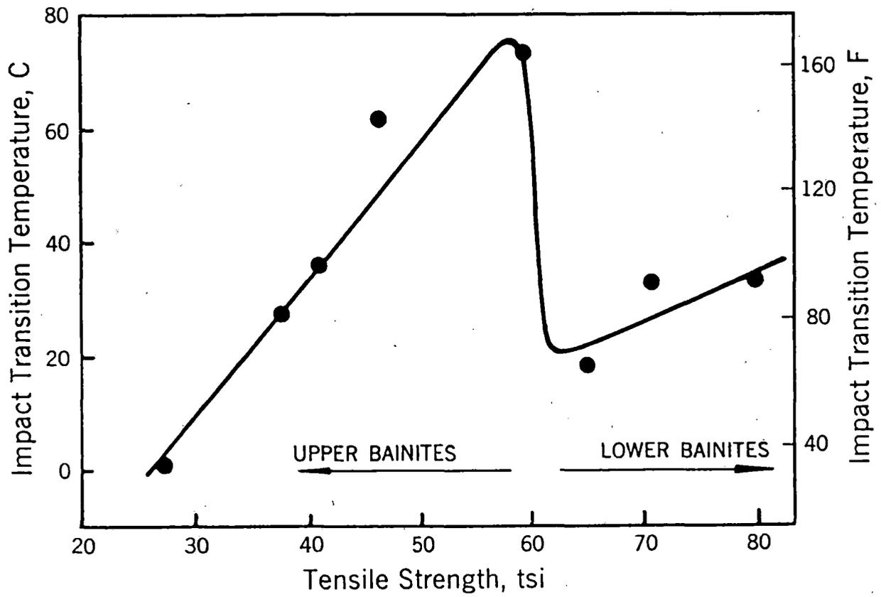
Figure 23: Effect of Tensile Strength on Impact Transition Temperature in Bainitic Steels (Source: Pickering, Ref 13)
