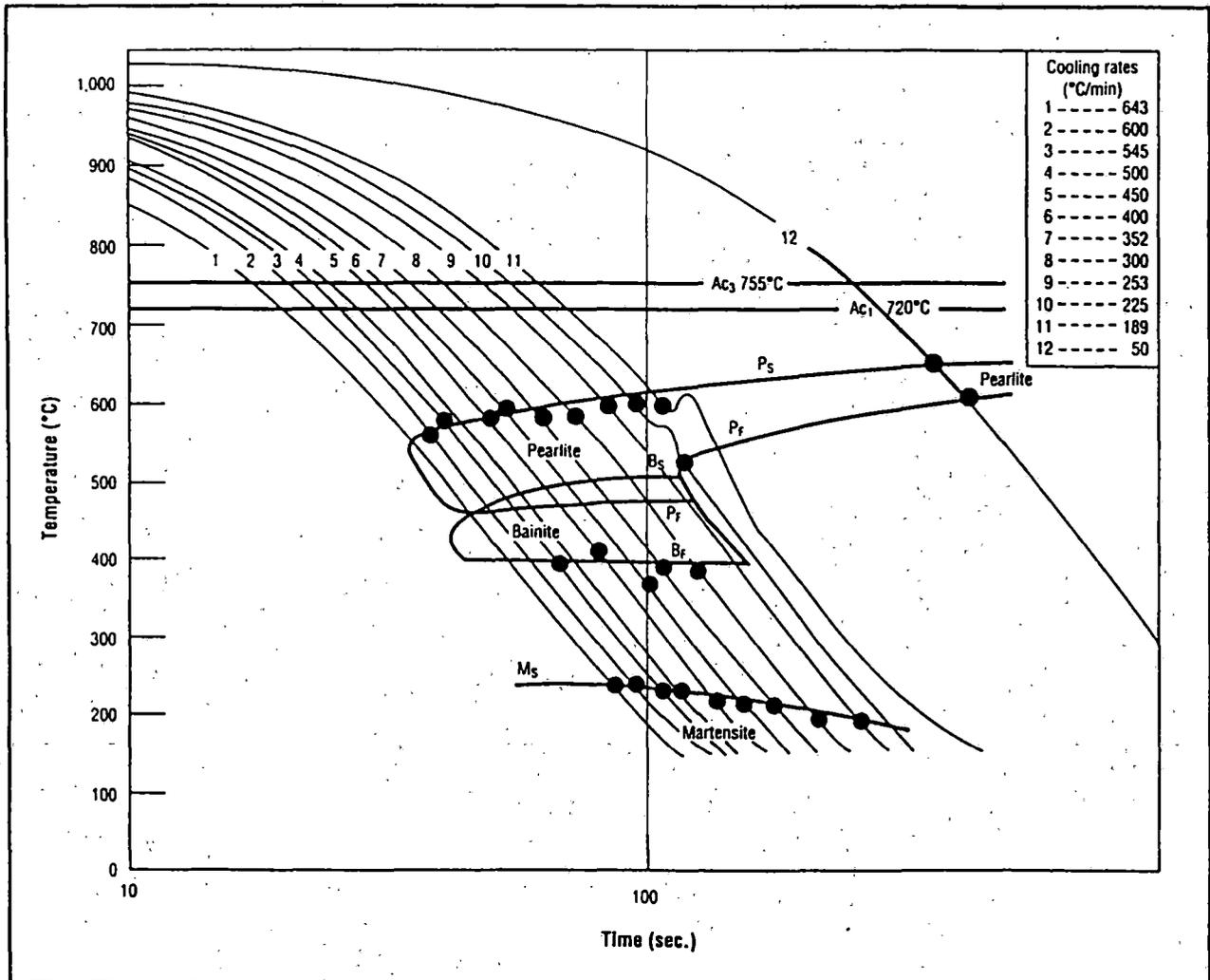
Figure 2: Continuous Cooling Transformation Diagram of a Rail Steel (Source: Bramfitt, Ref 2)
