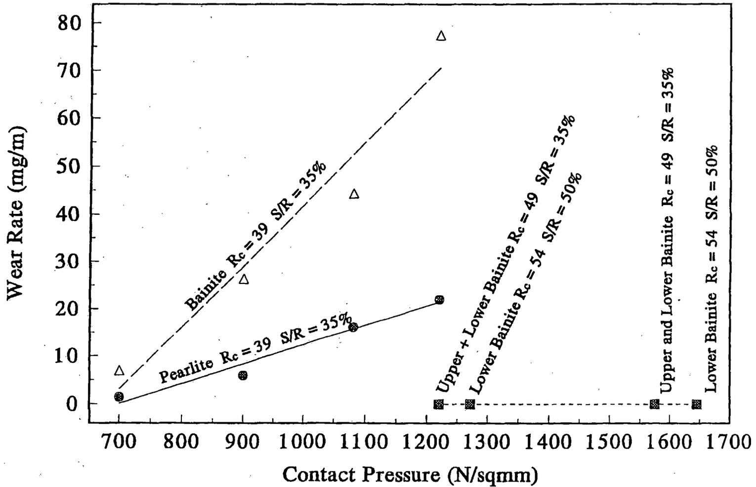
Figure 8: Wear Rates at Increasing Contact Pressures for Pearlitic and Bainitic Microstructures (Source: Clayton/Devanathan, Ref 9)
