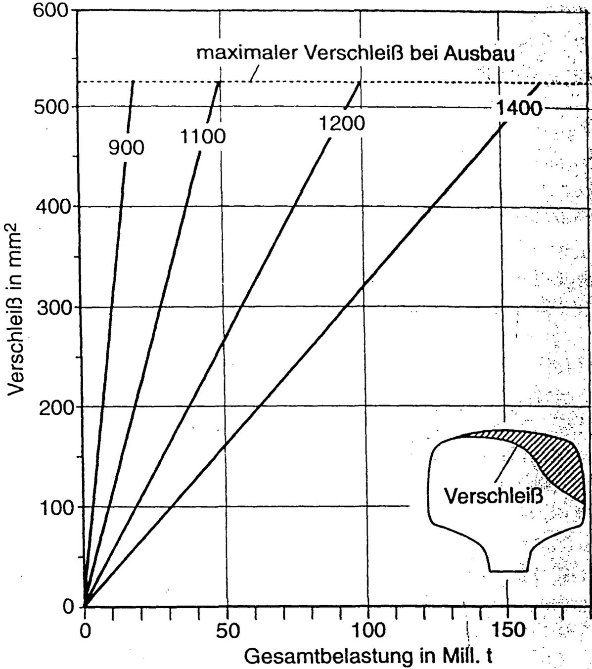
Figure 12: Wear Loss of Rail Steels in 300 Meter Radius Test Curves
