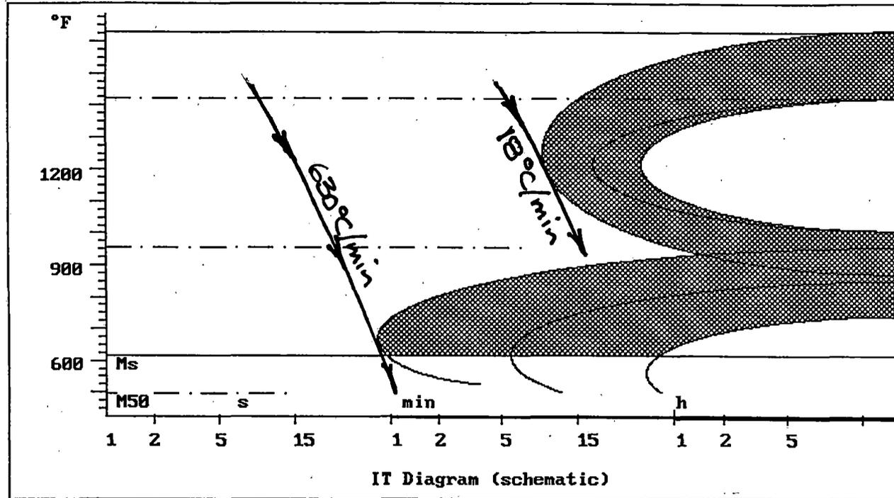
Figure 46: Critical Cooling Paths in the Unmodified Bainitic Rail Steel Composition
