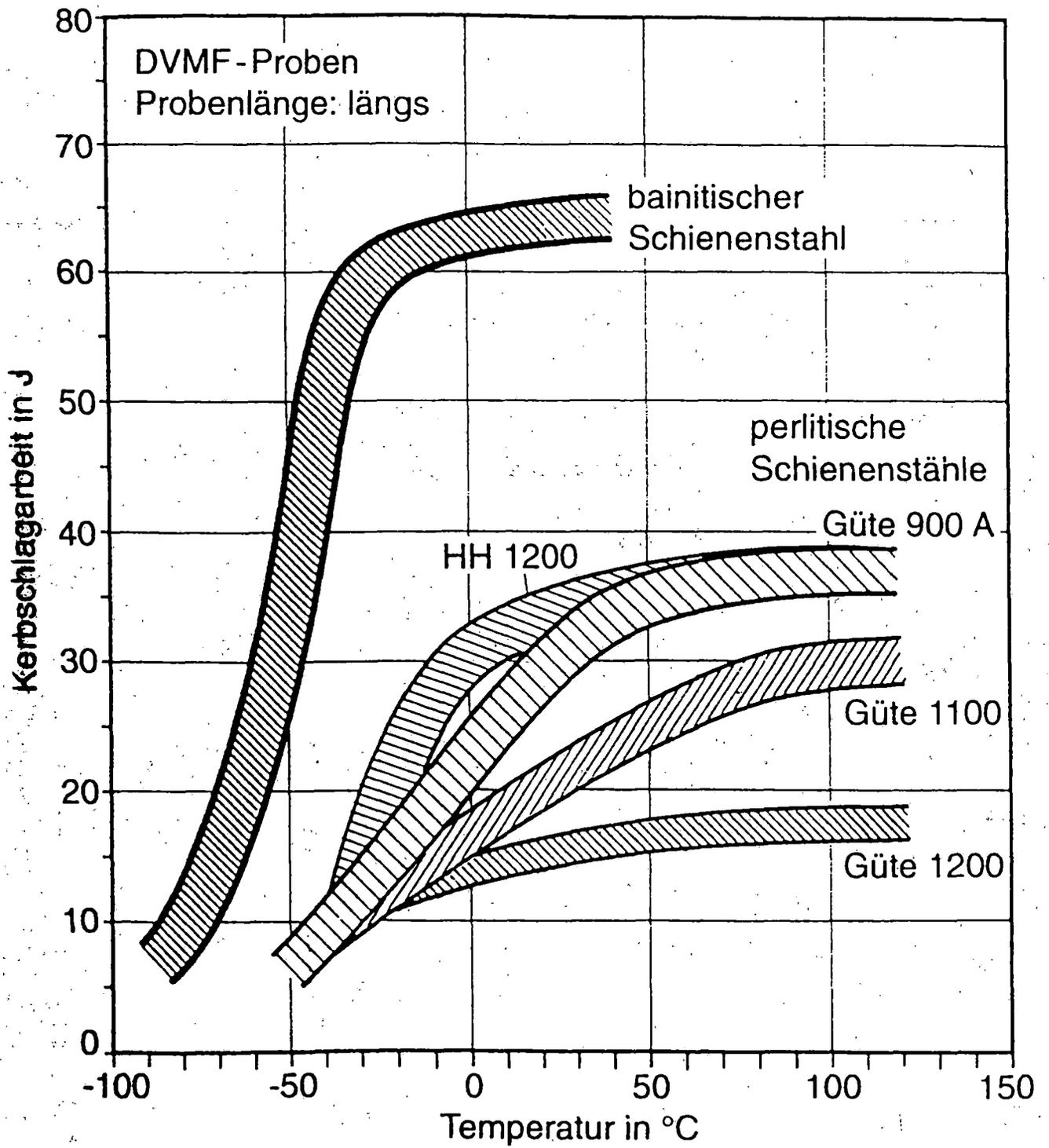
Figure 11: Impact Energy as a Function of Test Temperature
