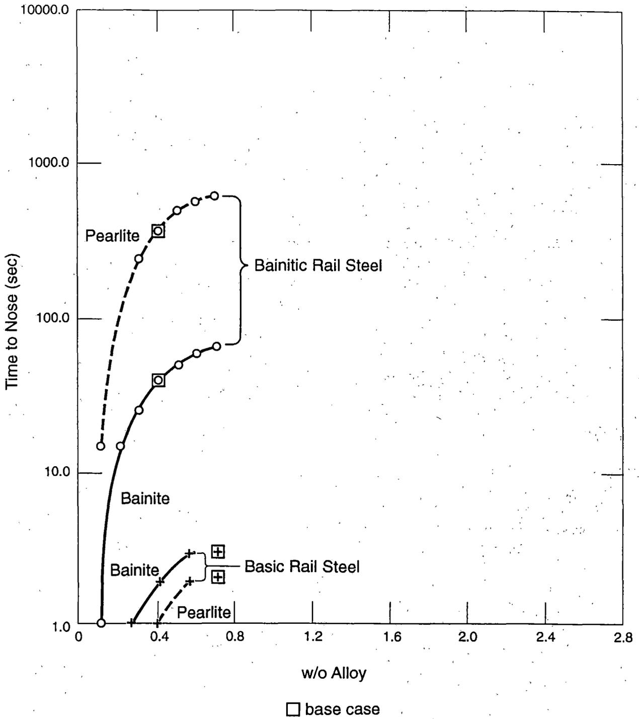
Figure 28: Effect of Carbon on the Times to Pearlite and Bainite Noses
