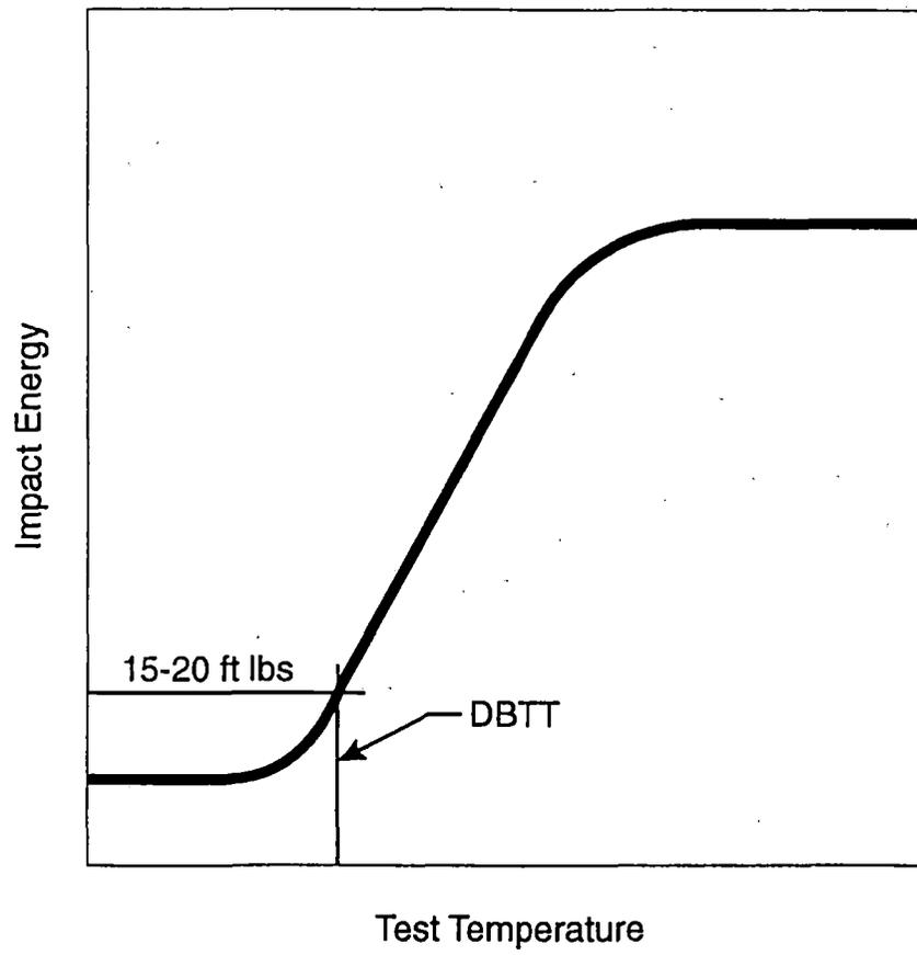
Figure 13: Illustration of the Impact Test Ductile to Brittle Transition Temperature
