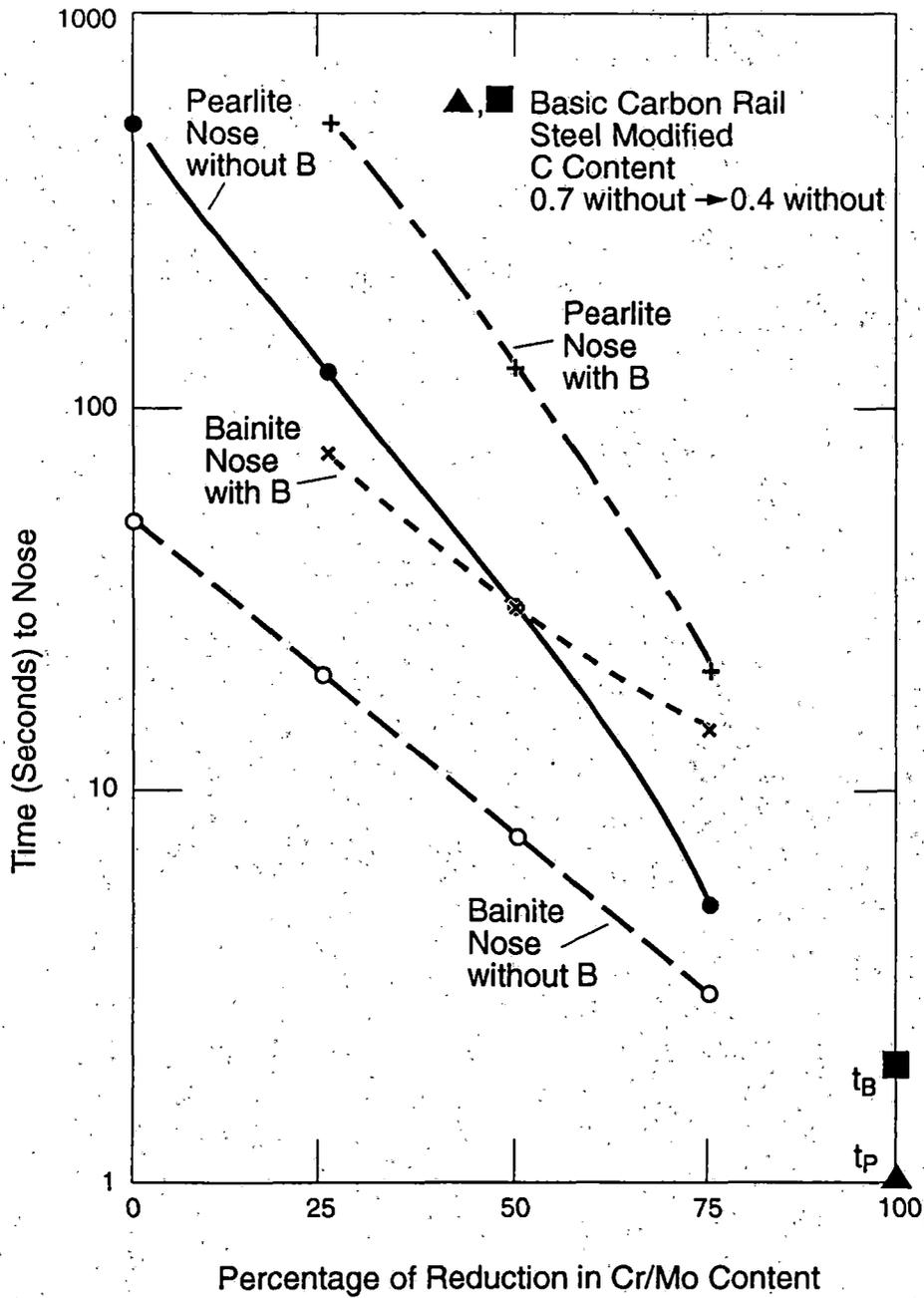
Figure 42b Effect of Cr and Mo Reduction on the Times to the Pearlite and Bainite Noses
