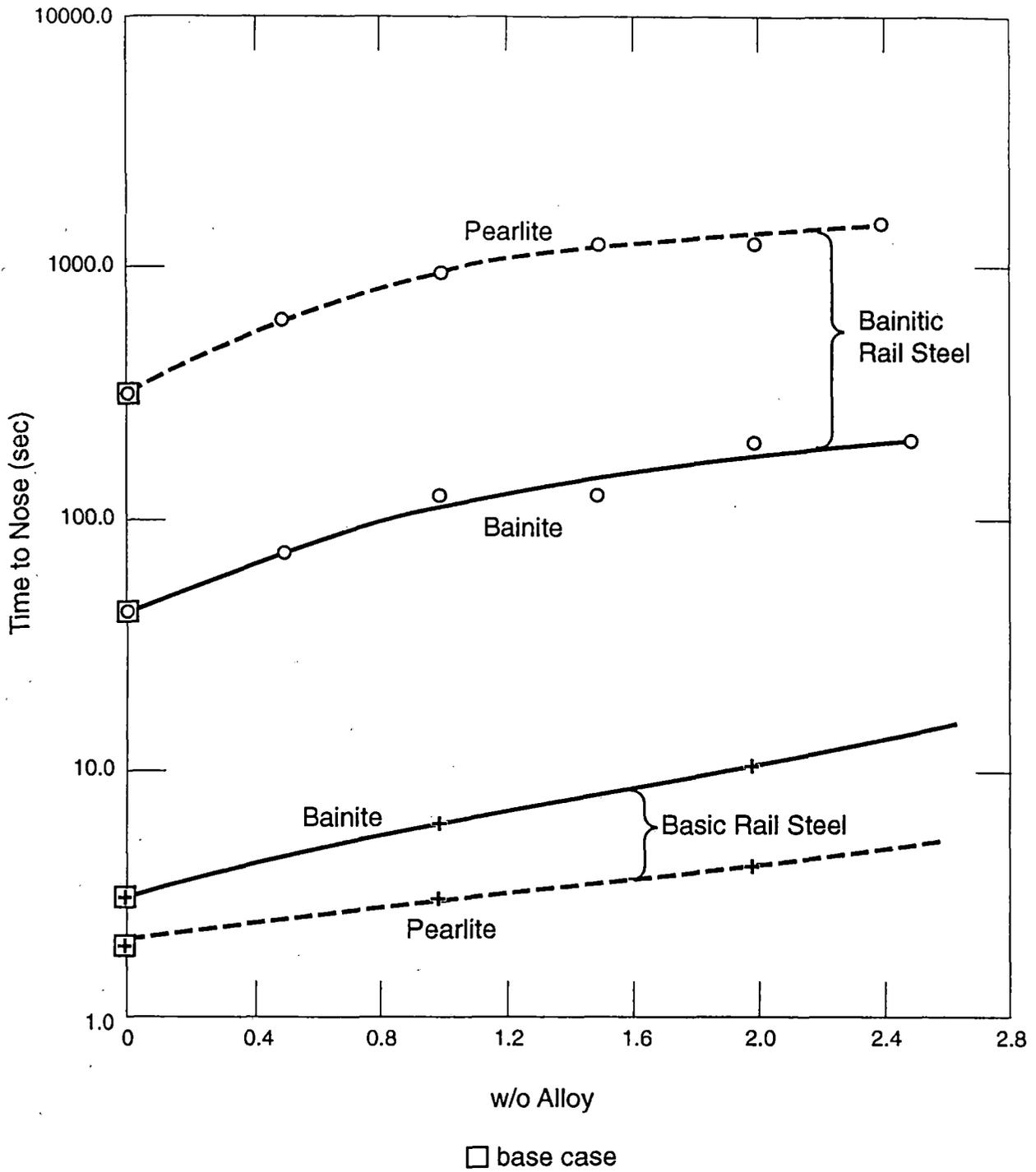
Figure 32: Effect of Nickel on the Times to Pearlite and Bainite Noses
