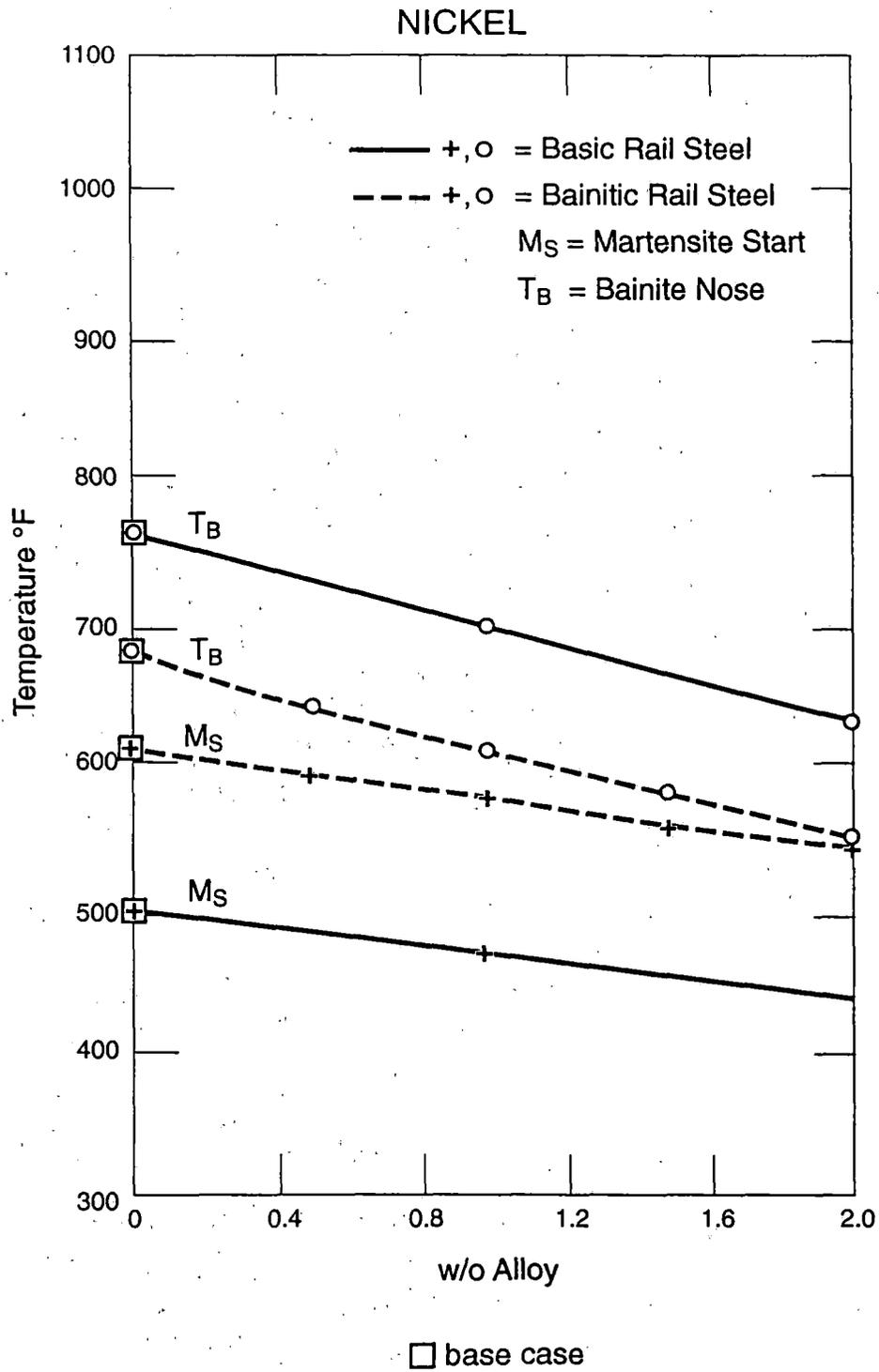
Figure 39: Effect of Nickel on the Martensite Start and Bainite Nose Temperatures
