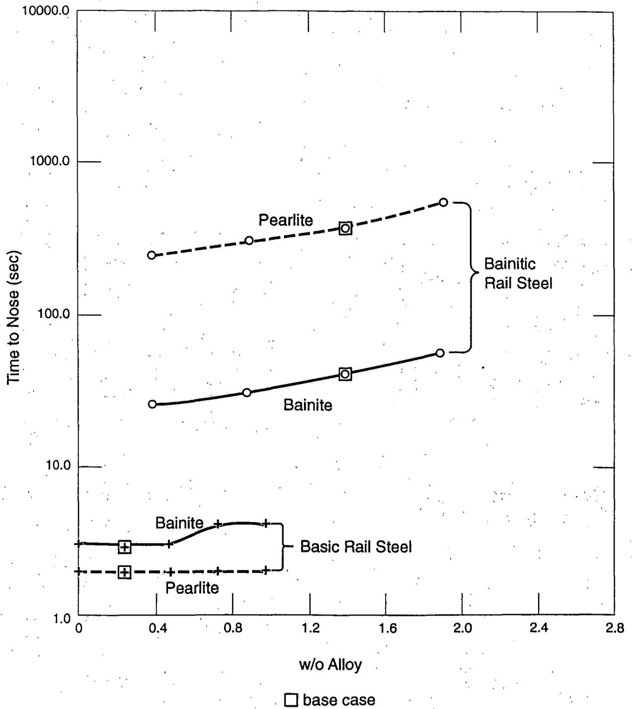
Figure 30: Effect of Silicon on the Times to Pearlite and Bainite Noses
