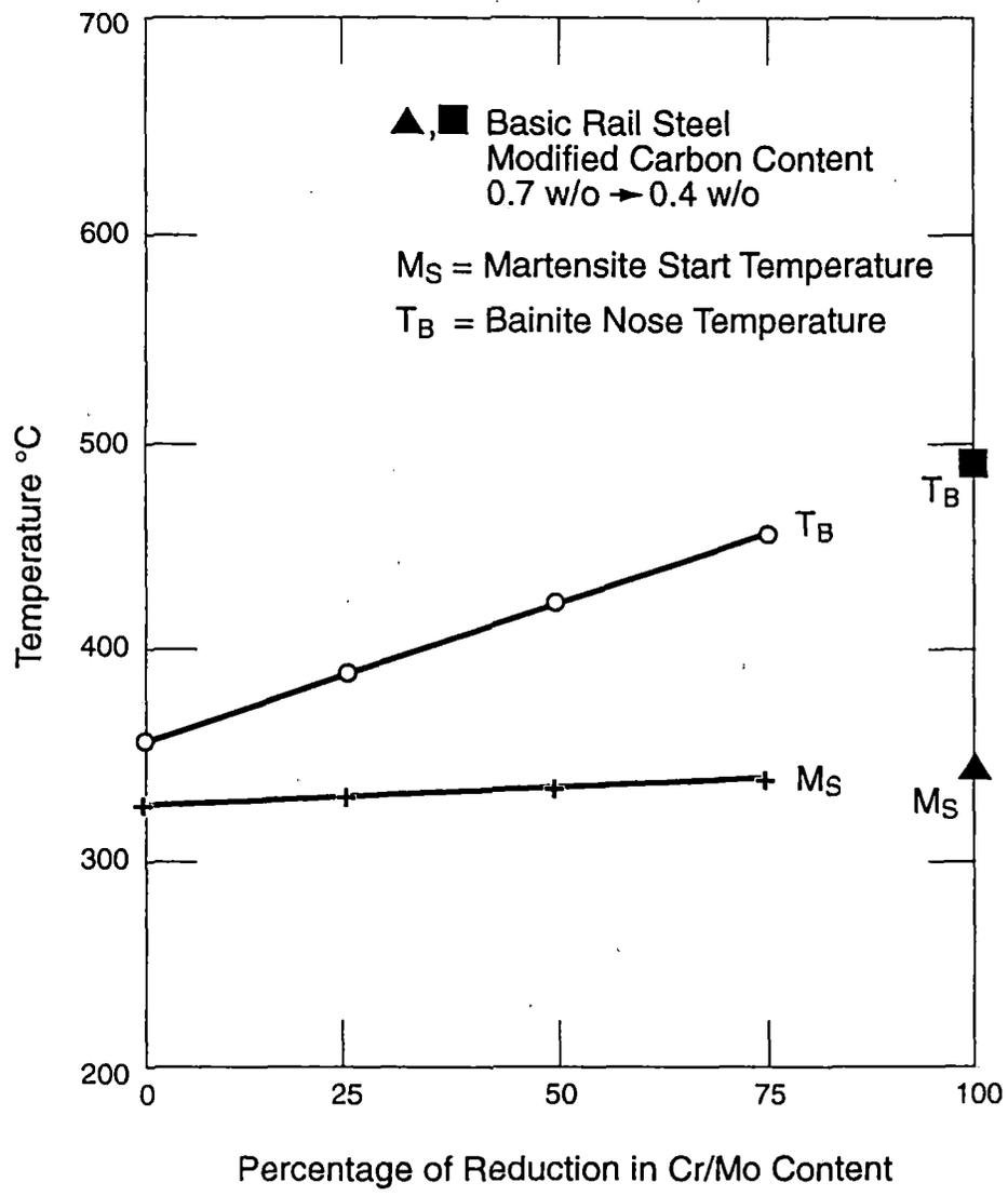
Figure 42a: Effect of Cr and Mo Reduction on the Martensite Start and Bainite Nose Temperatures
