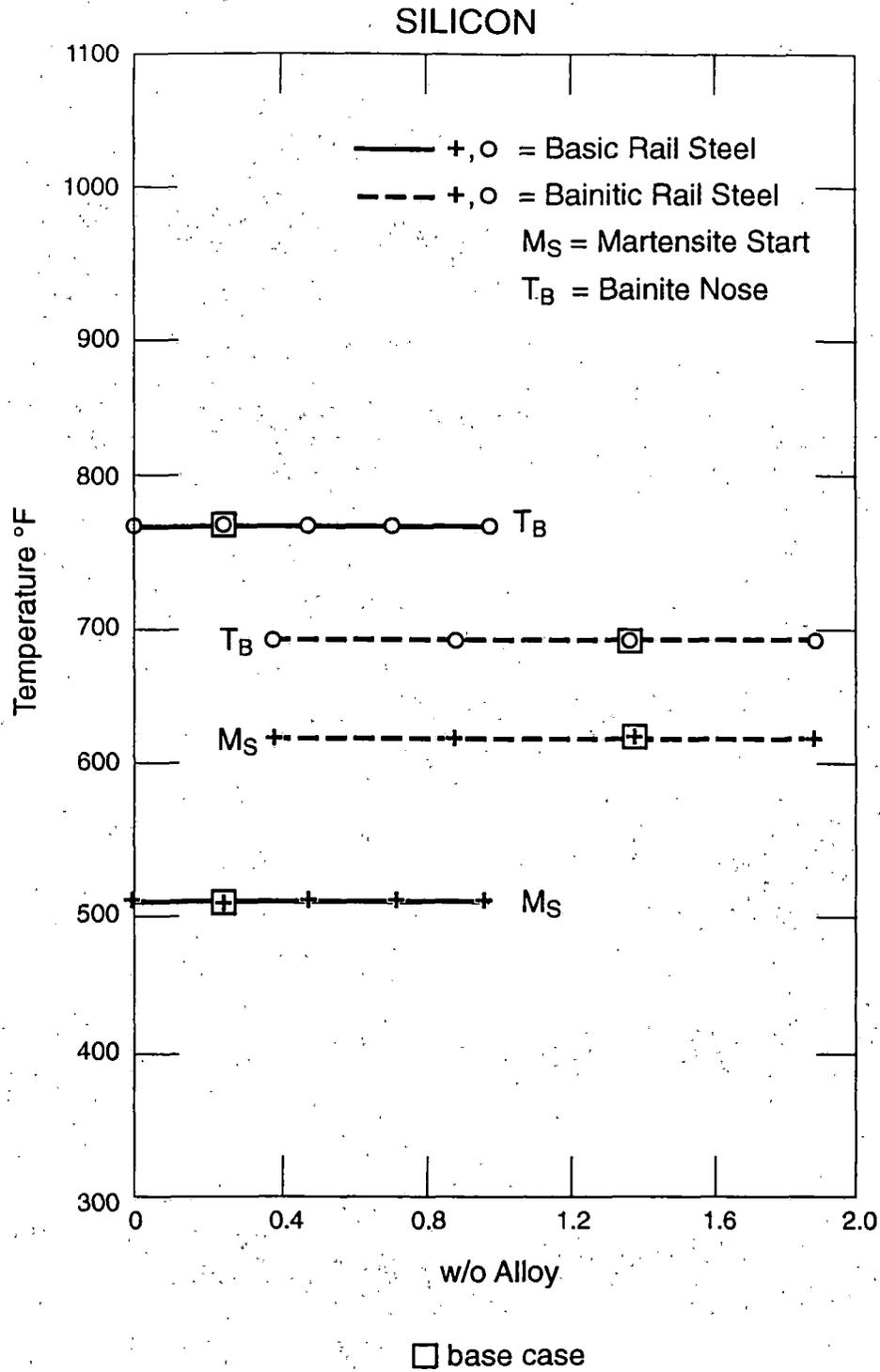
Figure 37: Effect of Silicon on the Martensite Start and Bainite Nose Temperatures
