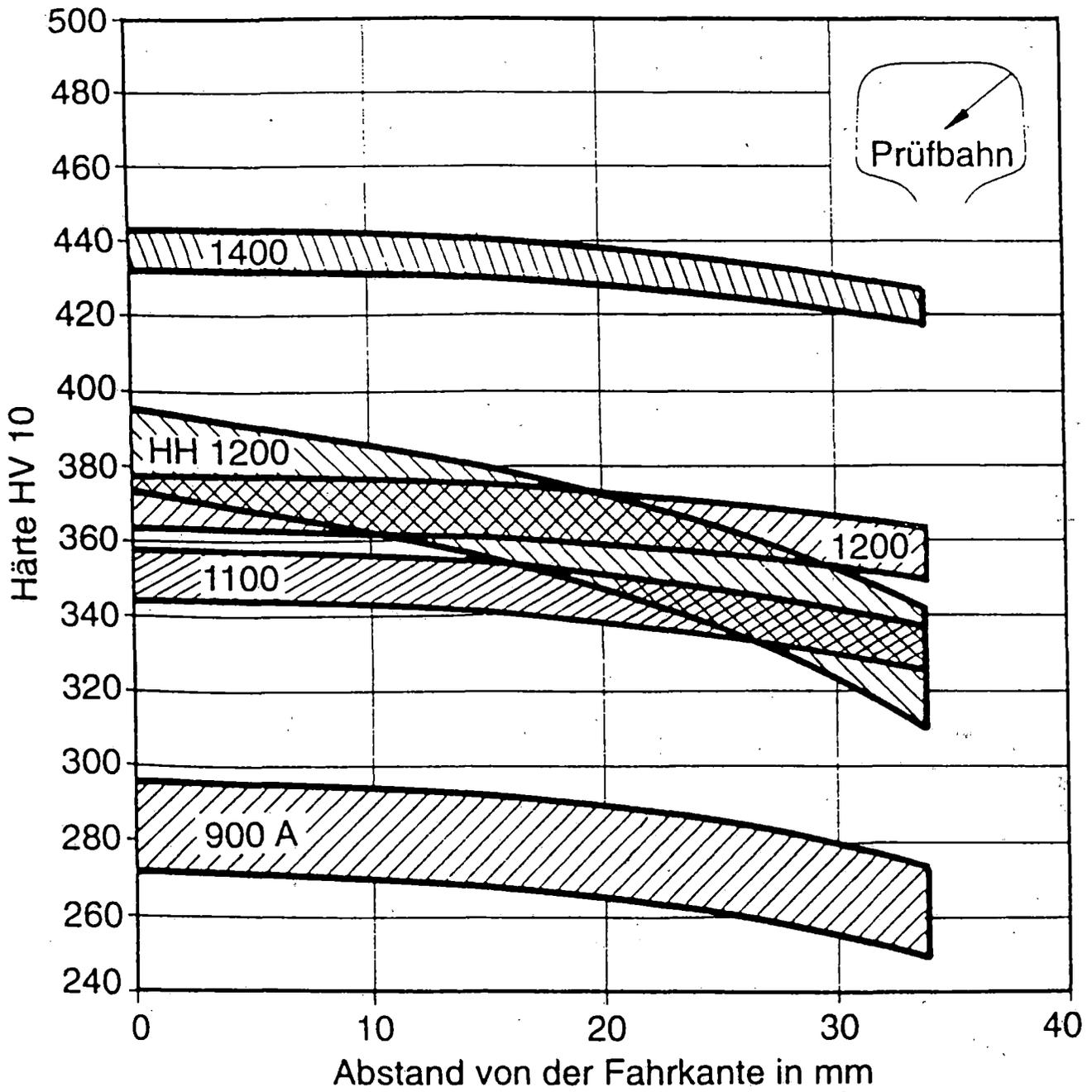
Figure 10: Hardness Traverses from Rail Head Corners
