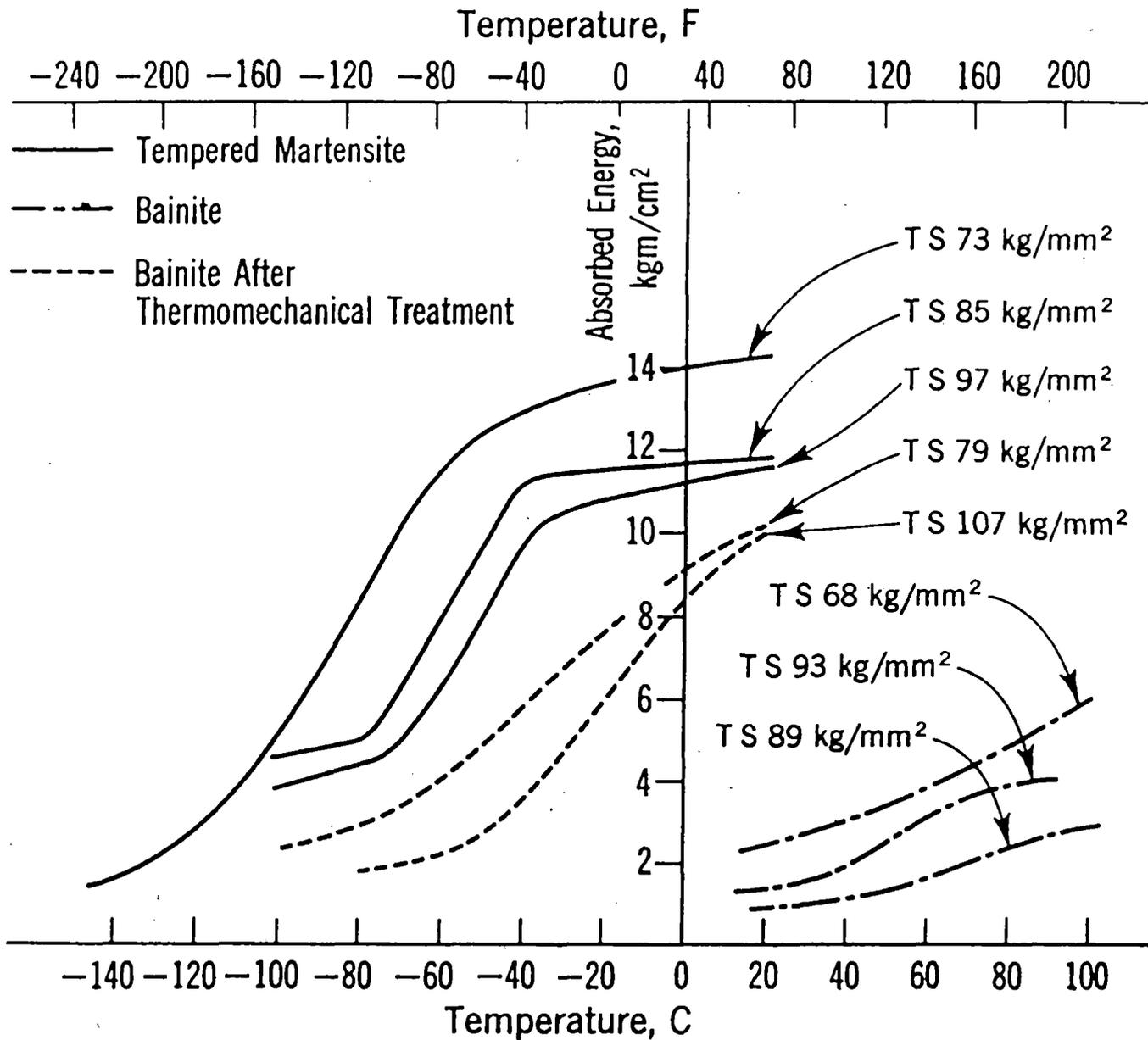
Figure 14: Impact Energy Transition Curves for a Manganese-Molybdenum-Boron Steel
