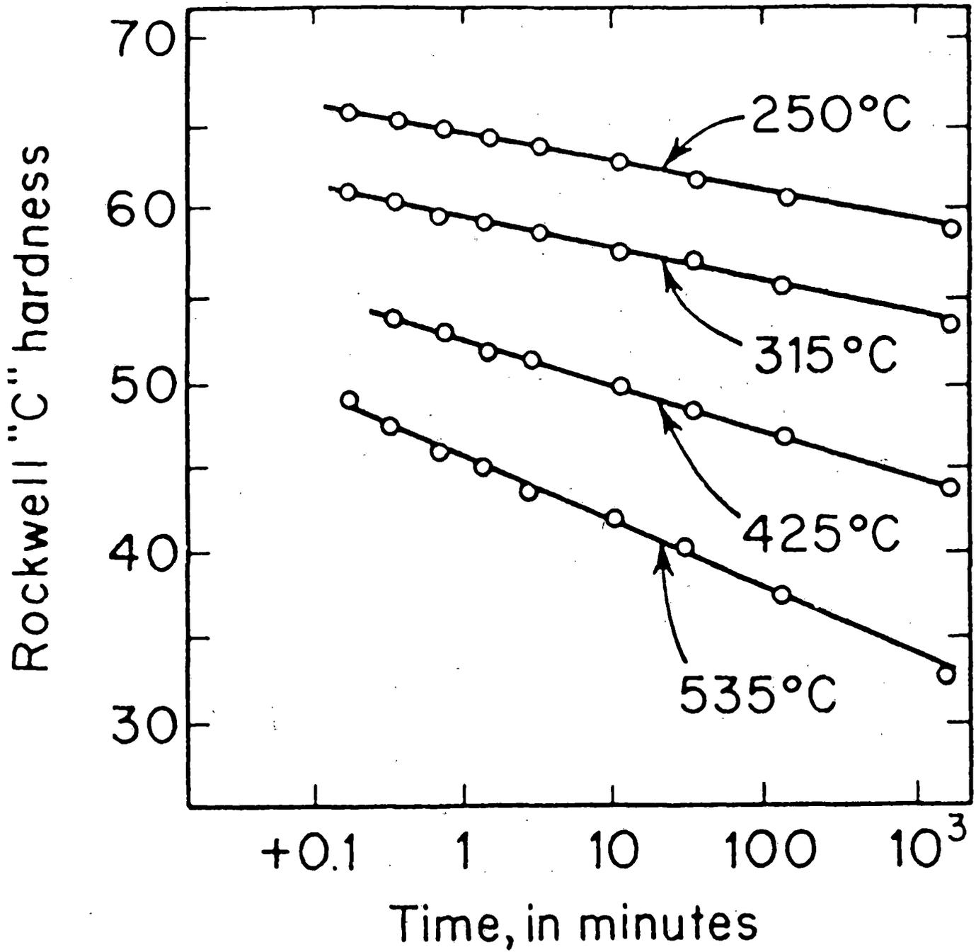
Figure 15: Decrease in Rockwell C Hardness of Eutectoid Steel for Different Tempering Times and Temperatures (Source: Bain, Ref 12)
