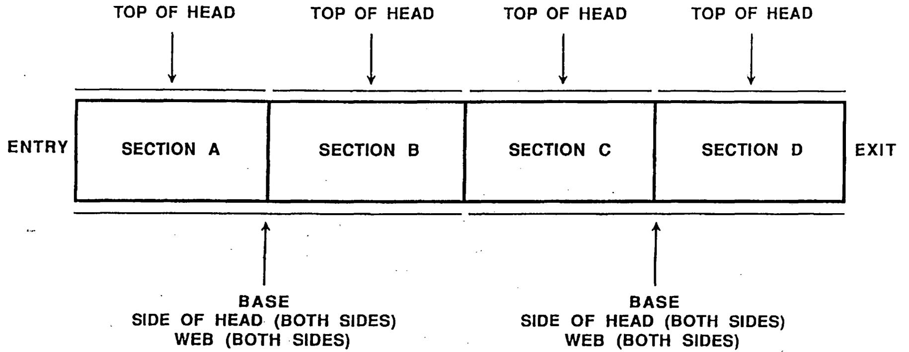
Figure 6: Illustration of Quenching Zones in In-Line Hardener (Source: Bramfitt et al, Ref 4)
