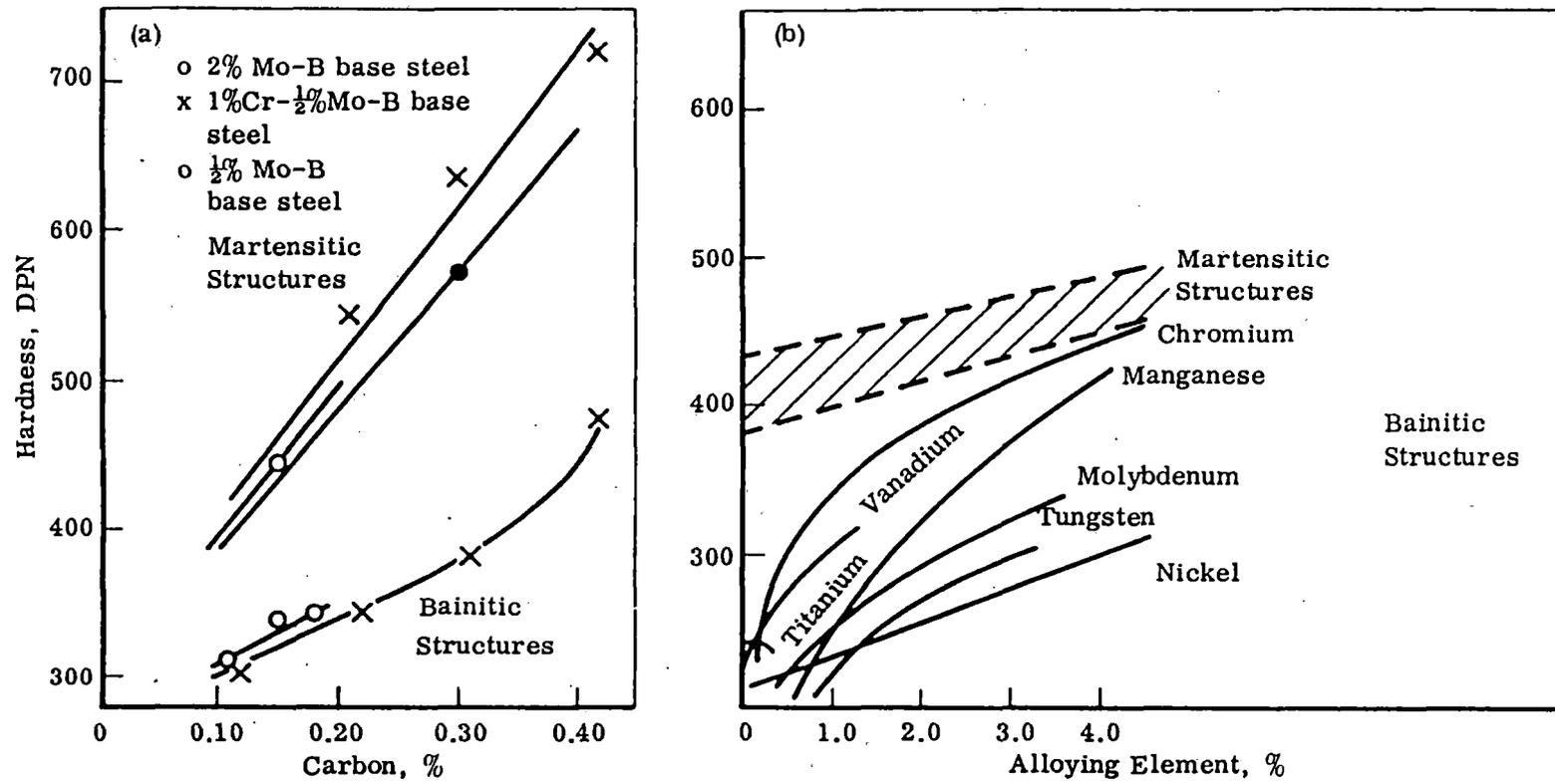
Figure 25: Effects of Carbon and Alloy Additions on Bainite and Martensite Hardness (Source: Irvine/Pickering, Ref 19)
