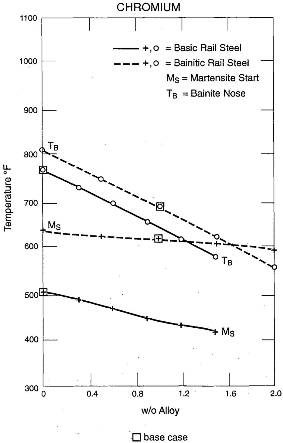
Figure 38: Effect of Chromium on the Martensite Start and Bainite Nose Temperatures
