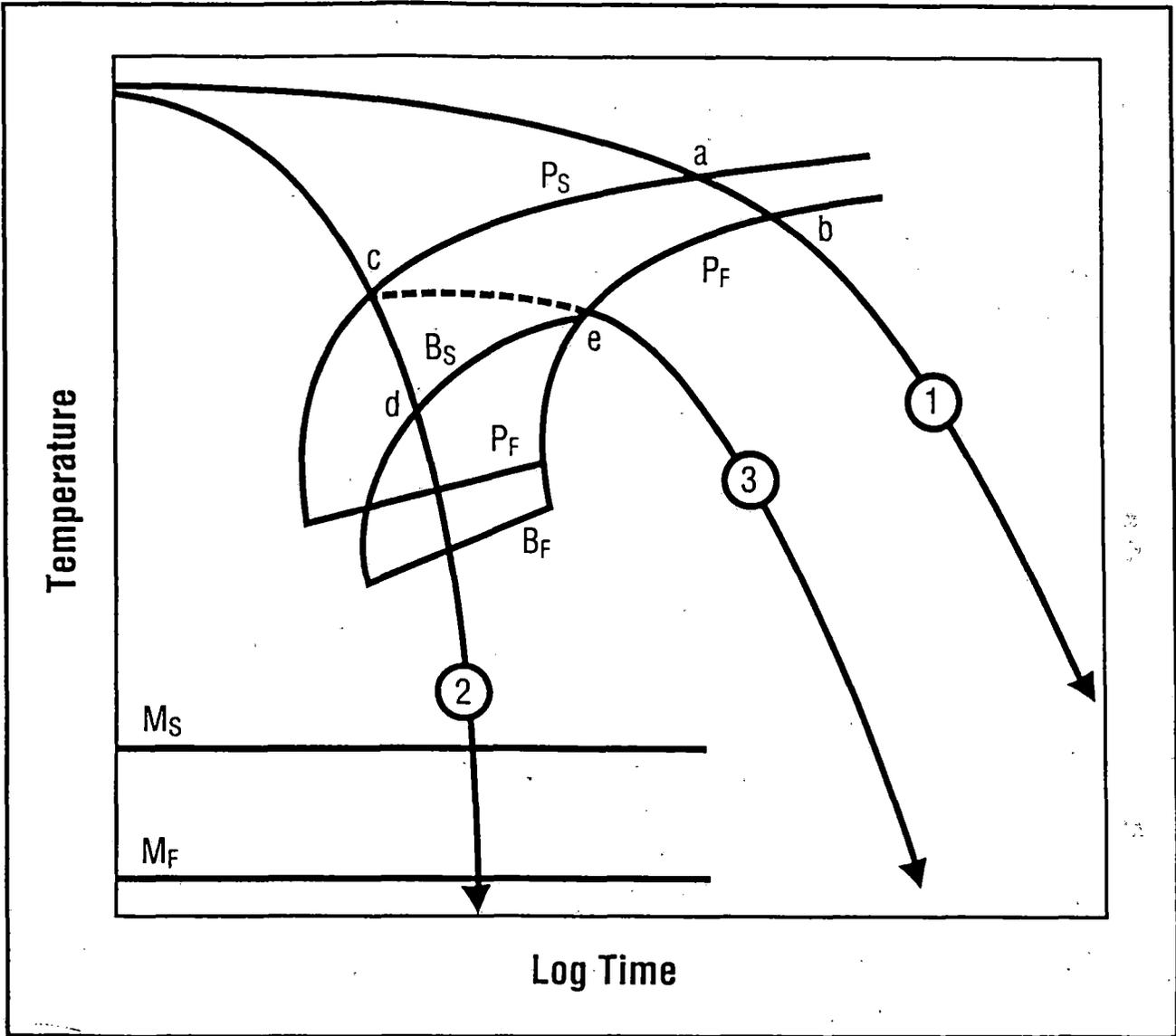
Figure 1: Schematic Representation of a Continuous Cooling Transformation Diagram of an Eutectoid Steel (Source: Kennon, Ref 7)
