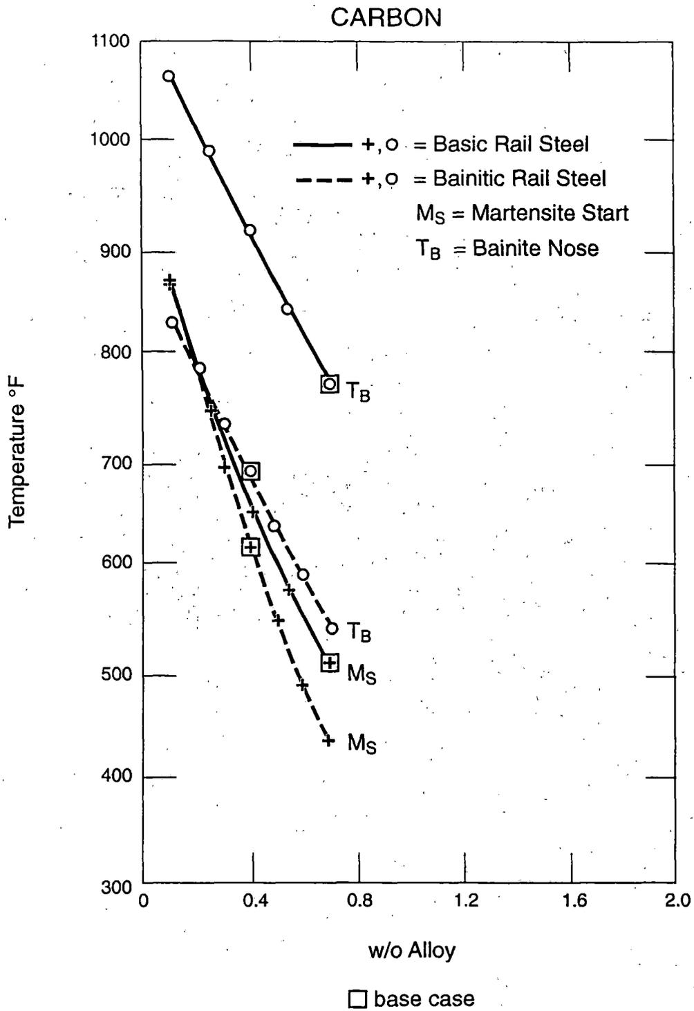
Figure 35: Effect of Carbon on the Martensite Start and Bainite Nose Temperatures
