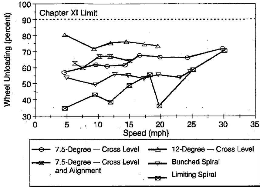
**Figure 8.13 Maximum Wheel Unloading on Curved-track, High Rail, Covered Hopper**
