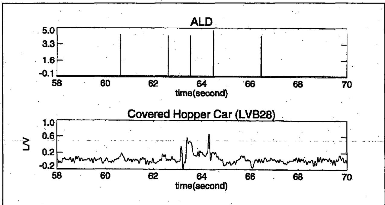
Figure 7.14 Wheel L/V Ratio Variations over a Cross Level/Alignment Perturbation
