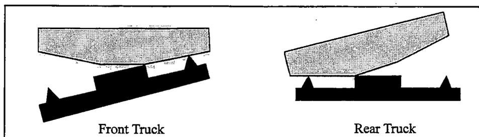
**Figure 1.1 Reaction of Vehicle to Track Twist**
