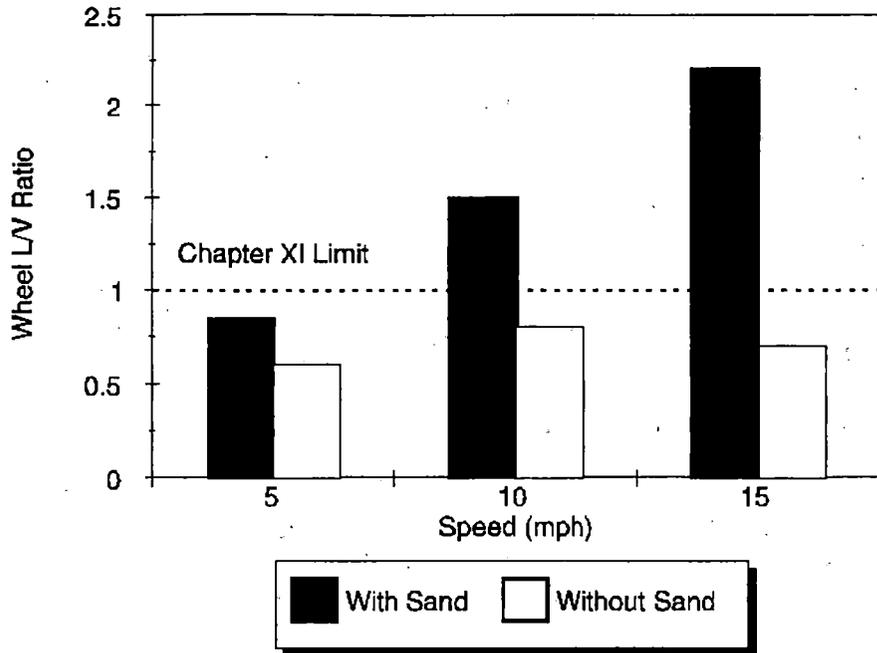
**Figure 8.15 Effect of Applying Sand on Curved-track**
