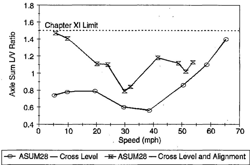
Figure 7.19 Axle Sum L/V Ratio on Tangent Track, Leading Axle, Covered Hopper
