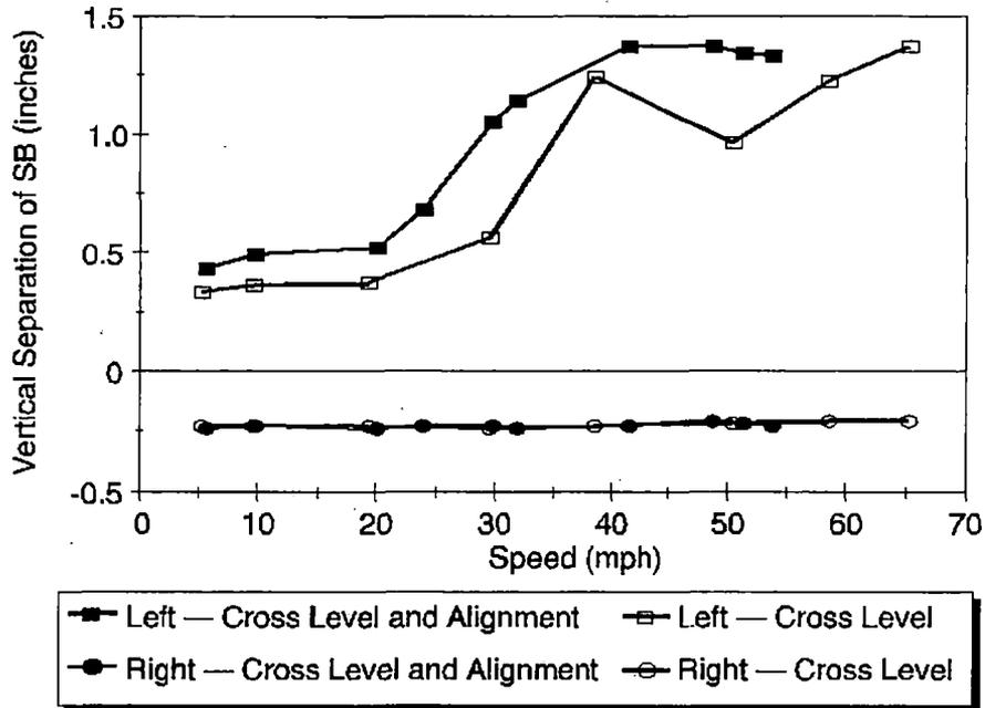
**Figure 7.23 Center Plate Separation Indicated by Displacement of Side Bearing, Leading Truck of Covered Hopper**
