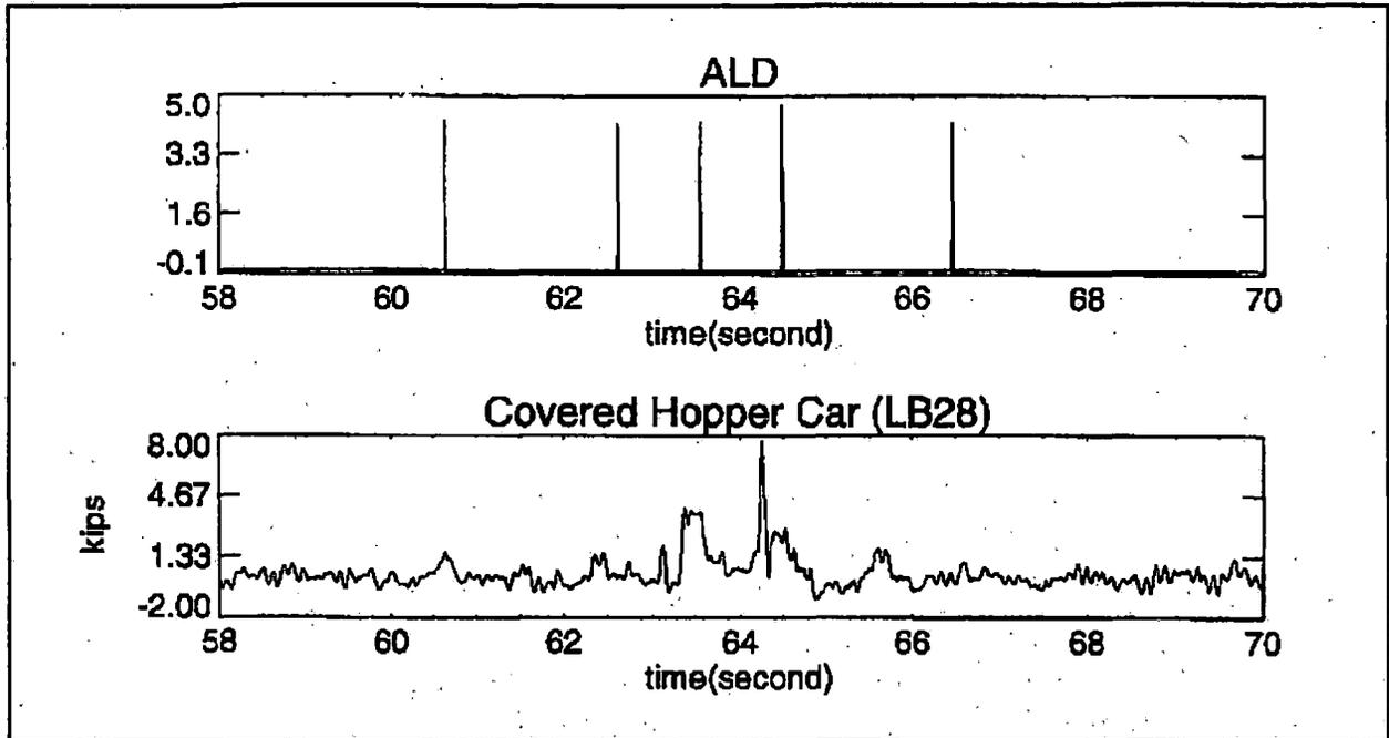
Figure 7.10 Wheel Lateral Force Variations over a Cross Level/Alignment Perturbation
