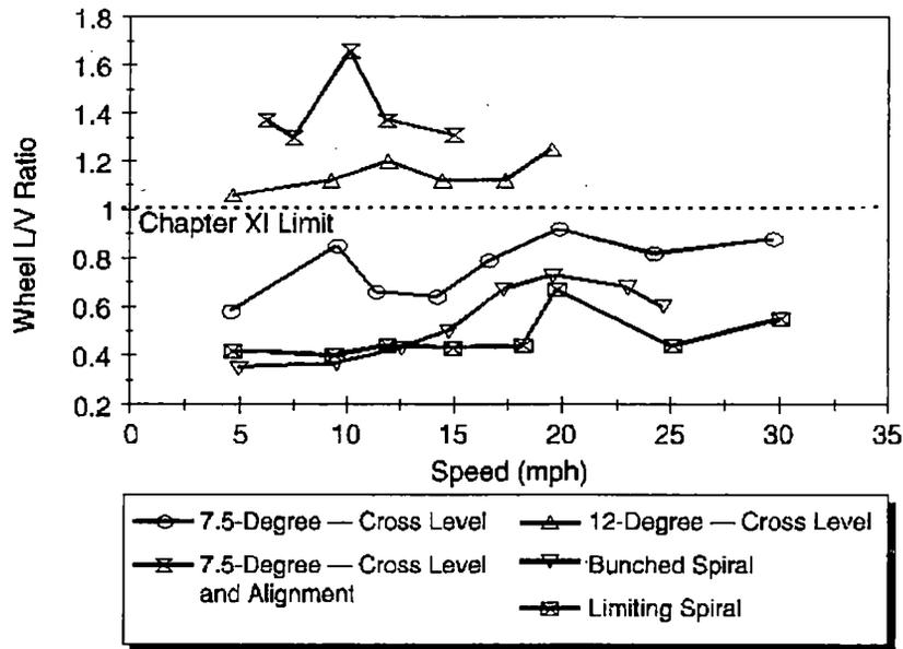
Figure 8.5 Maximum Wheel L/V Ratio on Curved-track, High Rail, Tank Car
