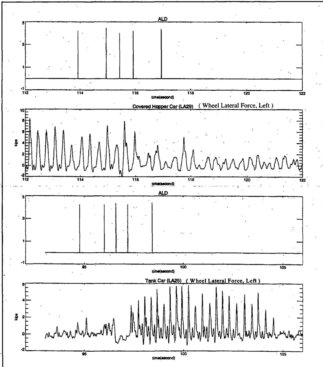
Figure 7.2 Effect of Track Perturbation to Vehicle Instability
