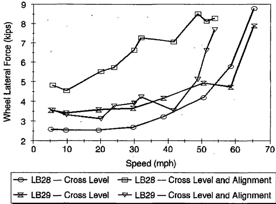
Figure 7.12 Wheel/Rail Lateral Force on Tangent Track, Right Wheels, Covered Hopper
