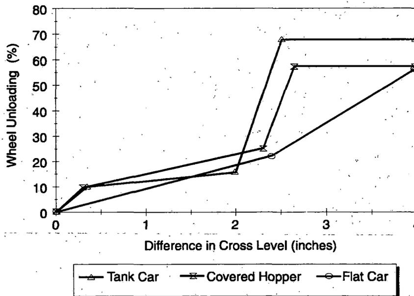
**Figure 3.1 Relationship Between Static Wheel Unloading and Cross Level Difference**
