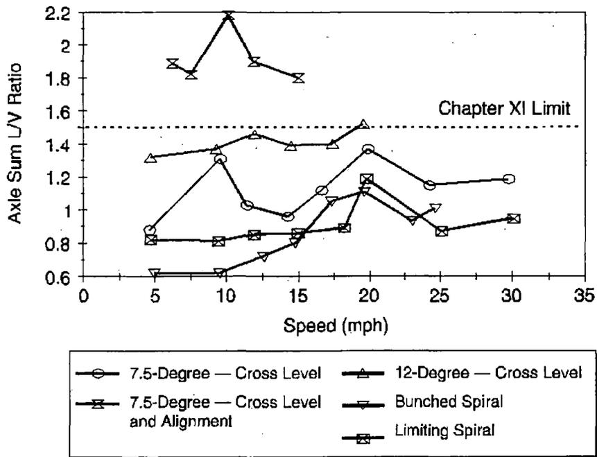
Figure 8.8 Maximum Axle Sum L/V Ratio on Curved-track High Rail, Tank Car
