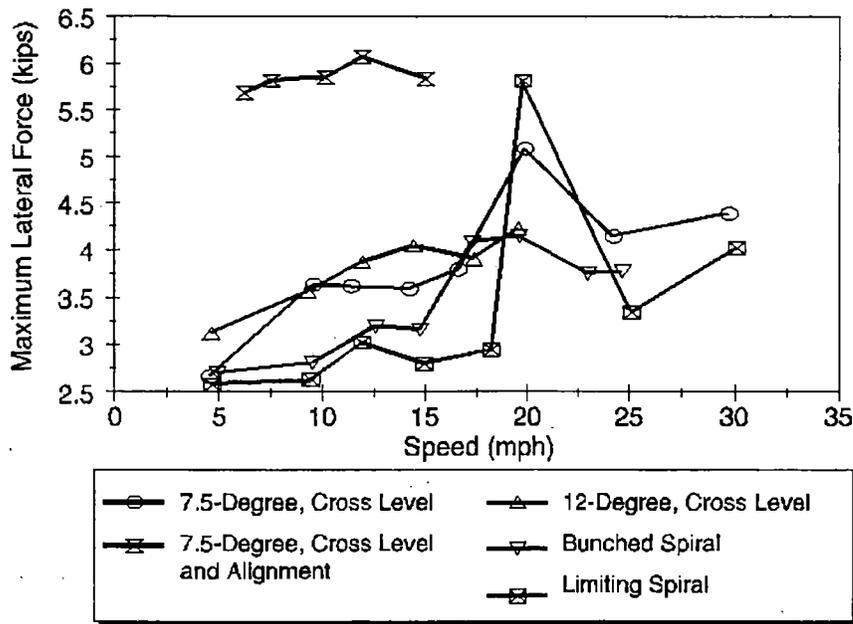
Figure 8.11 Maximum Wheel Lateral Forces on Curved-track, High Rail, Tank Car
