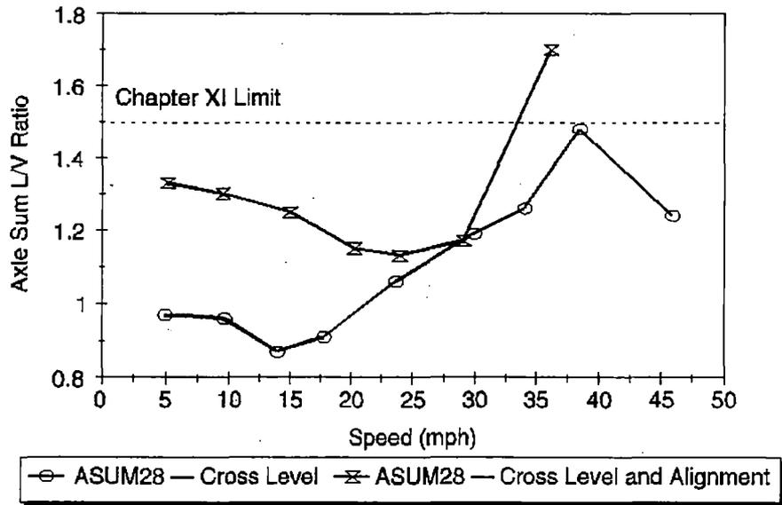
Figure 7.18 Axle Sum L/V Ratio on Tangent Track, Leading Axle, Flatcar
