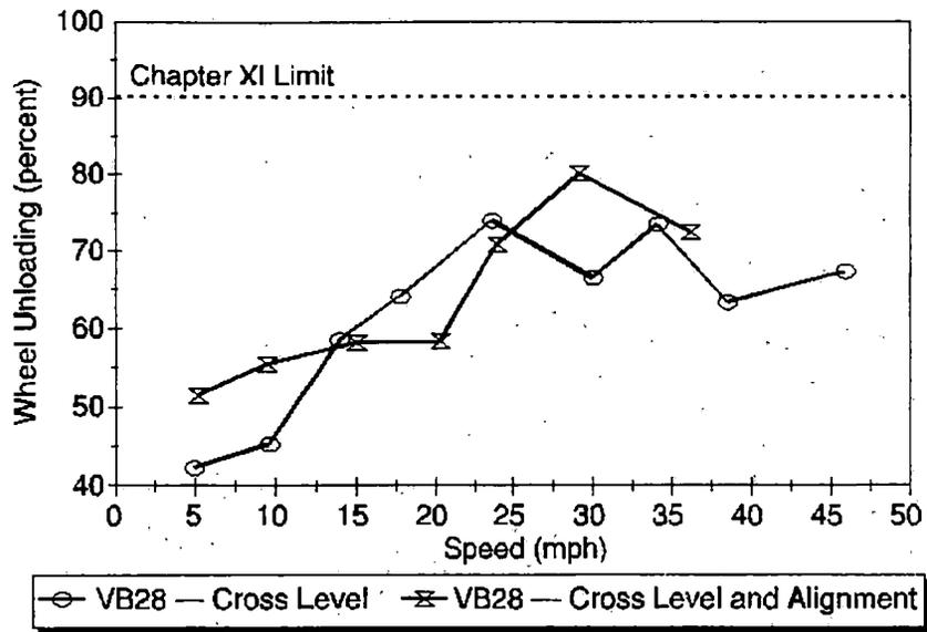
**Figure 7.5 Vertical Wheel Unloading on Tangent Track, Right Wheels, Flatcar**
