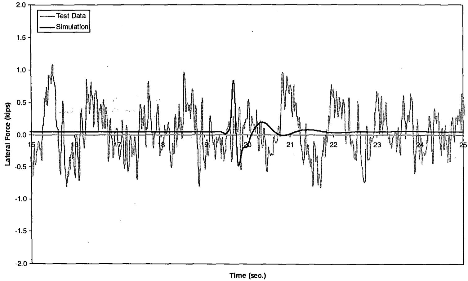
*Figure 5-44(d). Hunting test – lateral force time history, 130 mph (trailing right wheel)*
