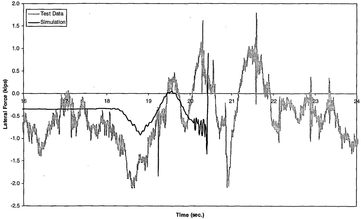
Figure 5-4(c). Vertical dip test – lateral force time history, 20 mph (trailing outer wheel)
