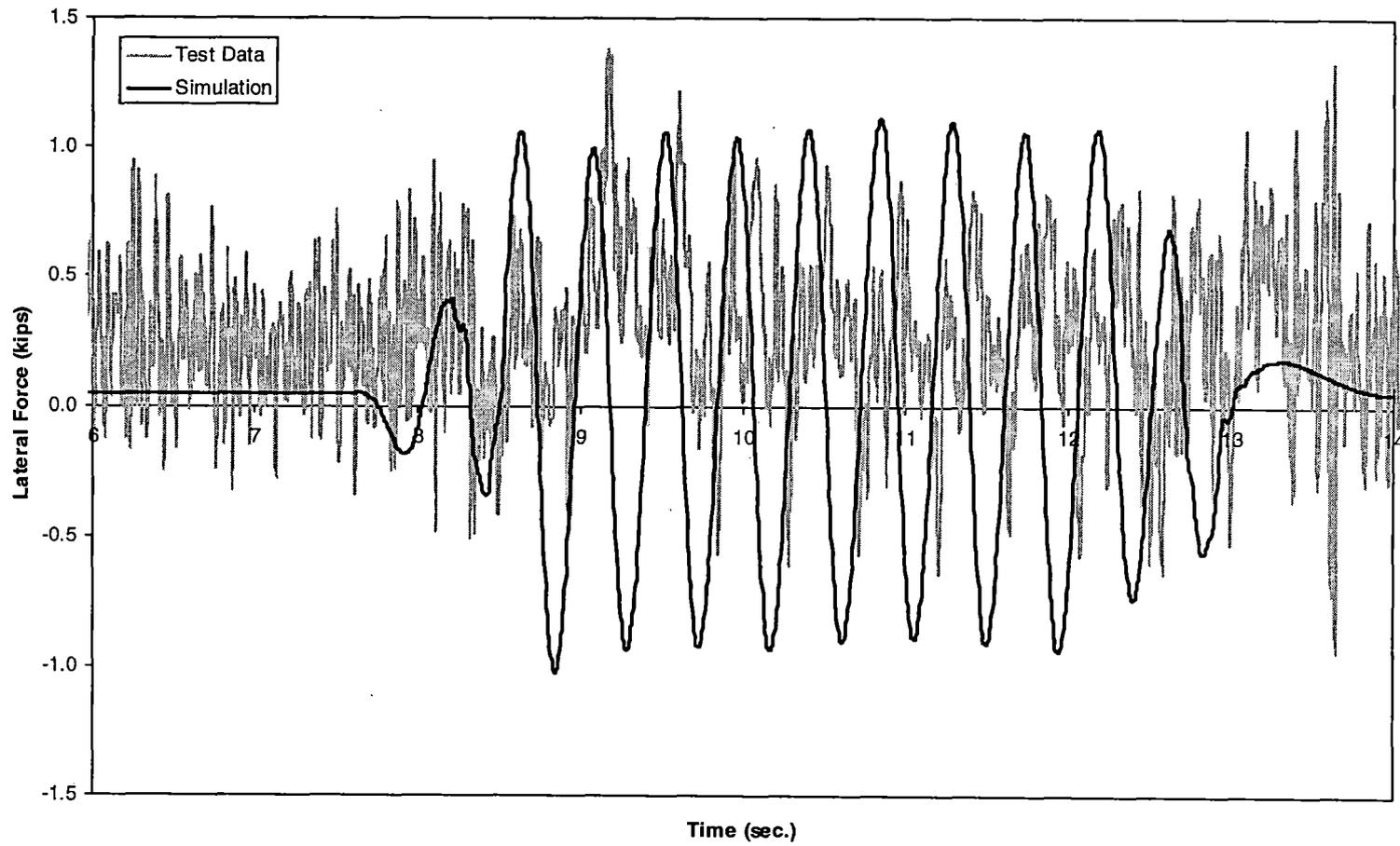
*Figure 5-35(c). Twist and roll – lateral force time history, 60 mph (trailing left wheel)*
