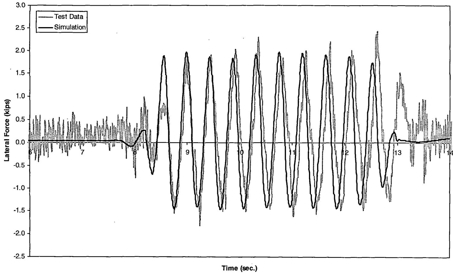
*Figure 5-35(a). Twist and roll – lateral force time history, 60 mph (lead left wheel)*
