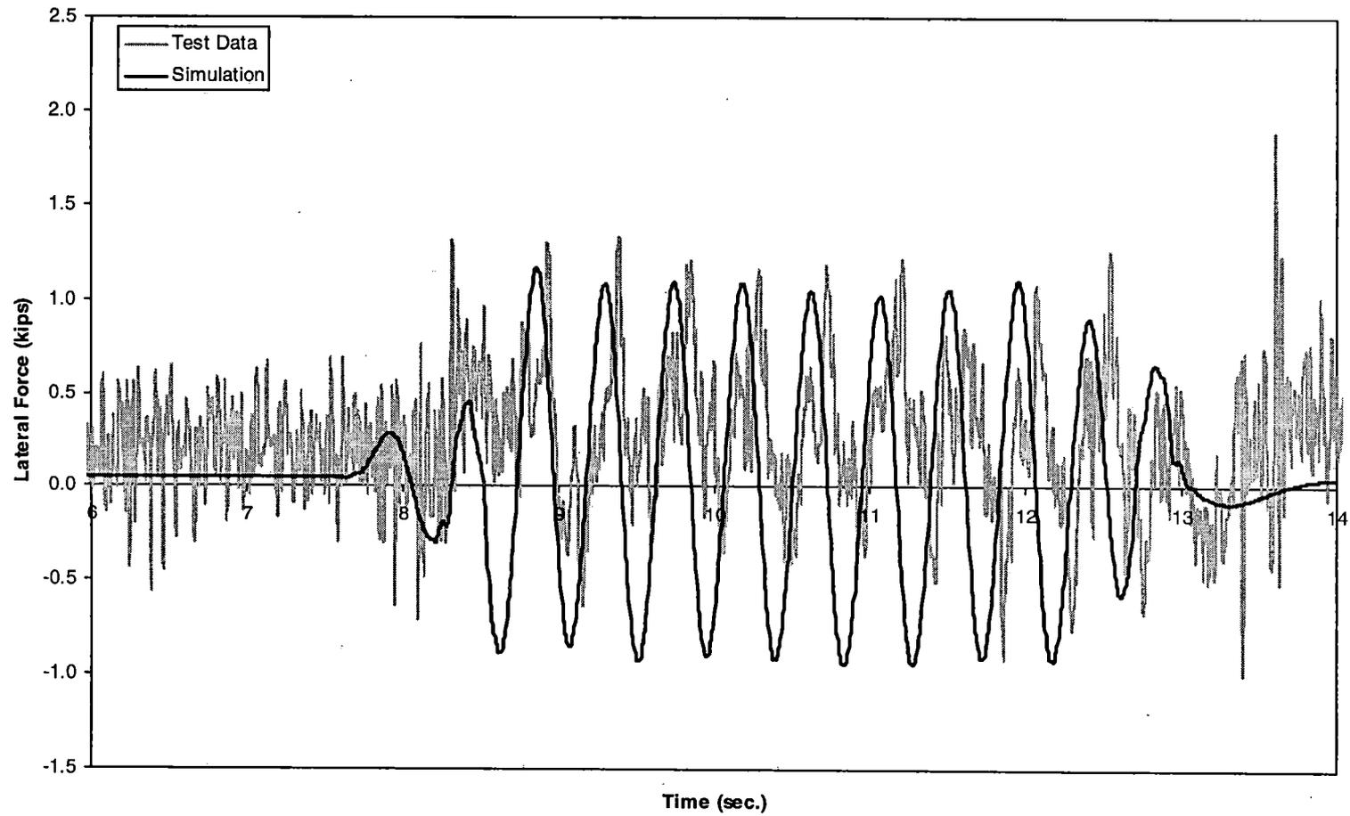
*Figure 5-35(d). Twist and roll – lateral force time history, 60 mph (trailing right wheel)*
