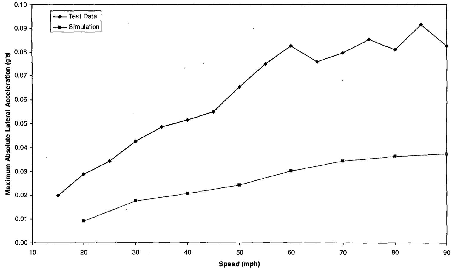
*Figure 5-30. Yaw and sway – maximum absolute lateral carbody acceleration*
