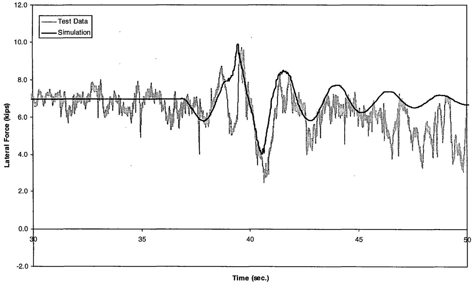
**Figure 5-6(b).** Vertical dip test – lateral force time history, 15 mph (lead inner wheel)
