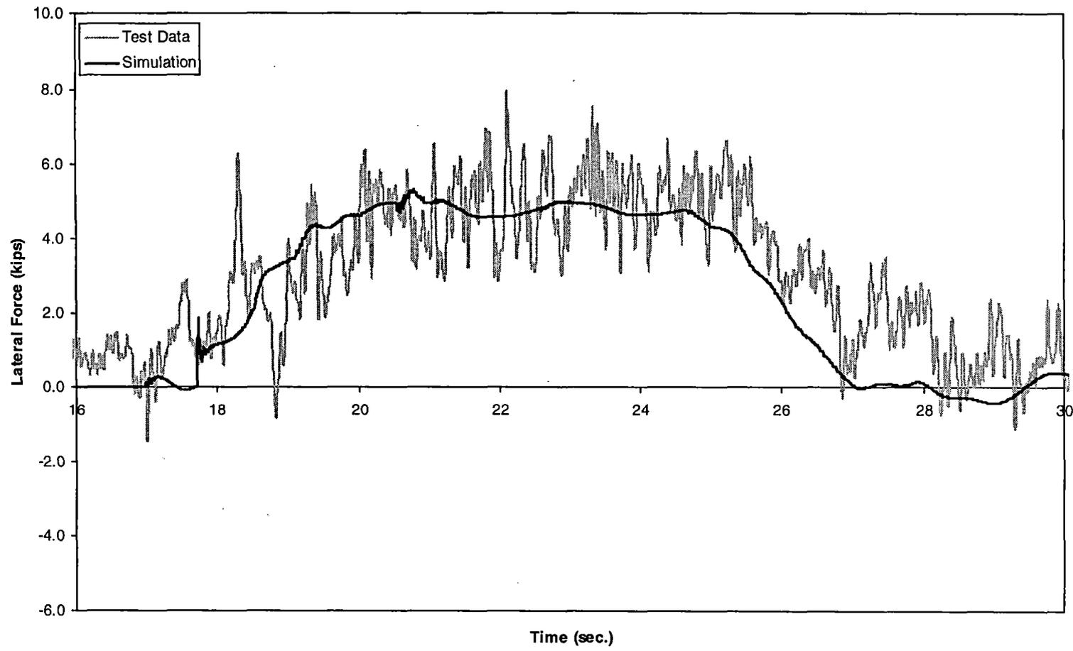
*Figure 5-13(a). Steady curving – net axle lateral force time history, 124 mph (lead axle)*
