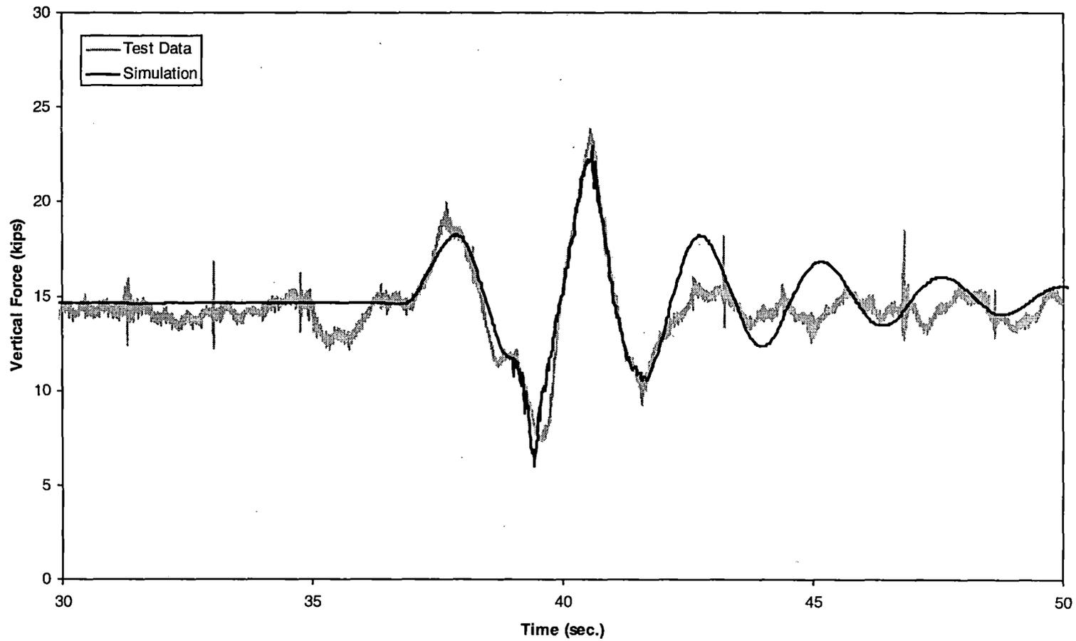
*Figure 5-5(a). Vertical dip test – vertical force time history, 15 mph (lead outer wheel)*
