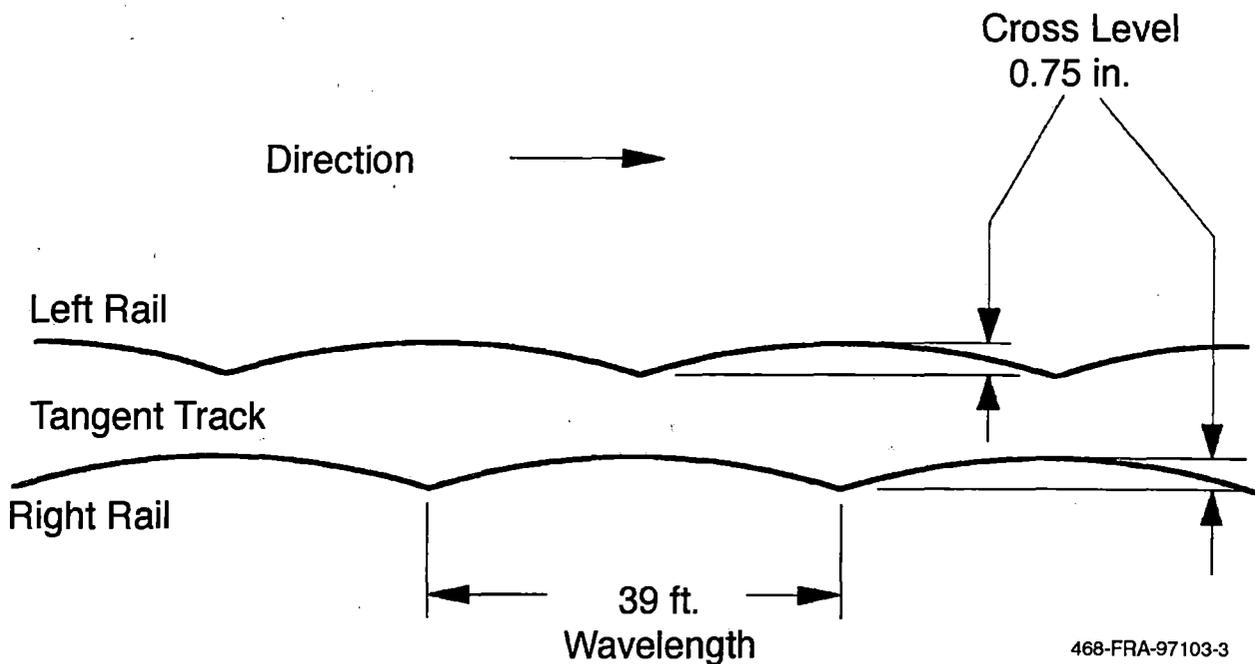
**Figure 5-31.** Crosslevel variation for twist and roll
