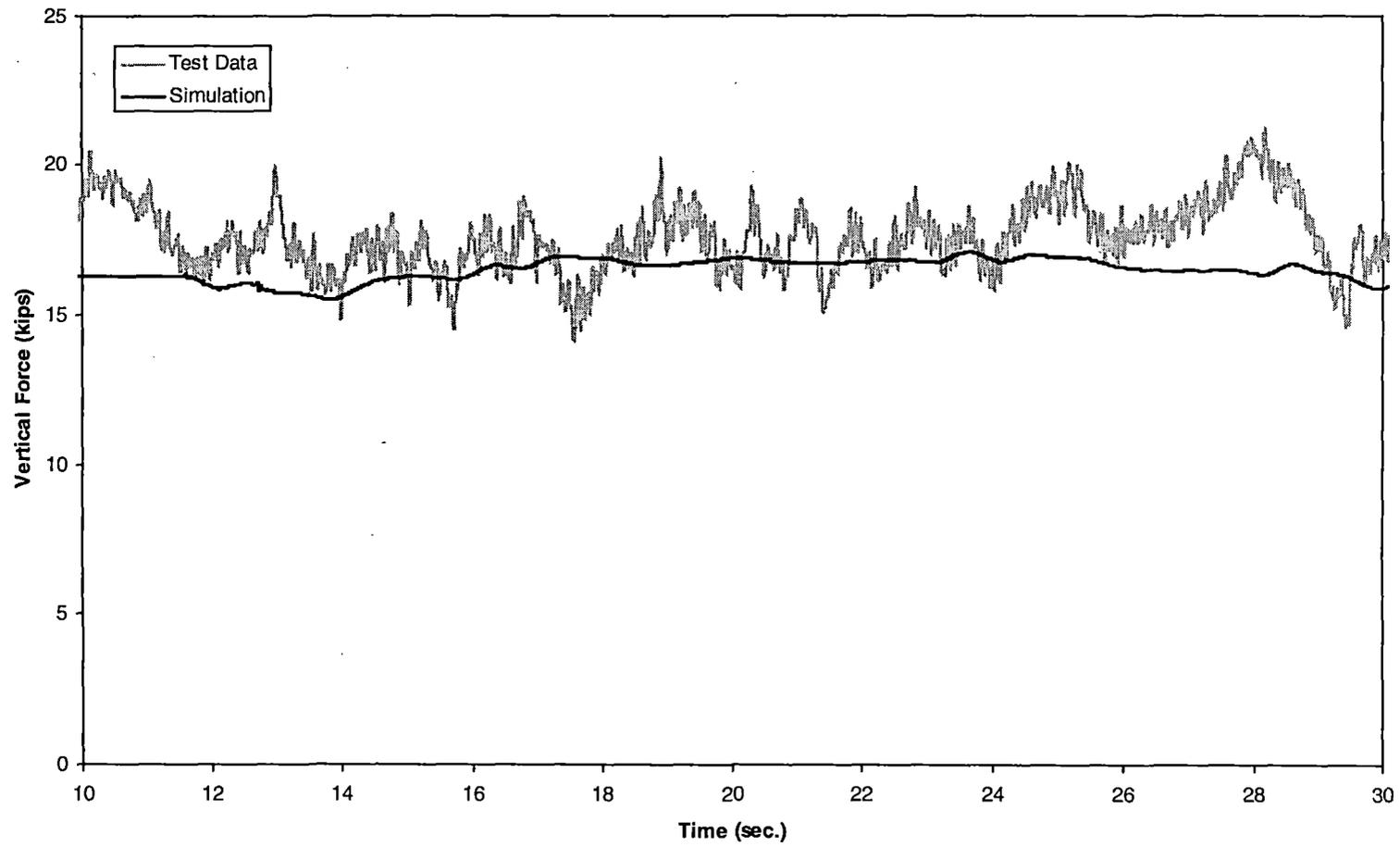
*Figure 5-8(d). Steady curving – vertical force time history, 84 mph (trailing inner wheel)*
