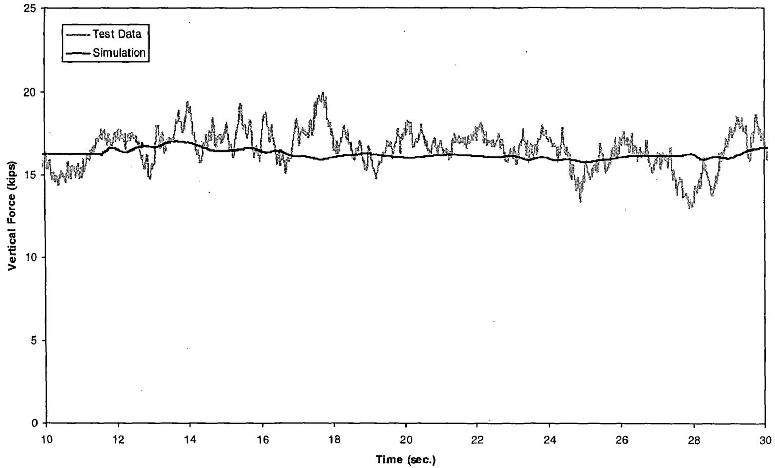
*Figure 5-8(c). Steady curving – vertical force time history, 84 mph (trailing outer wheel)*
