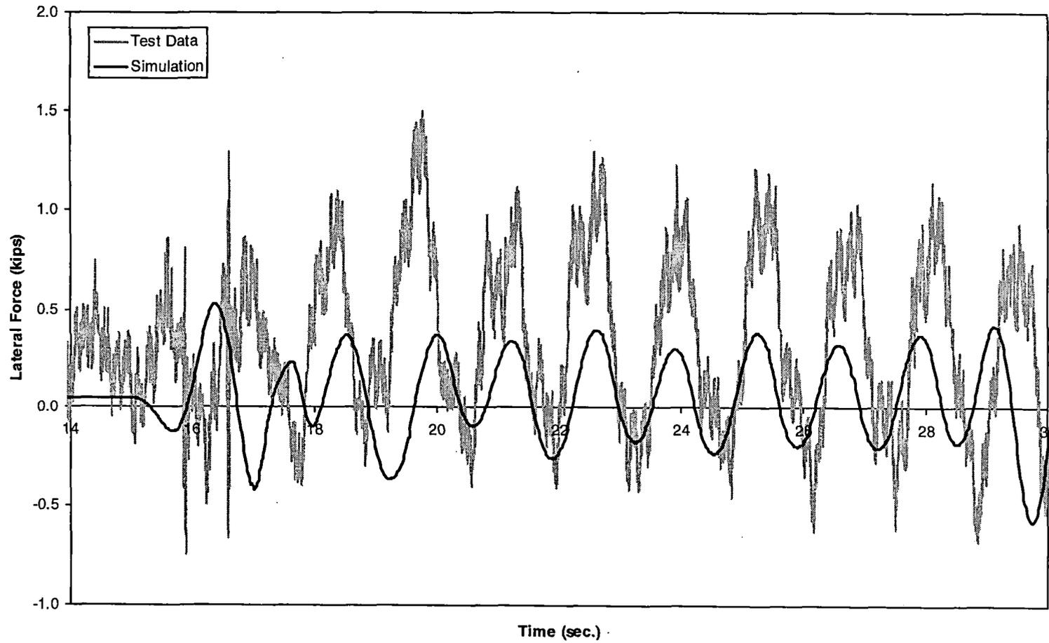
*Figure 5-33(c). Twist and roll – lateral force time history, 20 mph (trailing left wheel)*
