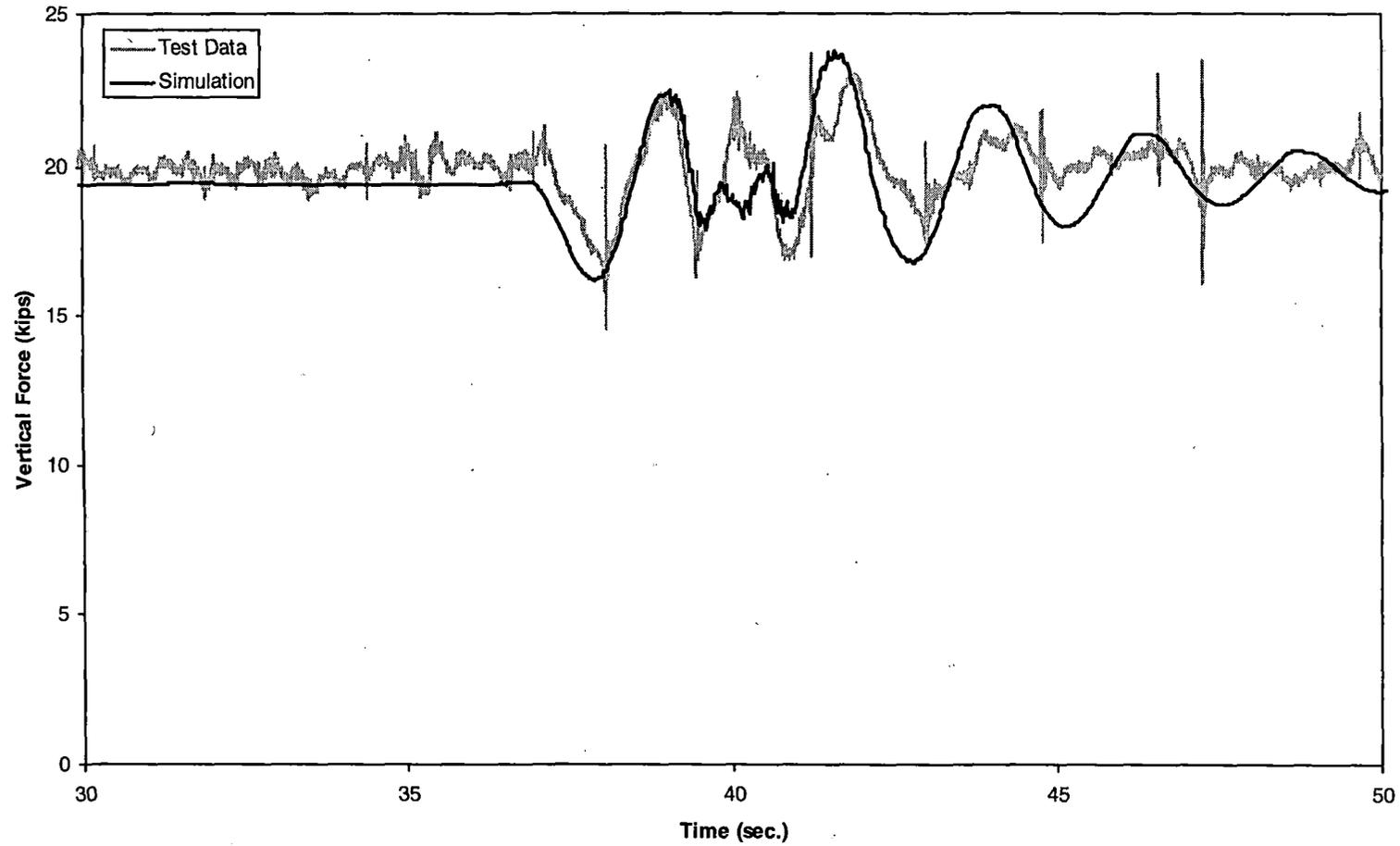
*Figure 5-5(d). Vertical dip test – vertical force time history, 15 mph (trailing inner wheel)*
