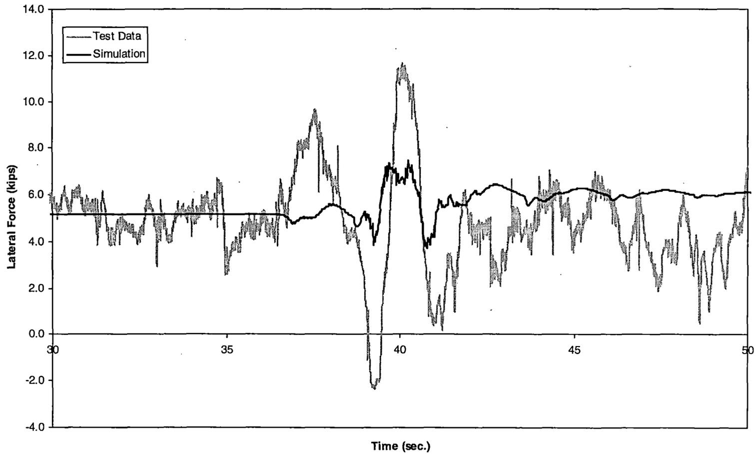
*Figure 5-6(a). Vertical dip test – lateral force time history, 15 mph (lead outer wheel)*
