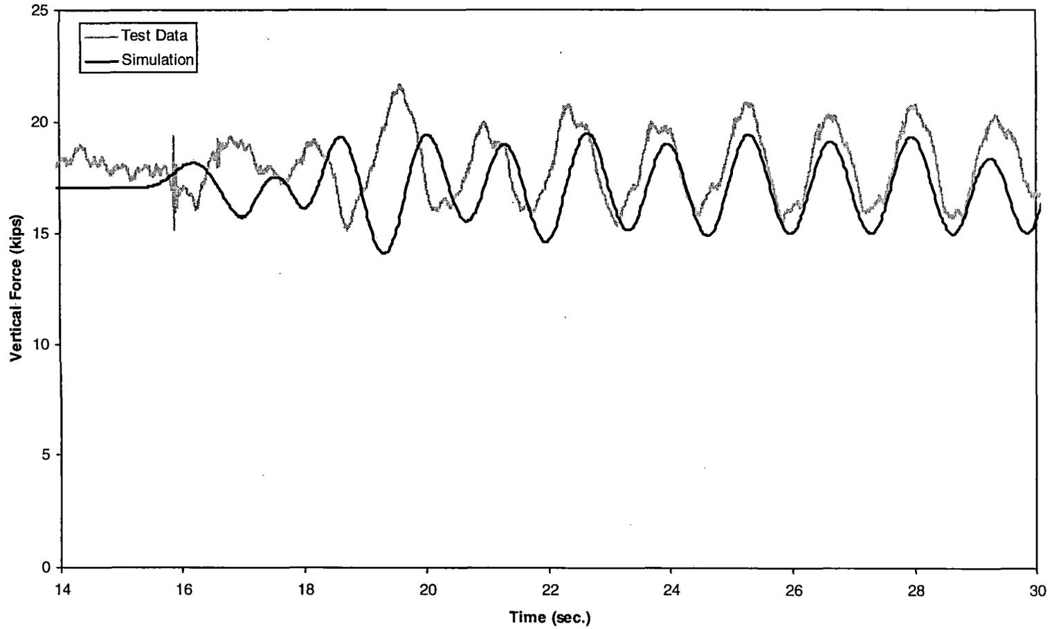
*Figure 5-32(c). Twist and roll – vertical force time history, 20 mph (trailing left wheel)*
