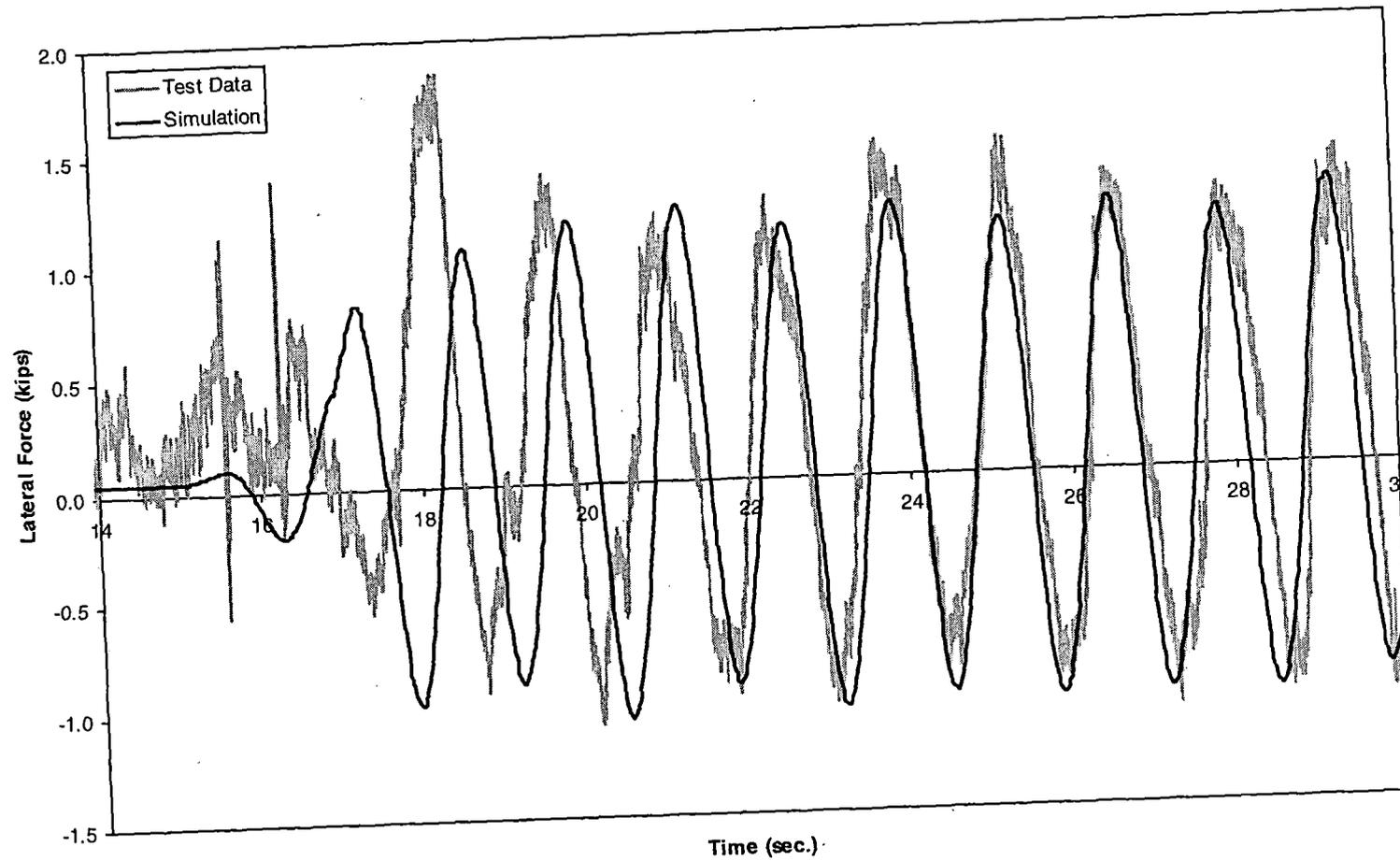
*Figure 5-33(b). Twist and roll – lateral force time history, 20 mph (lead right wheel)*
