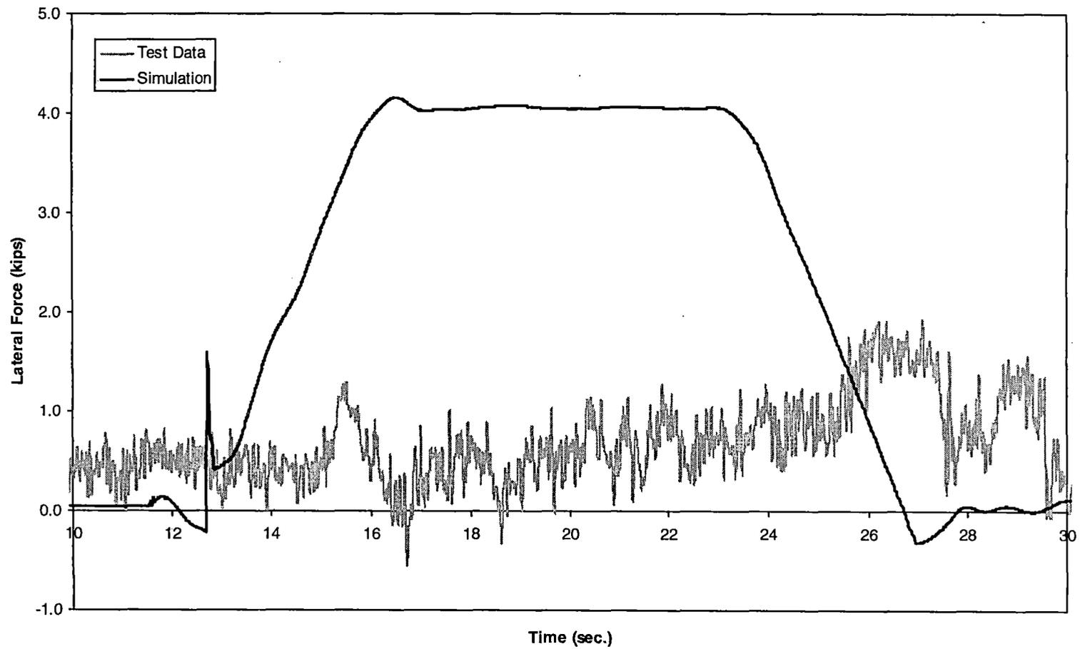
*Figure 5-9(a). Steady curving – lateral force time history, 84 mph (lead outer wheel)*
