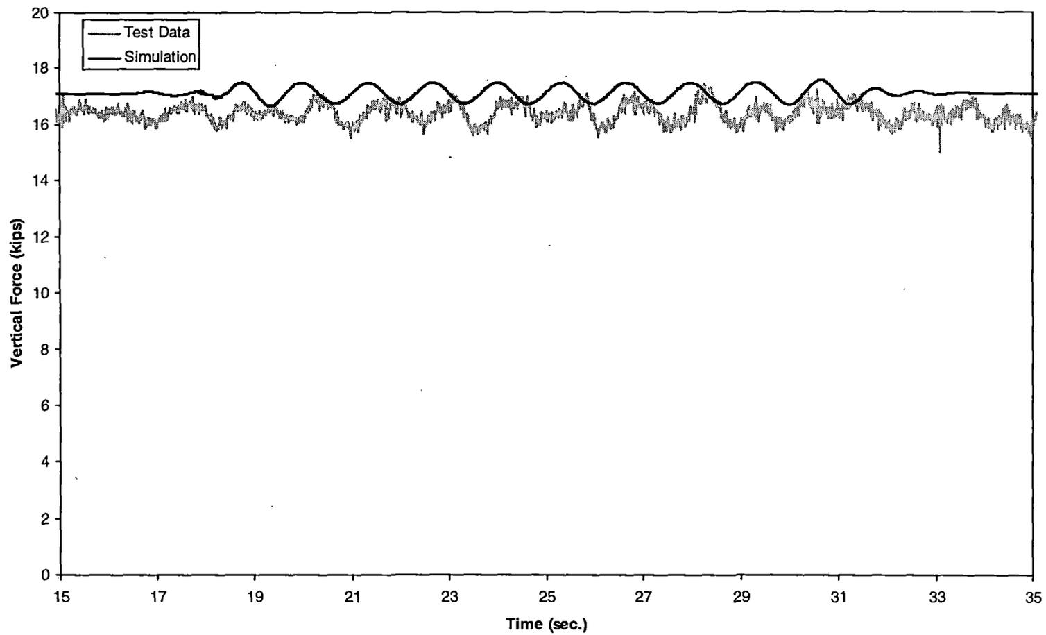
*Figure 5-40(d). Pitch and bounce – vertical force time history, 20 mph (trailing right wheel)*
