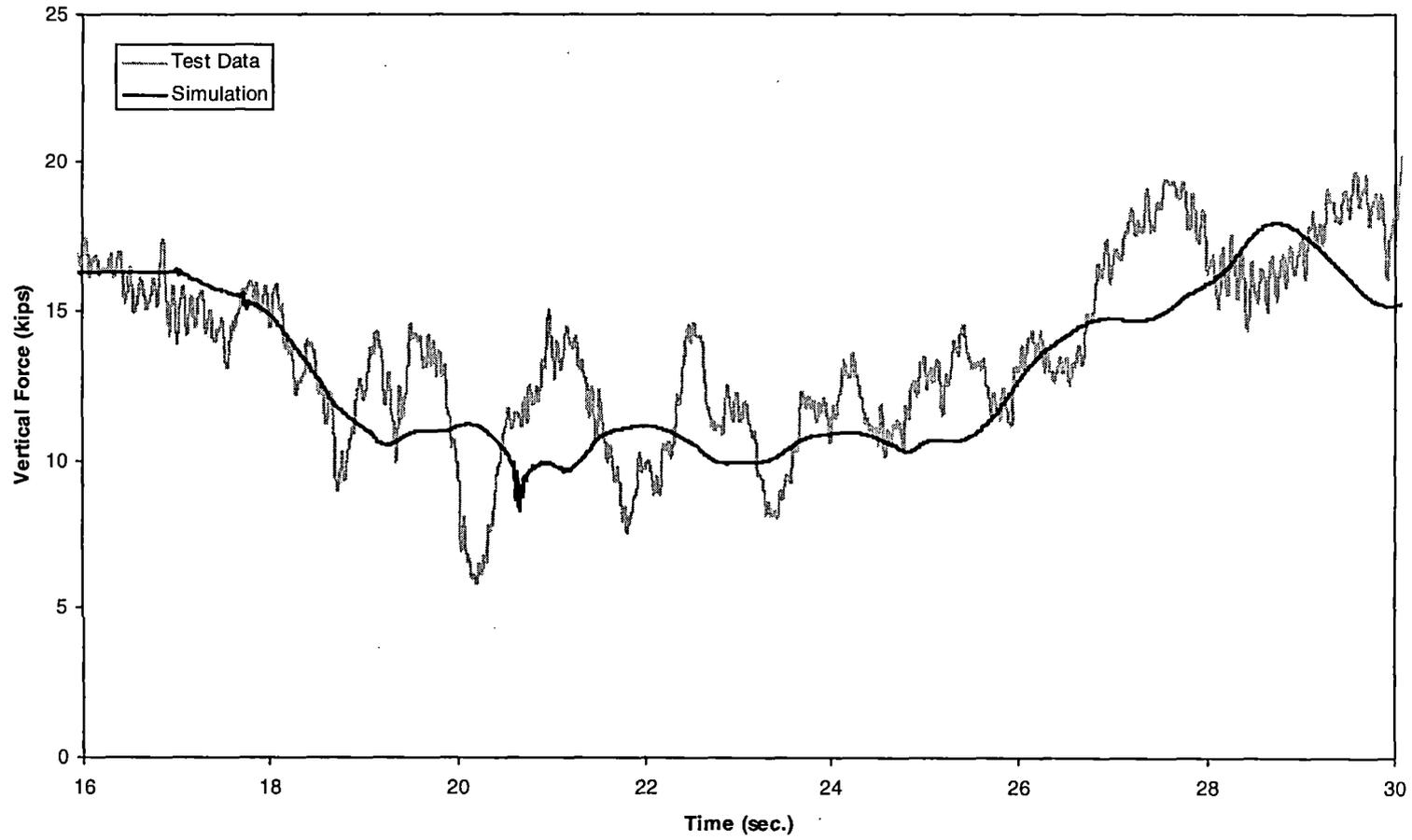
*Figure 5-11(d). Steady curving – vertical force time history, 124 mph (trailing inner wheel)*
