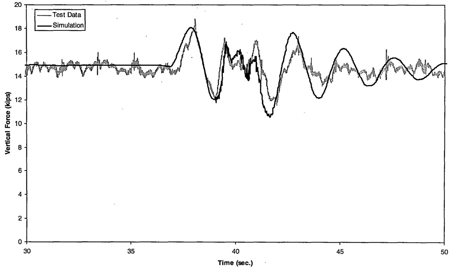
*Figure 5-5(c). Vertical dip test – vertical force time history, 15 mph (trailing outer wheel)*
