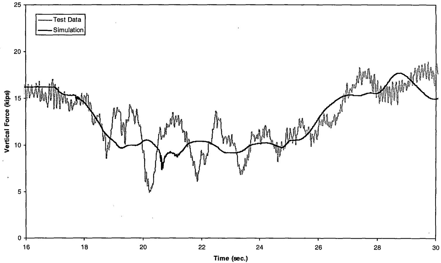
*Figure 5-11(b). Steady curving – vertical force time history, 124 mph (lead inner wheel)*
