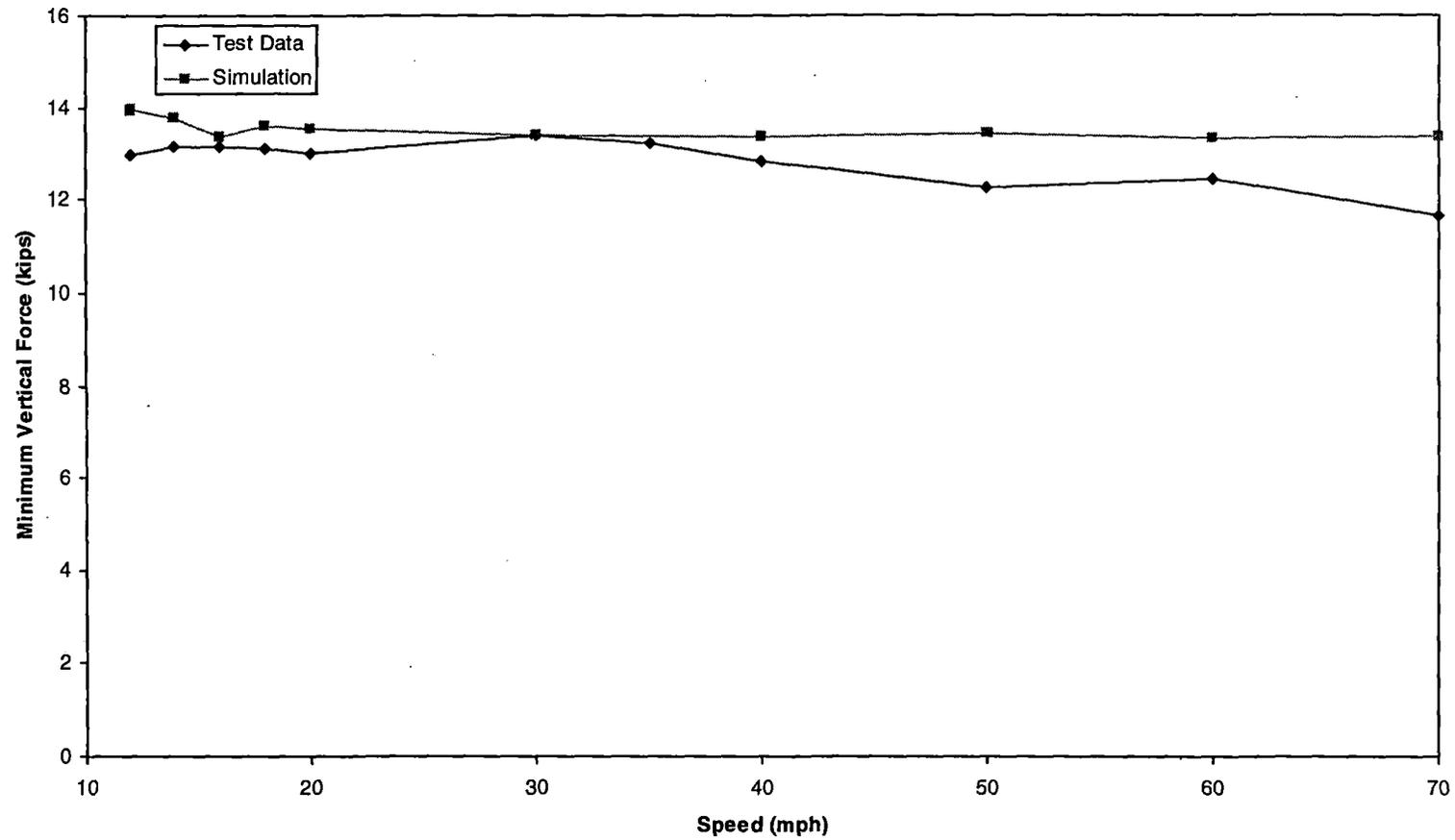
*Figure 5-36. Twist and roll – minimum vertical force*
