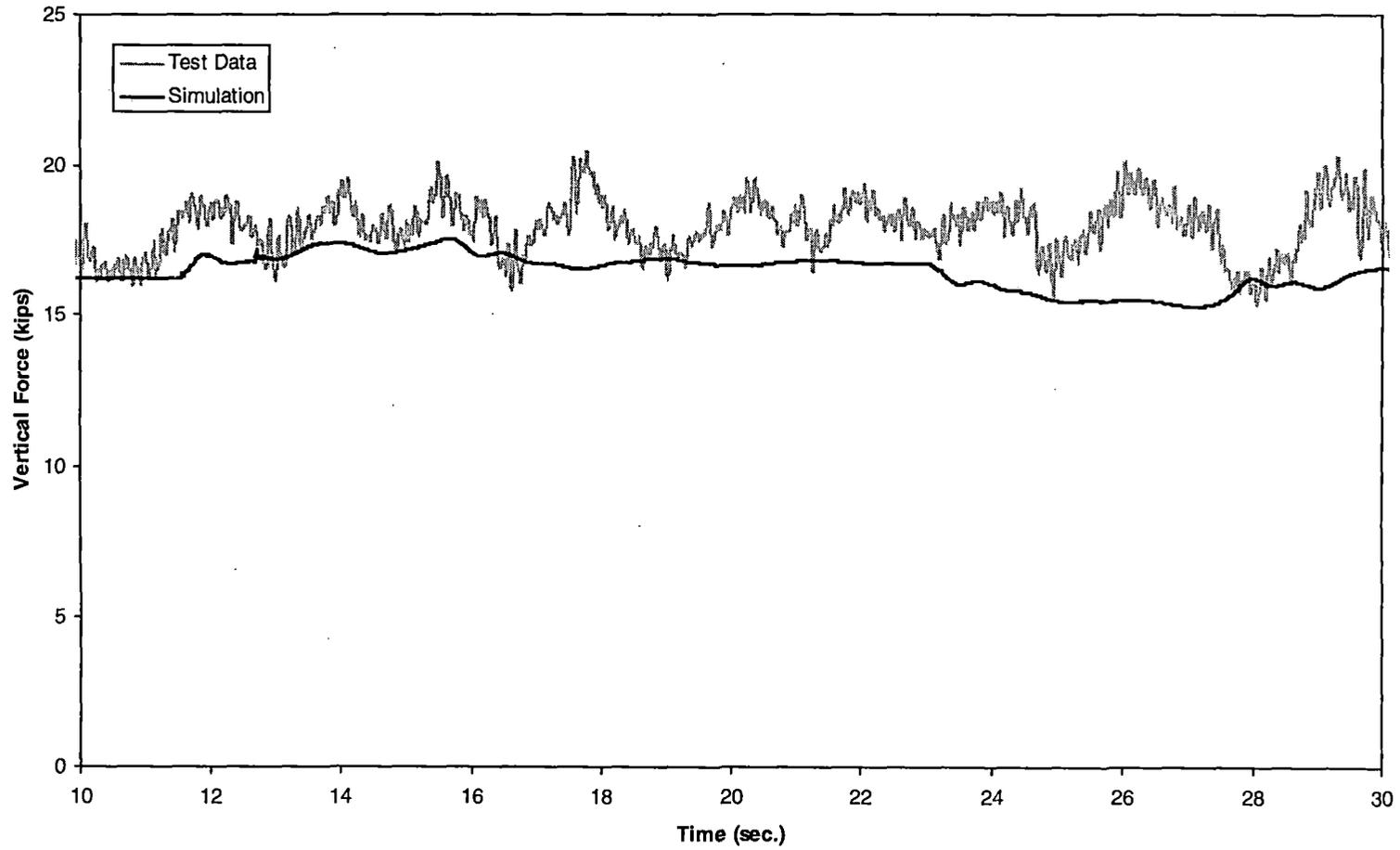
*Figure 5-8(b). Steady curving – vertical force time history, 84 mph (lead inner wheel)*
