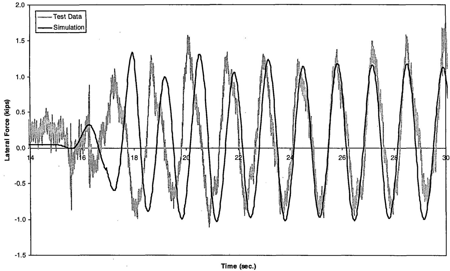
*Figure 5-33(a). Twist and roll – lateral force time history, 20 mph (lead left wheel)*
