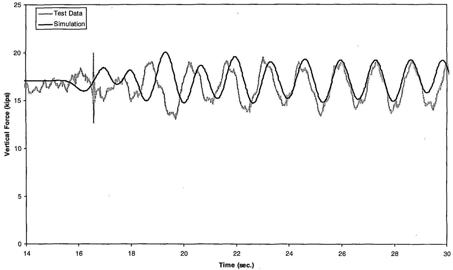
*Figure 5-32(d). Twist and roll – vertical force time history, 20 mph (trailing right wheel)*
