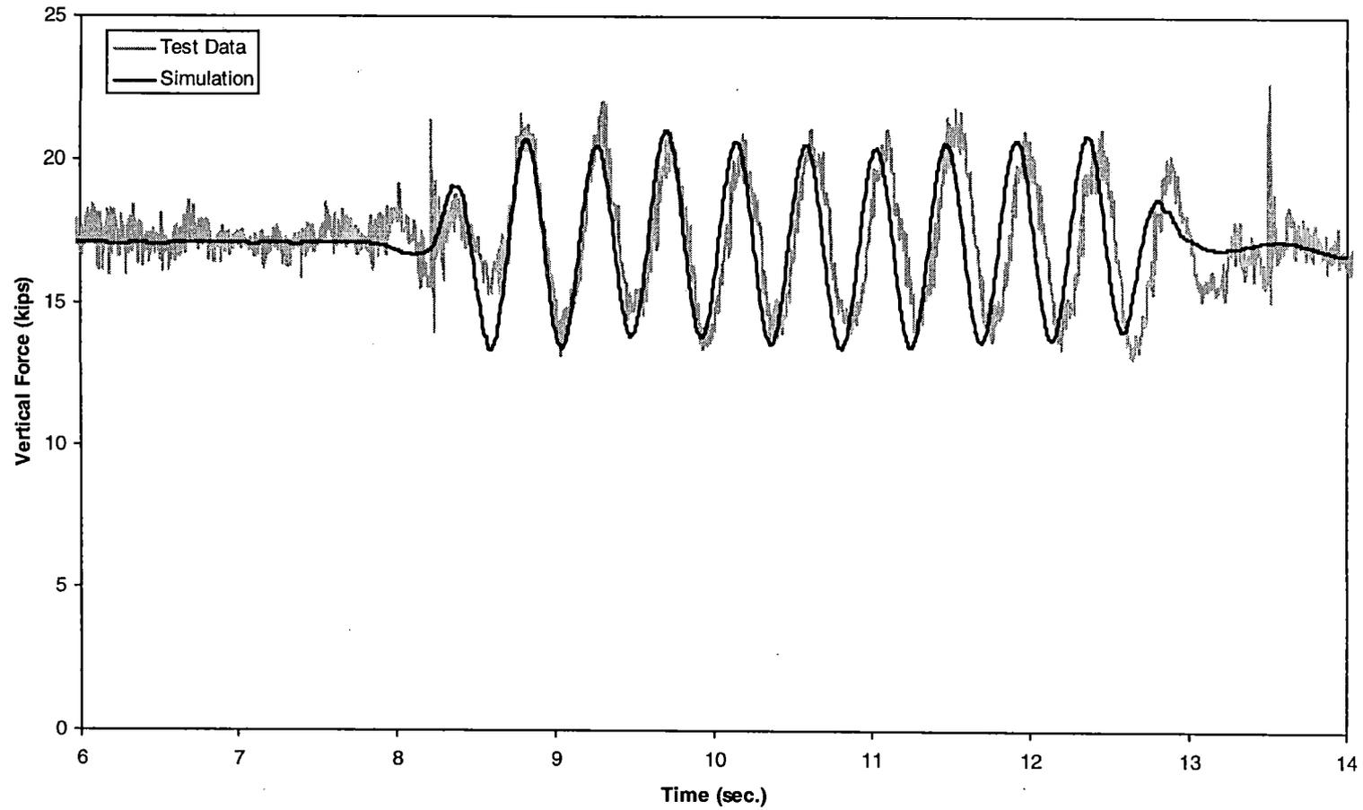
*Figure 5-34(b). Twist and roll – vertical force time history, 60 mph (lead right wheel)*
