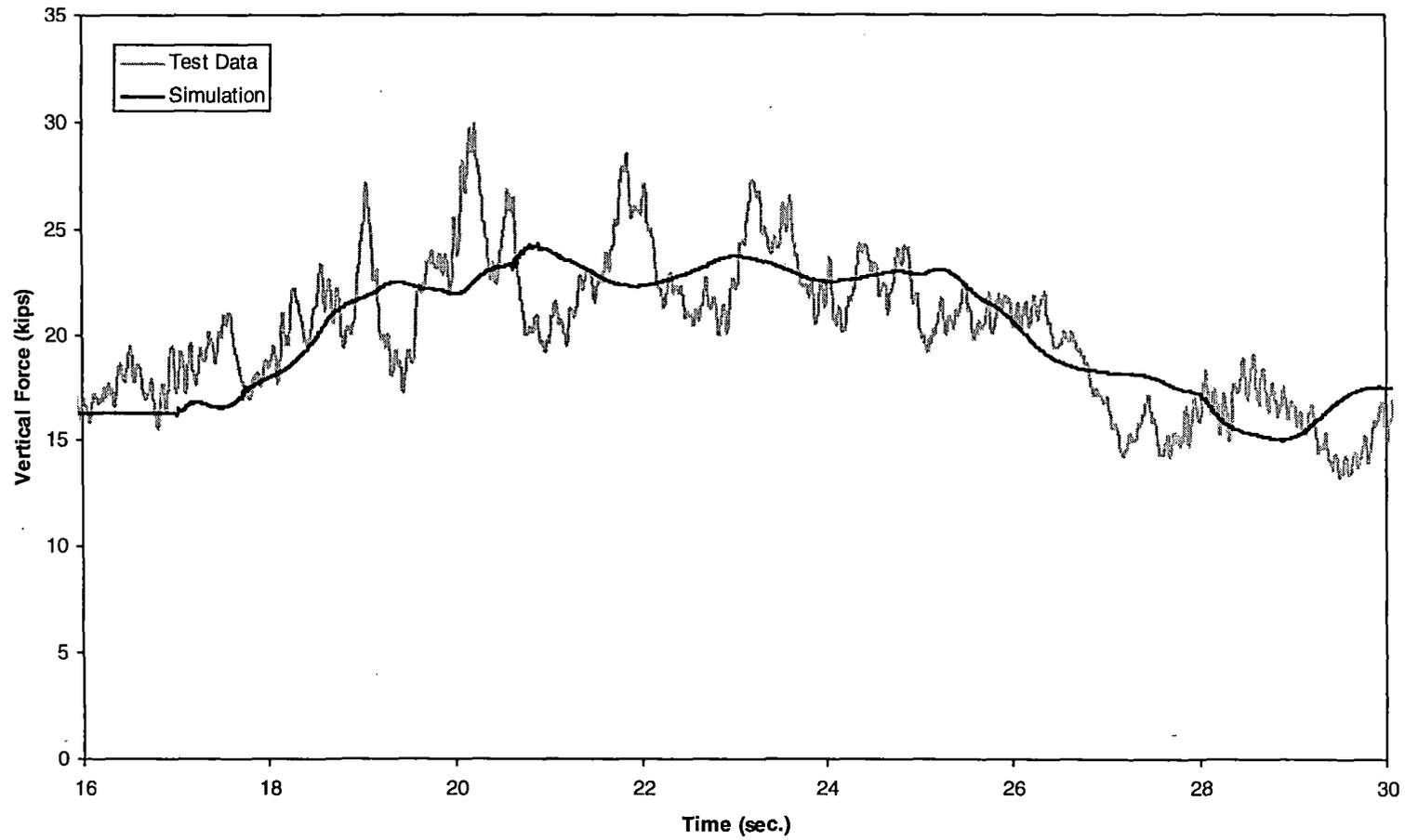
*Figure 5-11(c). Steady curving – vertical force time history, 124 mph (trailing outer wheel)*
