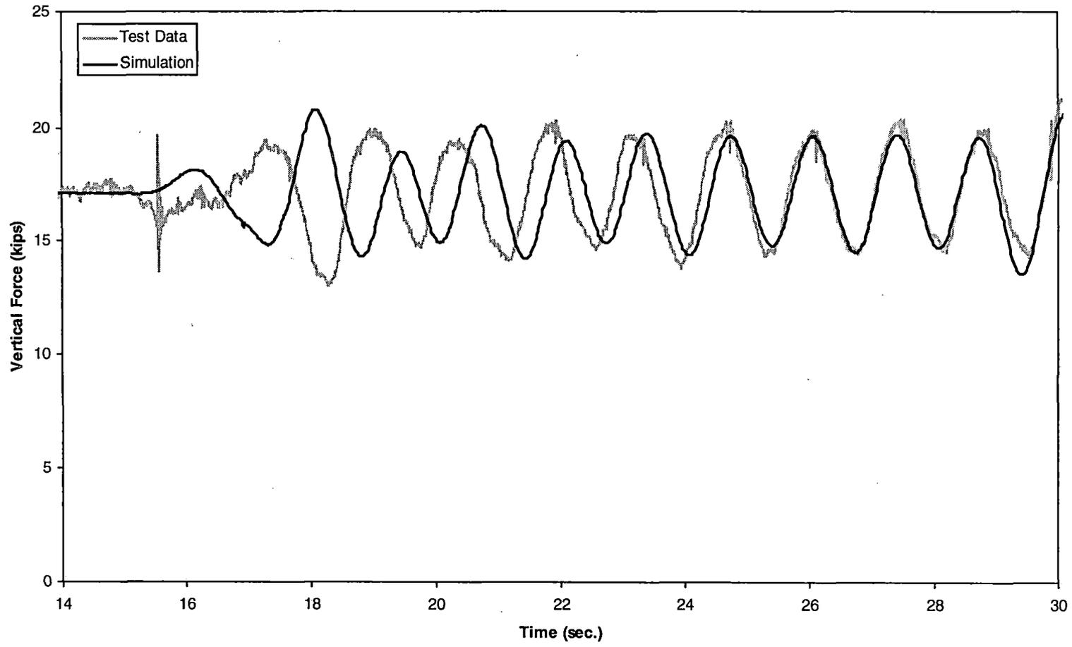
*Figure 5-32(a). Twist and roll – vertical force time history, 20 mph (lead left wheel)*
