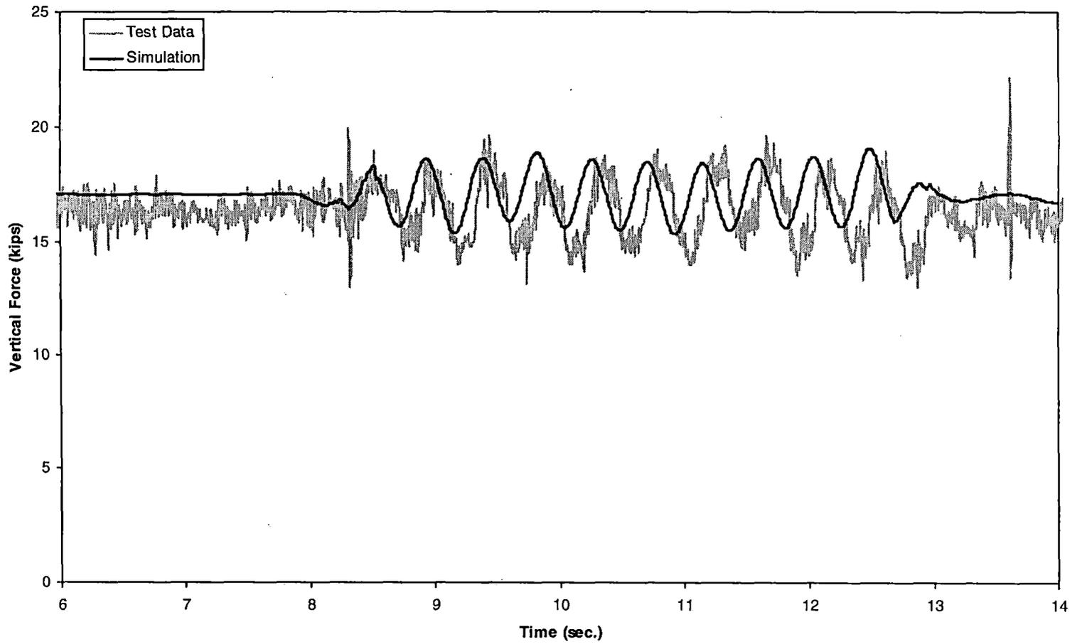
*Figure 5-34(d). Twist and roll – vertical force time history, 60 mph (trailing right wheel)*
