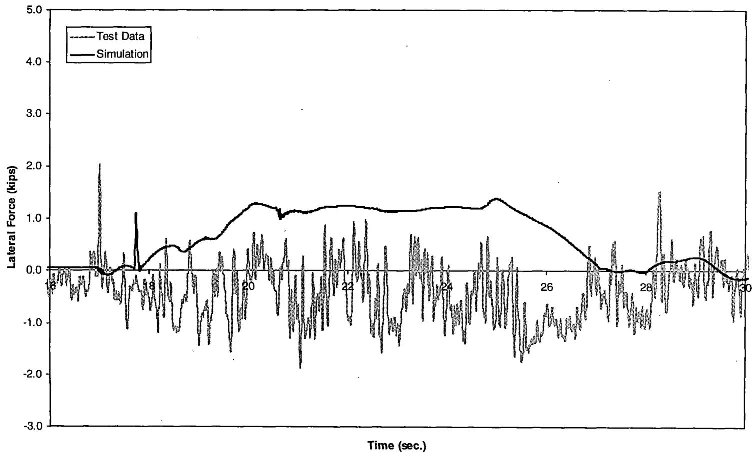
*Figure 5-12(b). Steady curving – lateral force time history, 124 mph (lead inner wheel)*
