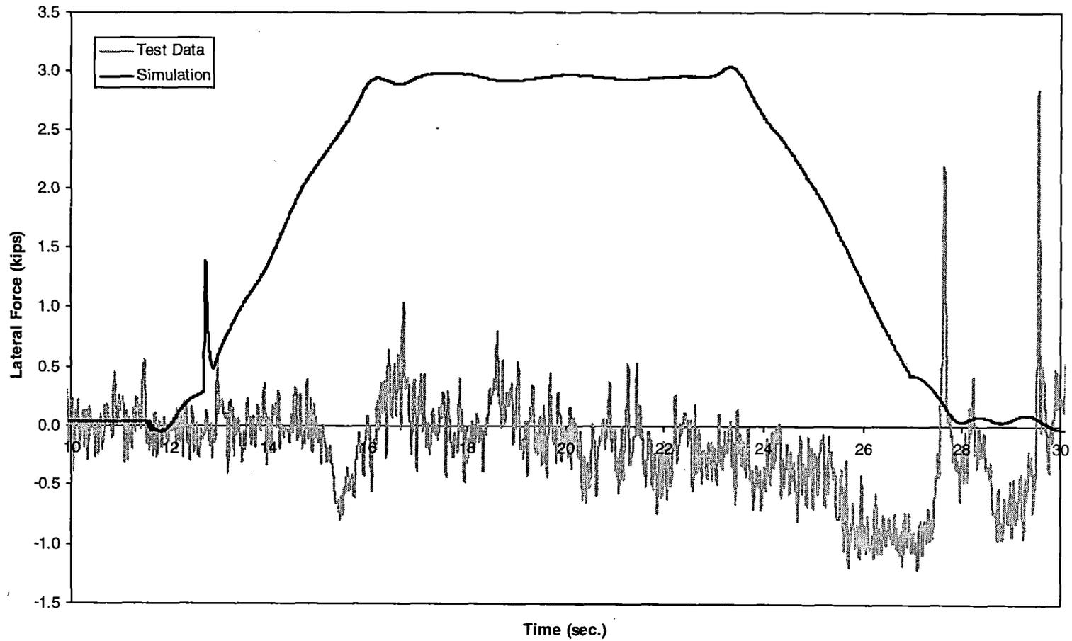
*Figure 5-9(b). Steady curving – lateral force time history, 84 mph (lead inner wheel)*
