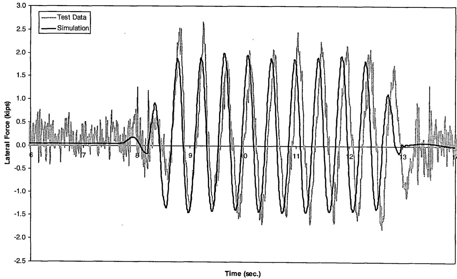
*Figure 5-35(b). Twist and roll – lateral force time history, 60 mph (lead right wheel)*
