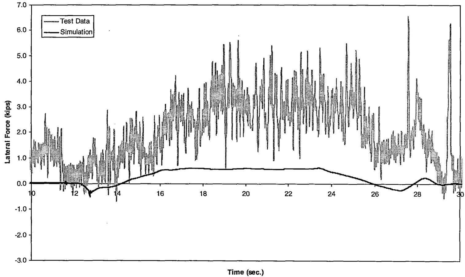
*Figure 5-9(d). Steady curving – lateral force time history, 84 mph (trailing inner wheel)*
