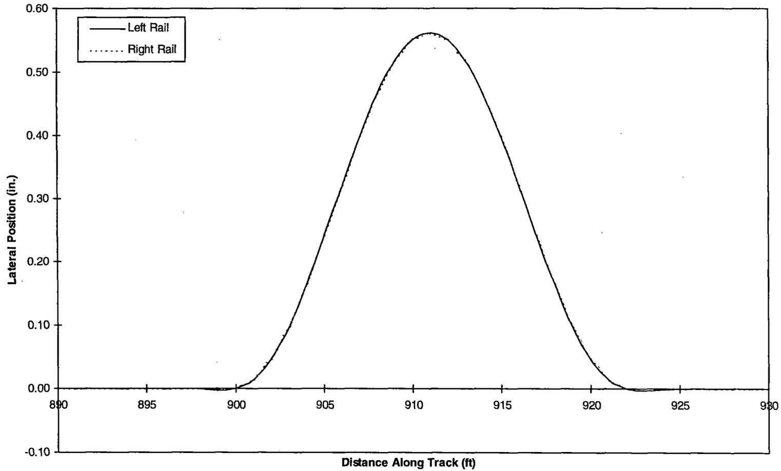
**Figure 5-43. Lateral perturbation for hunting test**
