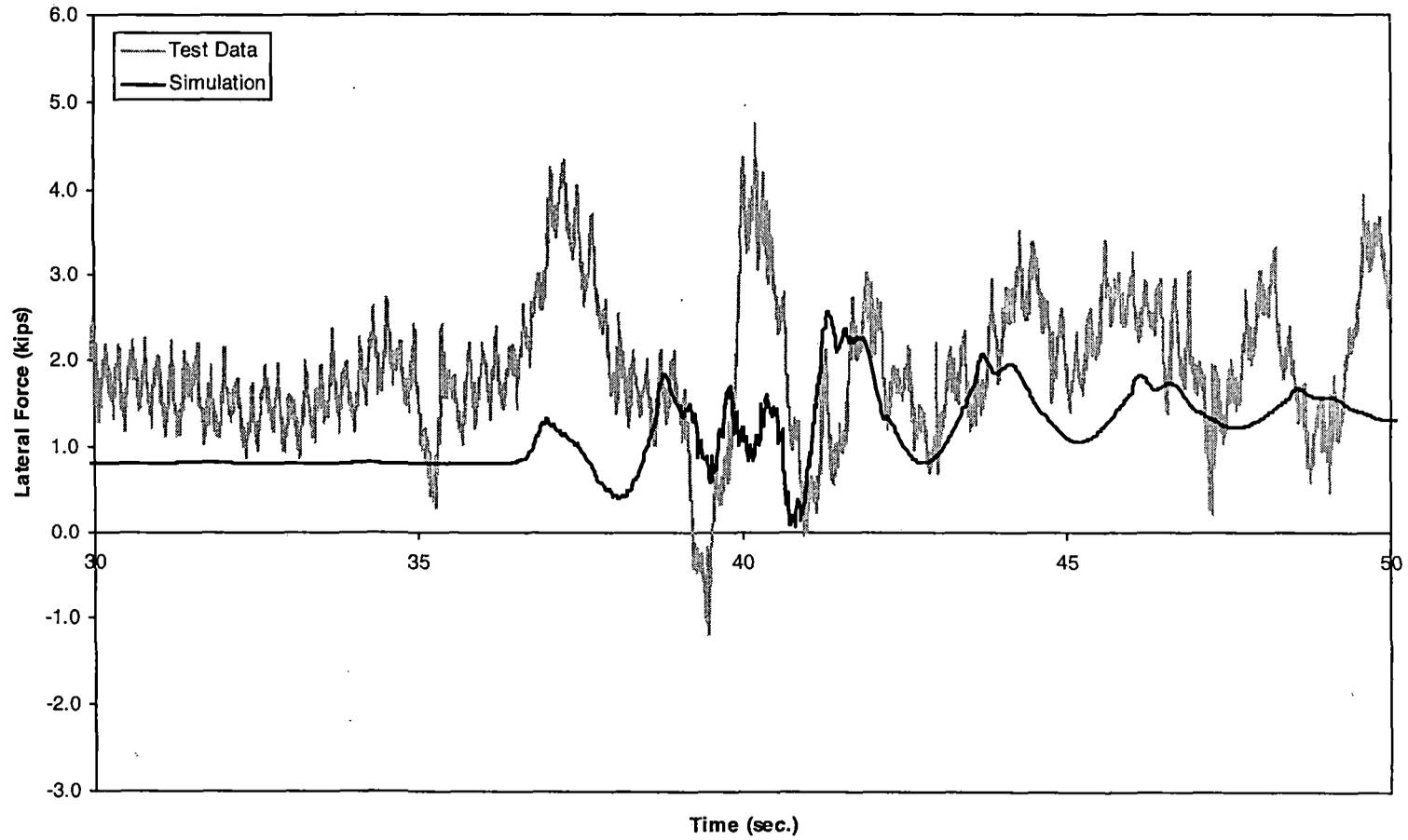
*Figure 5-6(d). Vertical dip test – lateral force time history, 15 mph (trailing inner wheel)*
