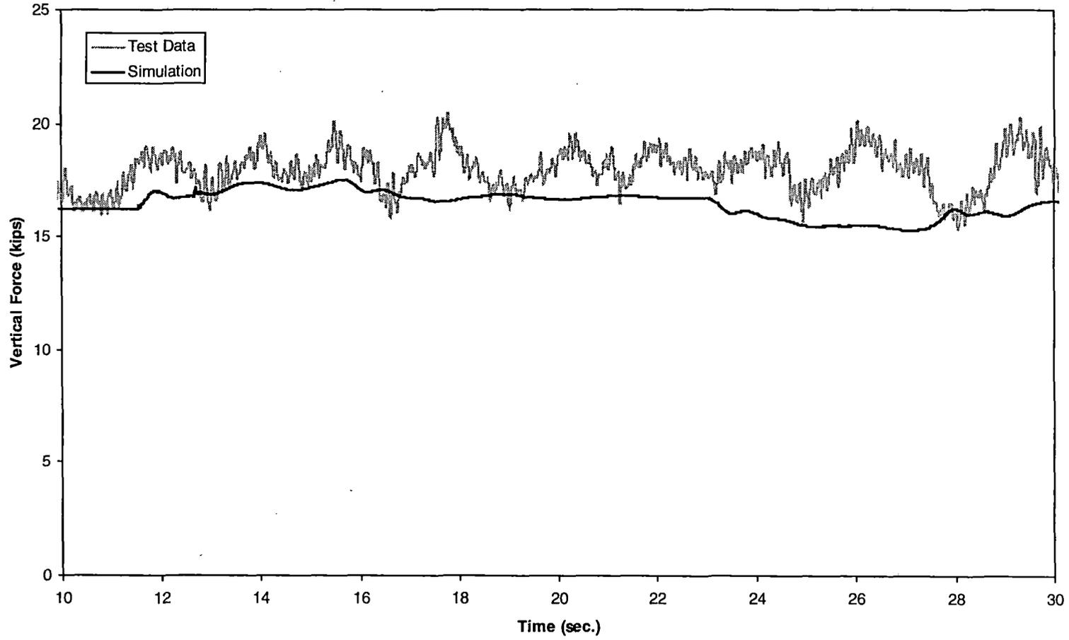
*Figure 5-8(a). Steady curving – vertical force time history, 84 mph (lead outer wheel)*
