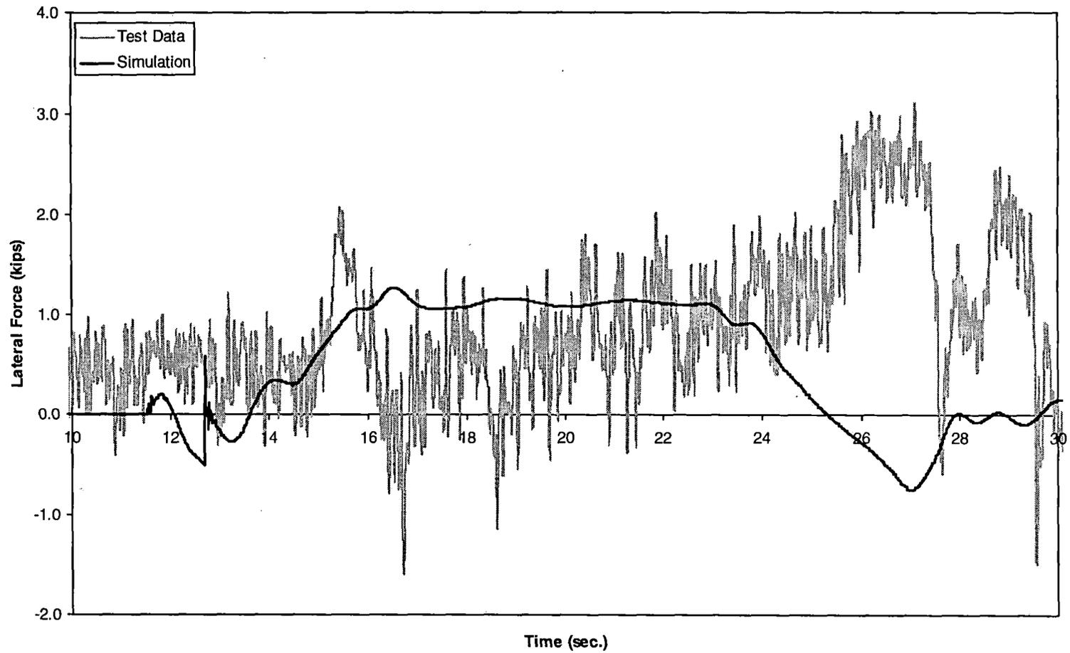
*Figure 5-10(a). Steady curving – net axle lateral force time history, 84 mph (lead axle)*
