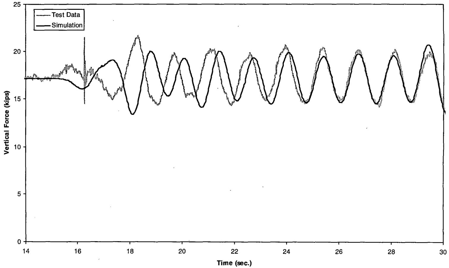
*Figure 5-32(b). Twist and roll – vertical force time history, 20 mph (lead right wheel)*
