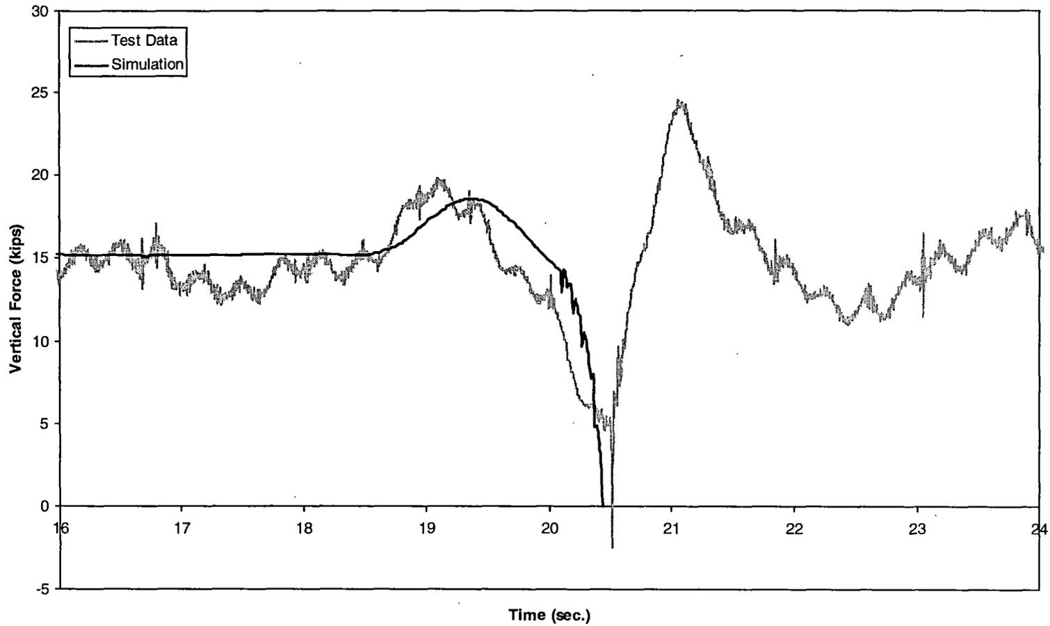
*Figure 5-3(a). Vertical dip test – vertical force time history, 20 mph (lead outer wheel)*
