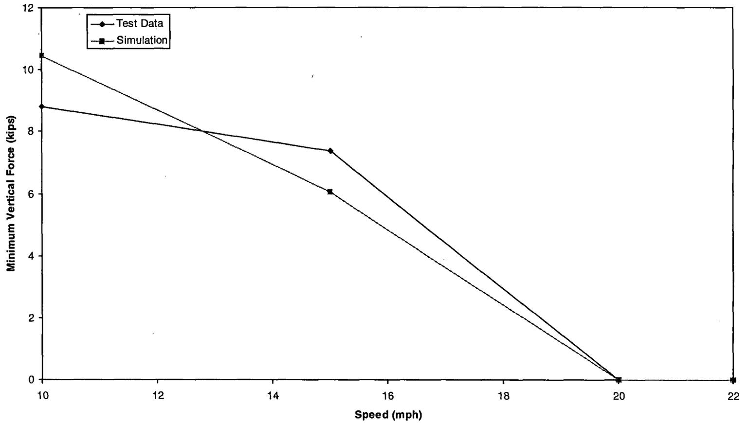
Figure 5-7. Vertical dip test – minimum vertical force
