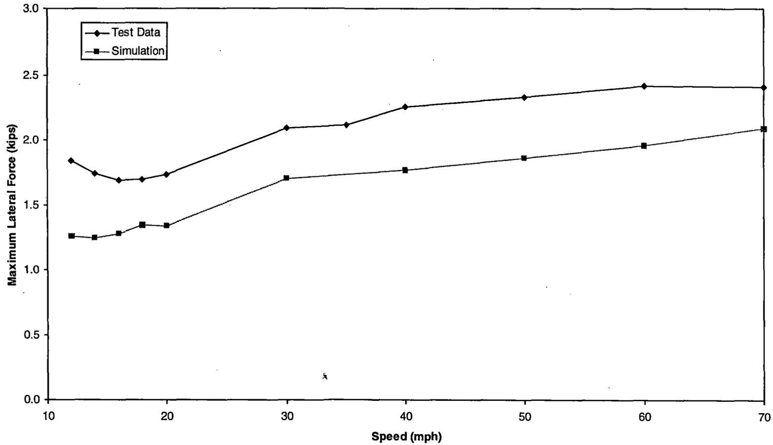
*Figure 5-37. Twist and roll – maximum lateral force*
