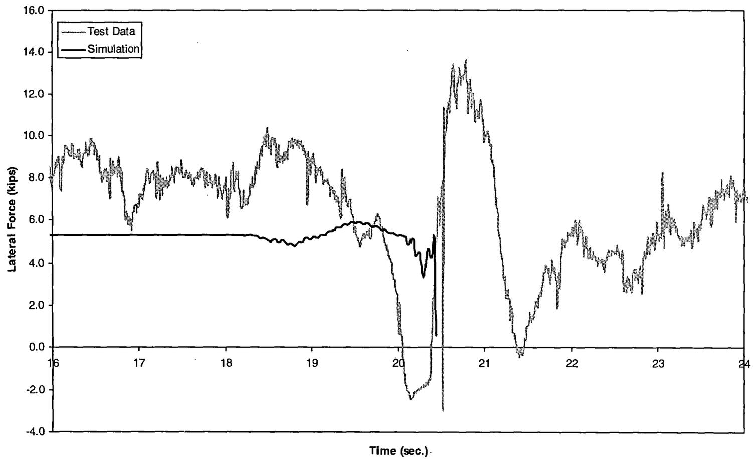
*Figure 5-4(a). Vertical dip test – lateral force time history, 20 mph (lead outer wheel)*
