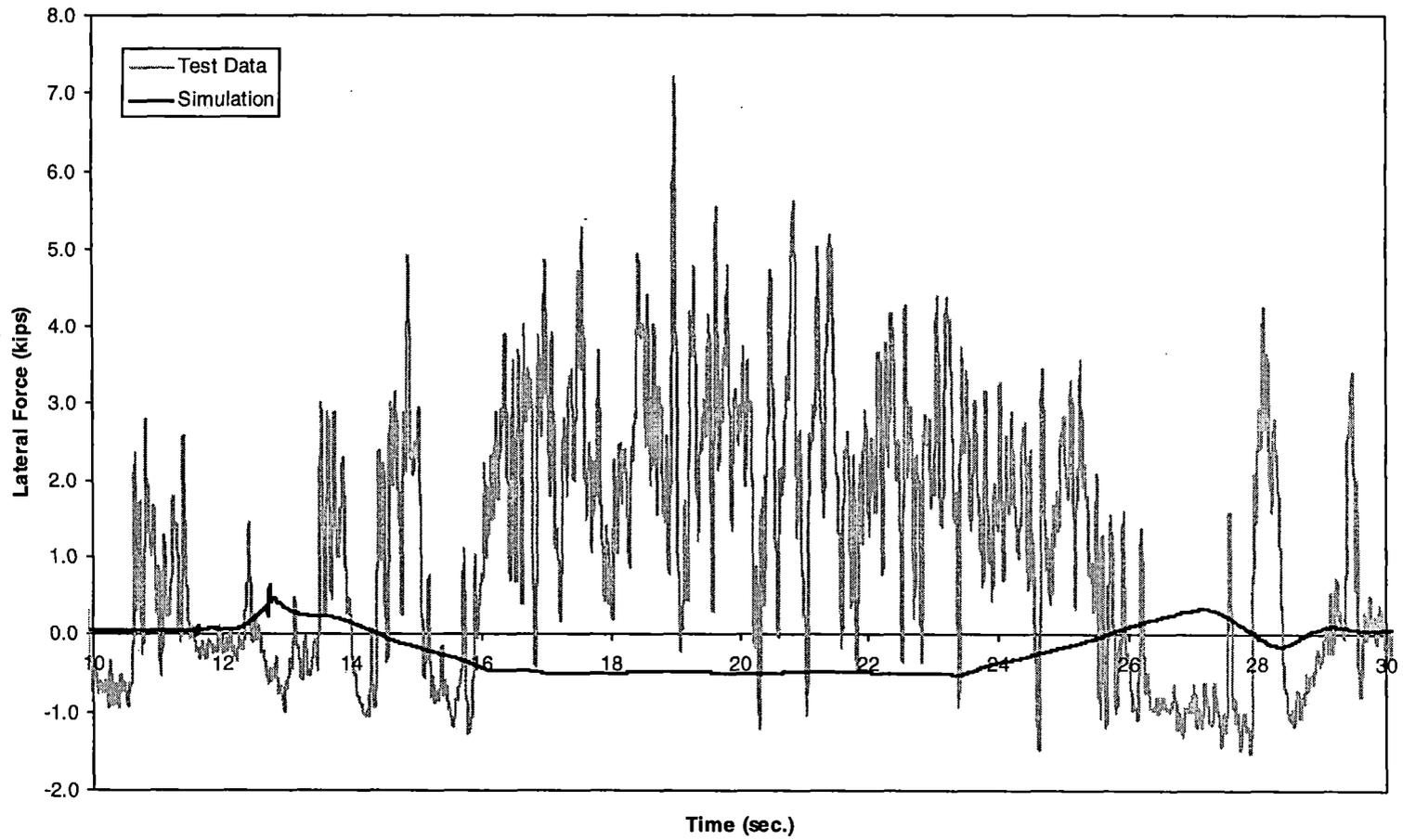
*Figure 5-9(c). Steady curving – lateral force time history, 84 mph (trailing outer wheel)*
