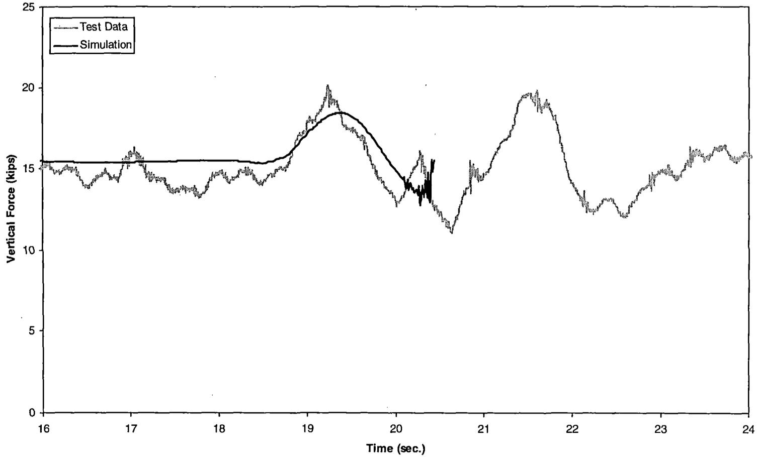
Figure 5-3(c). Vertical dip test – vertical force time history, 20 mph (trailing outer wheel)
