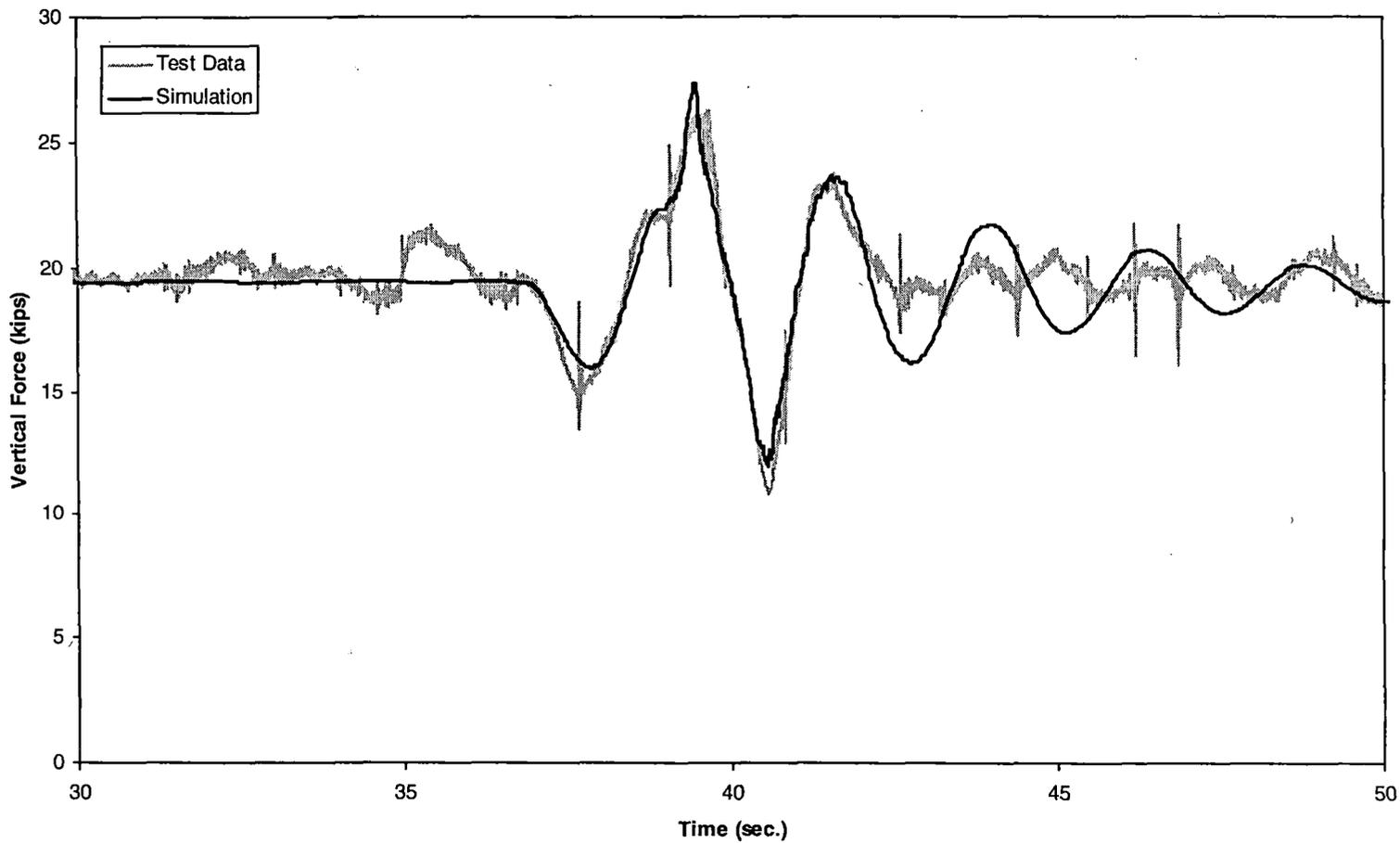
*Figure 5-5(b). Vertical dip test – vertical force time history, 15 mph (lead inner wheel)*
