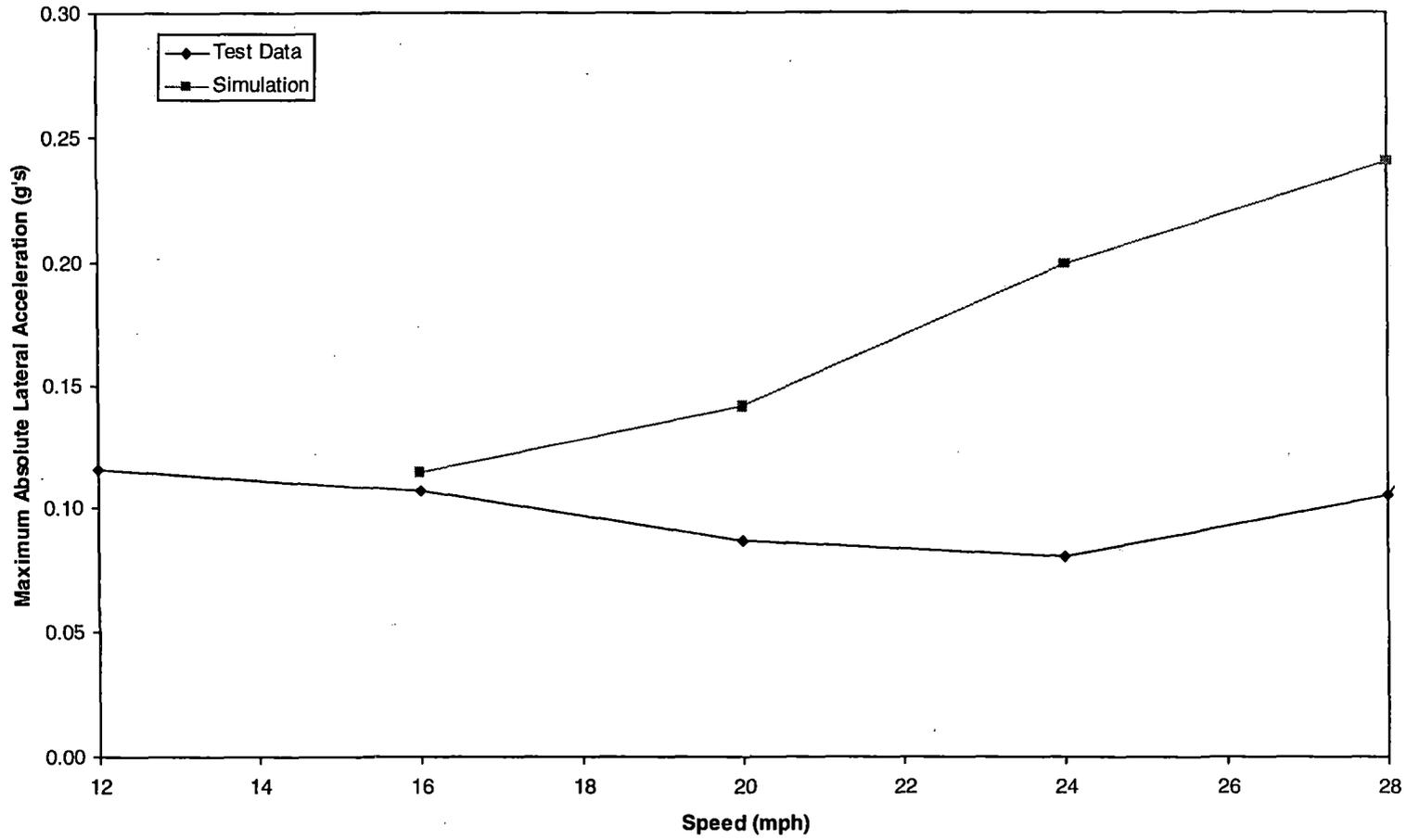
*Figure 5-22. Dynamic curving – maximum absolute lateral carbody acceleration*
