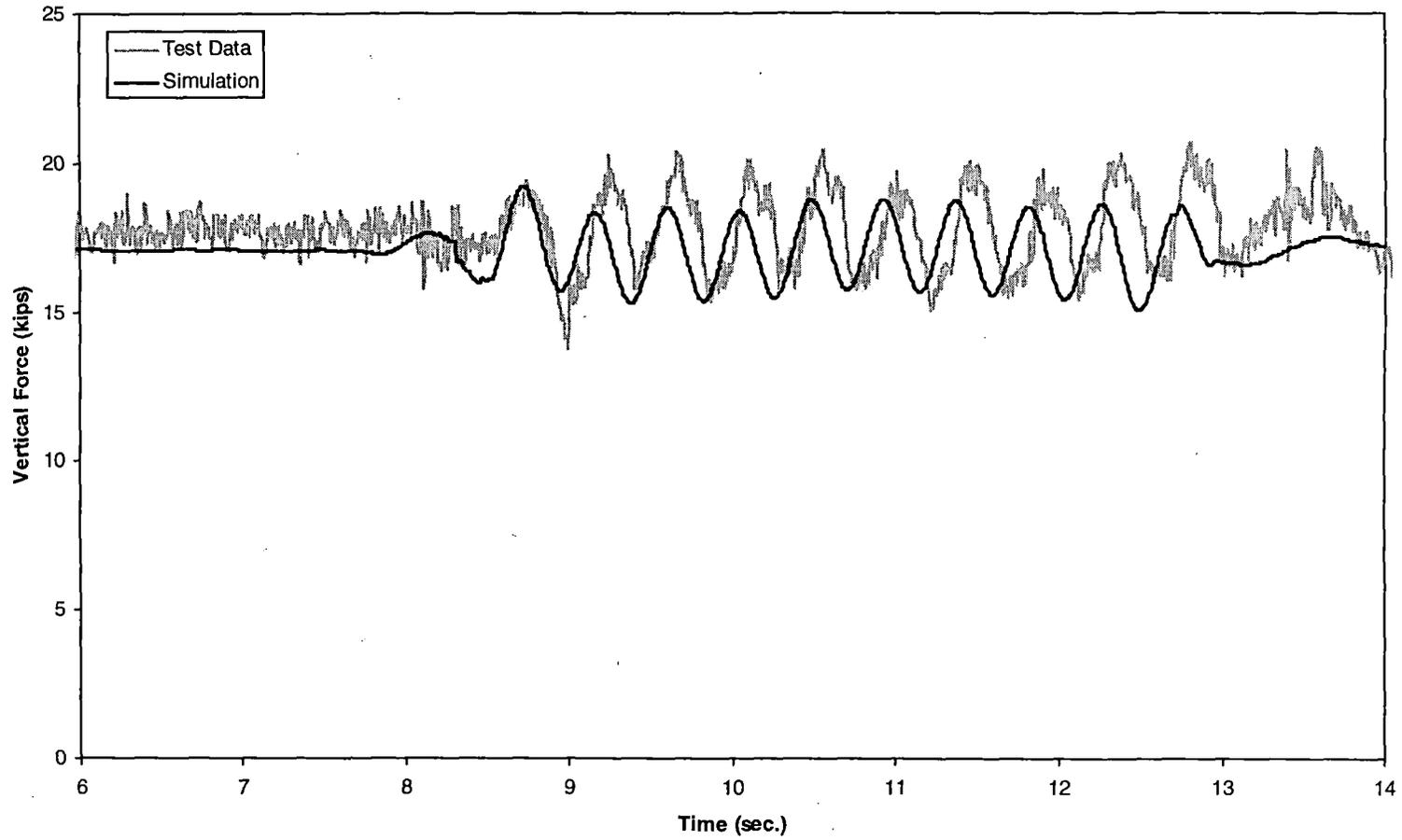
*Figure 5-34(c). Twist and roll – vertical force time history, 60 mph (trailing left wheel)*
