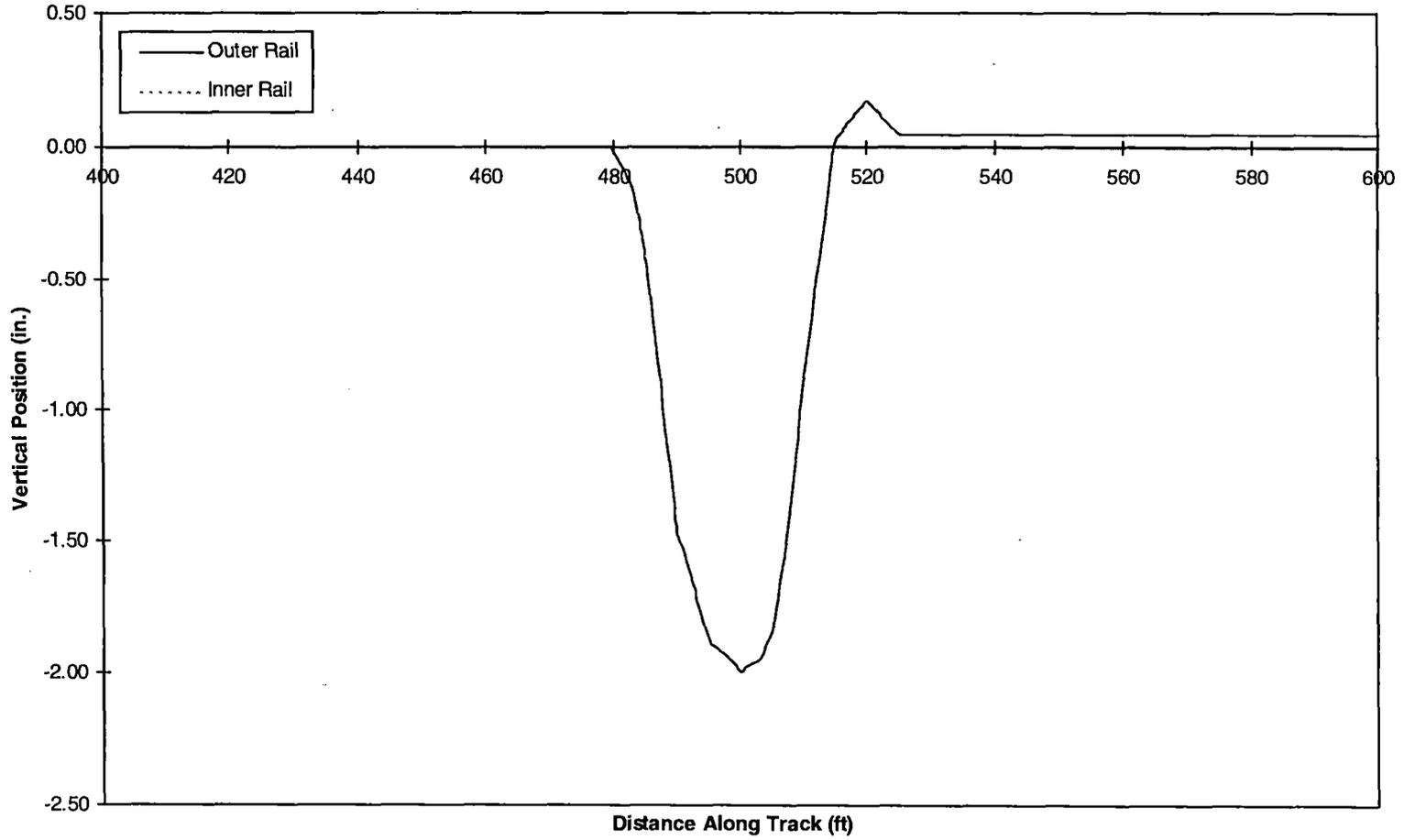
*Figure 5-2. Vertical dip in the 5 deg curve*
