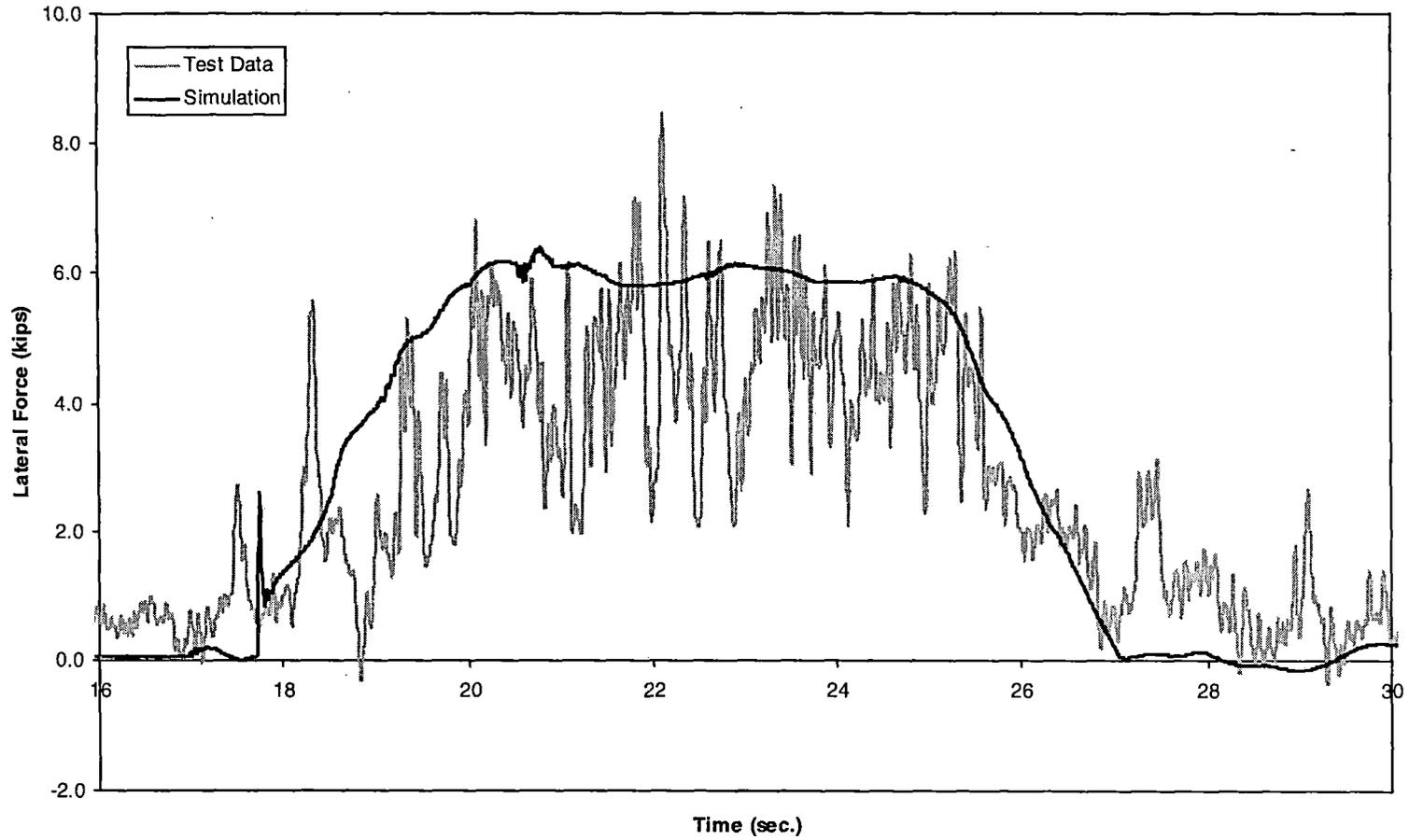
*Figure 5-12(a). Steady curving – lateral force time history, 124 mph (lead outer wheel)*
