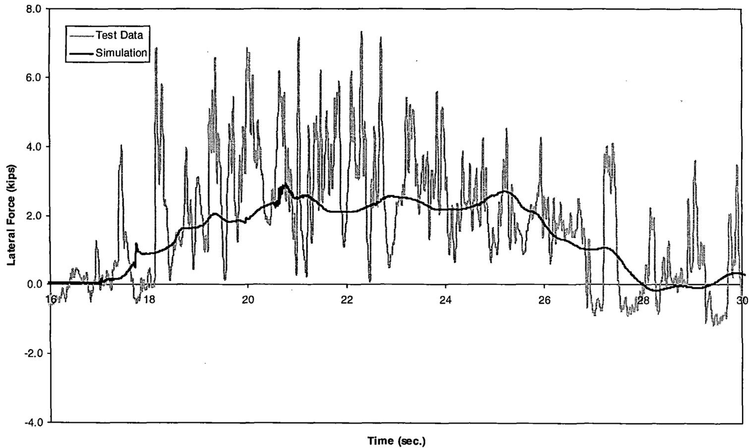
*Figure 5-12(c). Steady curving – lateral force time history, 124 mph (trailing outer wheel)*
