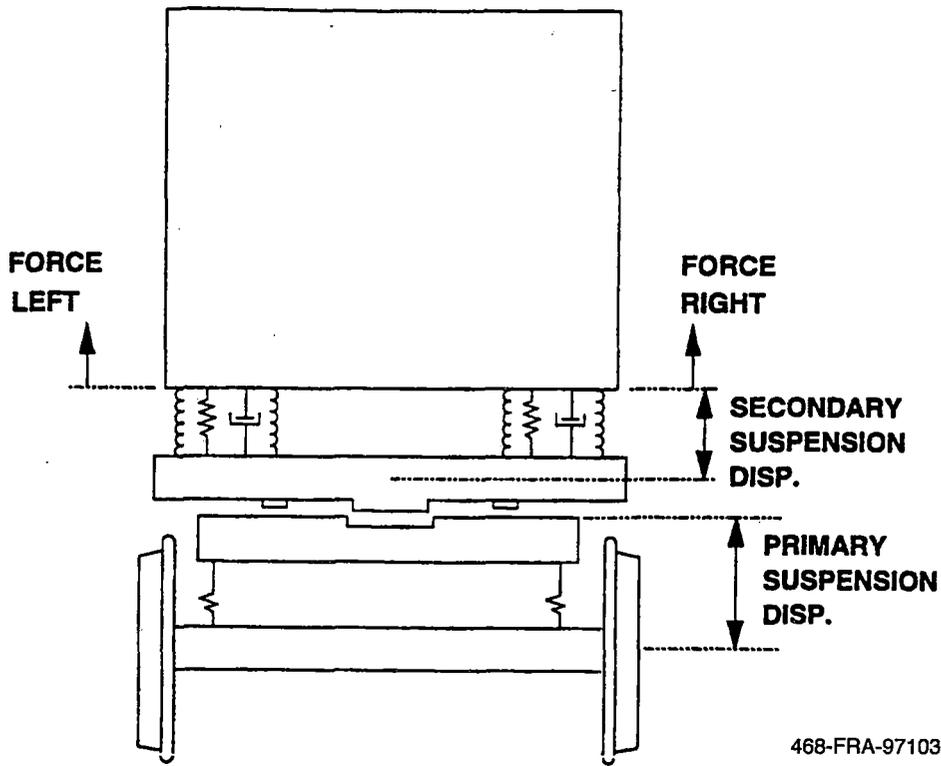
*Figure 4-1. Vertical suspension characterization test setup*
