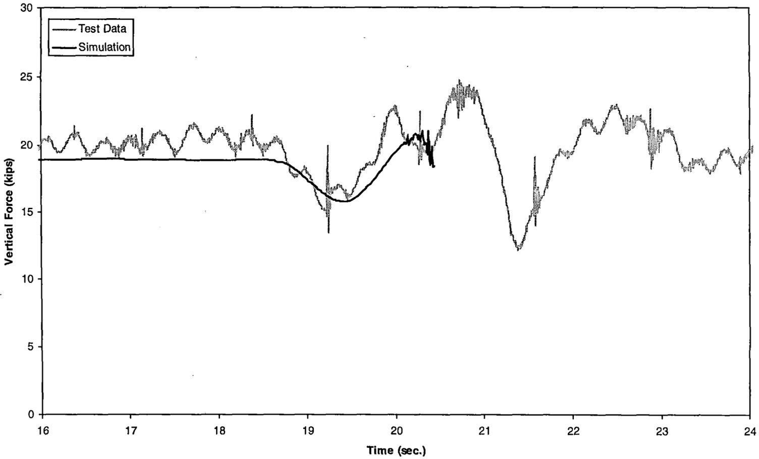
*Figure 5-3(d). Vertical dip test – vertical force time history, 20 mph (trailing inner wheel)*
