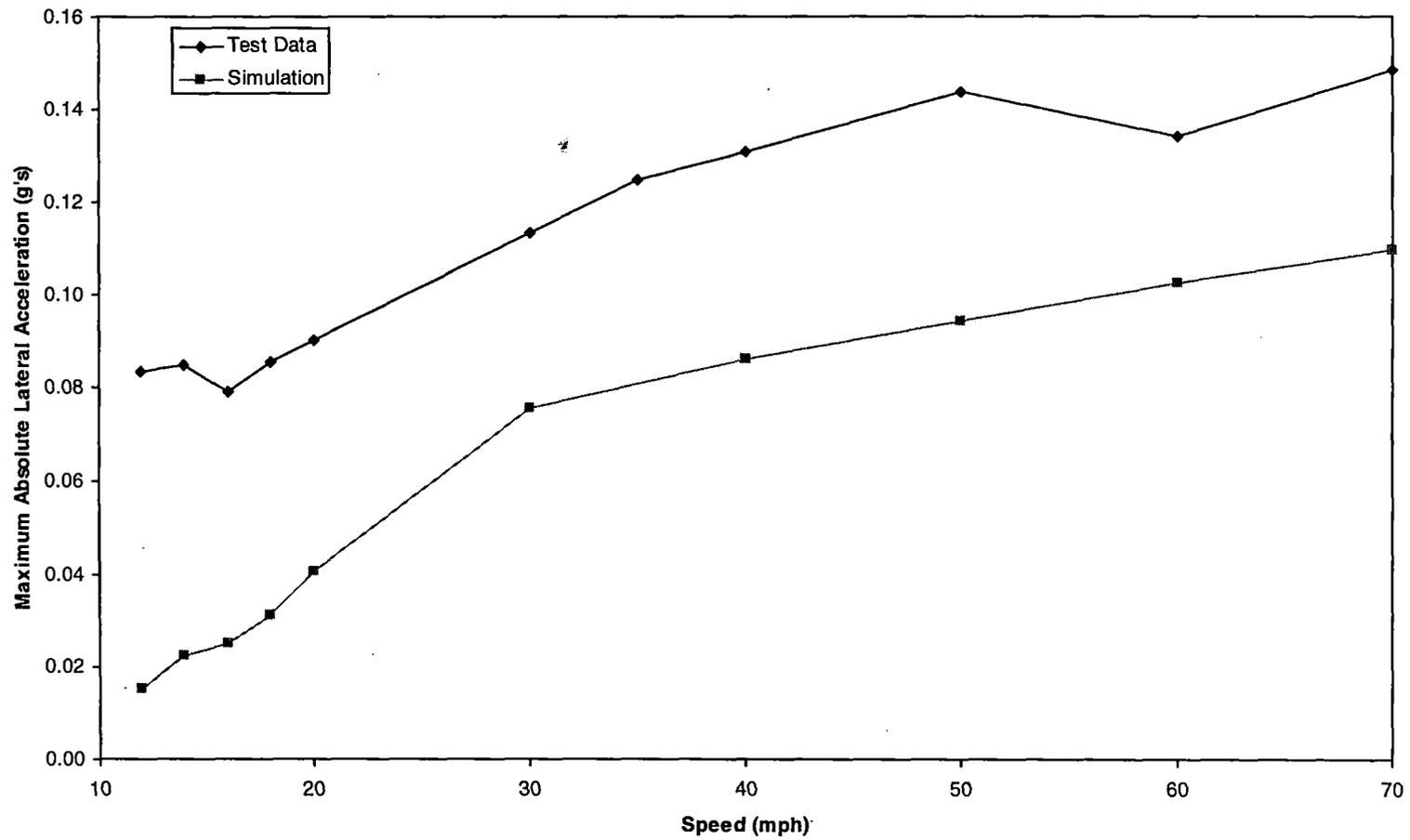
*Figure 5-38. Twist and roll – maximum absolute lateral carbody acceleration*
