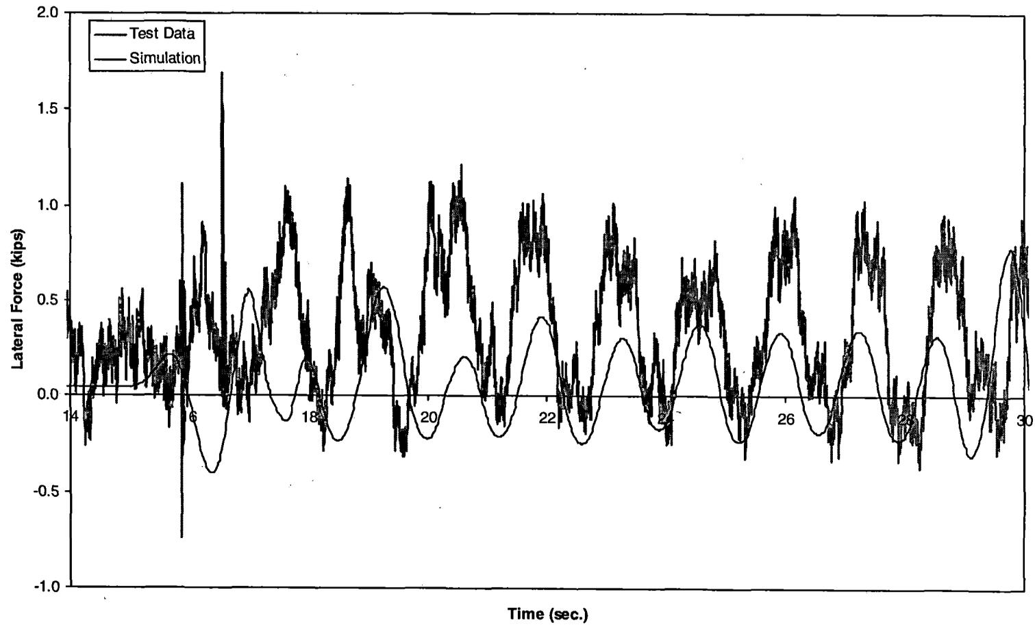
*Figure 5-33(d). Twist and roll – lateral force time history, 20 mph (trailing right wheel)*
