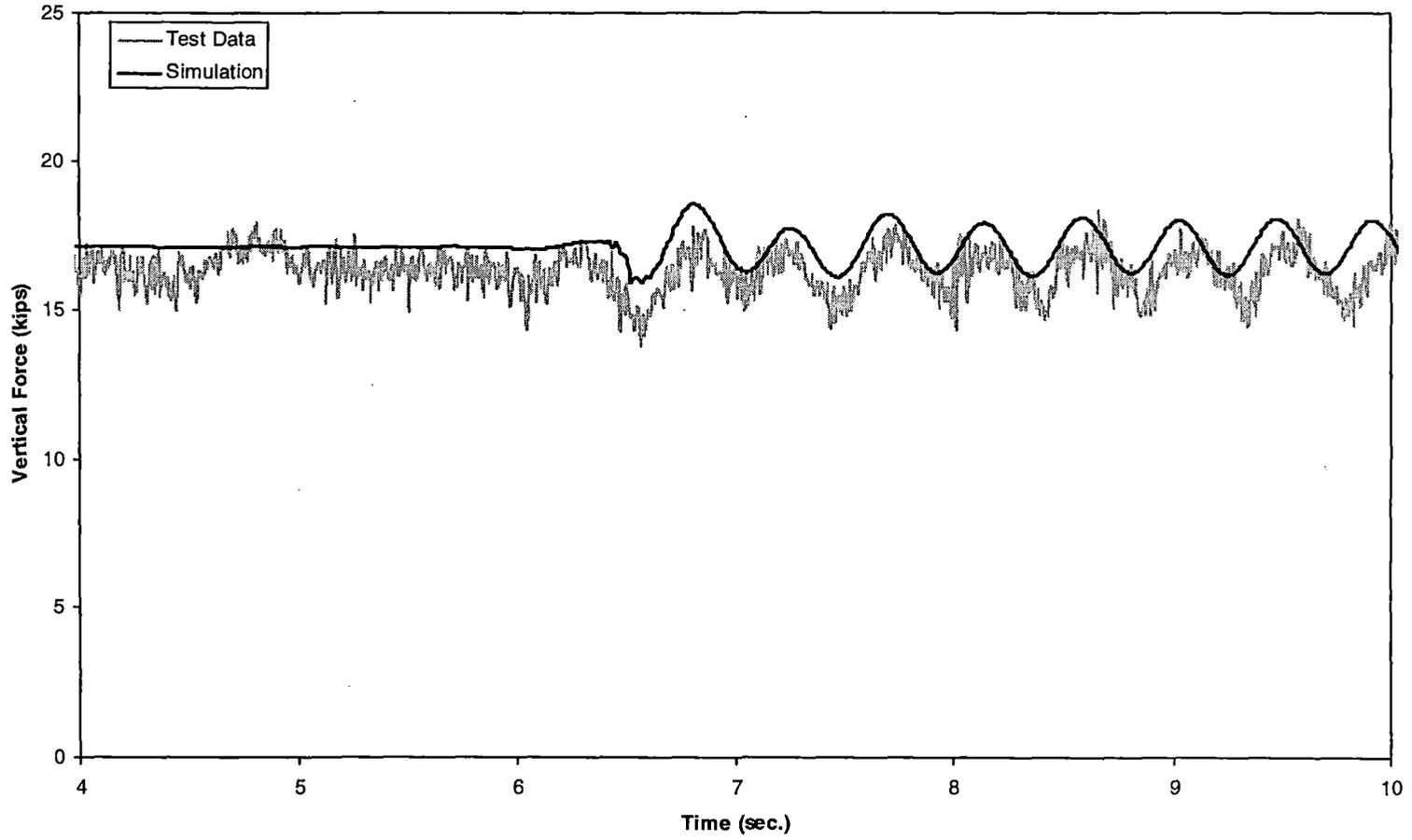
*Figure 5-41(d). Pitch and bounce – vertical force time history, 60 mph (trailing right wheel)*
