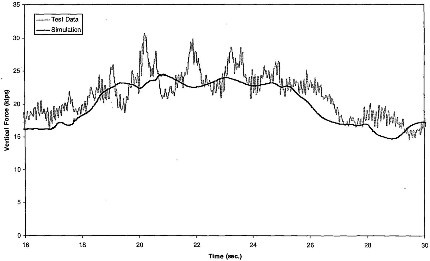
*Figure 5-11(a). Steady curving – vertical force time history, 124 mph (lead outer wheel)*
