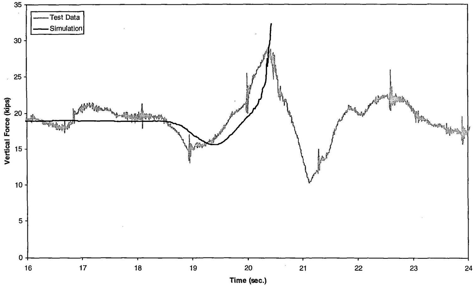
*Figure 5-3(b). Vertical dip test – vertical force time history, 20 mph (lead inner wheel)*
