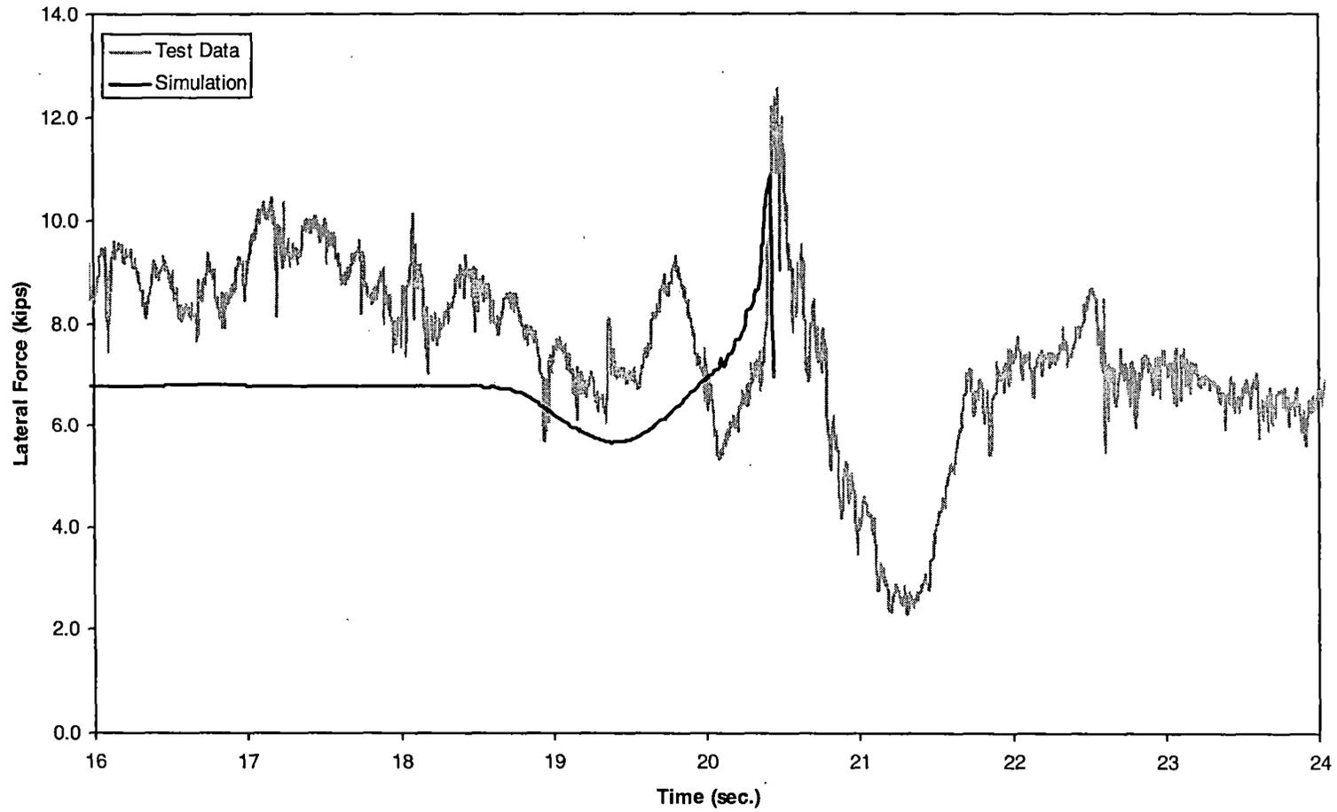
*Figure 5-4(b). Vertical dip test – lateral force time history, 20 mph (lead inner wheel)*
