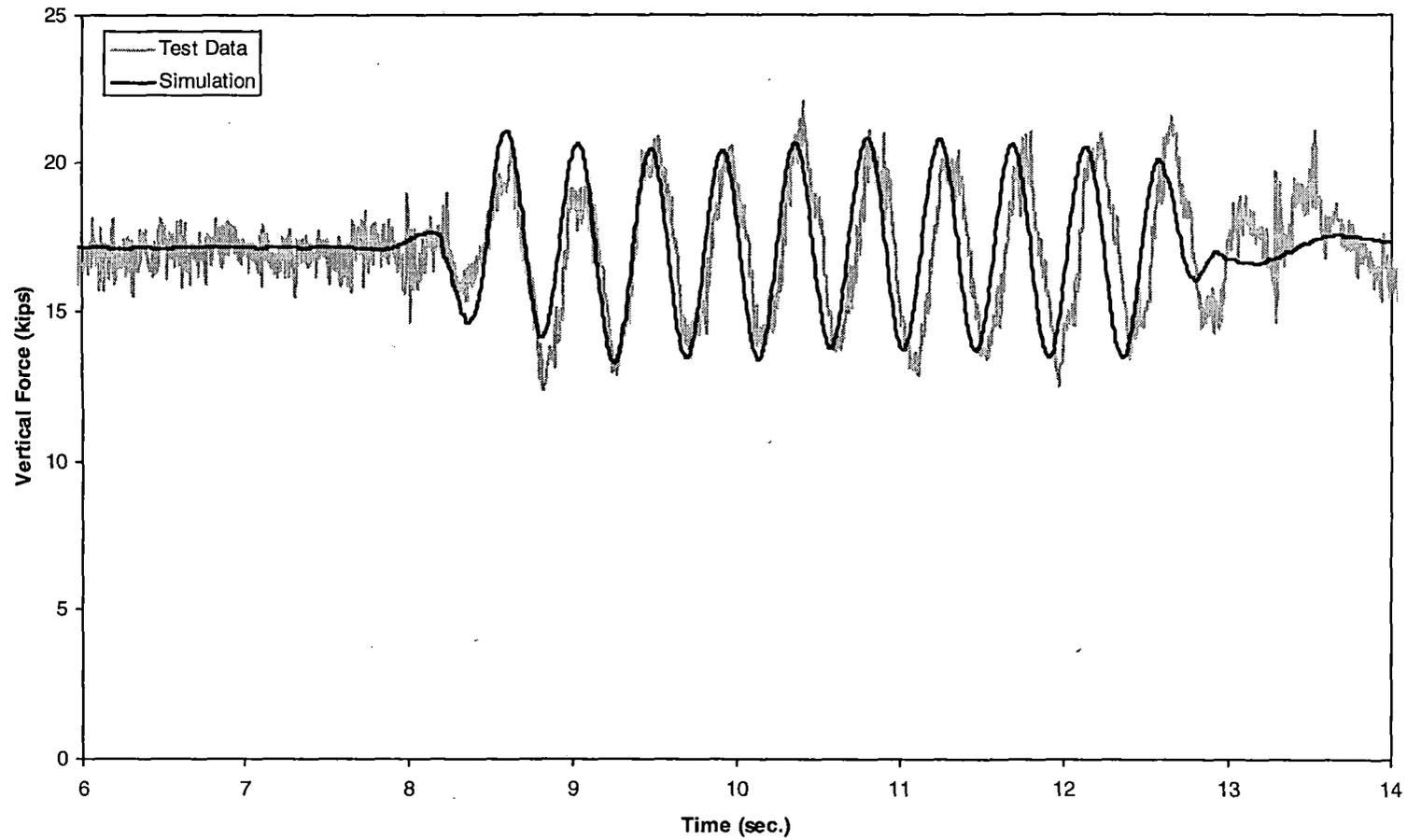
*Figure 5-34(a). Twist and roll – vertical force time history, 60 mph (lead left wheel)*
