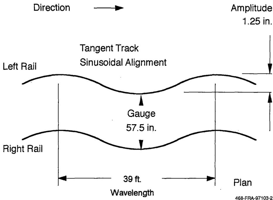
**Figure 5-23. Track alignment variation for yaw and sway**
