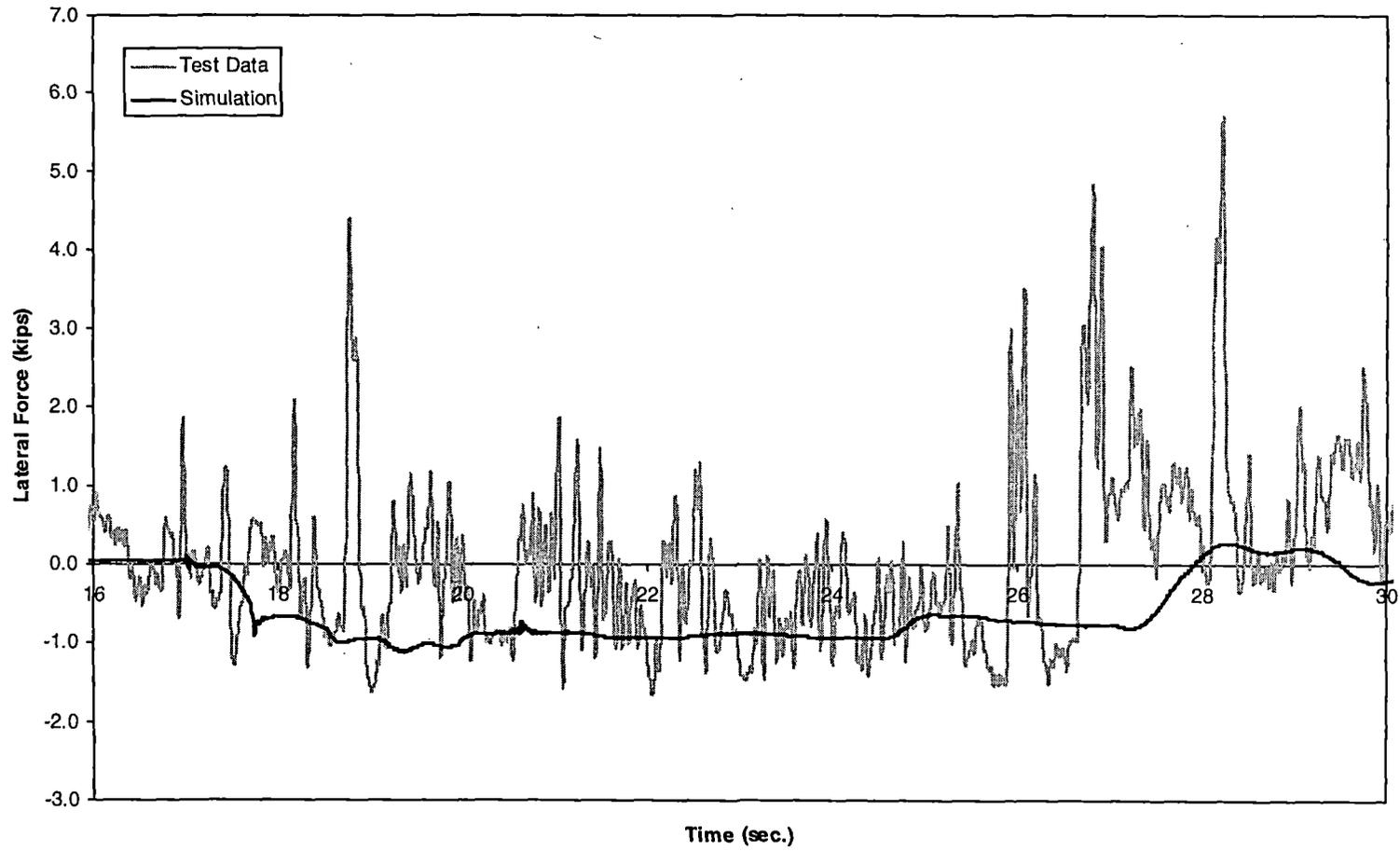
Figure 5-12(d). Steady curving – lateral force time history, 124 mph (trailing inner wheel)
