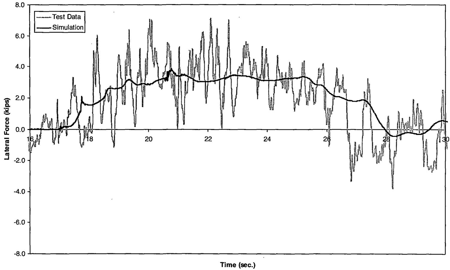
*Figure 5-13(b). Steady curving – net axle lateral force time history, 124 mph (trailing axle)*
