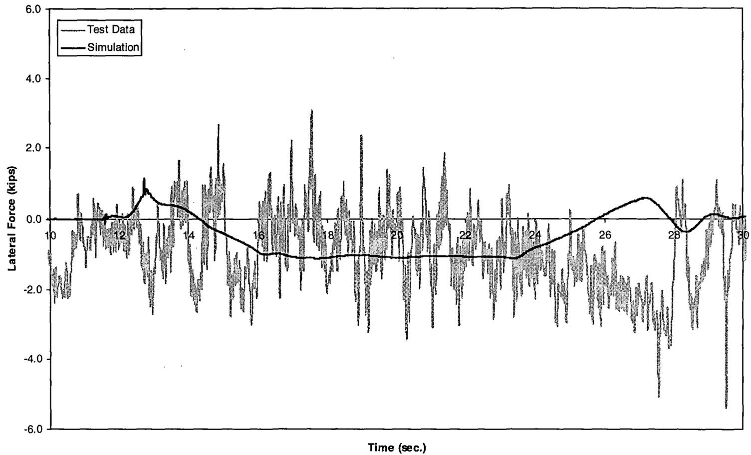
*Figure 5-10(b). Steady curving – net axle lateral force time history, 84 mph (trailing axle)*
