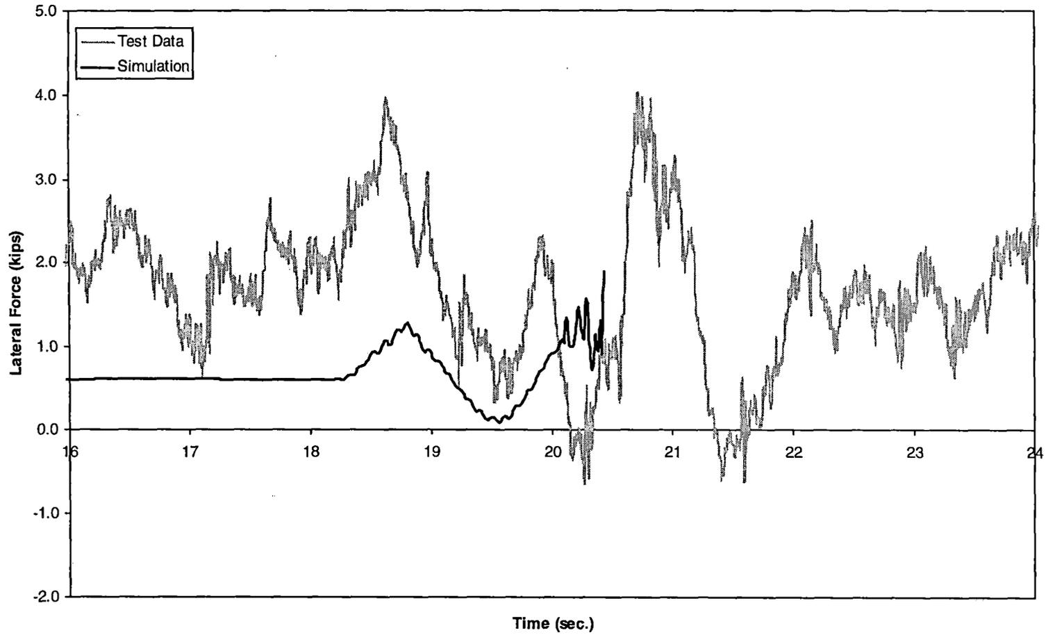
*Figure 5-4(d). Vertical dip test – lateral force time history, 20 mph (trailing inner wheel)*
