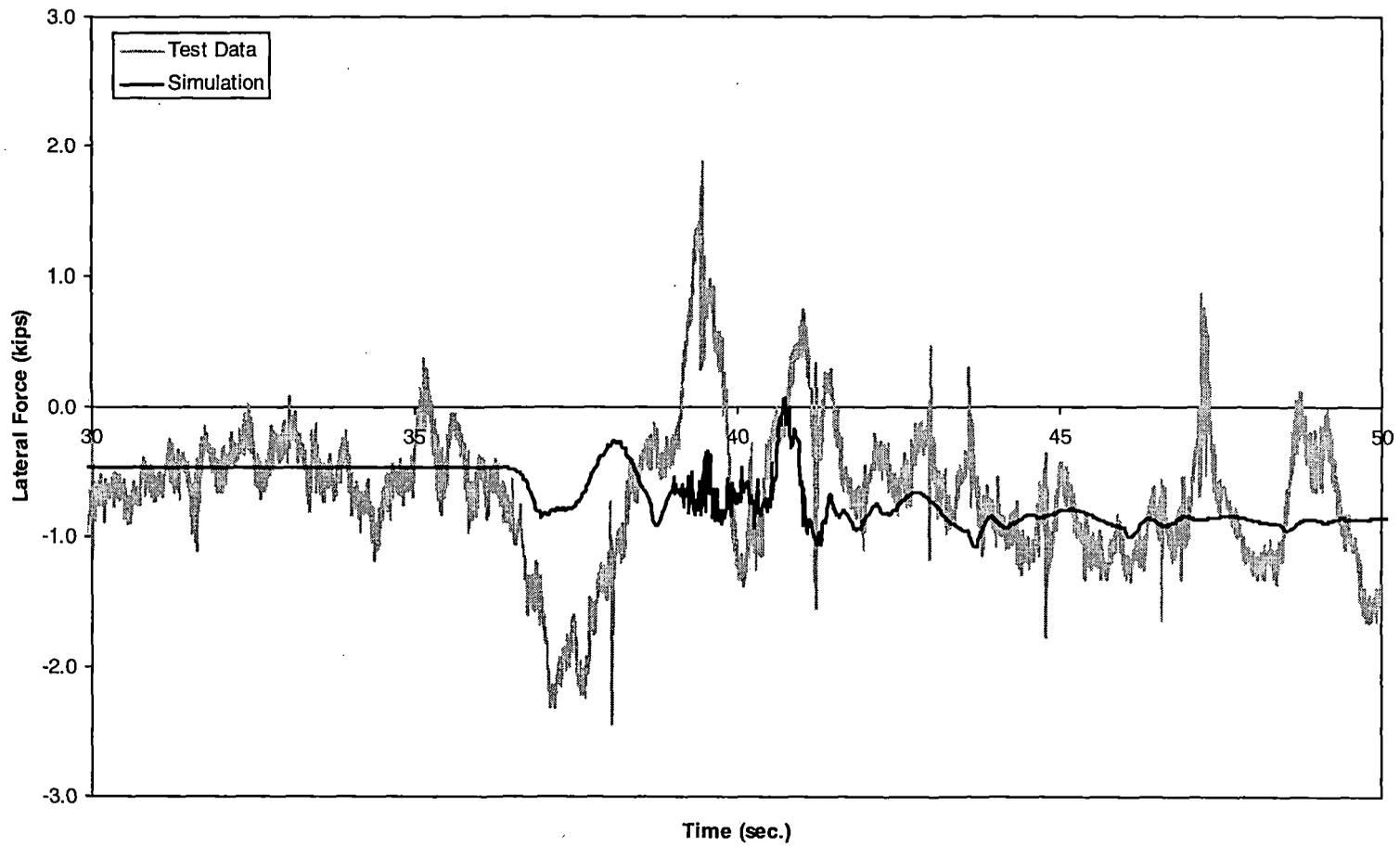
*Figure 5-6(c). Vertical dip test – lateral force time history, 15 mph (trailing outer wheel)*
