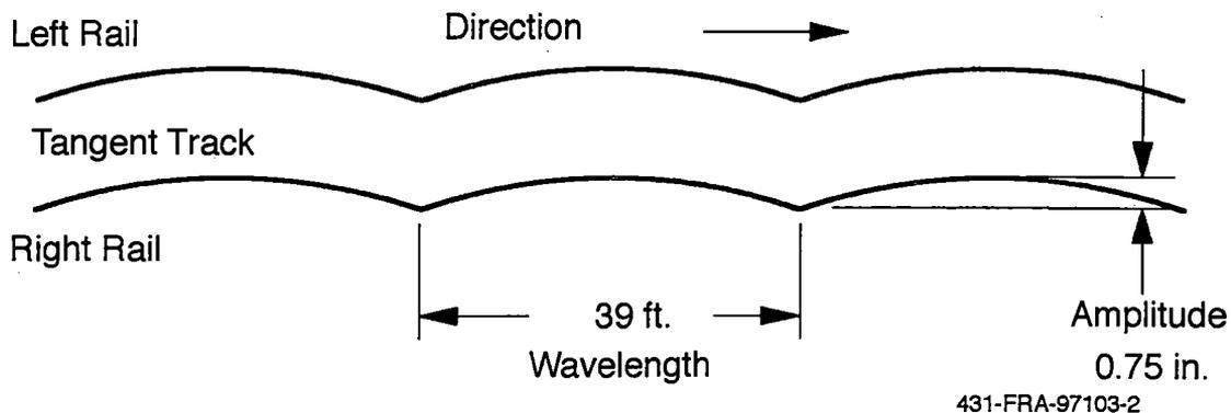
**Figure 5-39. Track surface variation for pitch and bounce**
