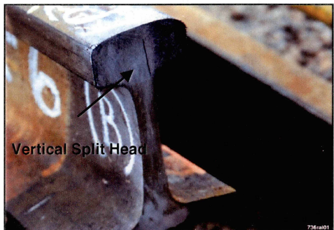
Figure B4. Vertical Split Head in Rail Donated to TTCI for Inclusion into the RDTF
