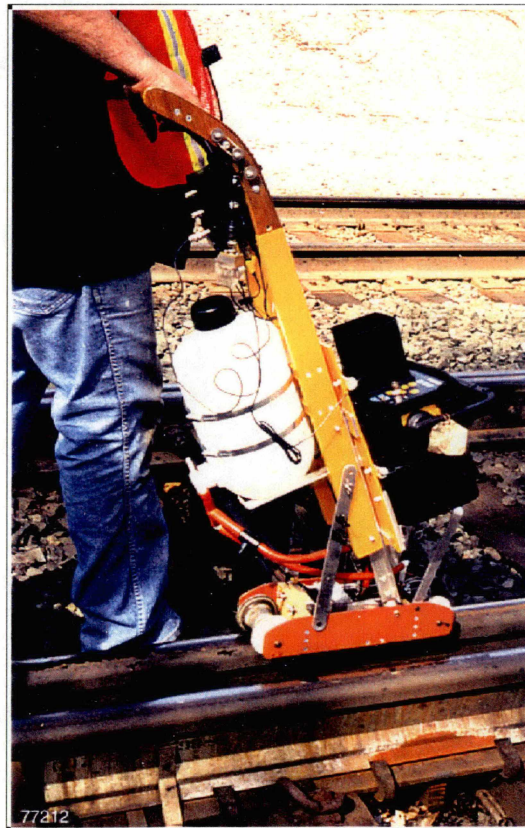
Figure C9. Hand Operated Single Rail Testing Device Used for Portable Rail Flaw Detection
