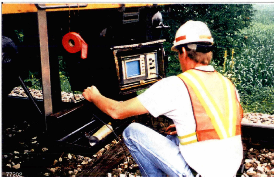
Figure C7. Ultrasonic Calibration Prior to Hand Mapping of a Rail
