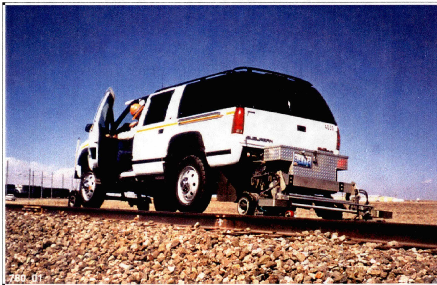
Figure C5. Hi-Rail Ultrasonic Inspection Vehicle Using a Transducer Array Set on a Sled System
