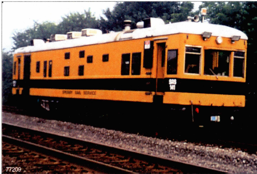
Figure C1. Rail Bound Induction/Ultrasonic Detector Car used for Rail Flaw Detection
