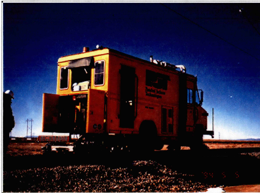
Figure C3. Hi-rail Ultrasonic Inspection Vehicle Using Roller Search Units for Rail Flaw Inspection
