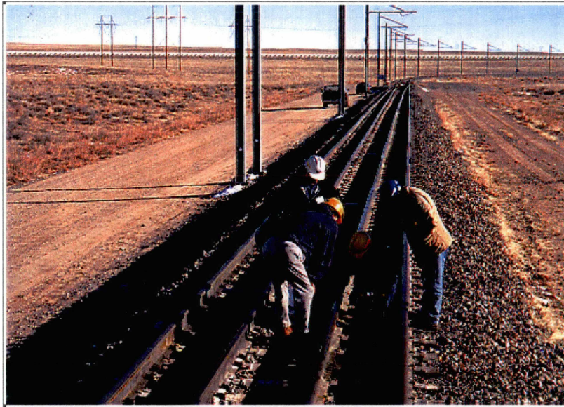
Figure 3. Flaw Verification Using Ultrasonic Hand Mapping with Participants Observing
