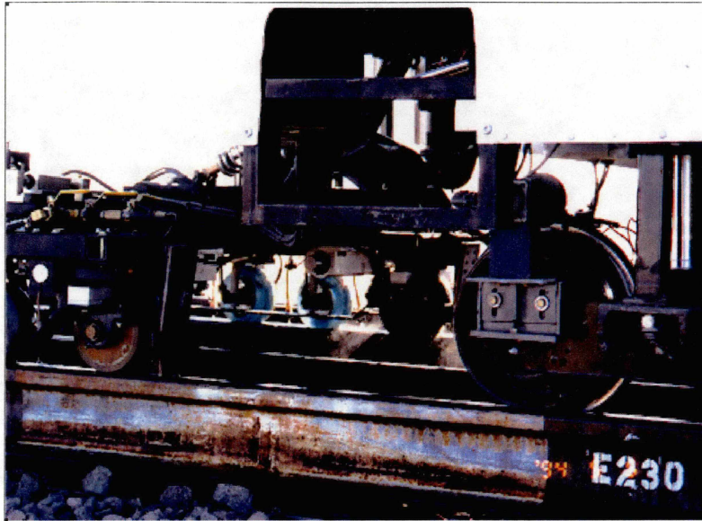
Figure C4. Roller Search Units on Hi-rail Ultrasonic Detector Car
