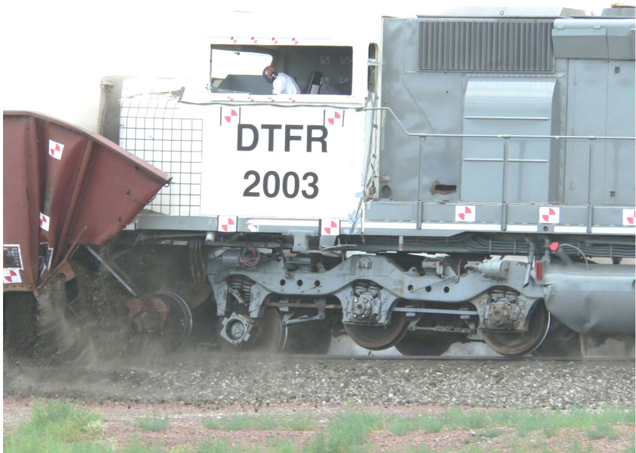
Figure 3. Locomotive Riding the Pilot Plate over Hopper Car Wheels
