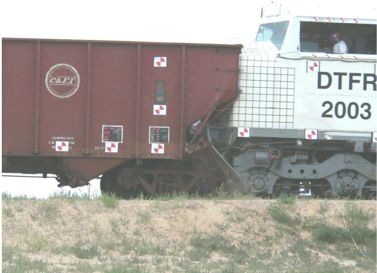
Figure 2. Pilot Plate Forced under Locomotive Structure
