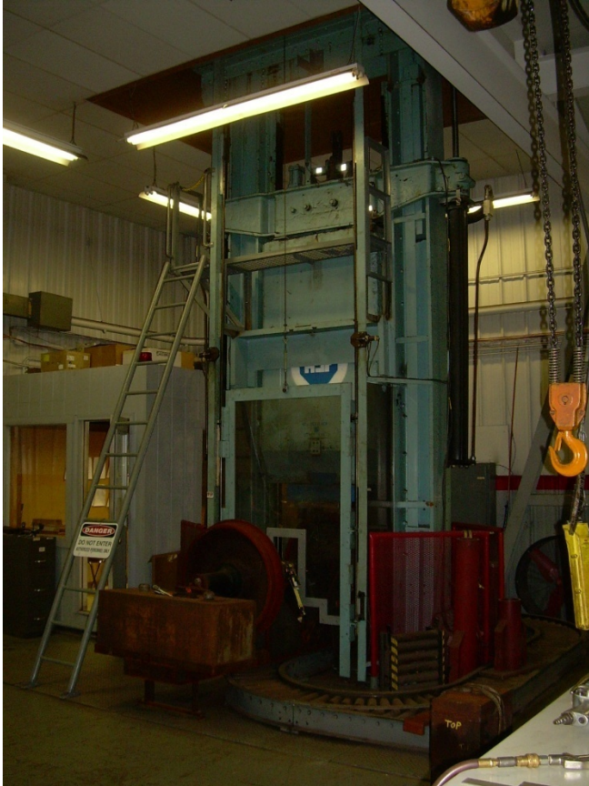
Figure 55. AFS-Keystone Drop Hammer Test Facility and Data Acquisition System
