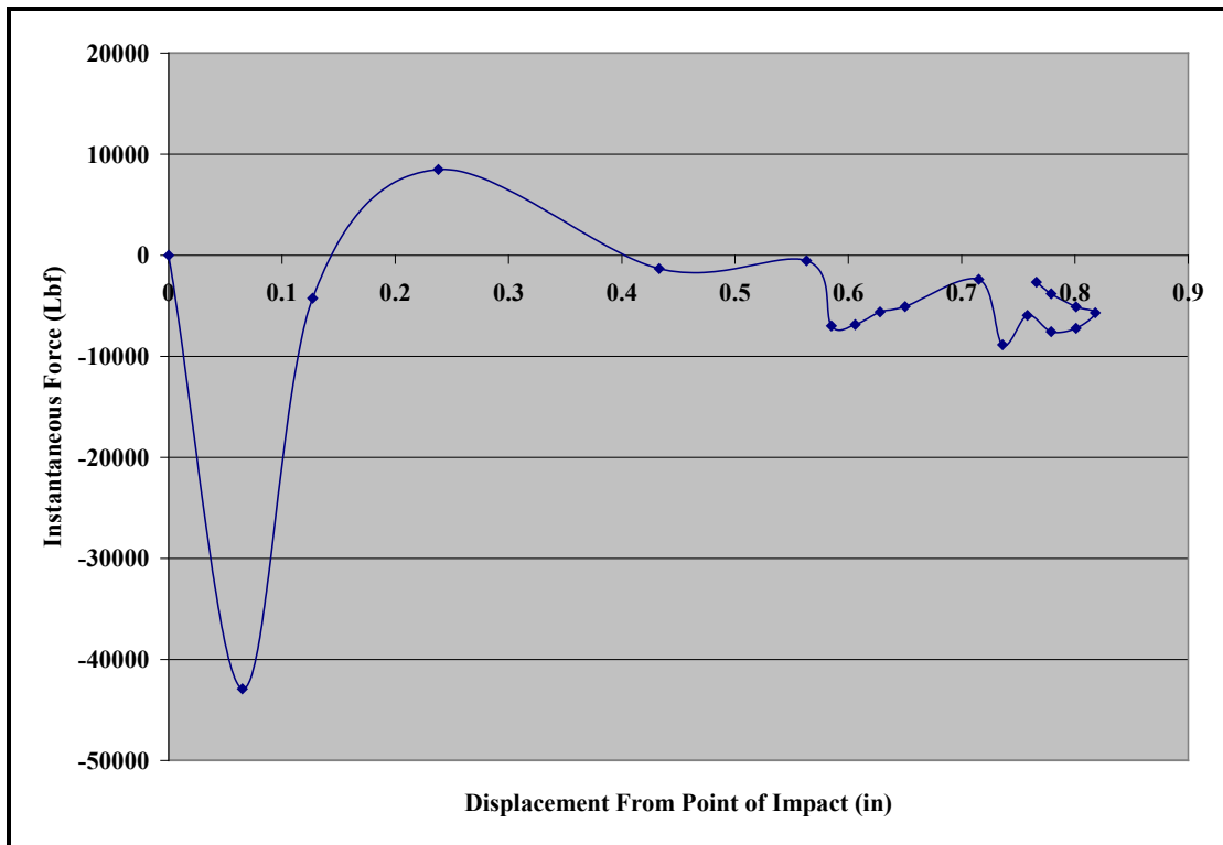
Figure 38. Instantaneous Inertia Force vs. Plunger Displacement
