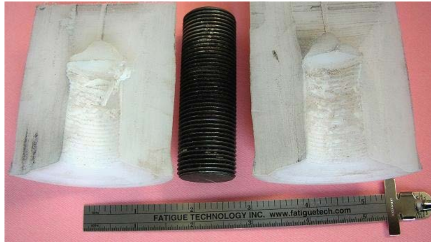
Figure 31. Test Sample with Thread Impressions and Solidified Face Material
