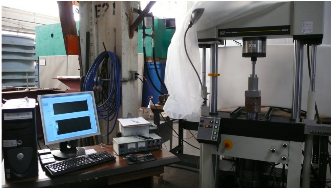
Figure 27. Test Setup for Quasi-Static Compression Test in Instron 8502 Test Machine
