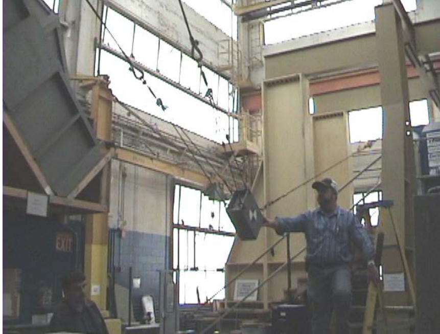
Figure 33. Pendulum Impact Test Setup with Mass Raised to a Height of 84 in above Ground
