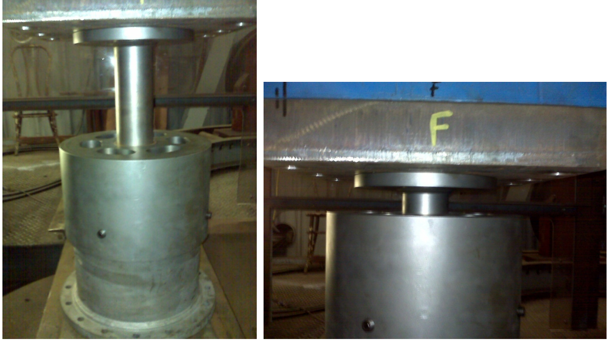
Figure 59. Prototype before and after Impact for 30-Inch Hammer Drop
