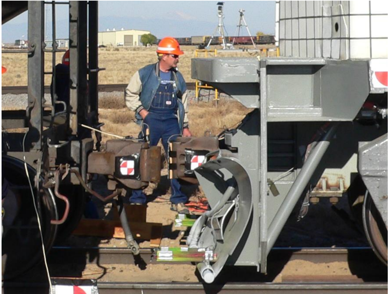
Figure 1. Mismatch between Hopper Car and Locomotive
