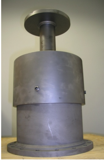
Figure 54. Picture of an Assembled SEA Prototype Fabricated for Drop Hammer Testing
