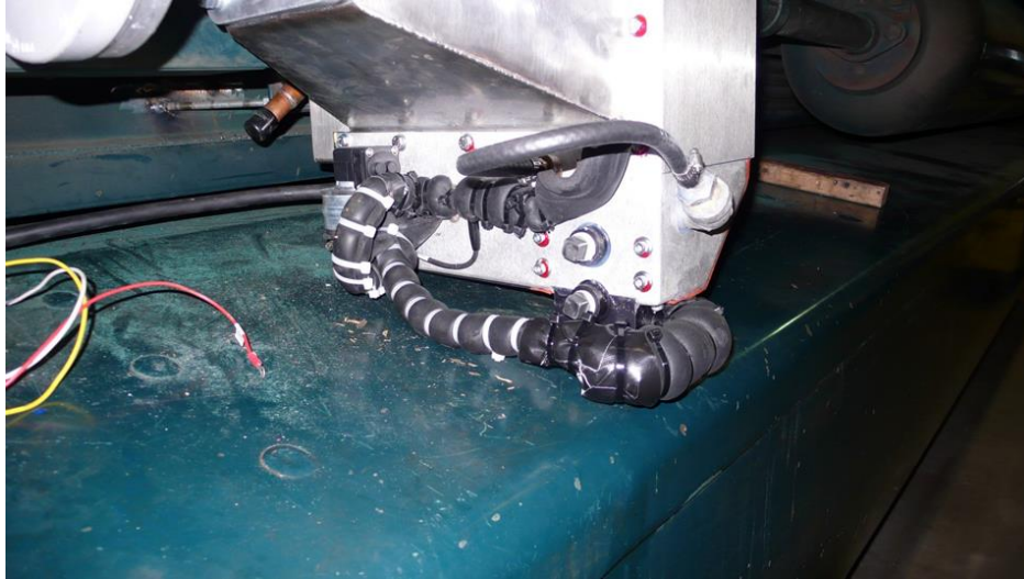
Figure 8. Condensed fuel measuring unit attached to the lower part of condenser
