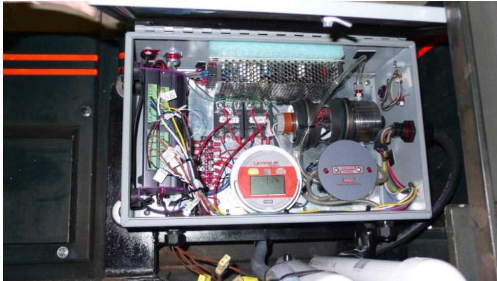
Figure 11. Electronics control and data communication box inside view
