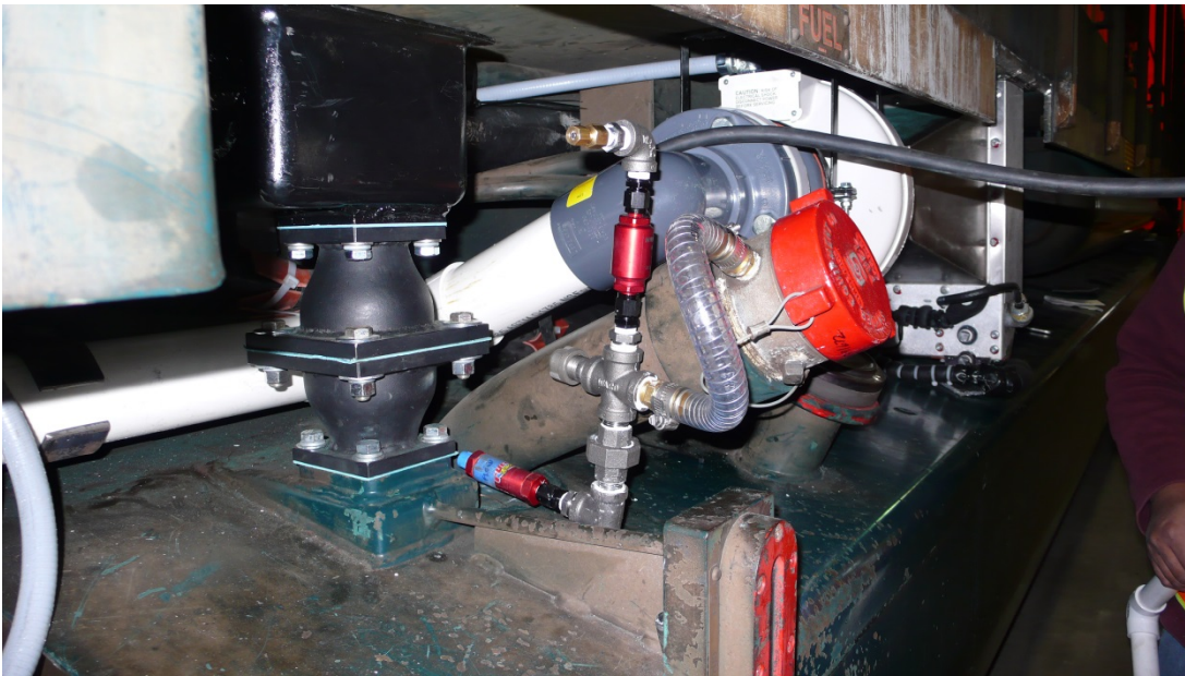
Figure 10. Temperature sensor and vapor sampling tube connection details to the fuel tank
