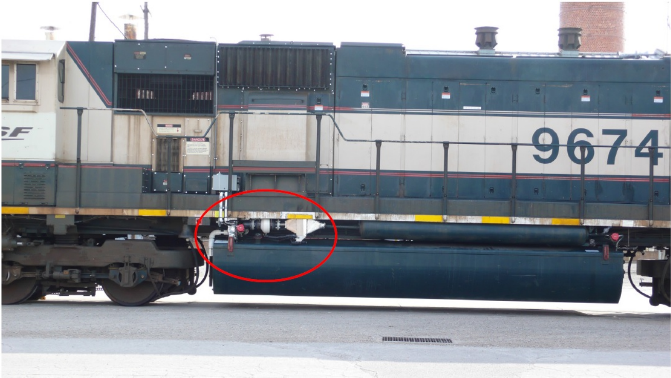
Figure 13. BNSF SD70 MAC locomotive # 9674 with installed DVRU in Topeka yard
