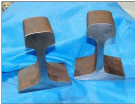
Figure 4. Two, 4-in. Long Rail Test Samples of 136RE
