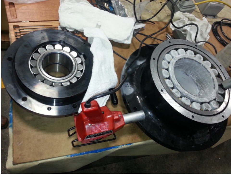
Figure 9. Large Oscillator Bearings Shown during Assembly
