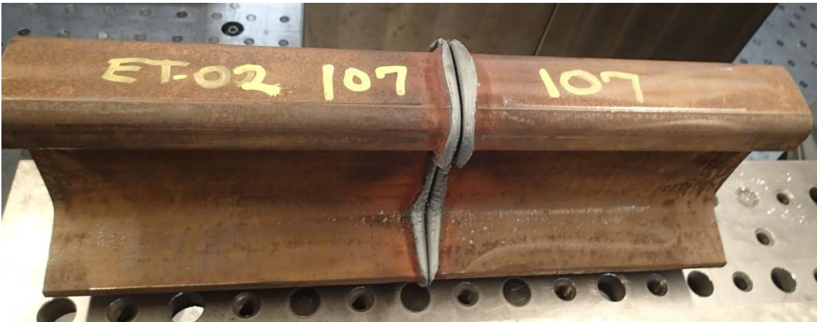
Figure 17. Weld 107 in the As-received Condition
