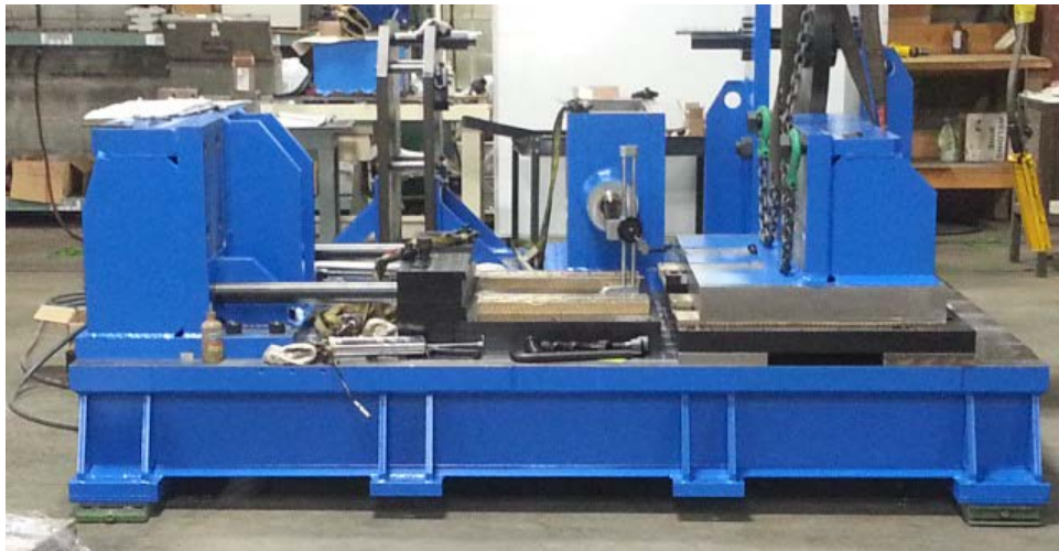
Figure 10. Side View of Frame; Forging Support (left), and Forging Bed (right)
