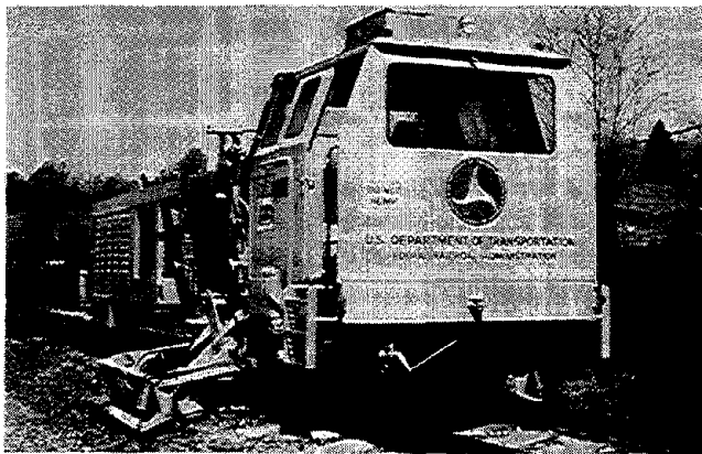
Fig. 14. The ballast consolidator.
