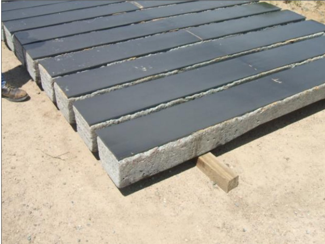
Figure 8. Cross-ties with Rubber Pads on Bottom Surface
