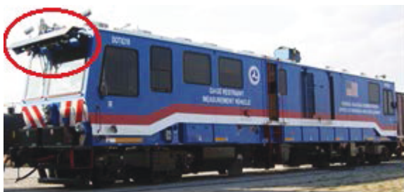
Figure 1. LiDAR-Based Scanning System for Grade Crossing Assessment Installed on FRA's DOTX 218
