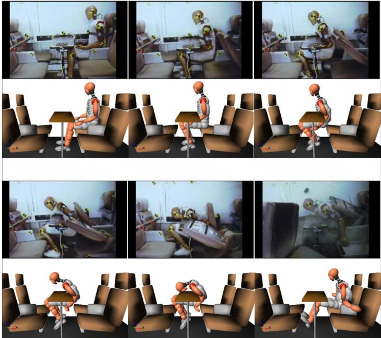
Figure H81. THOR Test Dummy Kinematics in Table Test, Simulation Results and Test Observations
