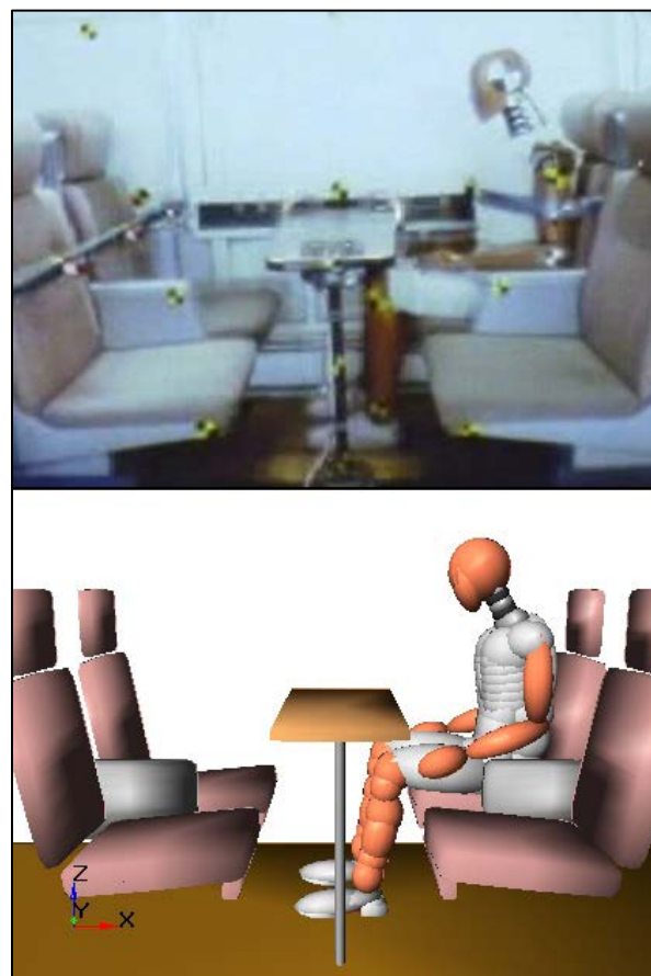
Figure G8. Test Photograph with H3RS ATD and Model Depiction with HIII ATD of Facing Seat Experiment with Workstation Table
