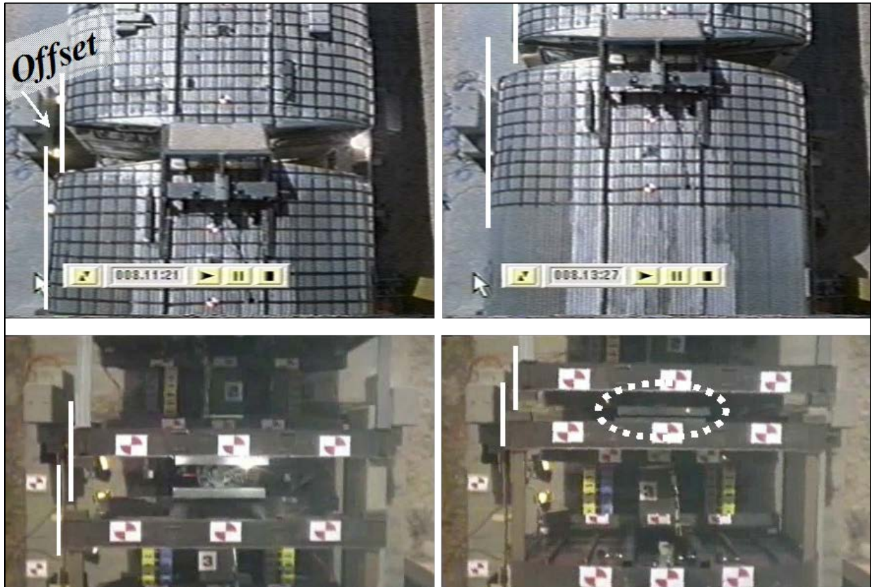
Figure 13. Still Photographs of Coupled Interface for Conventional (top) and CEM (bottom) at Time of Impact (left) and Maximum Crush (right)
