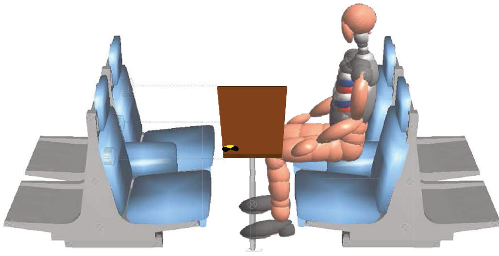
Figure F6. Placement of Photo Targets Visible to the Top- and Side-View Cameras in the Experiments with Workstation Tables
