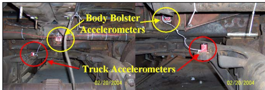
Figure B5. Typical Placement of Accelerometers mounted on the Body Bolster and Truck
