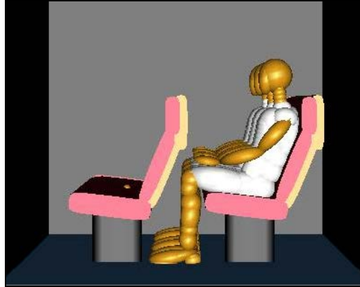
Figure G-19. Uninstrumented Hybrid II 50th-Percentile Male ATD in the Middle Seat Position
