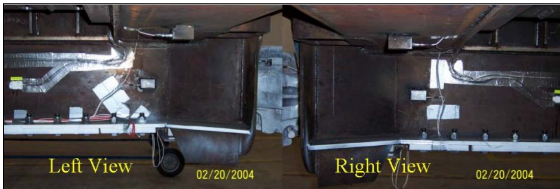
Figure B3. Typical Placement of Accelerometers on the Sliding Sill
