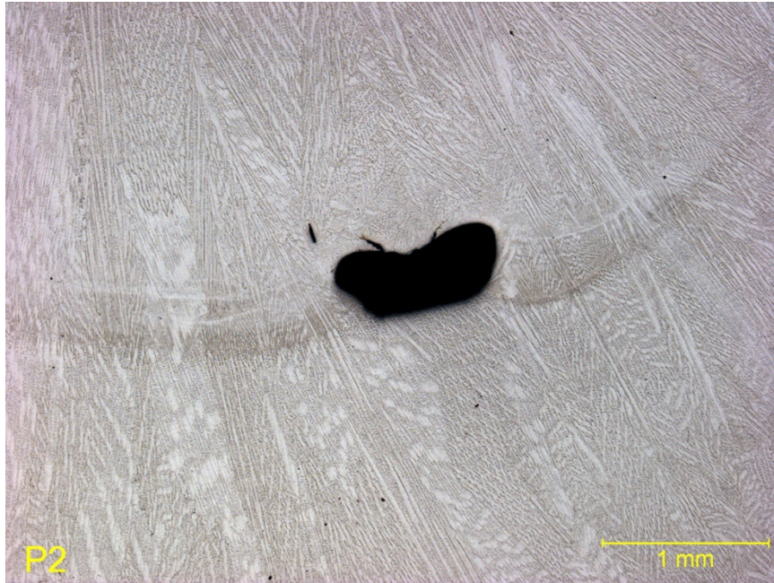
Figure 70: Weld Metal Showing Slag Inclusion
