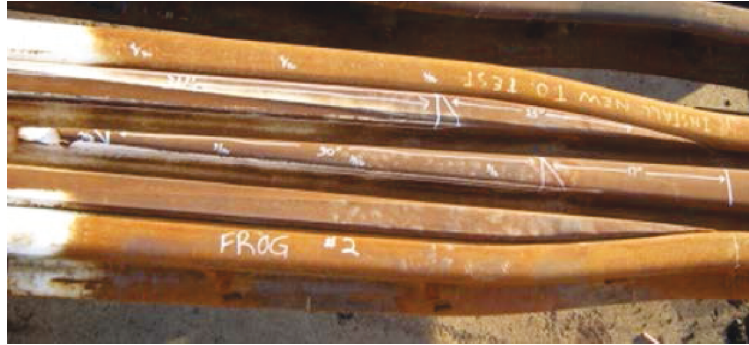
Figure 34: Frog #2 Marked for Carbon Arc Gouging
