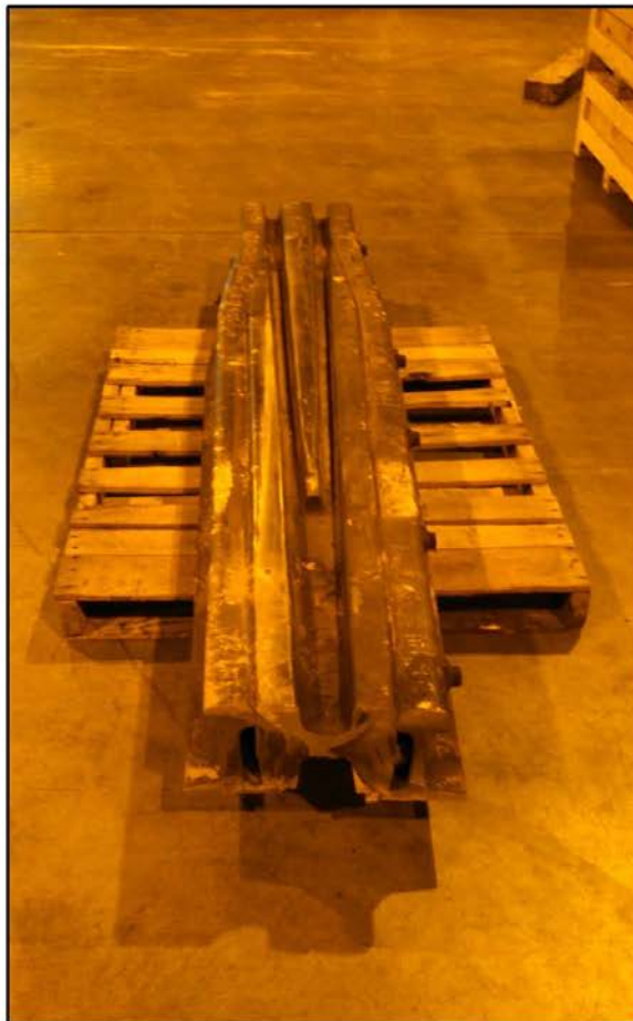
Figure 22. Test Frog 2 cut and ready for return shipping to EWI
