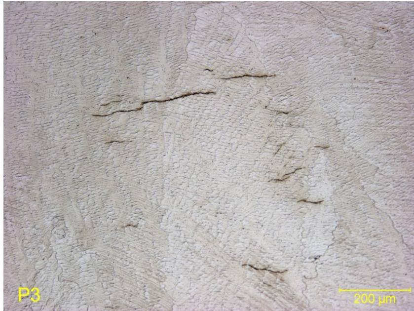
Figure 72: Horizontal Cracks Likely Due to Shear Loading (2)
