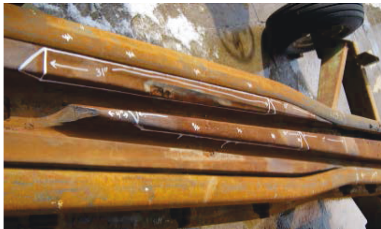
Figure 33: Frog #1 Marked for Carbon Arc Gouging
