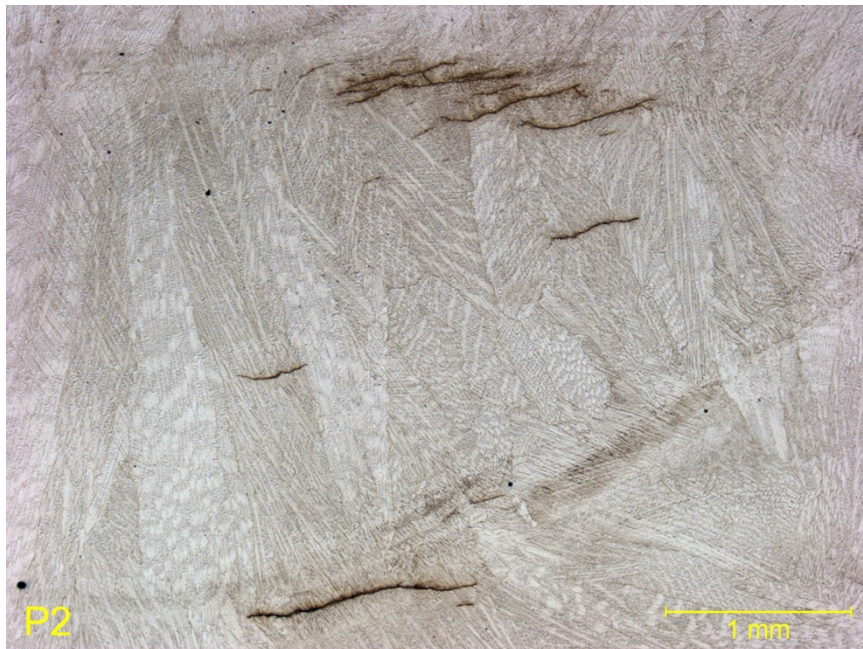
Figure 71: Horizontal Cracks Likely Due to Shear Loading (1)
