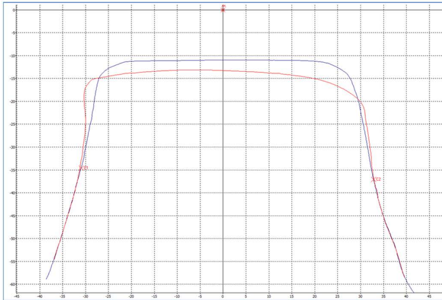
Figure 6. Frog Point: Measurement location 16, 32 inches past the POF — overlay of the newly ground (0 MGT) weld repaired frog point profile and the final profile (100 MGT)
