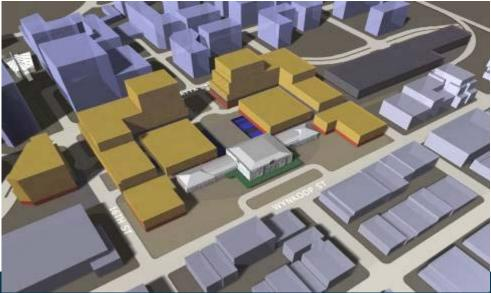
All transit elements underground: Green = LRT Blue = Amtrak and commuter rail Yellow = bus terminal On-site joint development stacked on roofs of underground transit structures.
