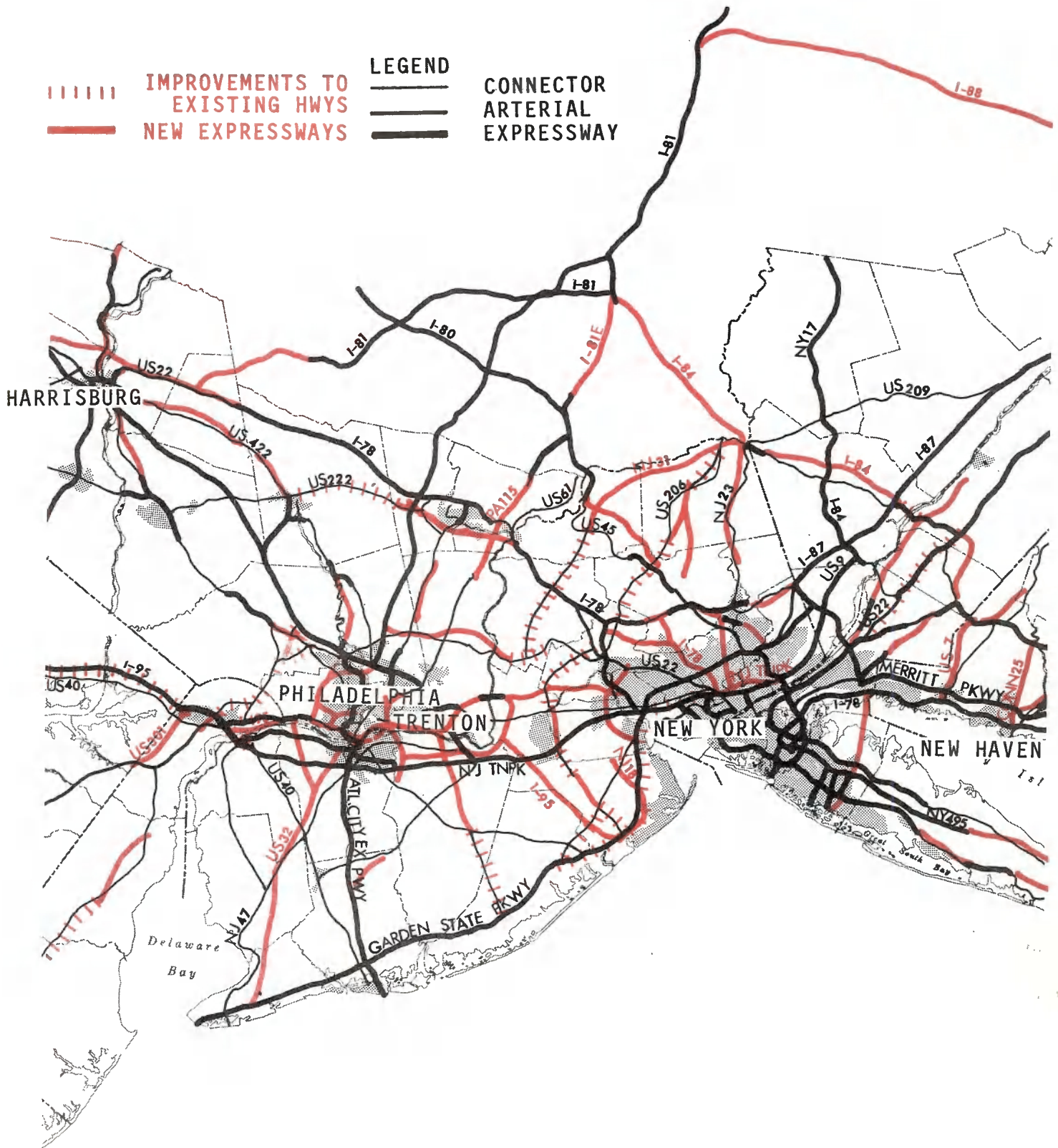
Figure T2-4-B. Principal highway improvements planned through 1980 in the Northeast Corridor -- Central sub-region
