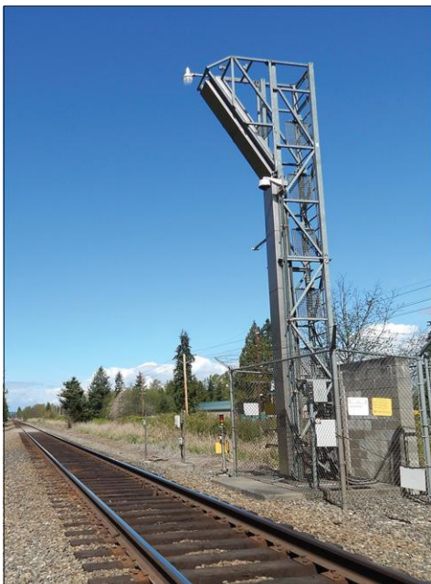
Example of R-VACIS in Blaine, WA (Photo Credit: GAO)
