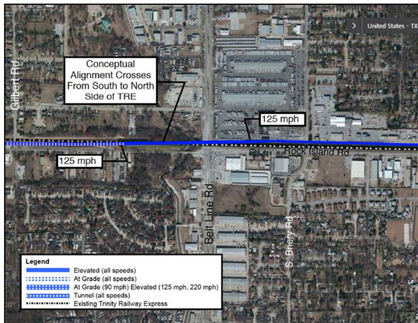
Figure 3-26: Alignment at Belt Line Rd.
