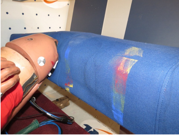
View of opposing (rear facing) seat pan cushion and witness marks from knee contacts.
