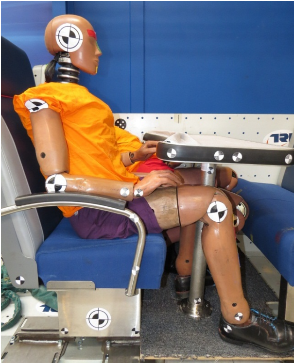
The Hybrid III-RS slid under the table such that its knees contacted the seat opposite.
