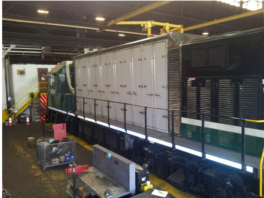
Figure 5. Battery ISO container in place on NS 999
