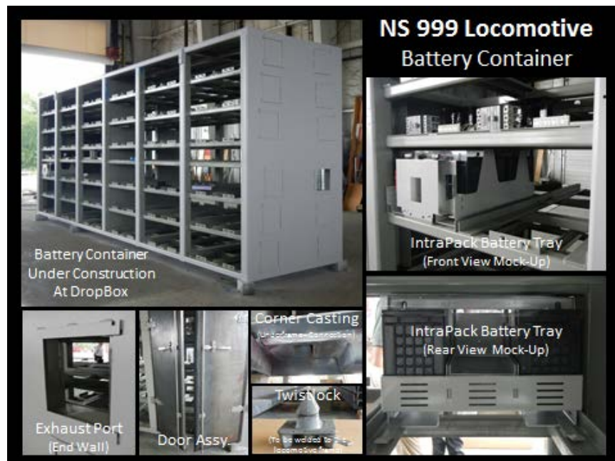
Figure 4. NS 999 battery ISO container manufactured at DropBox, Inc.
