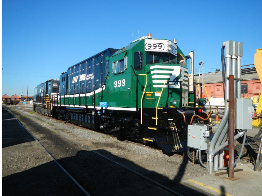
Figure 7. NS 999 charge and discharge testing at Juniata locomotive shop
