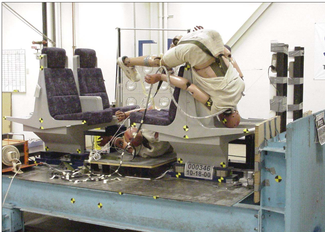
Figure 18. Post-test Photo of Test No. 1, Baseline Test
