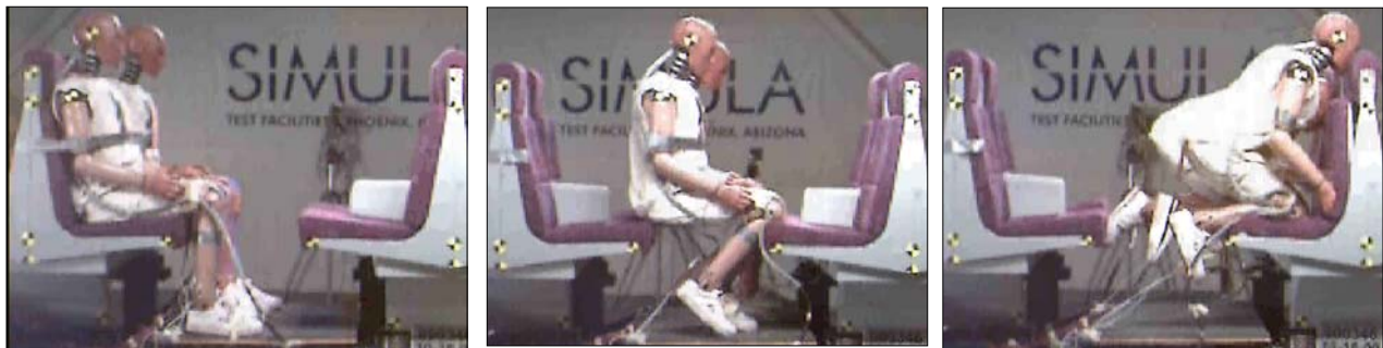
Figure 17. Test No. 1, Occupant Kinematic Sequence for Two 50th-percentile ATDs, 8 G Peak, No Table
