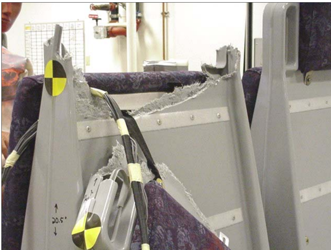
Figure 29. Jagged Seat Back Edge Resulting from Failed Headrest
