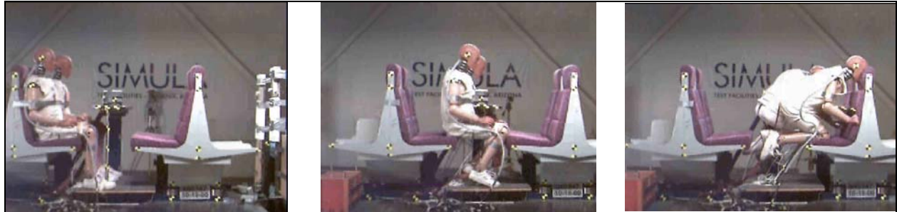
Figure 21. Test No. 2, Occupant Kinematic Sequence for Two 50th-Percentile ATDs, 8 G Peak, with Table Installed
