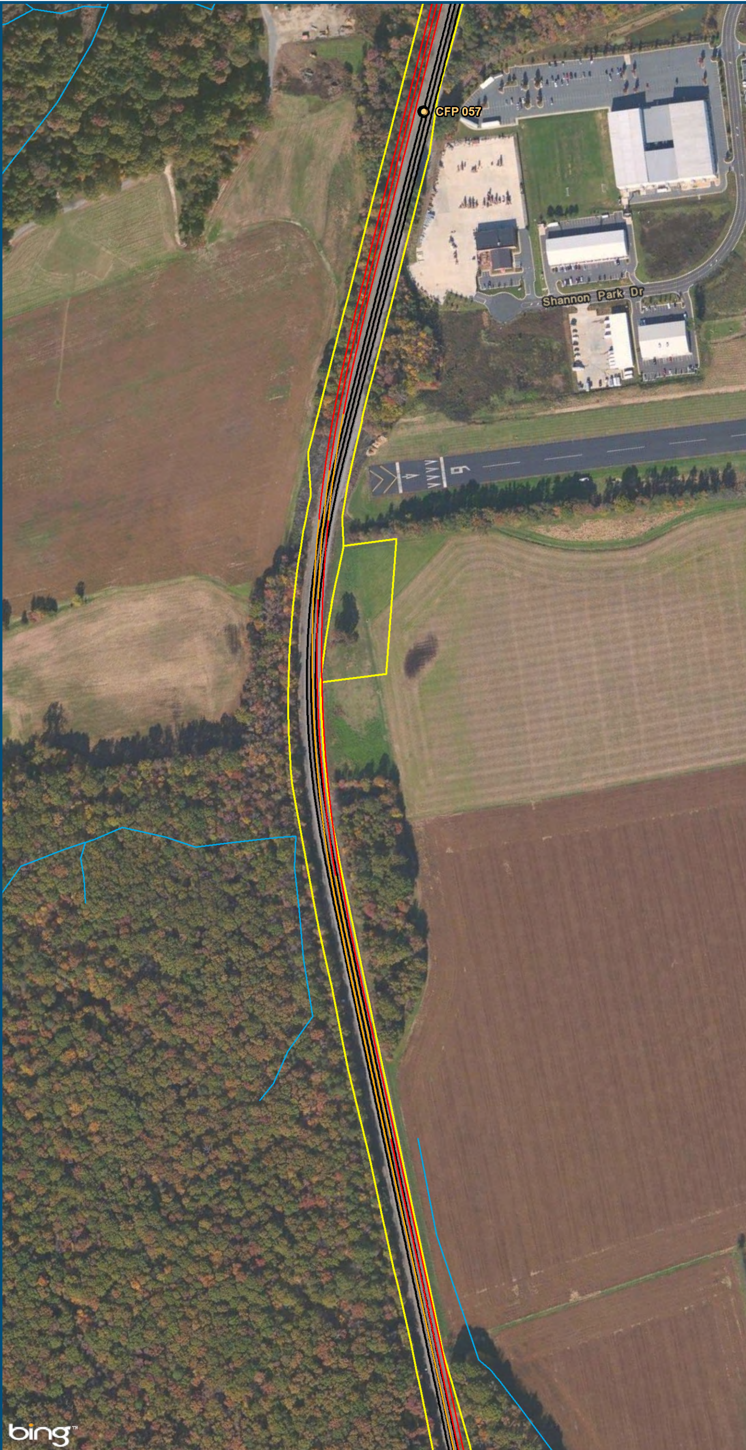
Figure G-64 Northern Virginia Constrained Alignment Option
