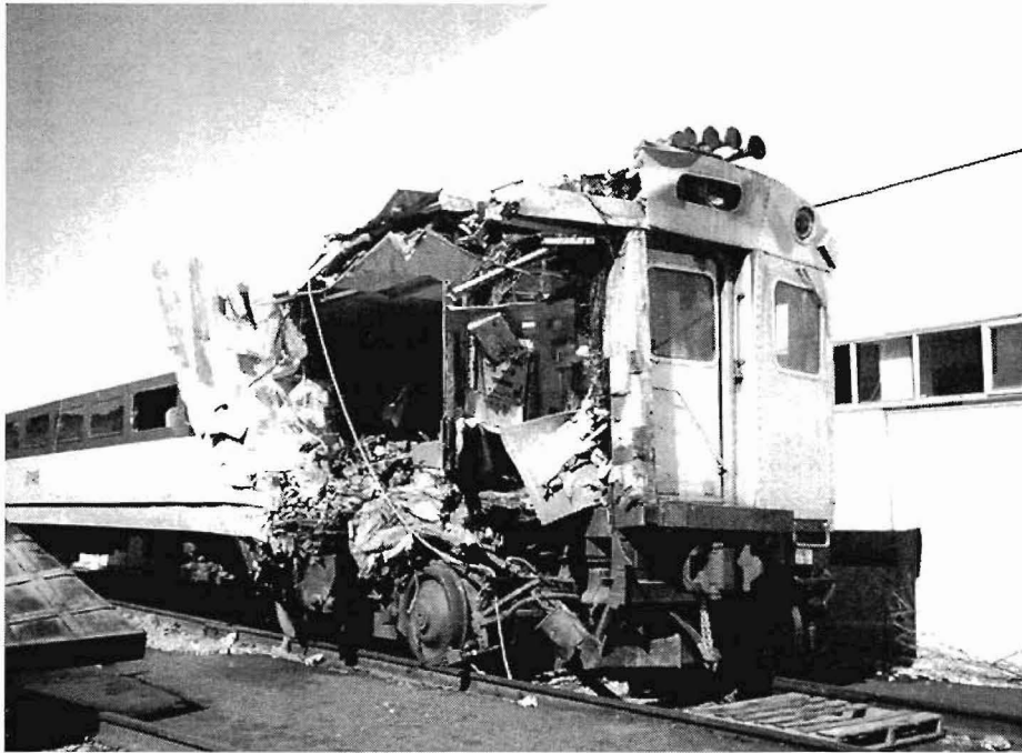
Figure 1. Photograph of the Cab Car Damaged in the Secaucus, New Jersey, Accident
