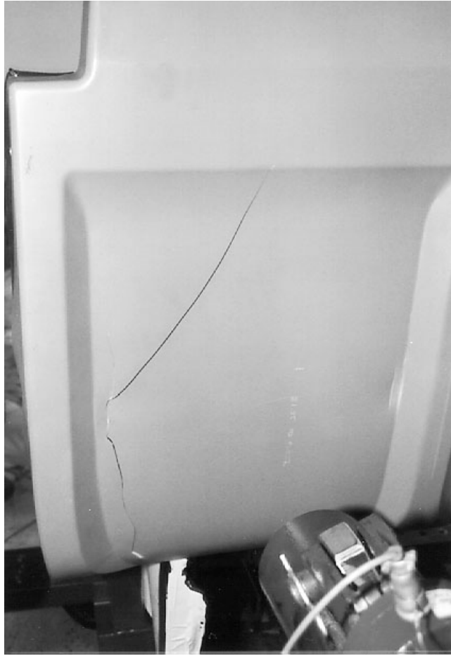
Figure 17. M-Style Lower (Post-test) - Plastic Shroud Cracked
