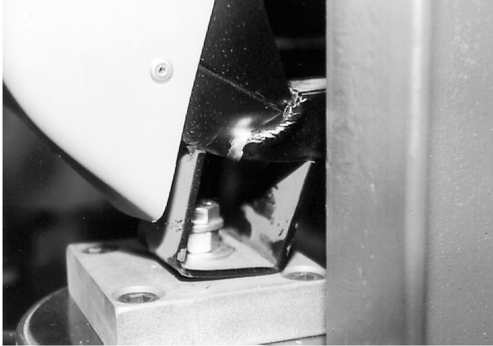
Figure 15. M-Style Upper (Post-test) - Square Beam Attachment Buckled
