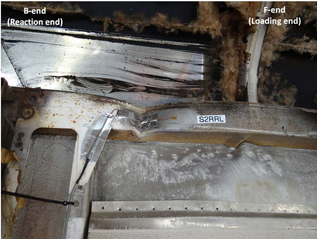
Figure B10. Post-test — Left Roof Rail Buckle at Section 2
