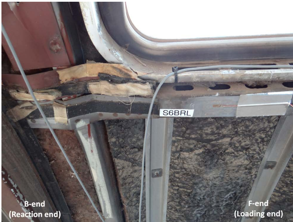
Figure B18. Post-test — Left Belt Rail Deformation near Section 6
