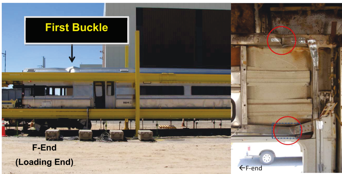
Figure 32. First Buckle at Approximately 700,000 lbs Exterior (left) and Interior (right)
