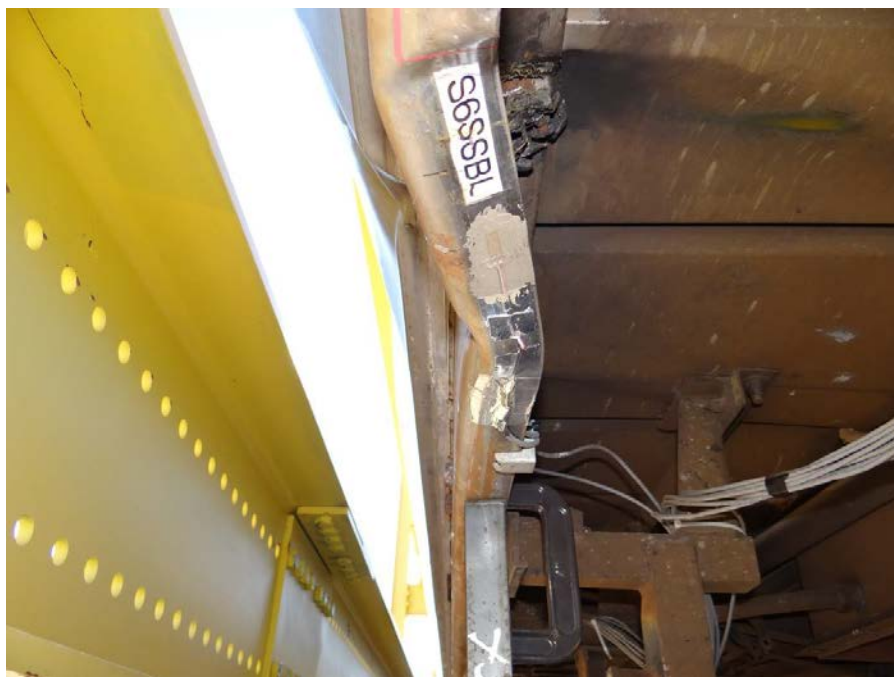
Figure 34. Section 4 Right Side Sill Buckle
