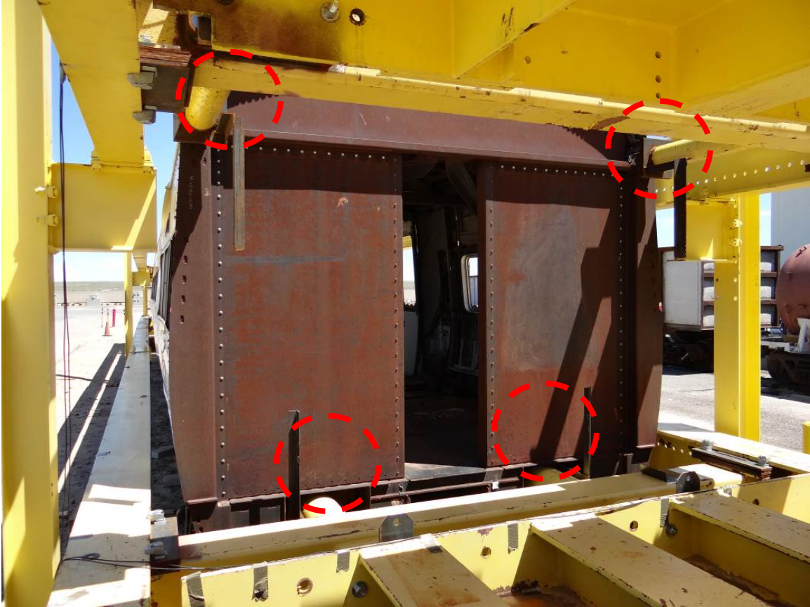
Figure 10. Loads Reacted at CEM Pockets on B-End of Car
