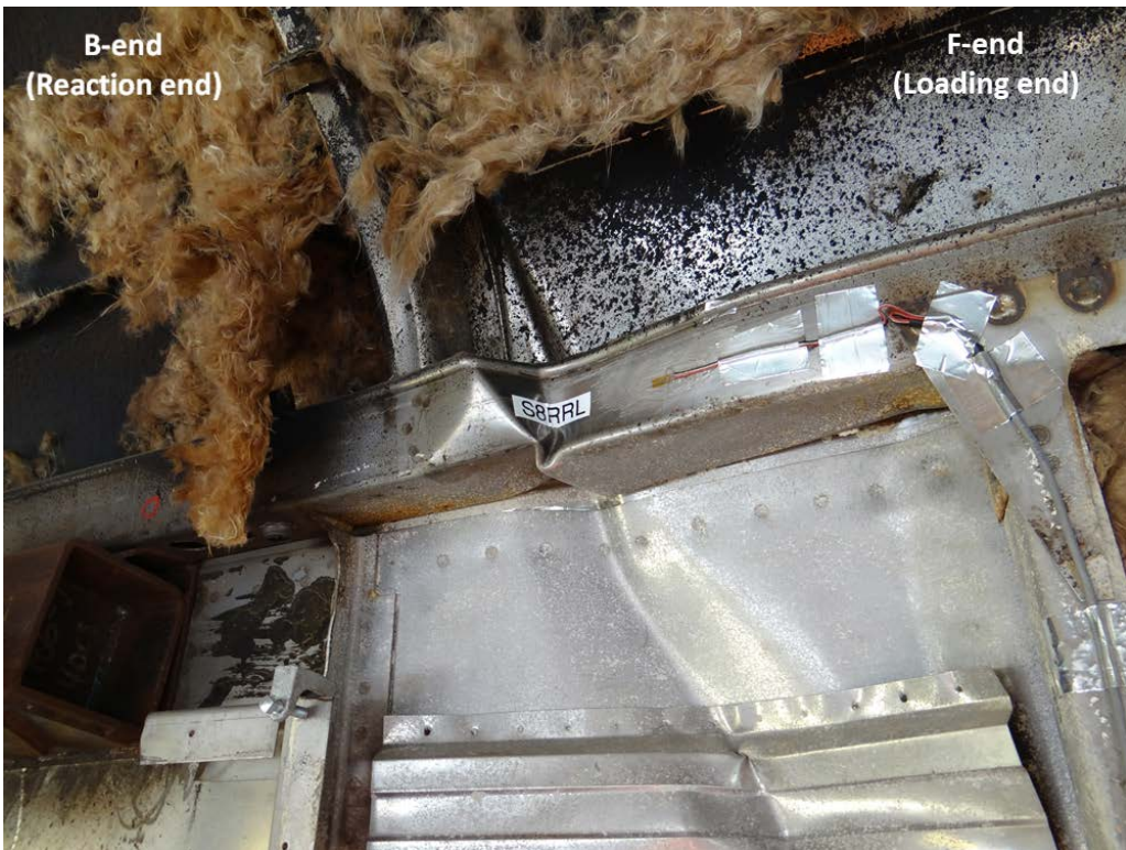
Figure B22. Post-test — Left Roof Rail Buckle at Section 8
