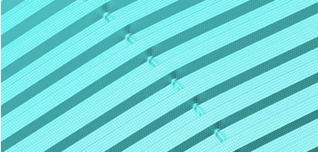
Figure H4. Local Folding in the Fine Meshed Corrugated Analysis
