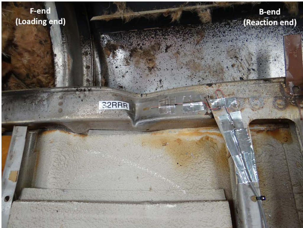
Figure B11. Post-test — Right Roof Rail Buckle at Section 2
