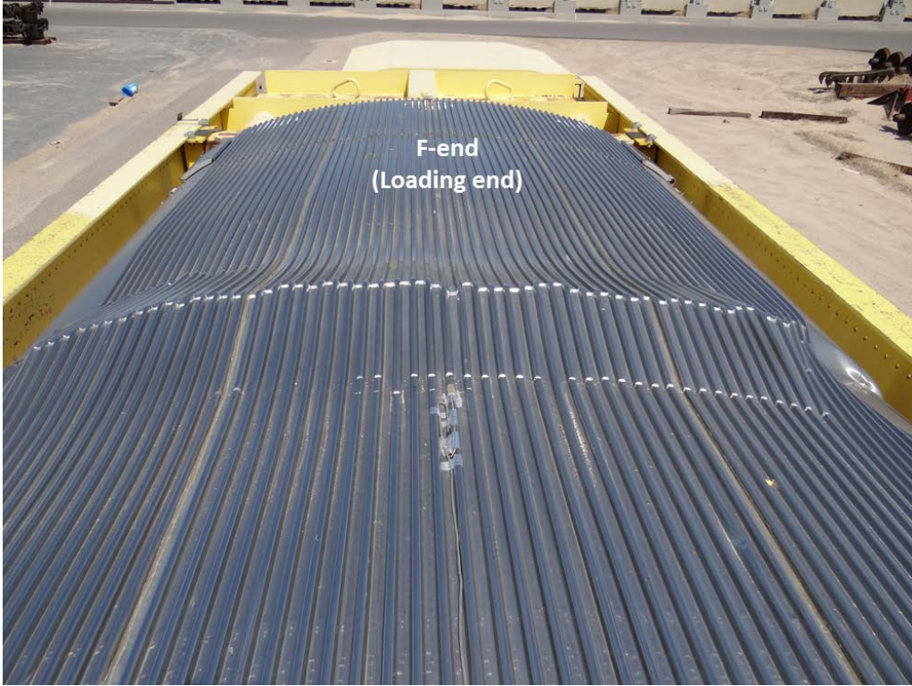
Figure B9. Post-test — Roof Buckle near Section 2
