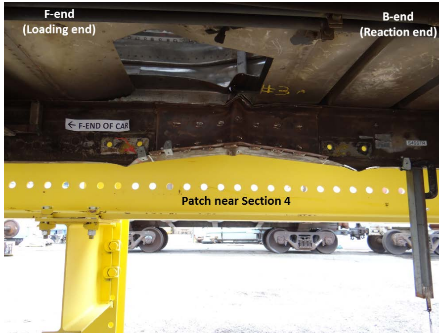
Figure 34. Section 4 Right Side Sill Buckle
