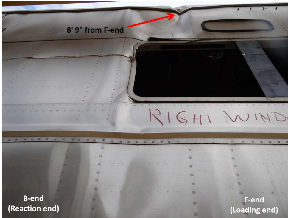
Figure B8. Post-test — Deformation at Section 2 on Right Side of Car
