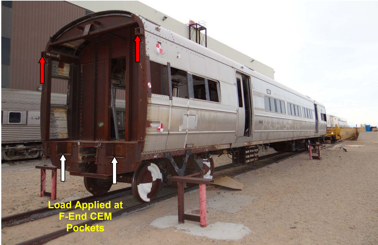
Figure 8. Load Application Sites at F-End CEM Pockets
