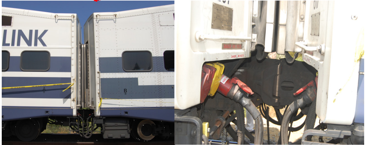
Figure A.1-8. Interaction of Second Passenger Car and Trailing Cab Car
