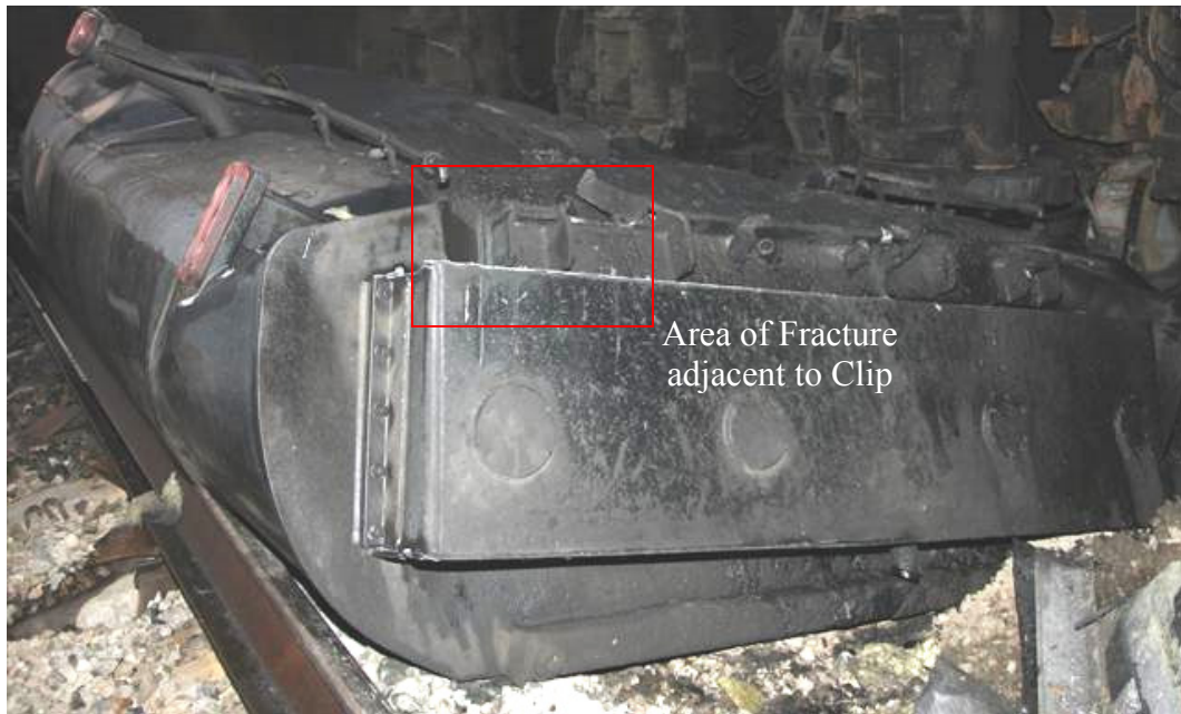
Figure A.3-8. Trailing End of Fuel Tank
