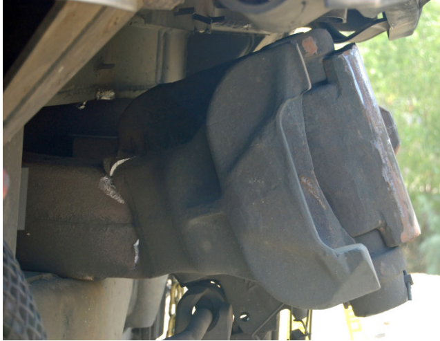
Figure A.1-7. Trailing Coupler of Lead Passenger Car and Leading Coupler of Second Passenger Car
