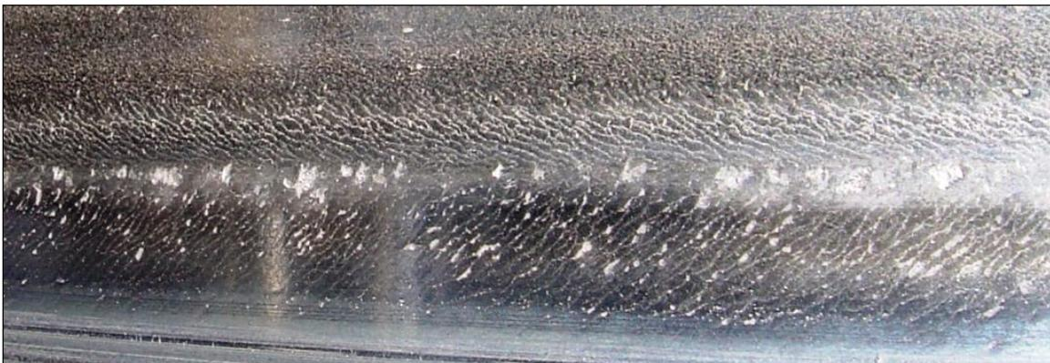
**Figure 1. Wheel Tread Surface with RCF Cracks**
