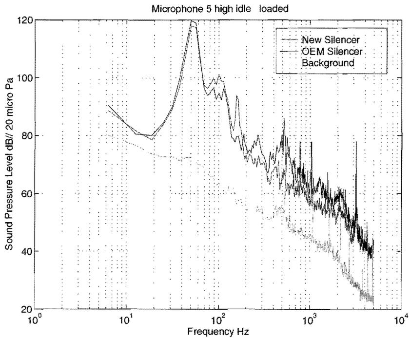
**Figure 95. Comparison of Noise Levels at Microphone 5 with the OEM and New Silencers Throttle 1 Loaded**
