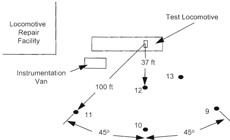
Figure 53. Test Site with Far Field Microphone Position
