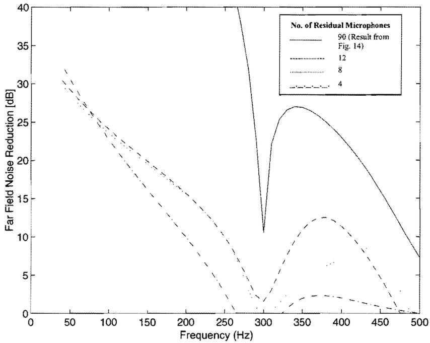
**Figure 18. Reduction in the Mean Square, Angular-Averaged Sound Pressure - Noise Reduction [dB] Versus Frequency [Hz] - at 30.4 Meters from the Exhaust Outlet with Eight Control Speakers and Various Numbers of Residual Microphones at 1.5 Meters from the Exhaust**
