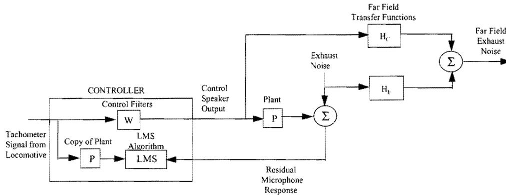
**Figure 10. Block Diagram**
