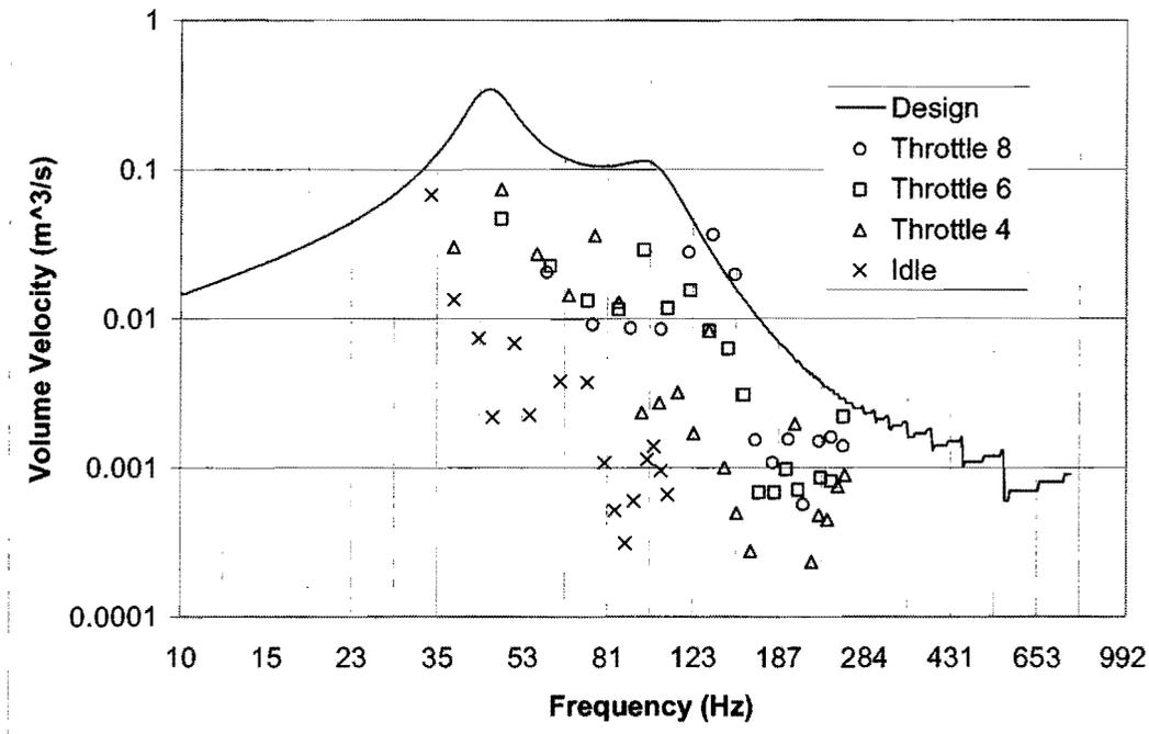
Figure 28. Predicted Speaker Volume Velocity Versus Frequency for Two McCauley 12-Inch Speakers in a Ported Enclosure Each Driven at 300 Watts
