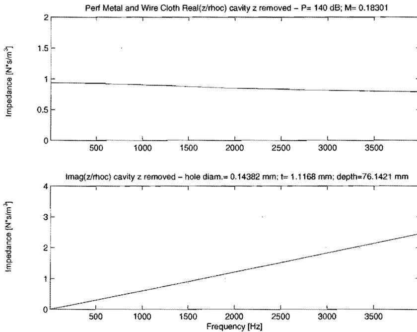
**Figure 33. Predicted Impedance [Nos/m<sup>3</sup>] of Five Layers of Screening on Perforated Metal Sheet Screening (60 Wires/Inch; 0.011 Inch Dia. Wire; 5 Layers Perforated Sheet: 20% Open Area; 0.1-Inch Dia. Holes; 0.1 Inches Thick; Mach No. = 0.2; SPL= 140 dB)**
