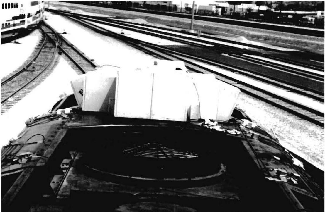
*(b) Microphones Taped to the Locomotive Hood*
