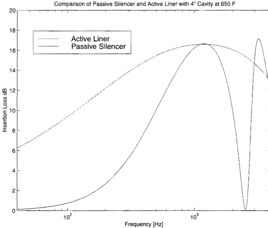
**Figure 3. Comparison of Active and Passive Liner Performance**
