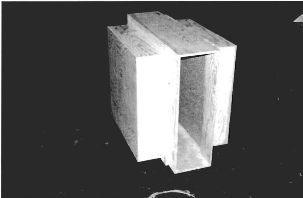
**Figure 36. The Silencer Prepared for Testing with Sintered Metal Liner**
