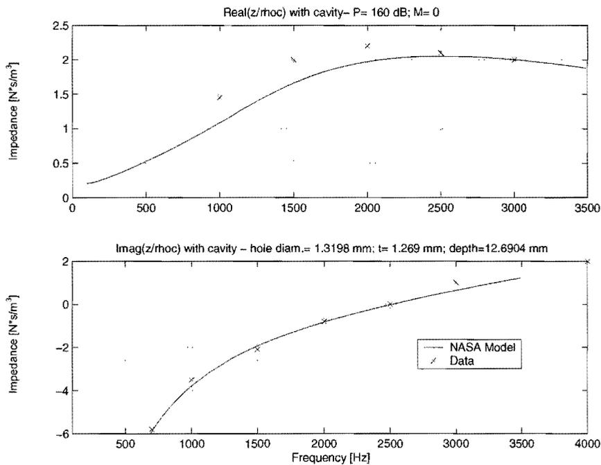
**Figure 31. Comparison of Liner Impedance [N•s/m<sup>3</sup>] Predictions and Measurements (5.2 Percent Open Area; 0.052-Inch Dia. Holes; 0.05-Inch Thick Sheet Over ½ Inch Cavity; Mach No. = 0; SPL 160 dB)**
