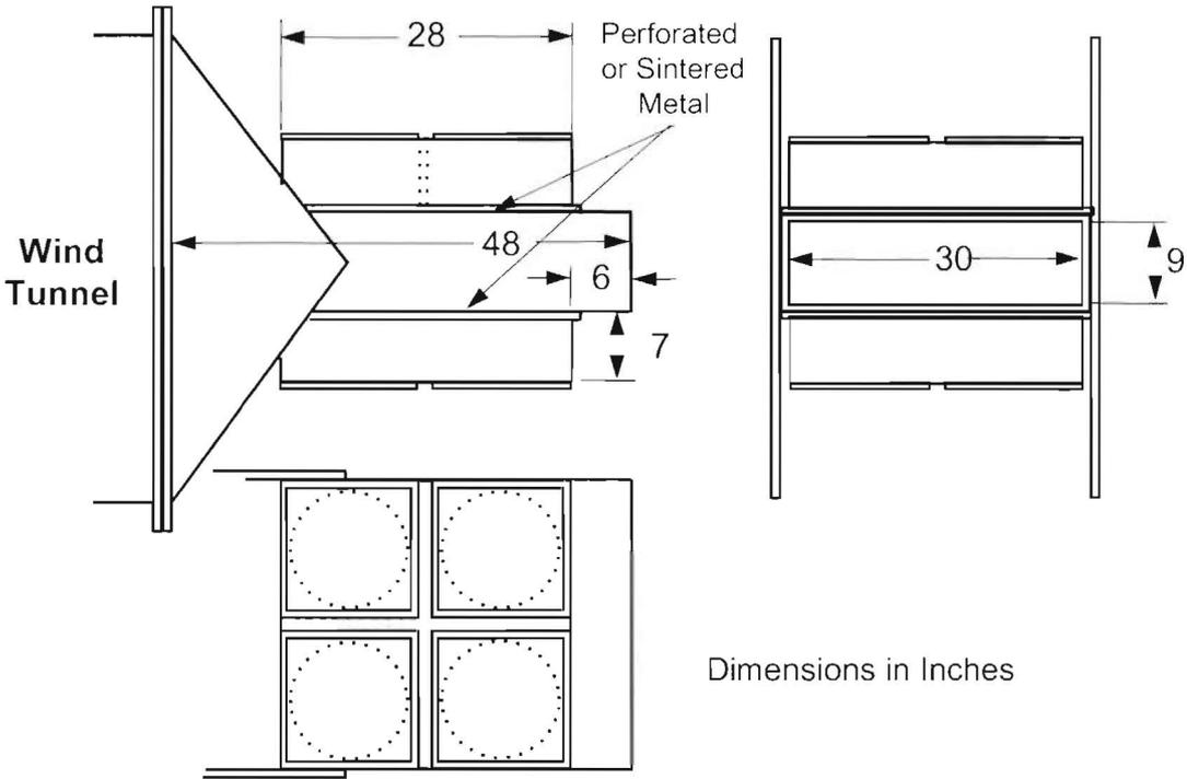
**Figure 34. Setup for the Wind Tunnel Test of Insertion Loss for the Active Liner Concept**
