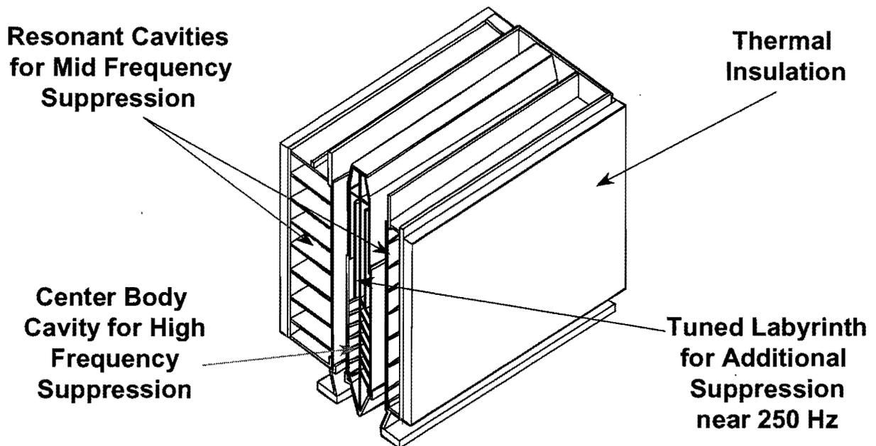
**Figure 29. Passive Silencer Design, a Straight-Through Resistive Silencer**
