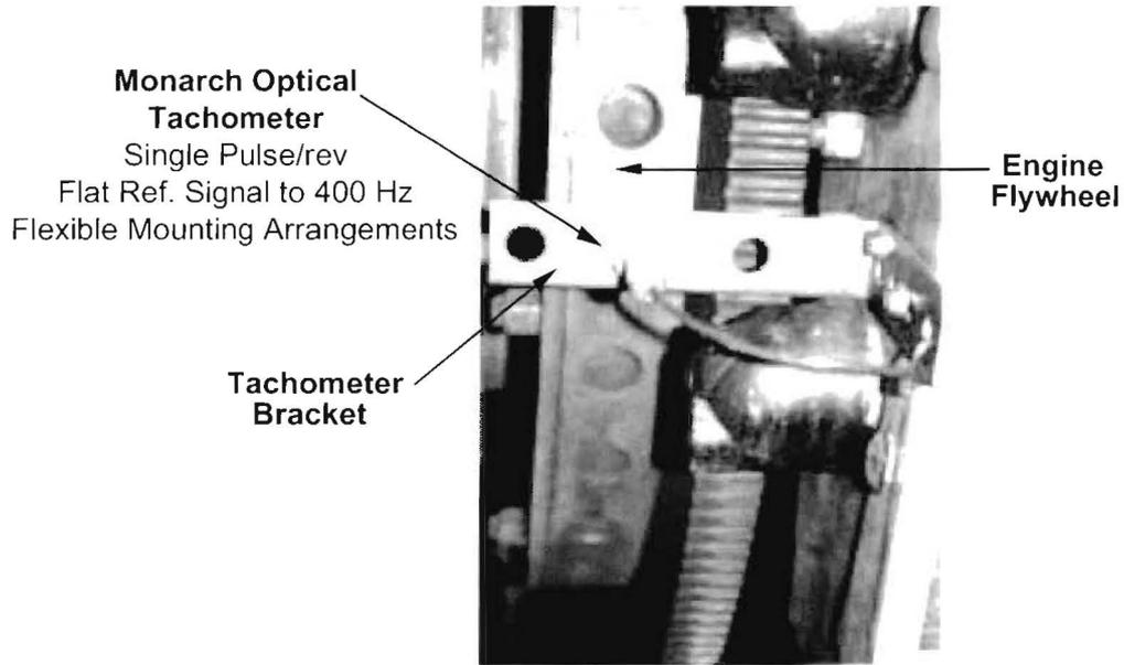
**Figure 72. Tachometer Mounted Near the Locomotive Flywheel**
