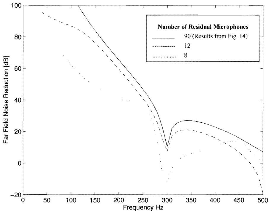
**Figure 16. Reduction in the Mean Square, Angular-Averaged Sound Pressure at 30 Meters from the Exhaust Outlet with Eight Control Speakers and Various Numbers of Residual Microphones in the Far Field at 30.4 Meters from the Exhaust**
