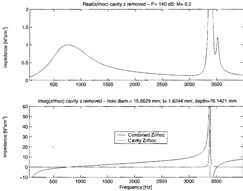
**Figure 32. Predicted Impedance [Nos/m<sup>3</sup>] of Perforated Metal Sheeting (5% Open Area; 1/16-Inch Dia. Holes; 0.064 Inches Thick; Mach No. = 0.2; SPL= 140 dB)**
