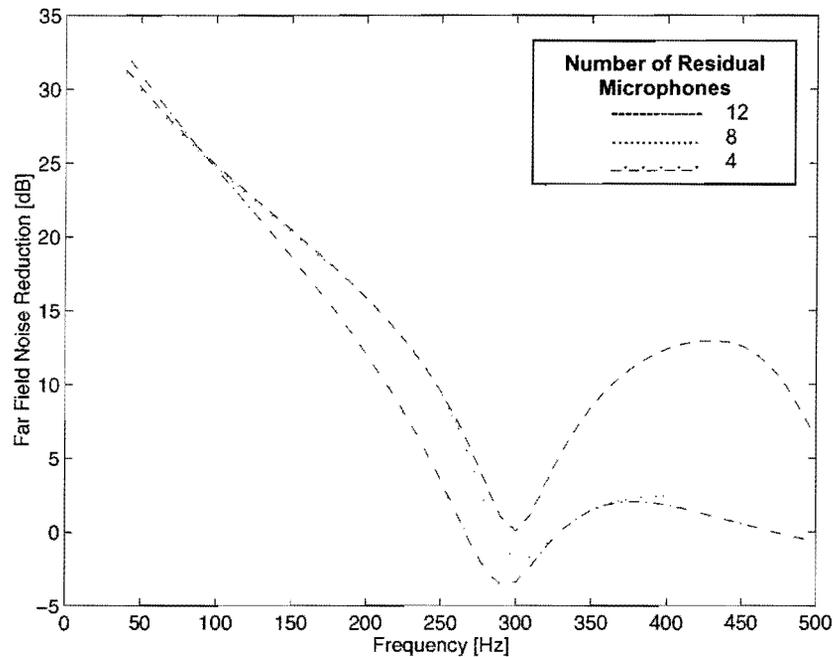
**Figure 20. Reduction in the Mean Square, Angular-Averaged, Sound Pressure at 30.4 Meters from the Exhaust Outlet with Eight Control Speakers and Various Numbers of Residual Microphones at 1.5 Meters from the Exhaust**
