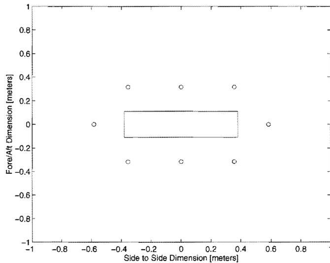
**Figure 14. Control Speaker Locations Around the Exhaust Stack**
