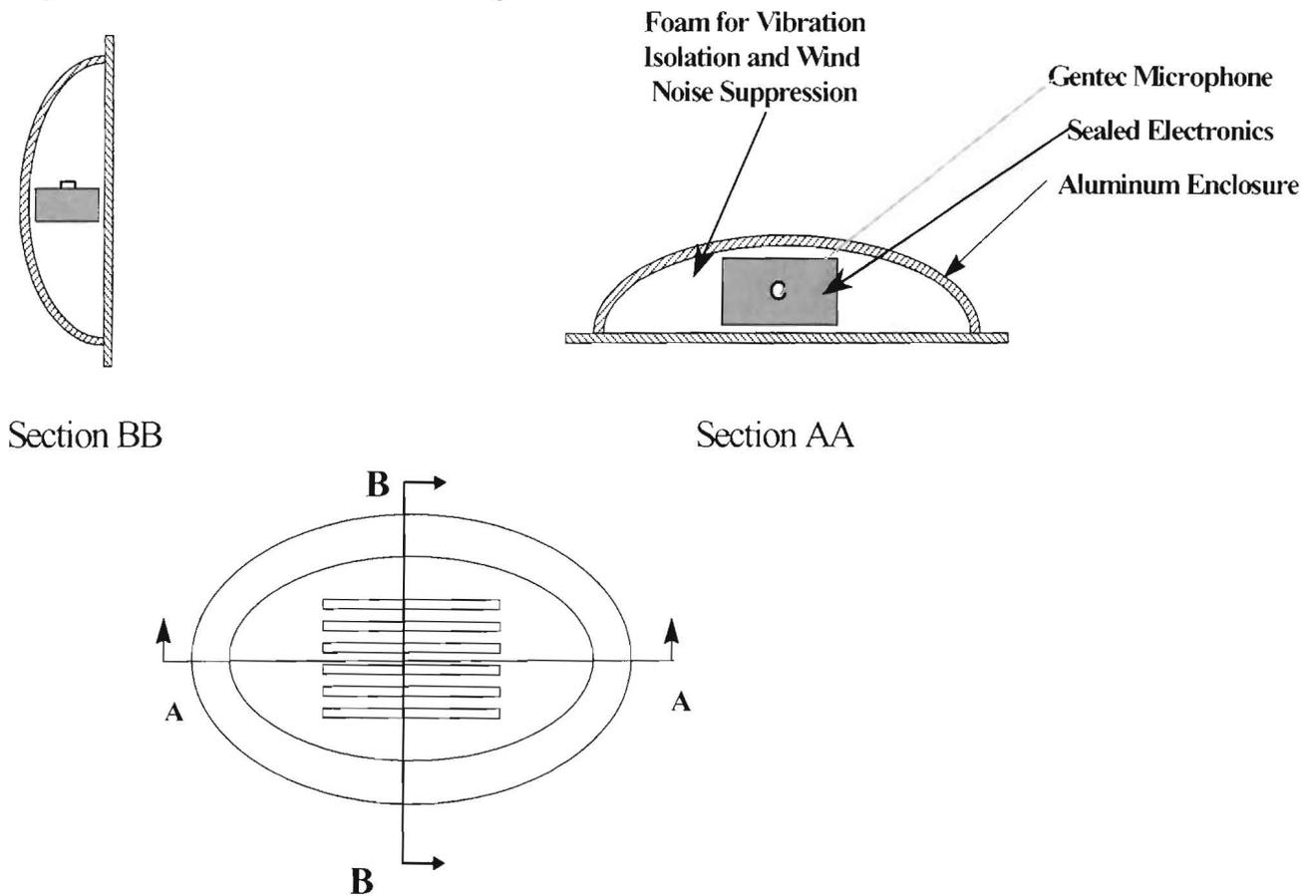
**Figure 70. Control Microphone Package**
