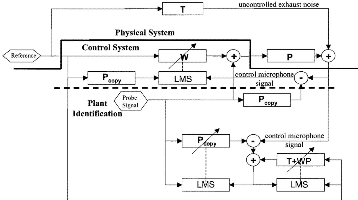
**Figure 43. System Block Diagram Showing System Identification Module**
