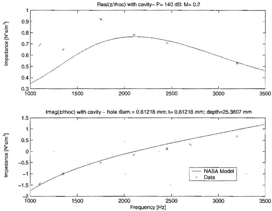
**Figure 30. Comparison of Liner Impedance [N•s/m<sup>3</sup>] Predictions and Measurements (6.7 Percent Open Area; 0.032-Inch Dia. Holes; 0.032-Inch Thick Sheet Over 1 Inch Cavity; Mach No. = 0.2; SPL 140 dB)**
