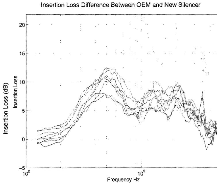
**Figure 101. The Average Insertion Loss Difference Between the OEM and New Silencer**
