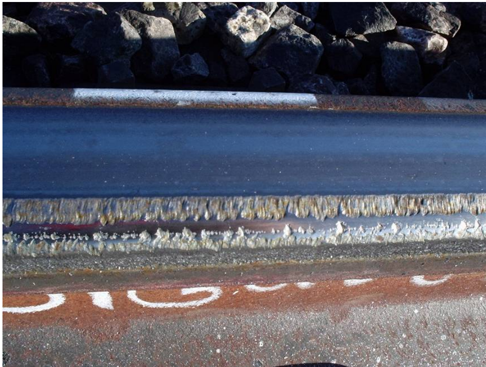
Figure 18. Typical View of Gage Corner on Laser-Treated Rail, No Spalls. Compare to Figures 3 and 4, Which Show the Gage Corner Before Train Operation
