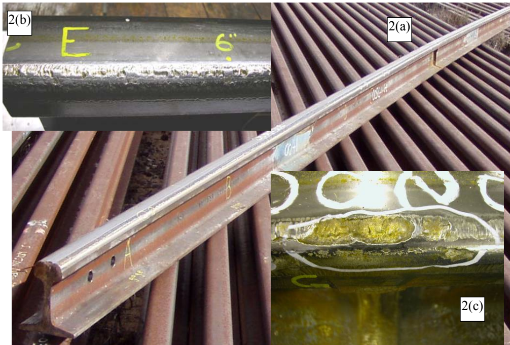
Figure A-2. Figure A-2(a) Rail Removed from FAST Facilities After Approximately 5.6 MGT of HAL Traffic, Figure A-2(b). Macro-Picture Showing Severe Wear, and Figure A-2(c). Macro-Picture Showing Shelling Regions of the Laser-Glazed Rail
