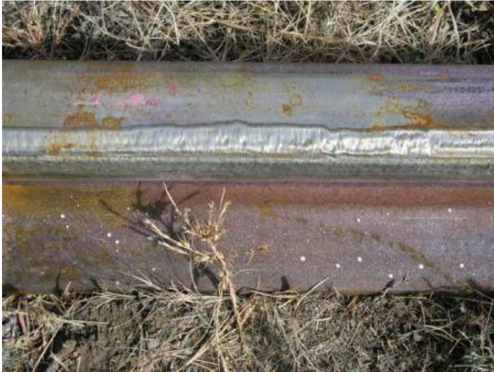
Figure 3. Overall View of Laser-Treated Rail Before Installation
