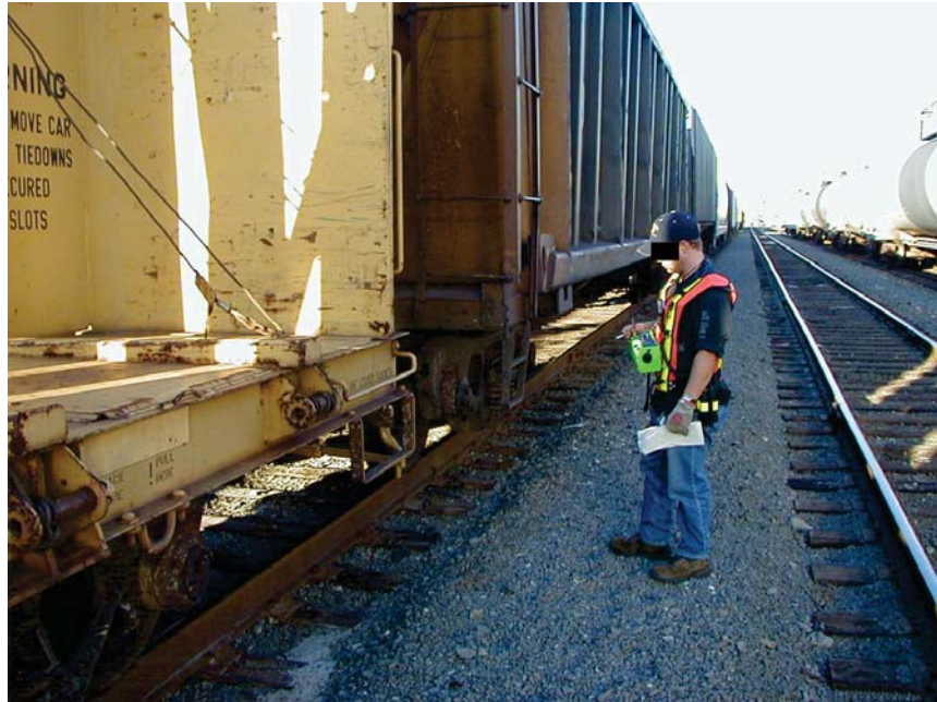
Figure 4. RCO making coupling
